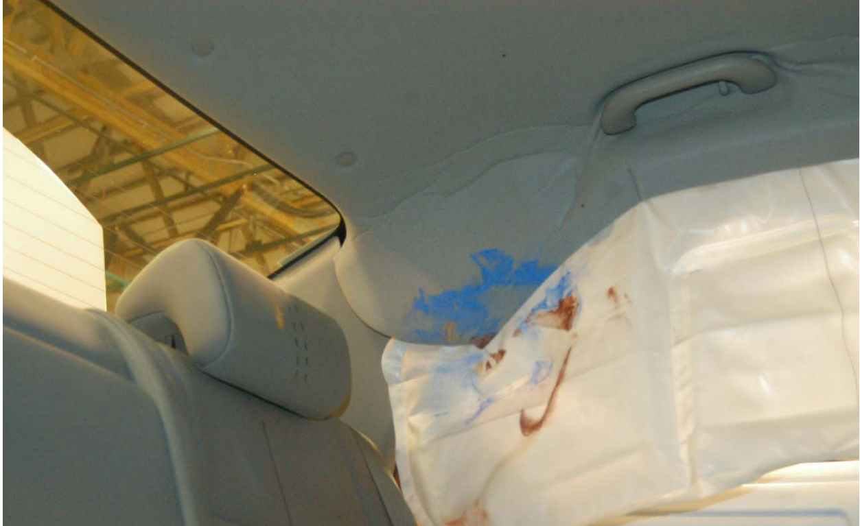
Figure A-73: Post-Test Rear Passenger Dummy Close-Up Head Contact with Vehicle View
