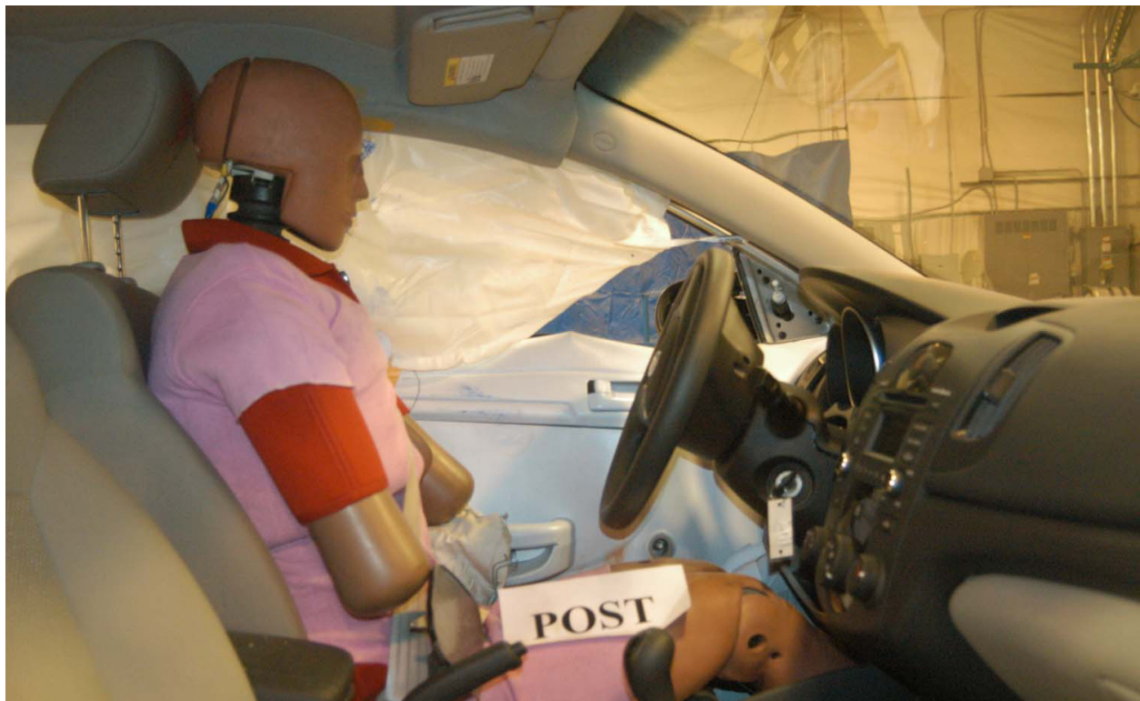
Figure A-44: Post-Test Right Side View of Driver Dummy and Front Seat of Occupant Compartment
