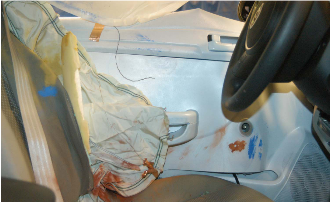
Figure A-49: Post-Test Driver Dummy Close-Up Torso Contact with Vehicle Interior View
