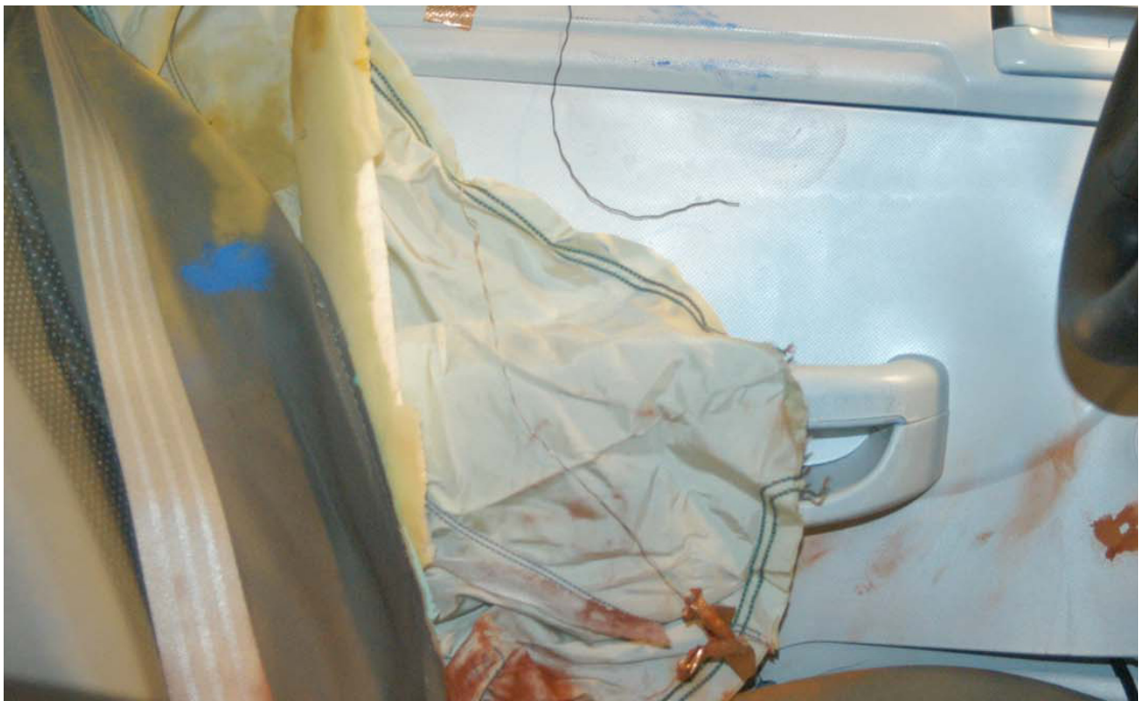
Figure A-50: Post-Test Driver Dummy Close-Up Torso Contact with Side Airbag View
