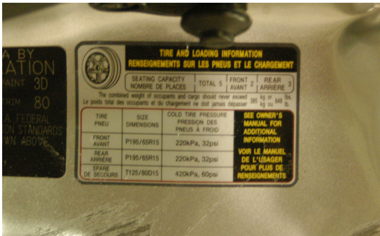
Figure A-89: Close-Up View of Vehicle's Certification Label
