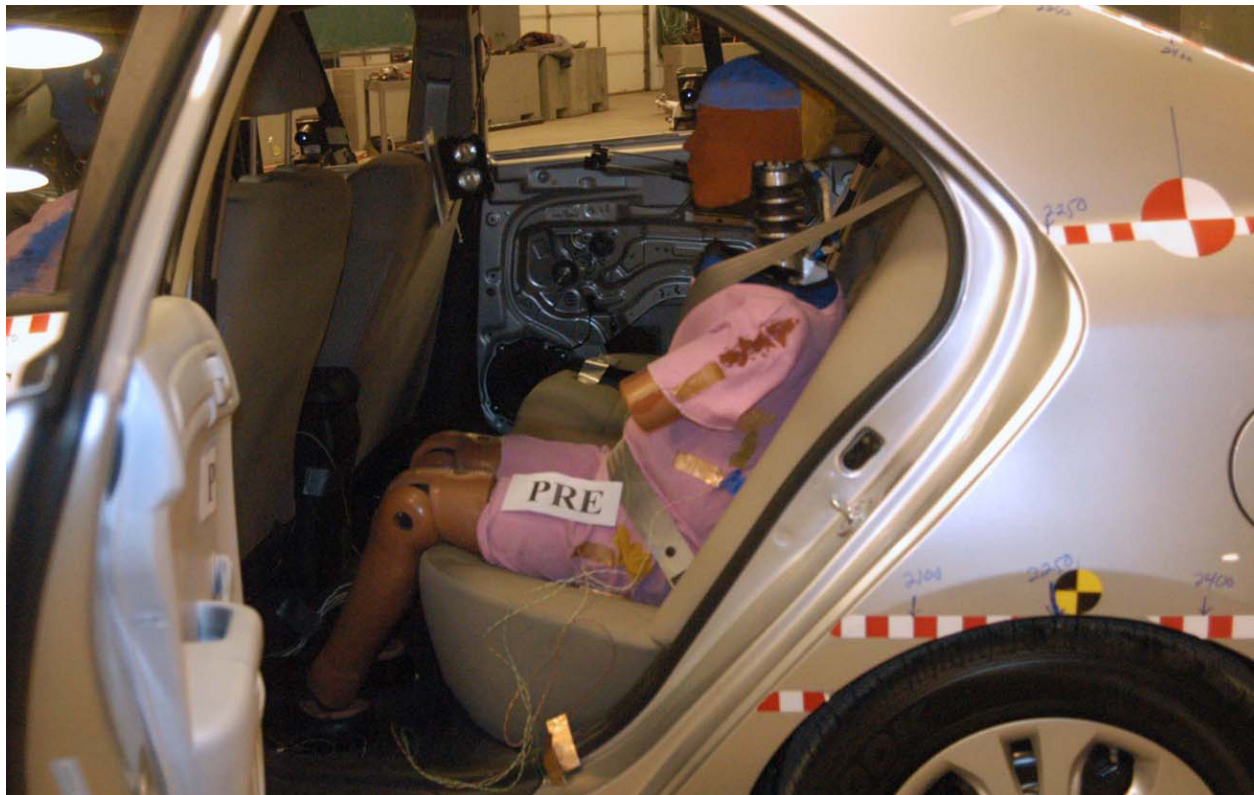
Figure A-53: Pre-Test Left Side View of Rear Passenger Dummy Showing Belt, Chalking, and Contact Switches
