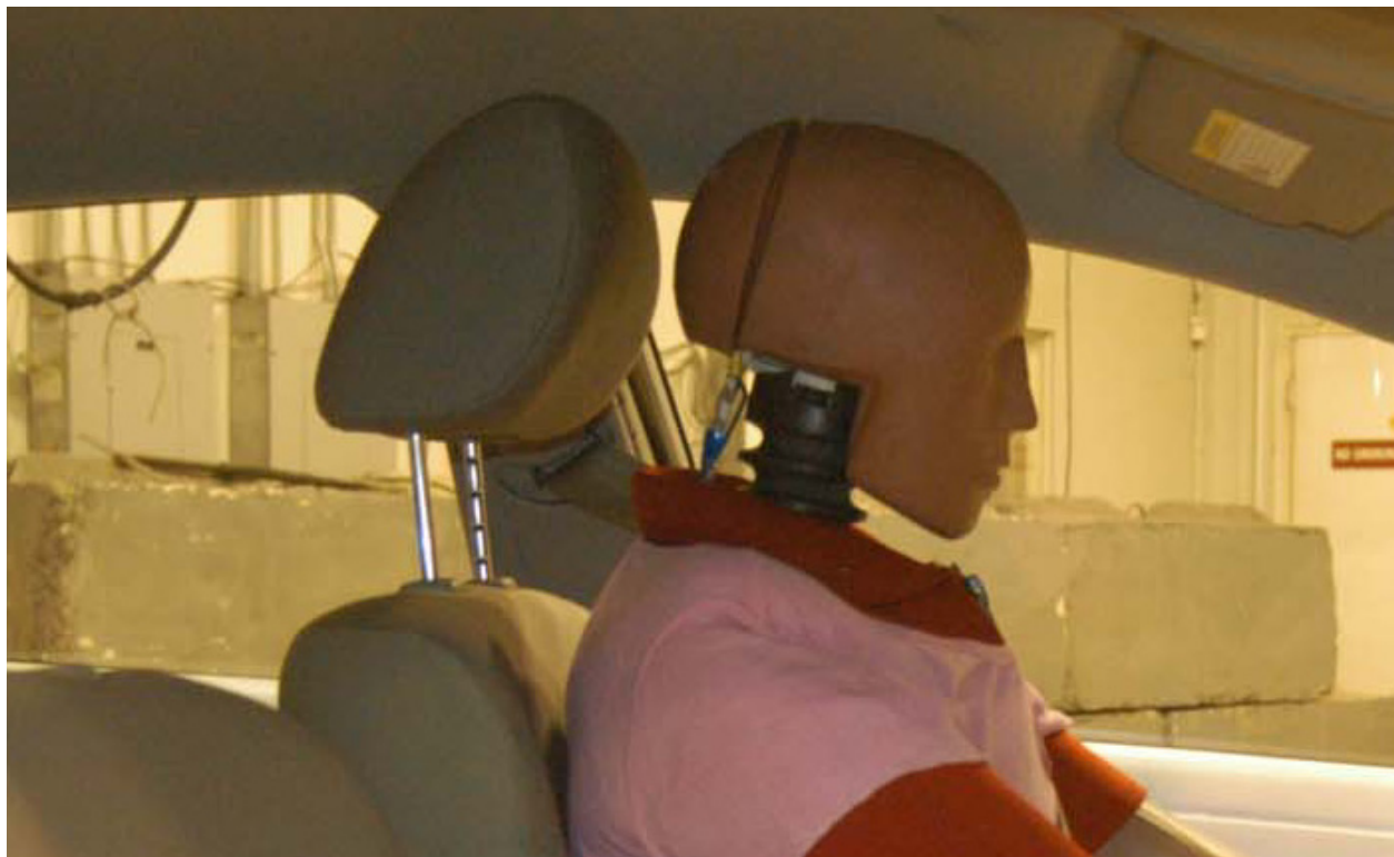
Figure A-40: Pre-Test Close-Up View of Head Restraint
