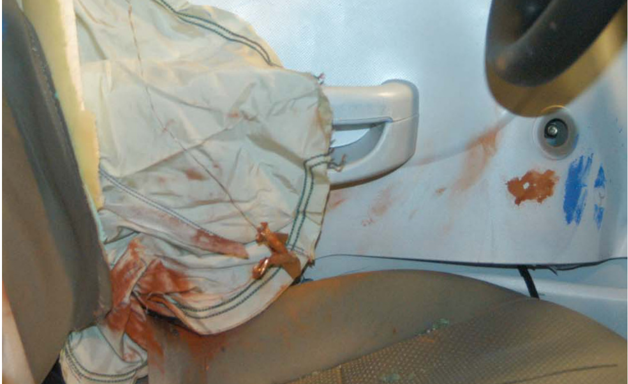
Figure A-51: Post-Test Driver Dummy Close-Up Pelvis Contact View
