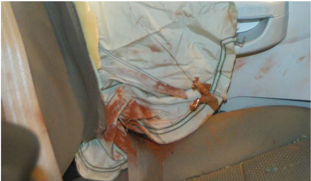
Figure A-52: Post-Test Driver Dummy Close-Up Pelvis Contact With Side Airbag View
