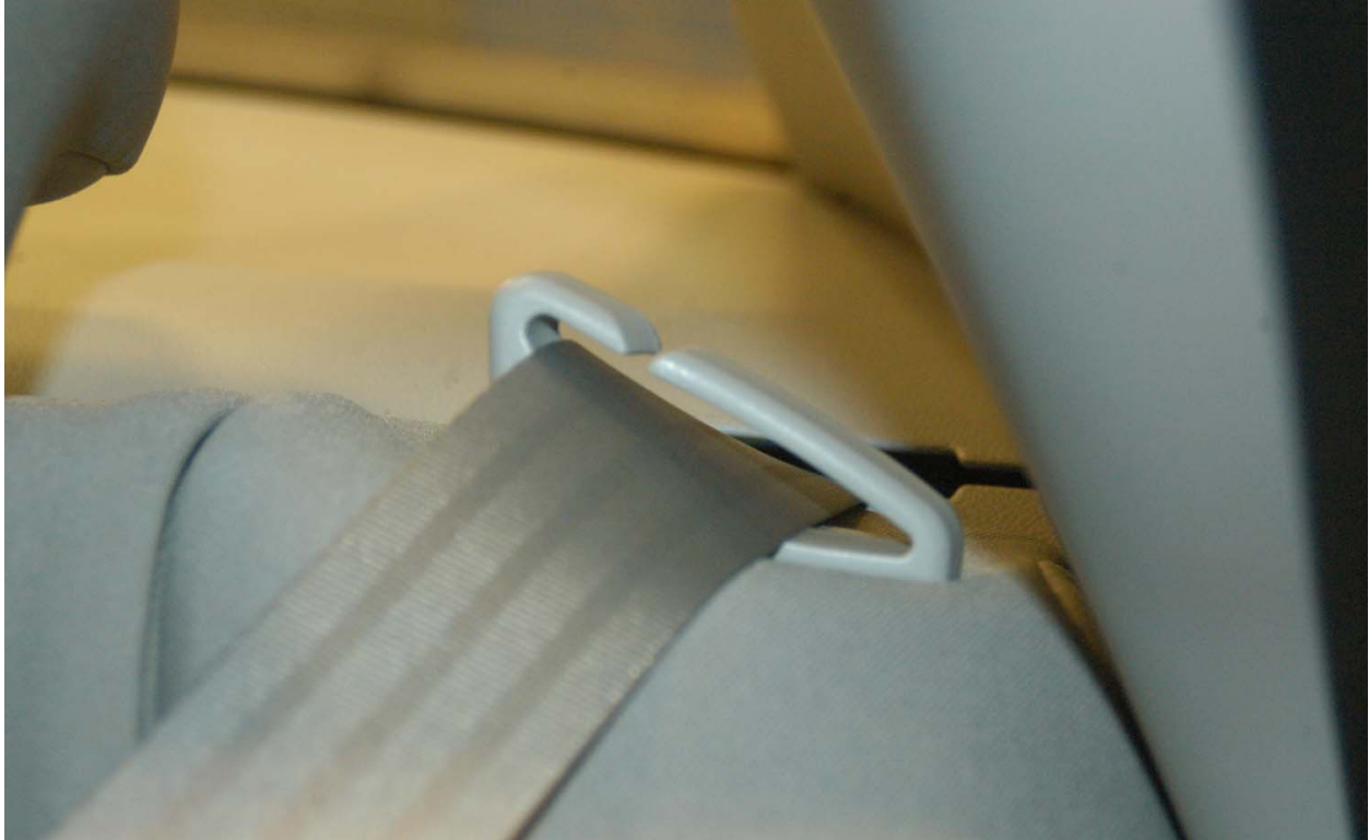
Figure A-63: Pre-Test View of Belt Anchorage for Rear Passenger Dummy
