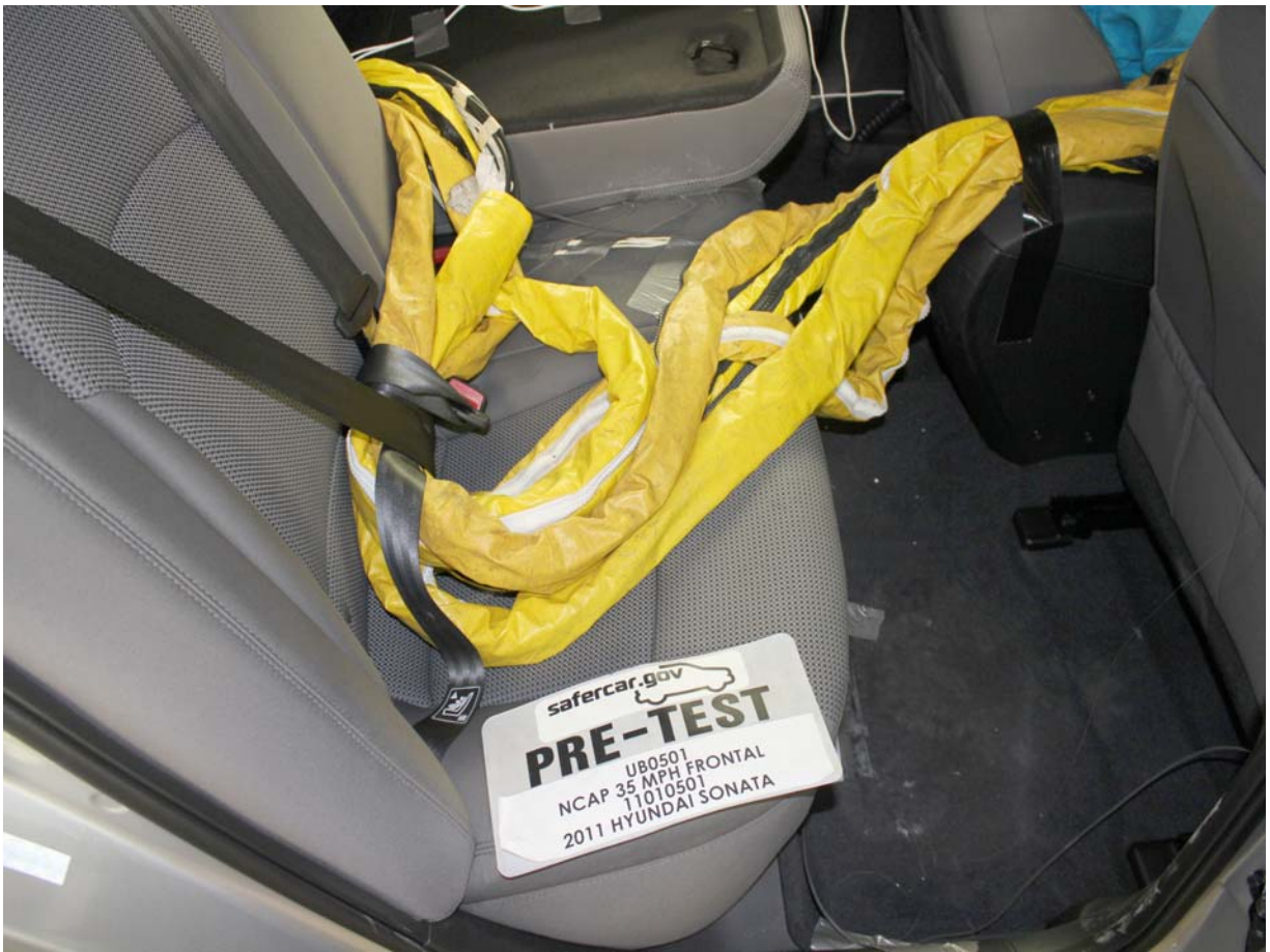
Pre-Test Dummy Cable Routing
