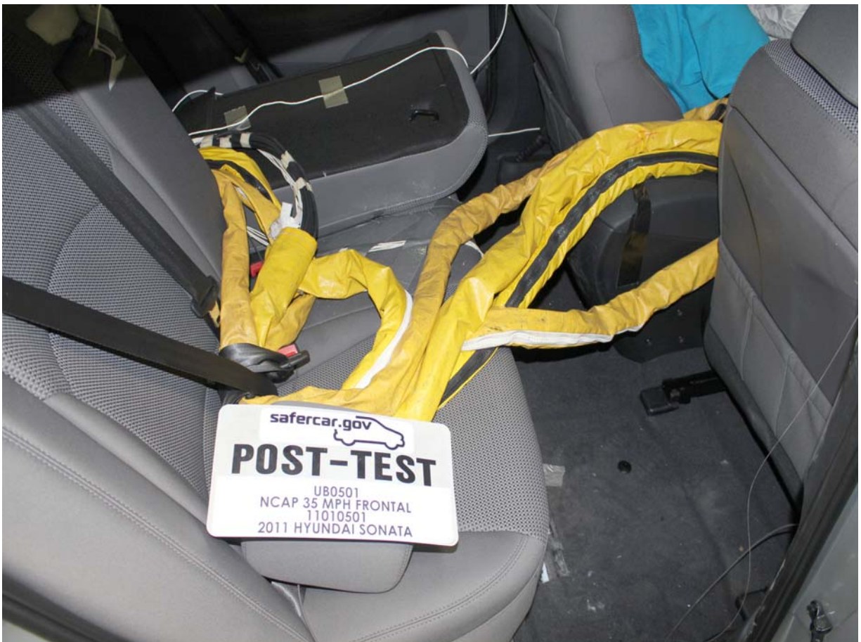
Post-Test Dummy Cable Routing
