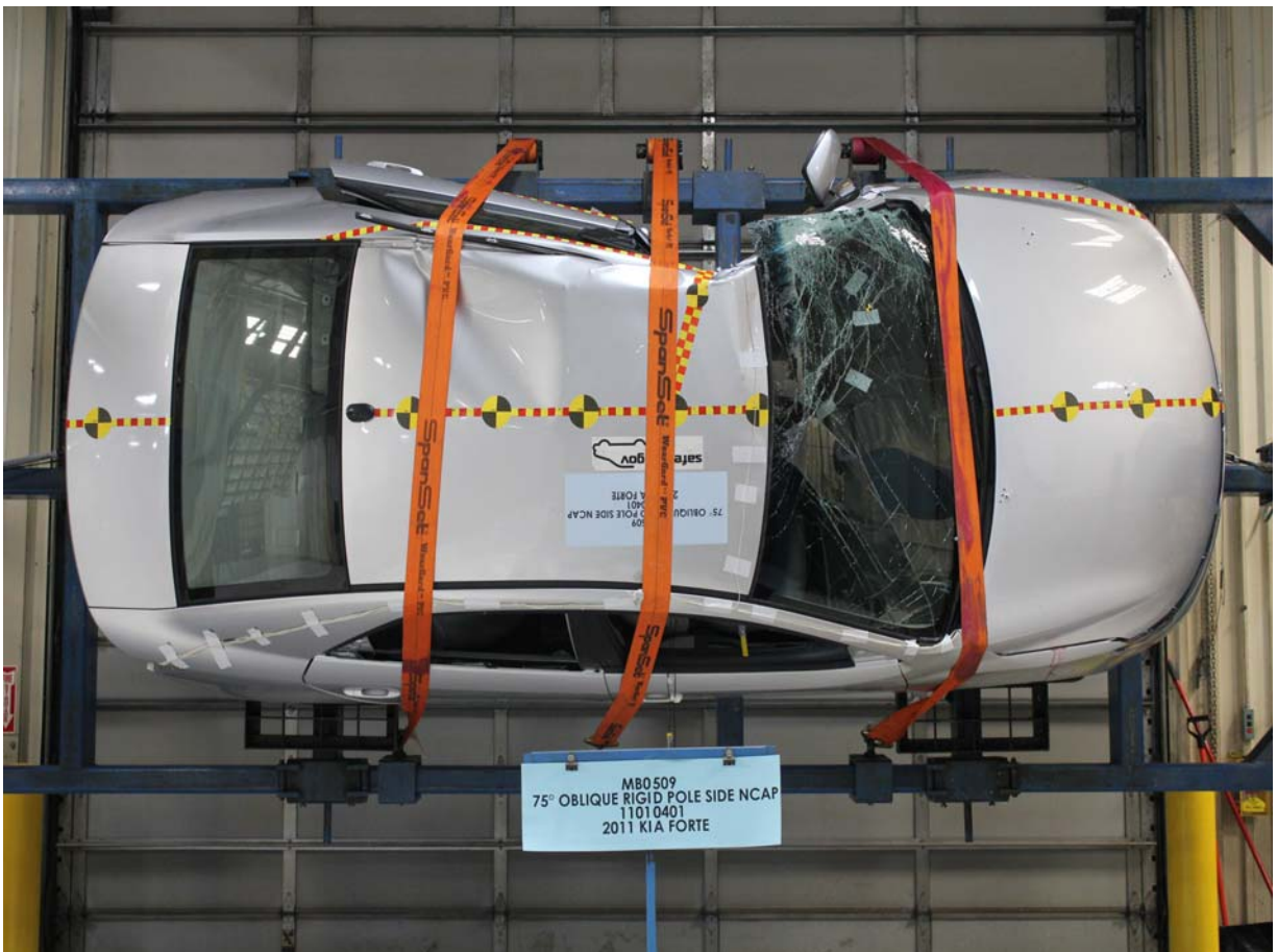
FMVSS No. 301/305 Rollover 270 Degrees
