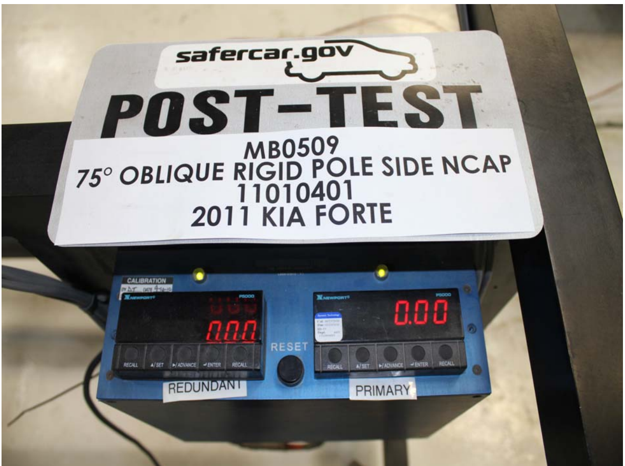
Post-Test Primary and Redundant Speed Trap Read-Out
