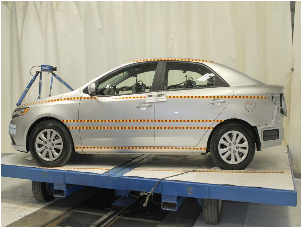
Pre-Test Left Side View of Test Vehicle
