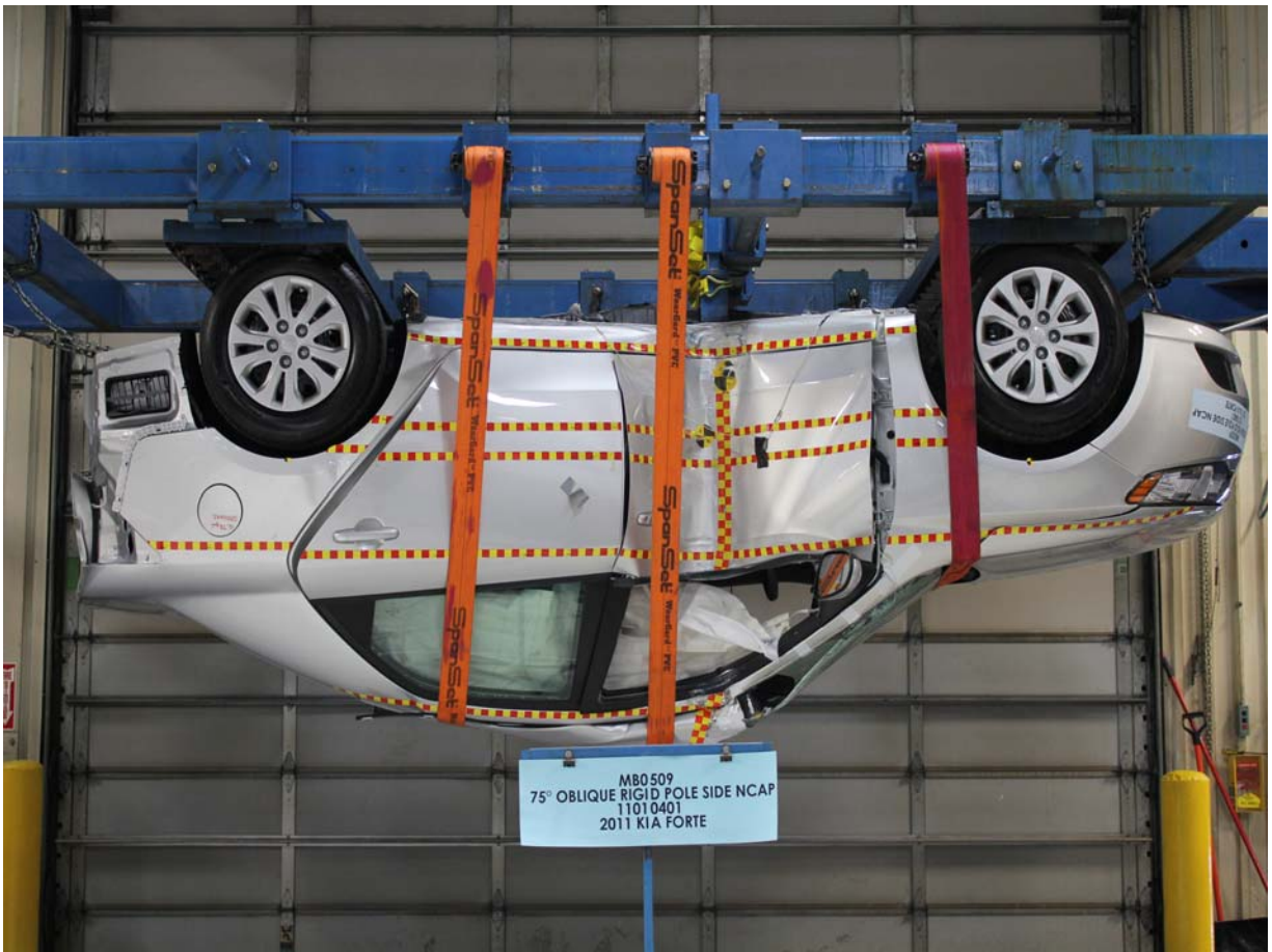
FMVSS No. 301/305 Rollover 180 Degrees
