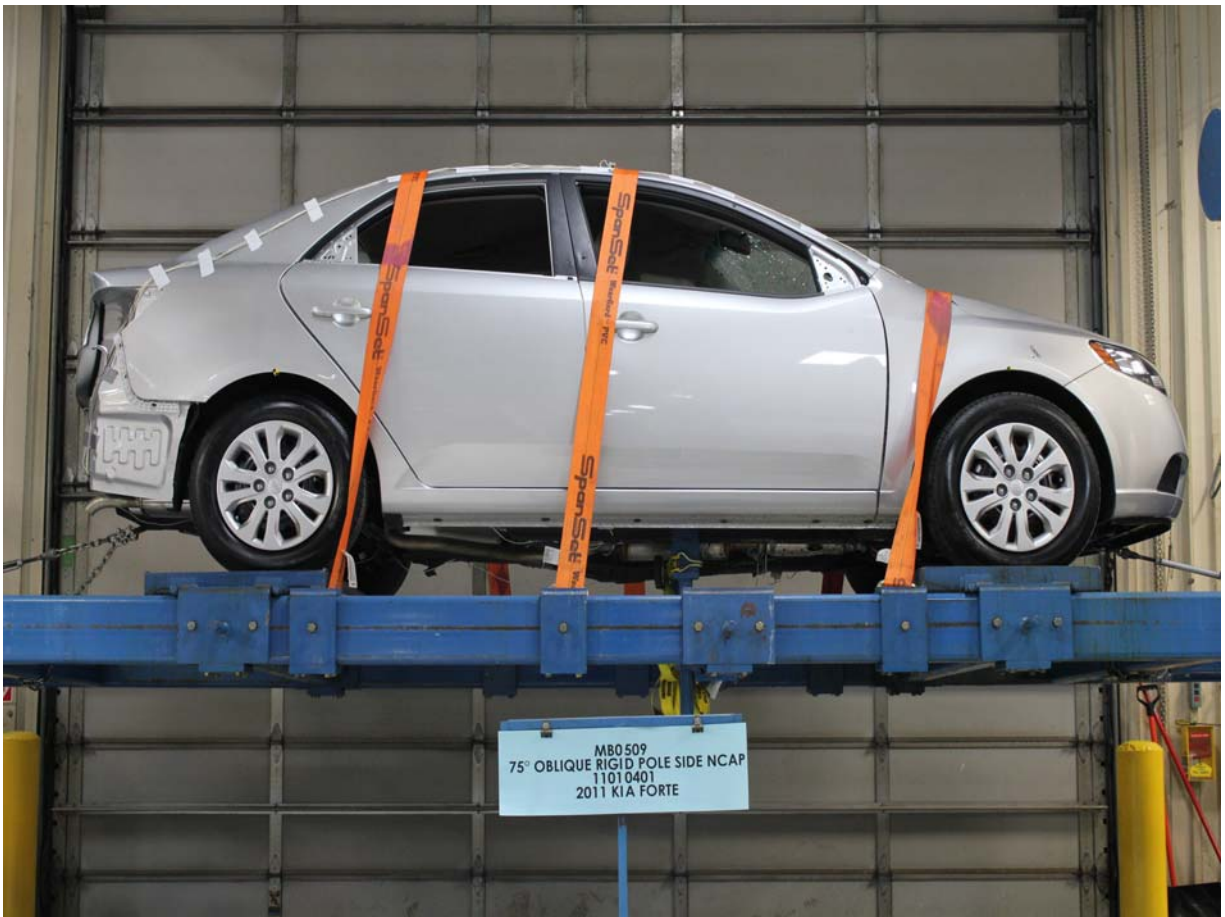
FMVSS No. 301/305 Rollover 0 Degrees
