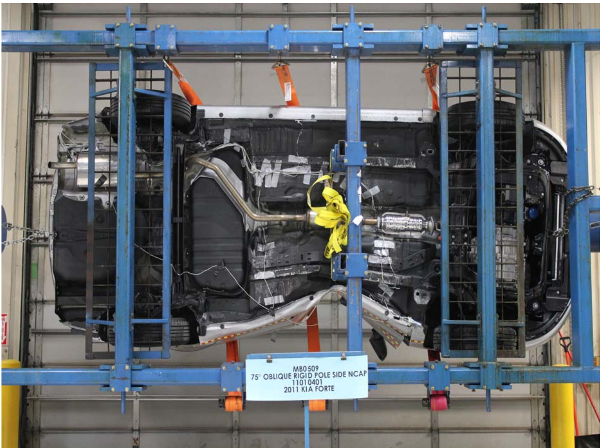
FMVSS No. 301/305 Rollover 90 Degrees
