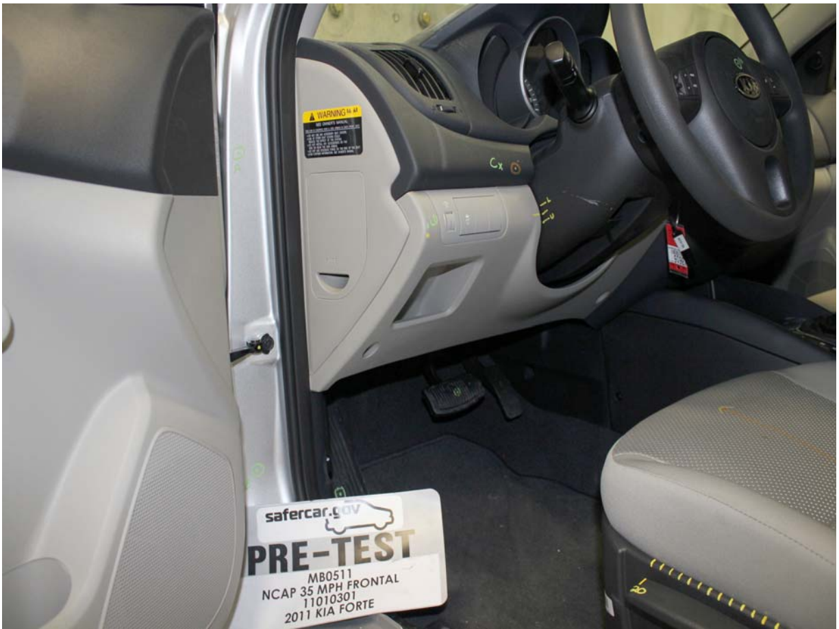
Pre-Test Driver's Side Knee Bolster (without dummy)
