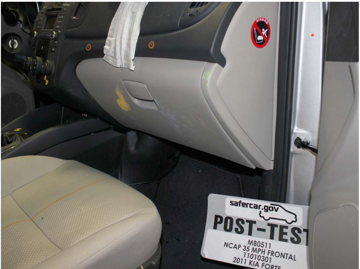
Post-Test Passenger's Side Knee Bolster (without dummy)
