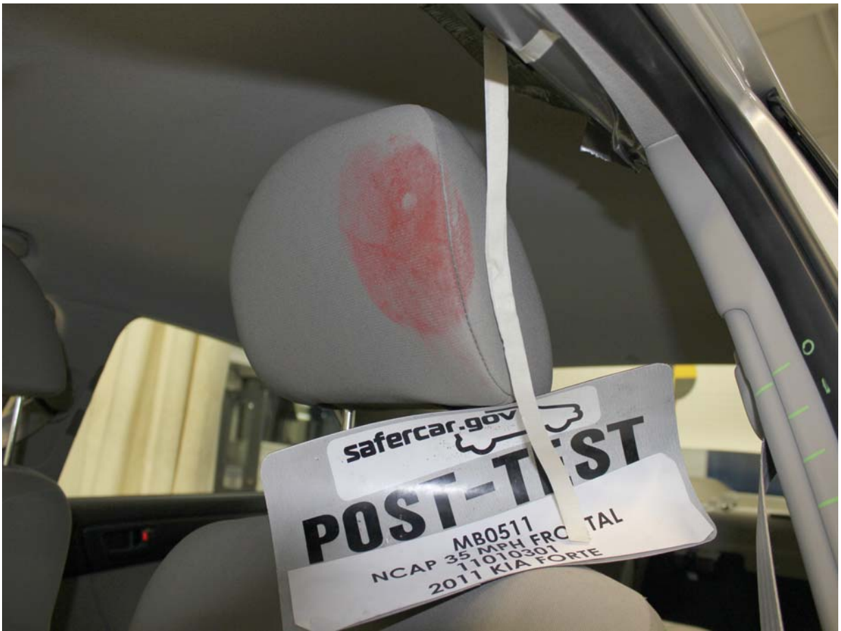
Post-Test Driver Dummy Contact with Headrest
