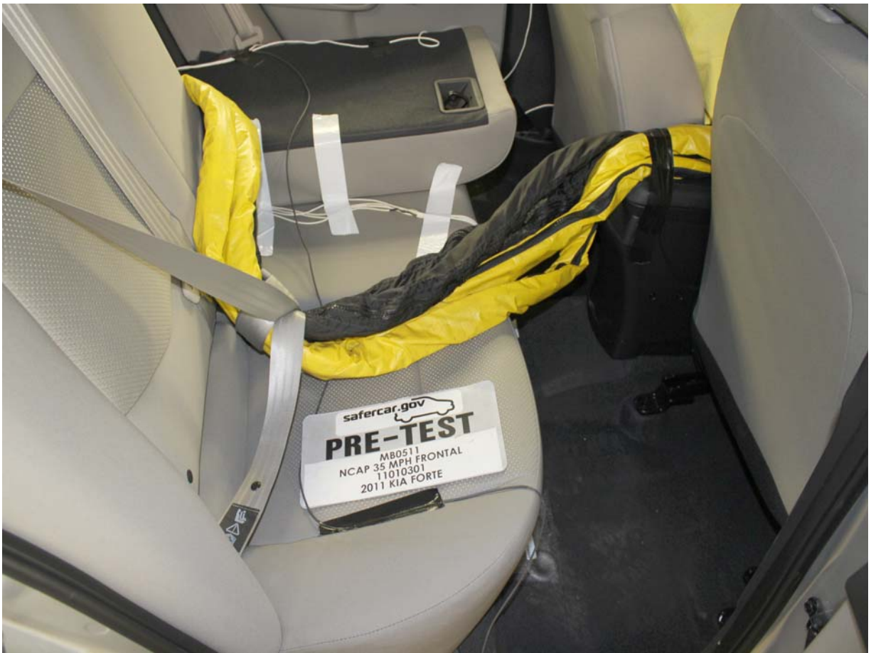
Pre-Test Dummy Cable Routing
