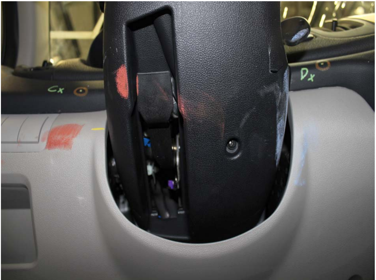
Post-Test Driver Dummy Contact with Knee Bolster
