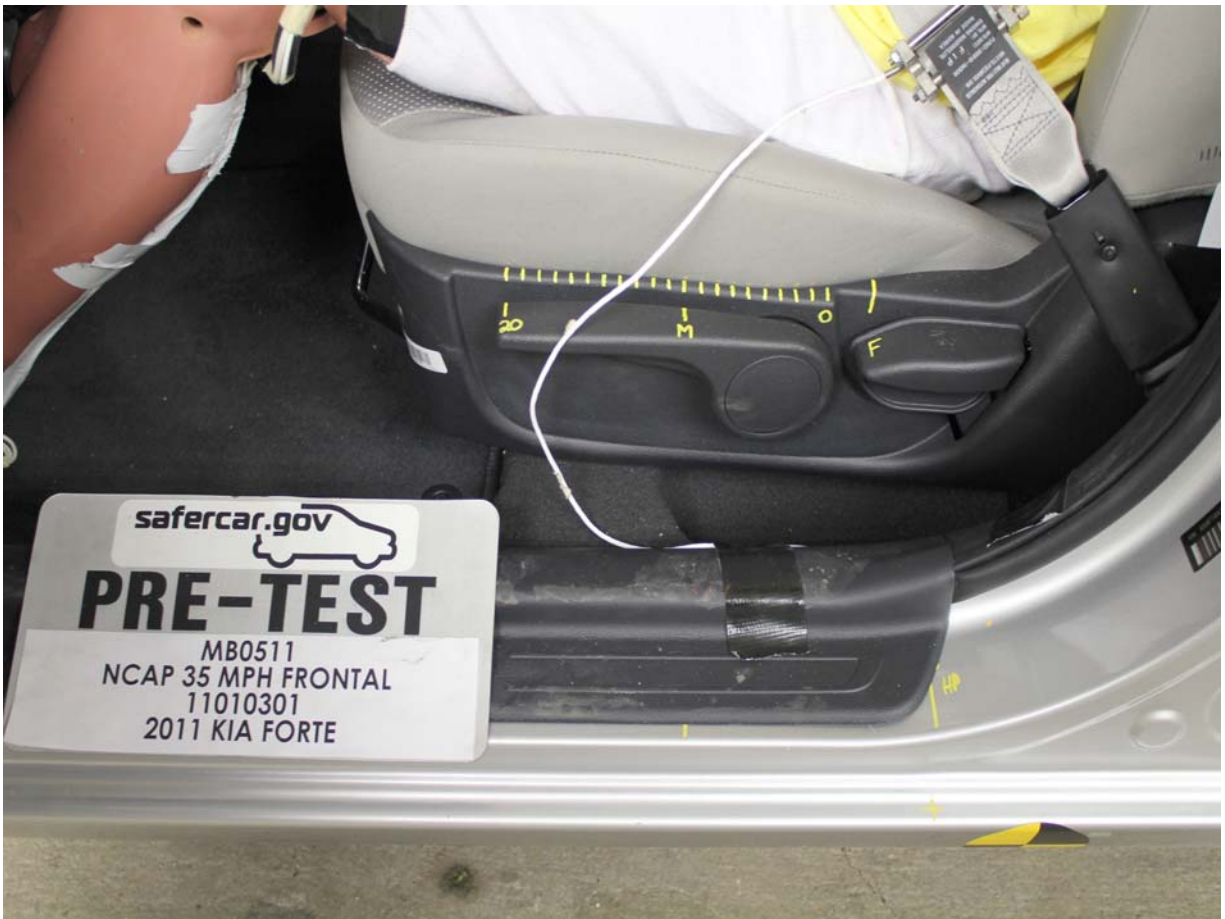
Pre-Test Driver's Seat Fore-Aft Markings
