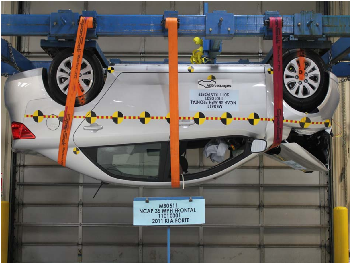
Vehicle at 180 Degrees on Static Rollover Device
