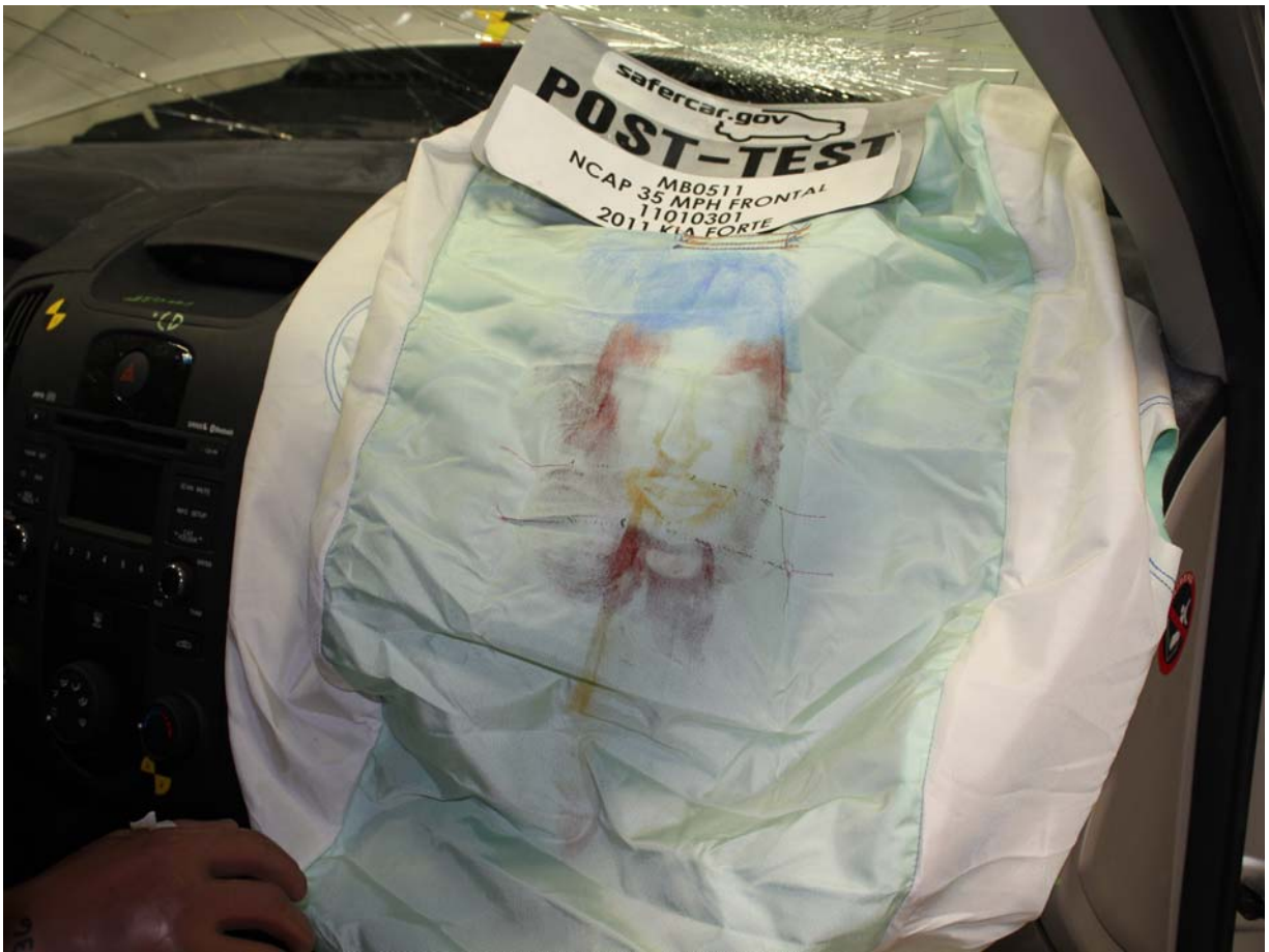
Post-Test Passenger Dummy Contact with Airbag
