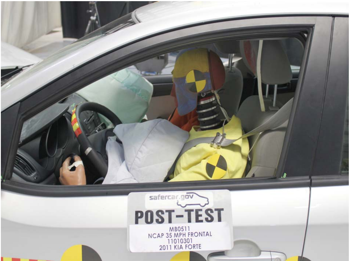
Post-Test Driver Dummy Window View
