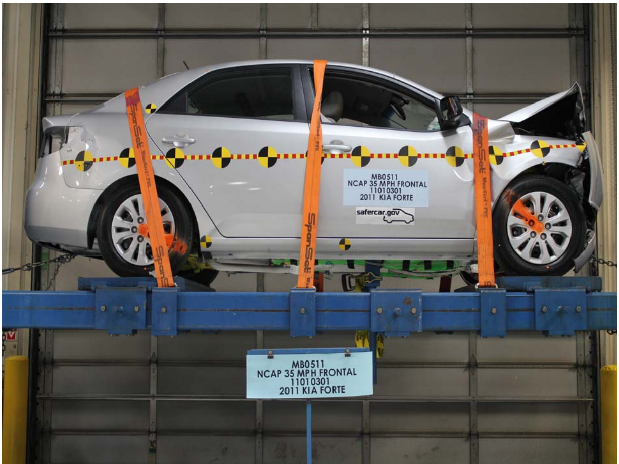
Vehicle at 0 Degrees on Static Rollover Device
