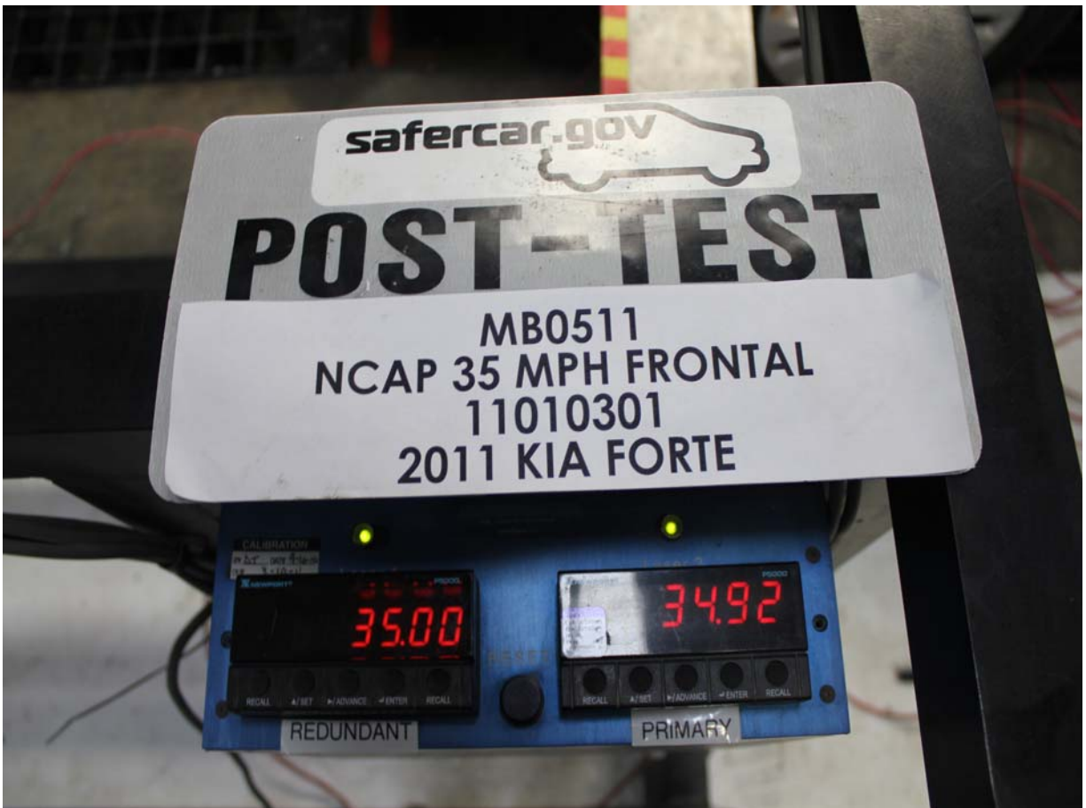
Post-Test Speed Trap Read-Out
