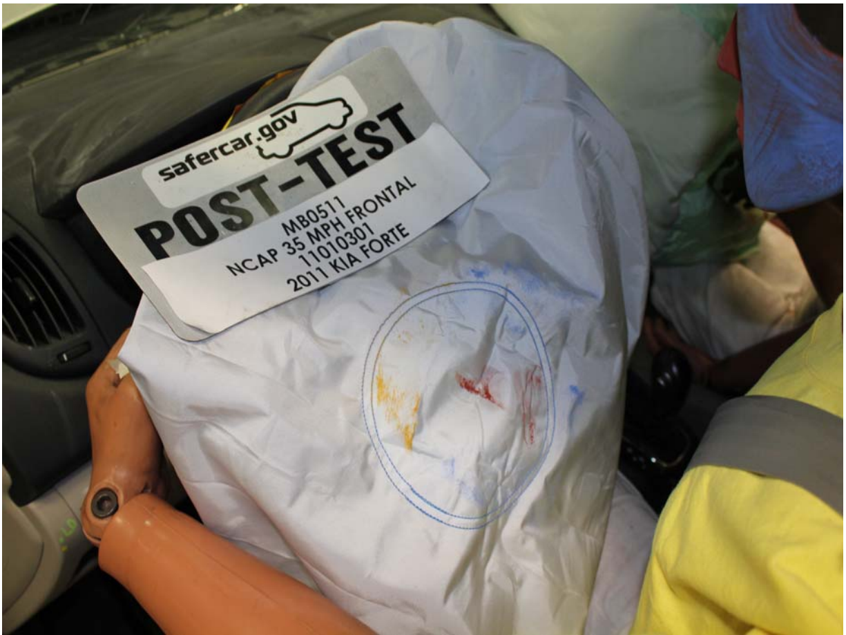
Post-Test Driver Dummy Contact with Airbag
