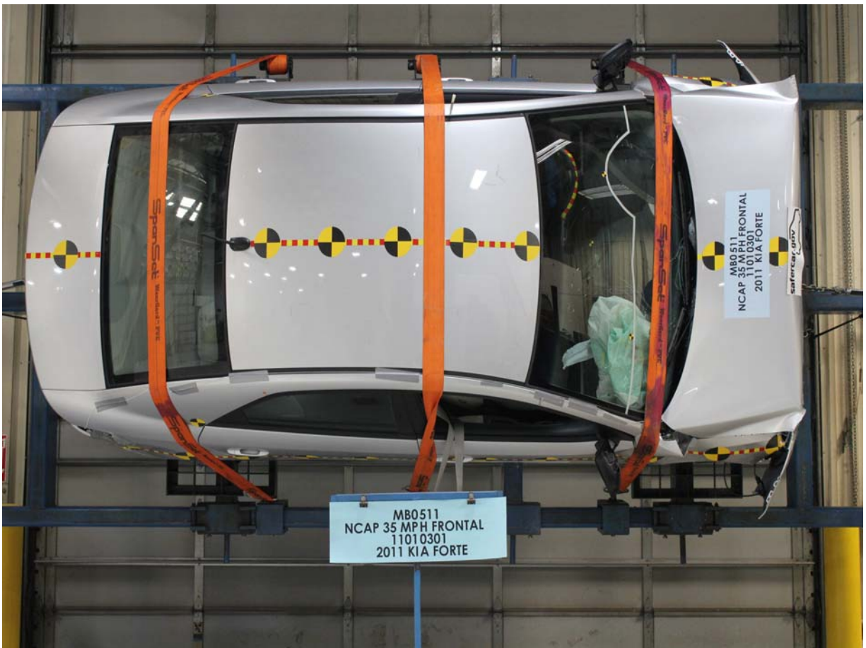
Vehicle at 270 Degrees on Static Rollover Device
