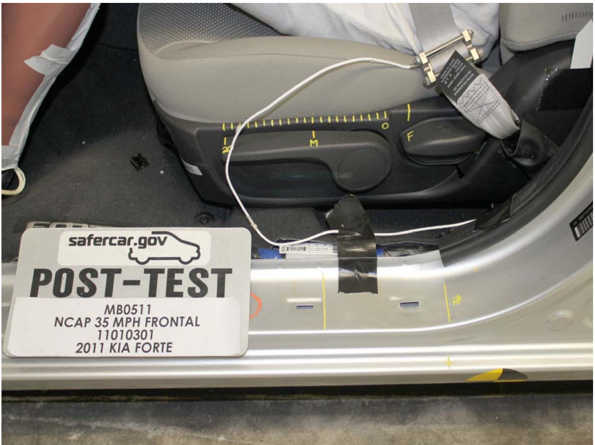
Post-Test Driver's Seat Fore-Aft Markings
