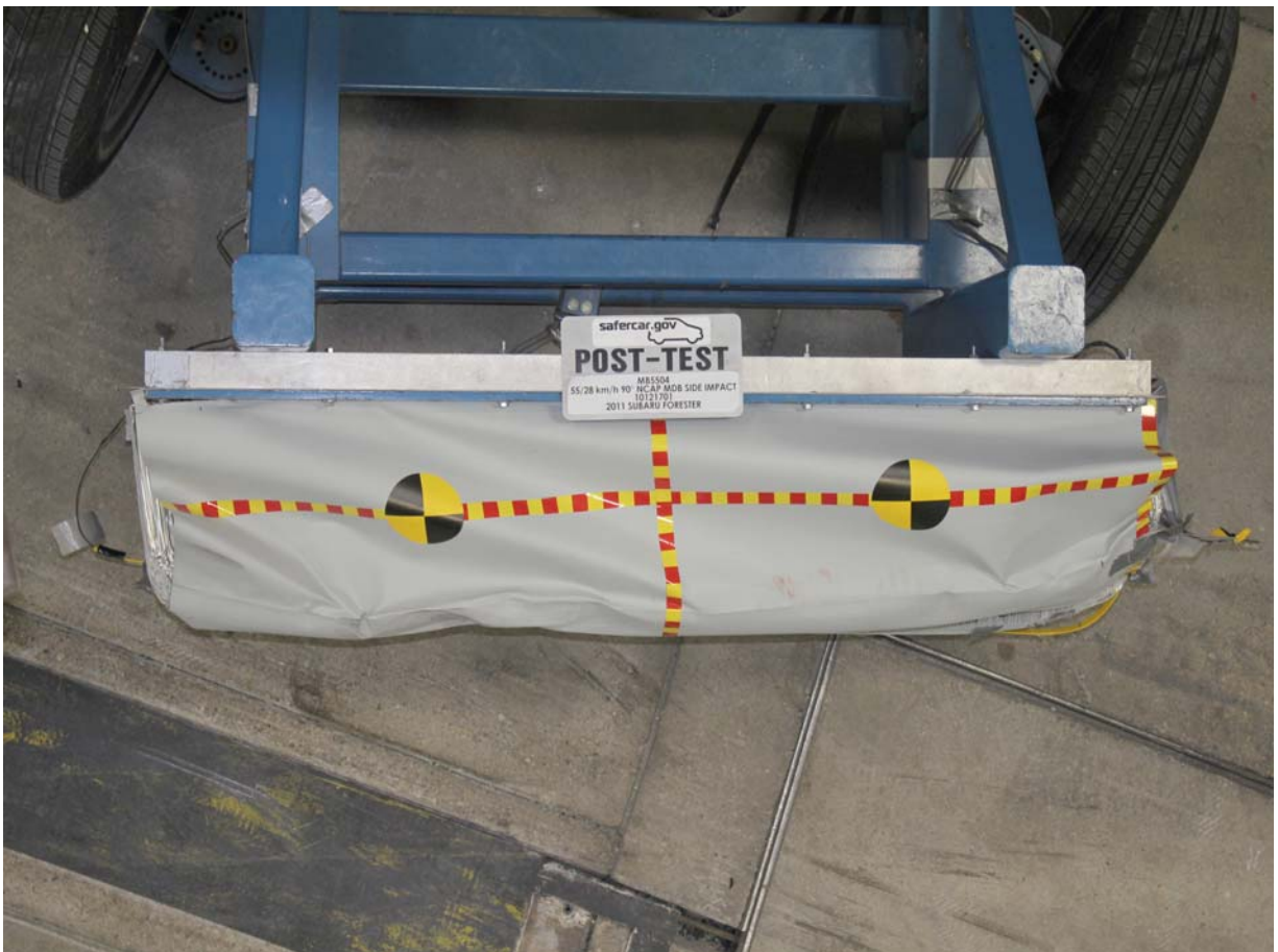
Post-Test Top View of MDB Impactor Face
