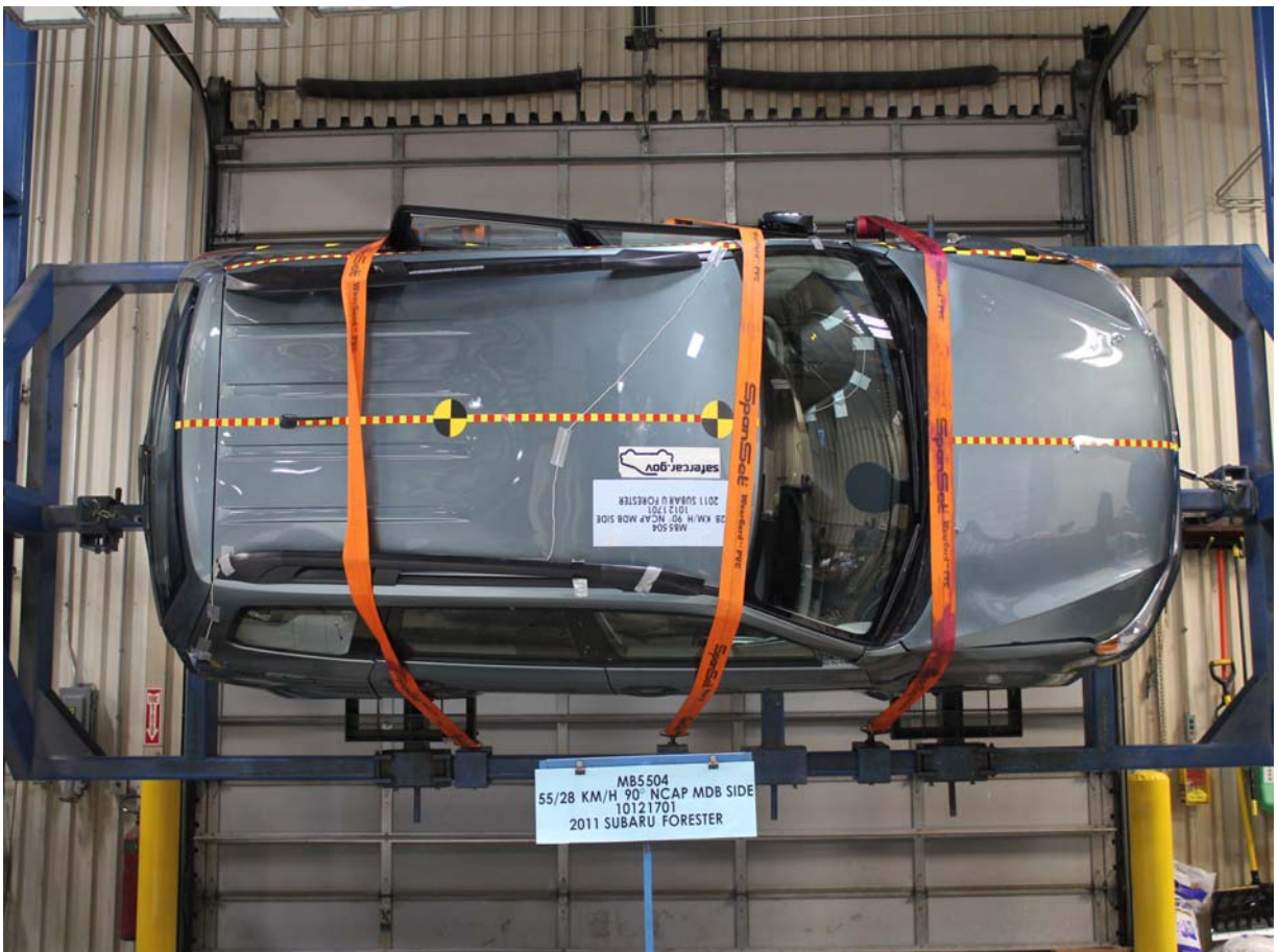
FMVSS No. 301/305 Rollover 90 Degrees
