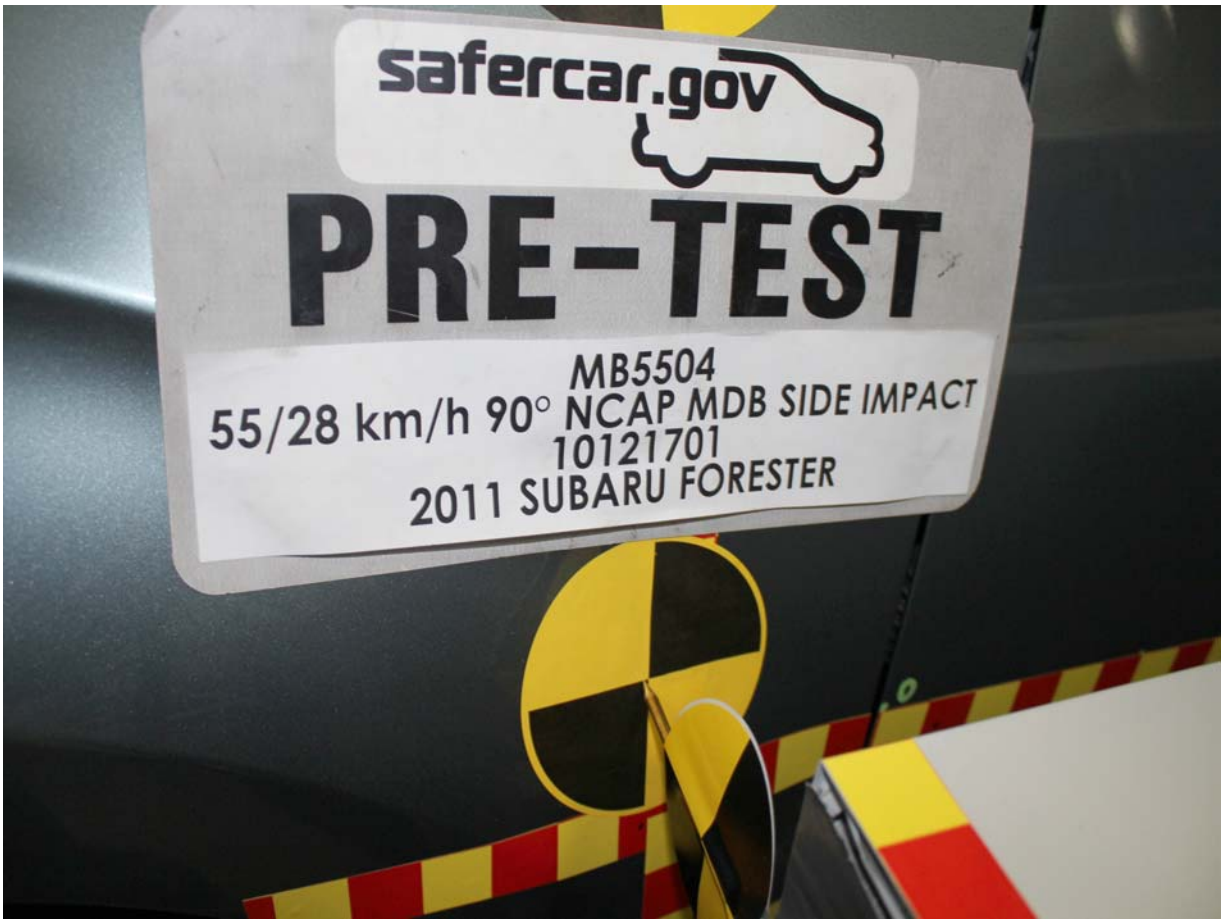
Pre-Test Close-Up View of Impact Point Target
