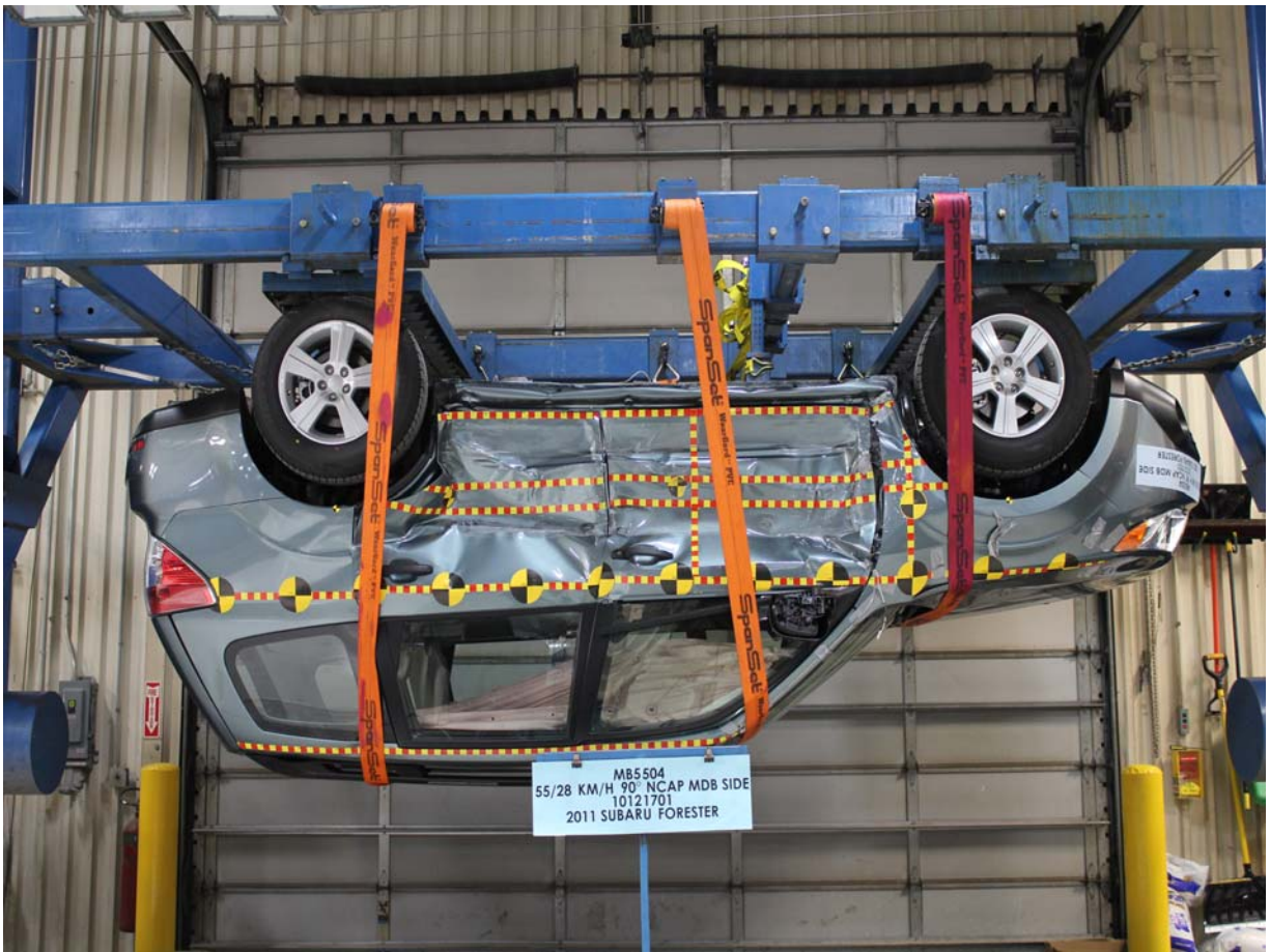
FMVSS No. 301/305 Rollover 180 Degrees
