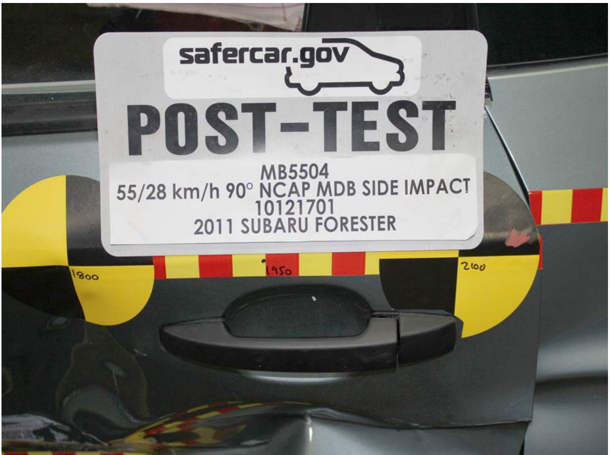
Post-Test Left Rear Door Latch Close-Up
