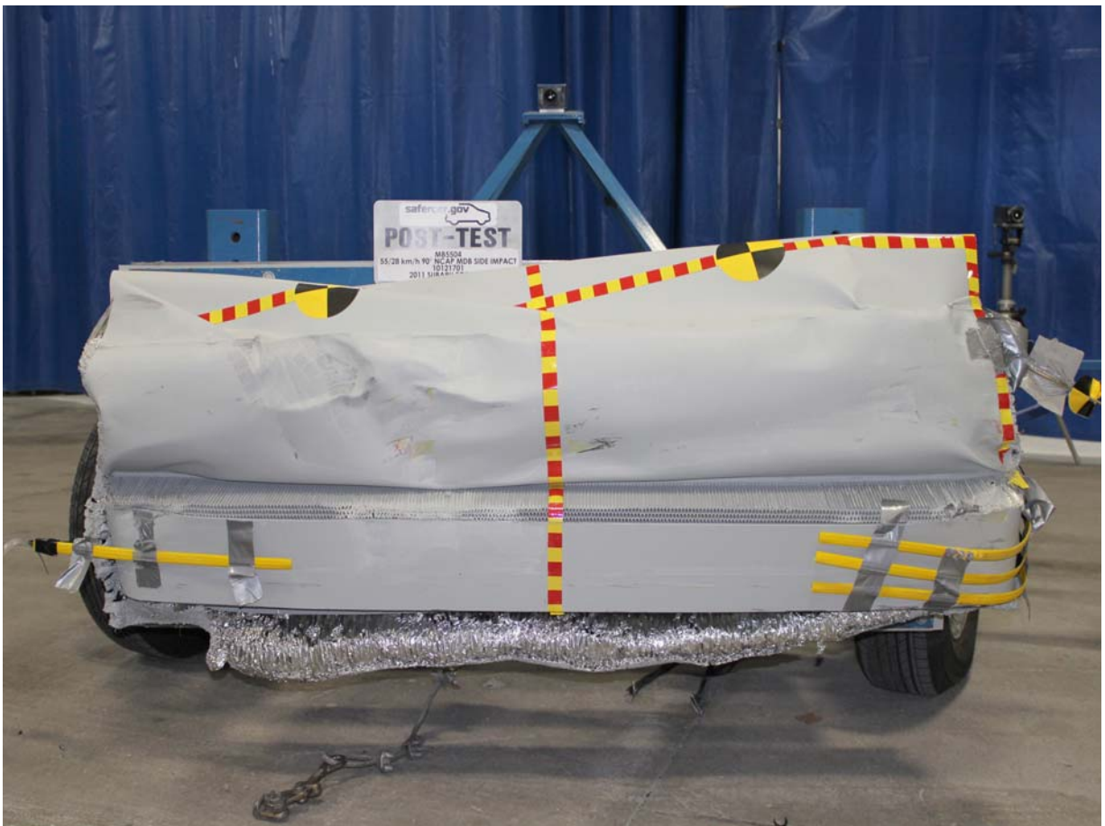
Post-Test Front View of MDB Impactor Face
