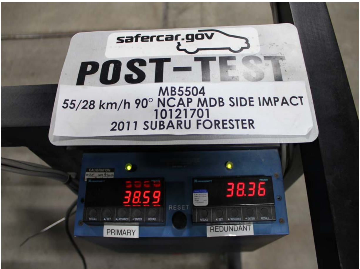
Post-Test Primary and Redundant Speed Trap Read-Out
