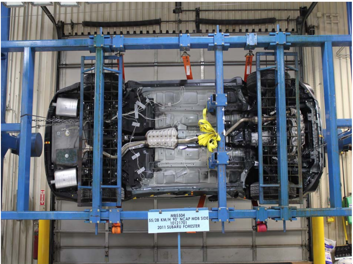
FMVSS No. 301/305 Rollover 270 Degrees
