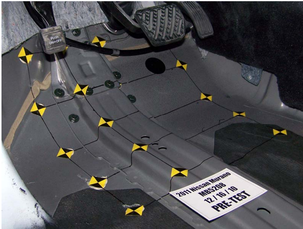
FIGURE 41. Pre-Test Driver's Side Floorpan
