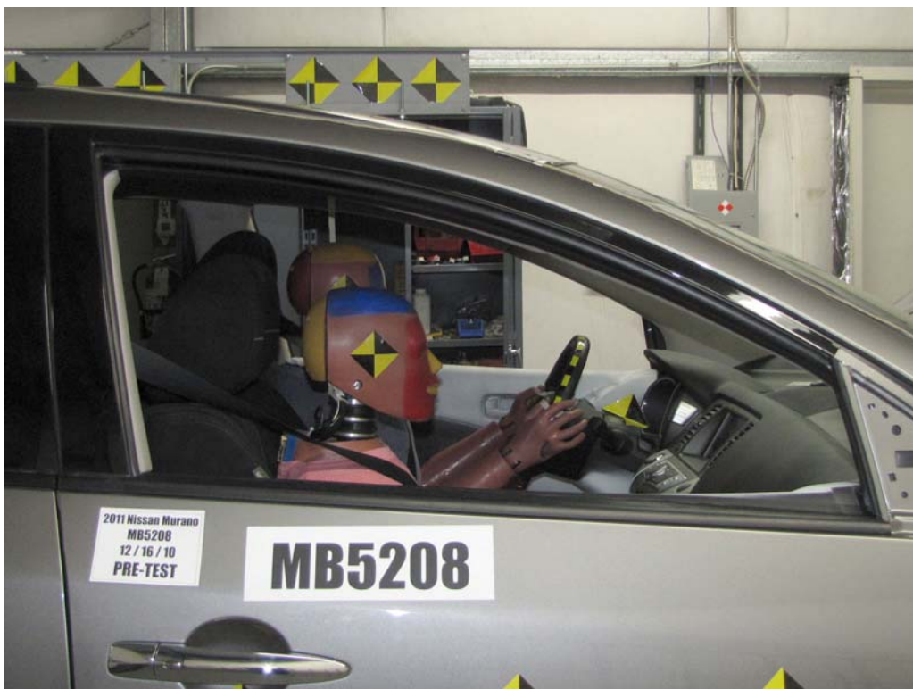
FIGURE 48. Pre-Test Passenger Dummy Window View
