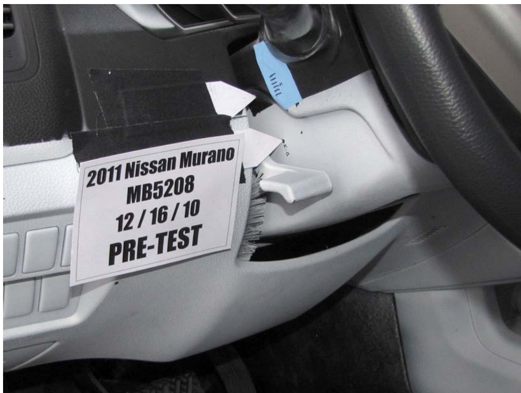
FIGURE 44. Pre-Test View of Steering Column Shear Capsule
