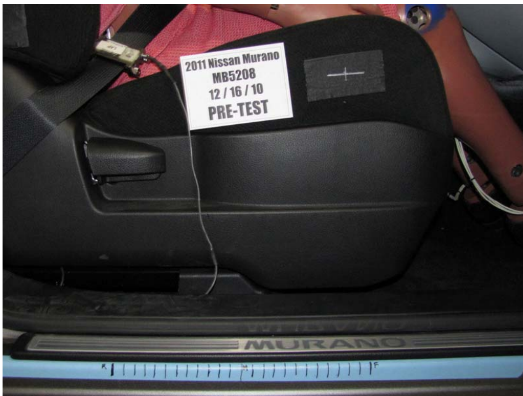
FIGURE 52. Pre-Test Passenger's Seat Fore-Aft Markings
