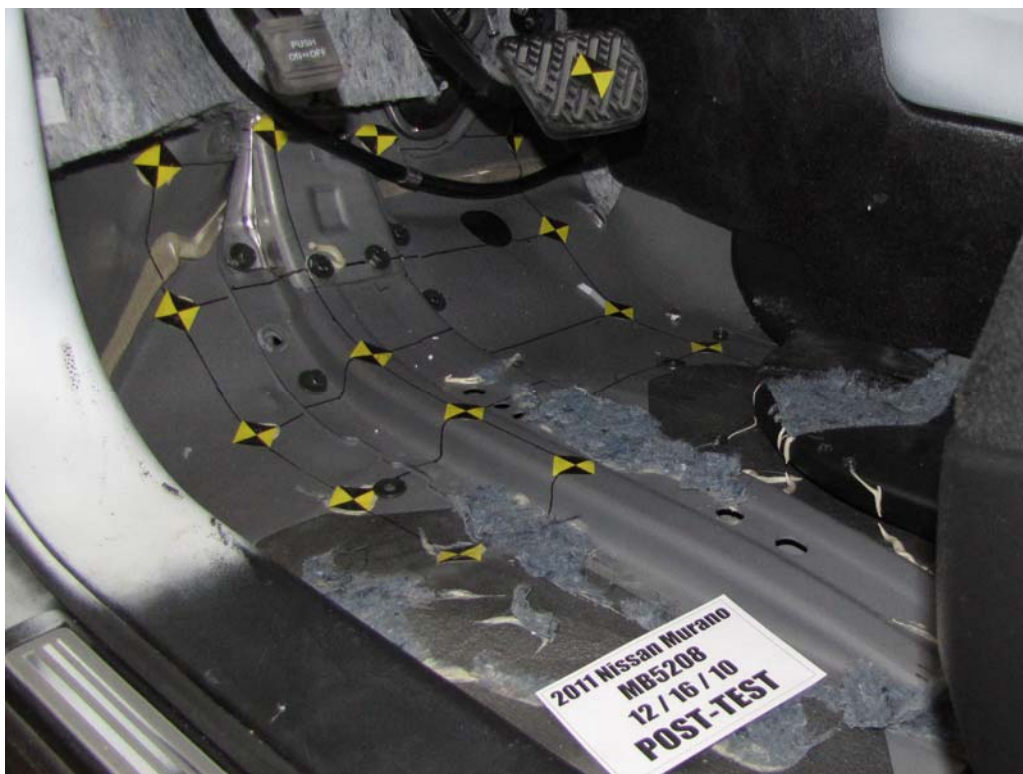
FIGURE 42. Post-Test Driver's Side Floorpan
