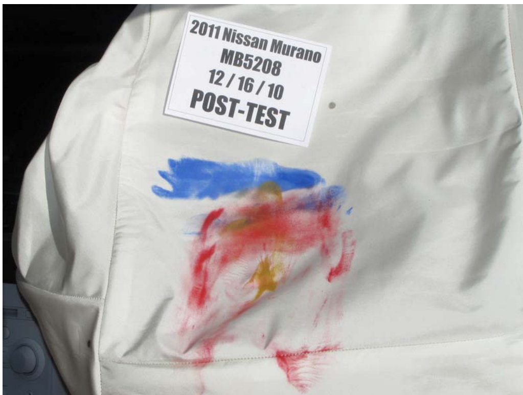
FIGURE 60. Post-Test Passenger Dummy Contact With Airbag
