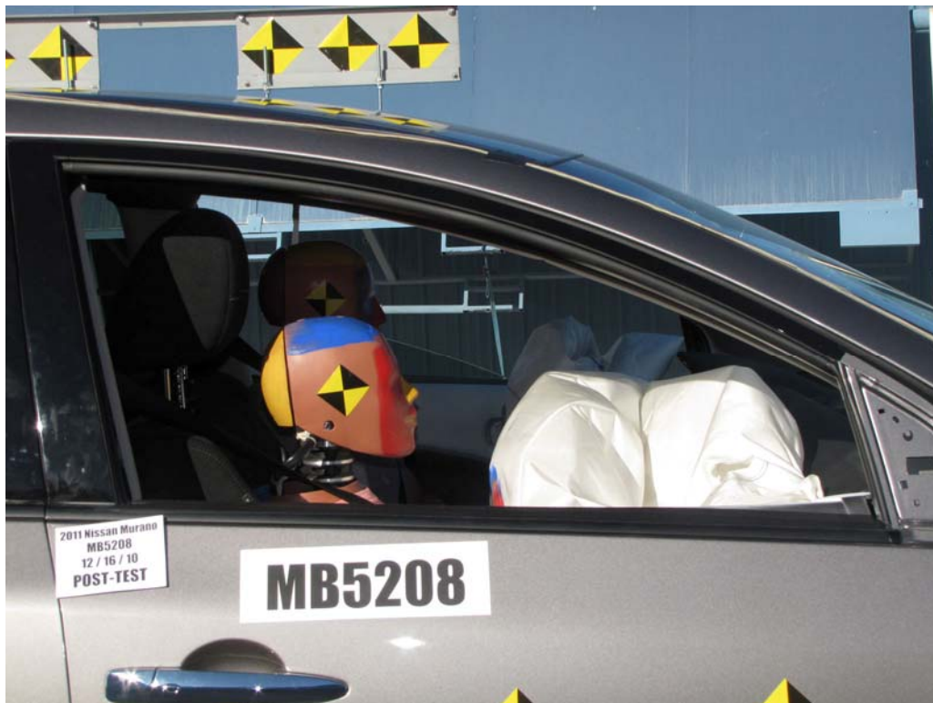
FIGURE 49. Post-Test Passenger Dummy Window View
