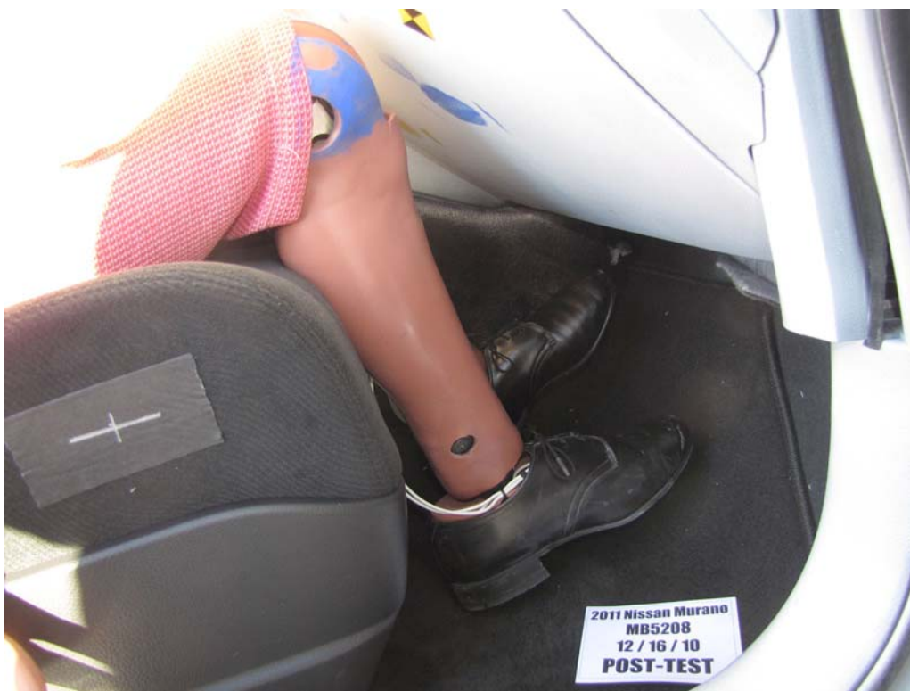
FIGURE 55. Post-Test Passenger Dummy Feet
