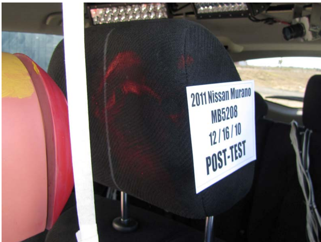
FIGURE 43a. Post-Test Driver Dummy Contact With Headrest
