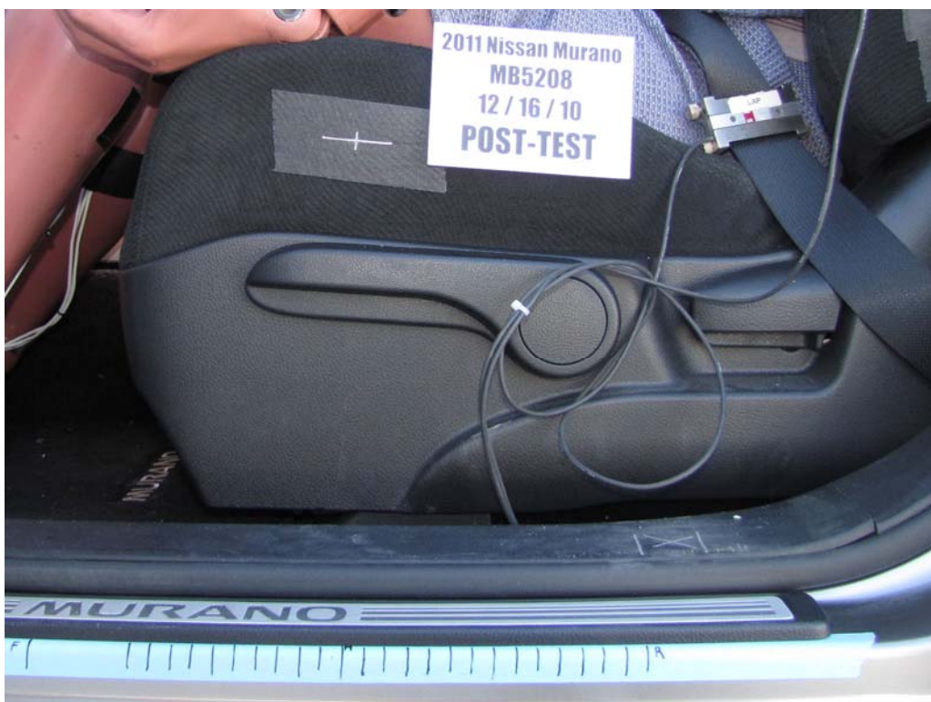
FIGURE 36. Post-Test Driver's Seat Fore-Aft Markings
