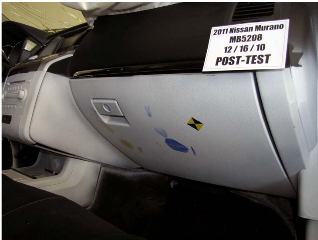
FIGURE 57. Post-Test Passenger's Side Knee Bolster
