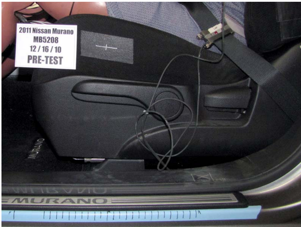
FIGURE 35. Pre-Test Driver's Seat Fore-Aft Markings
