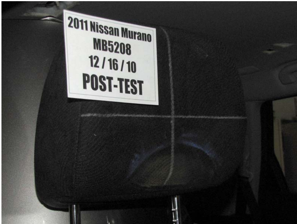
FIGURE 60a. Post-Test Passenger Dummy Contact With Headrest
