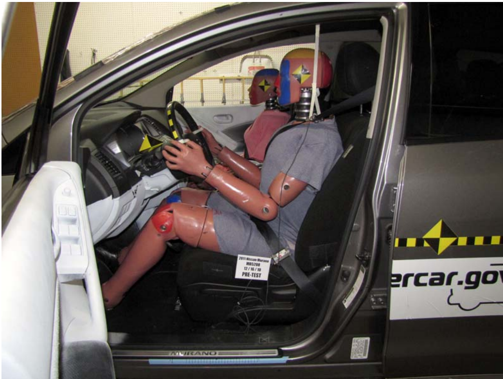
FIGURE 33. Pre-Test Driver Dummy and Vehicle Interior View
