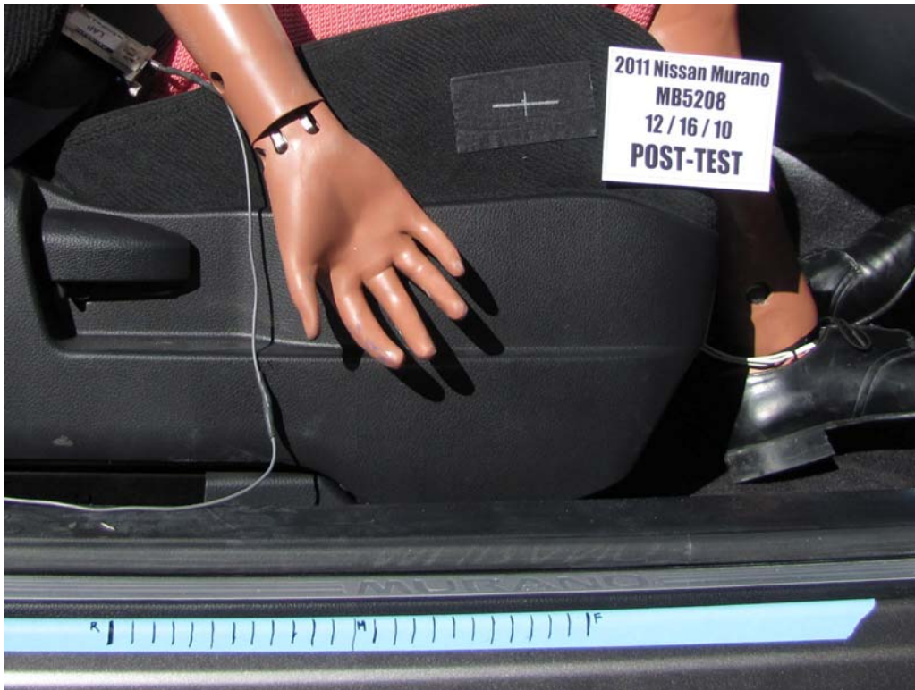
FIGURE 53. Post-Test Passenger's Seat Fore-Aft Markings
