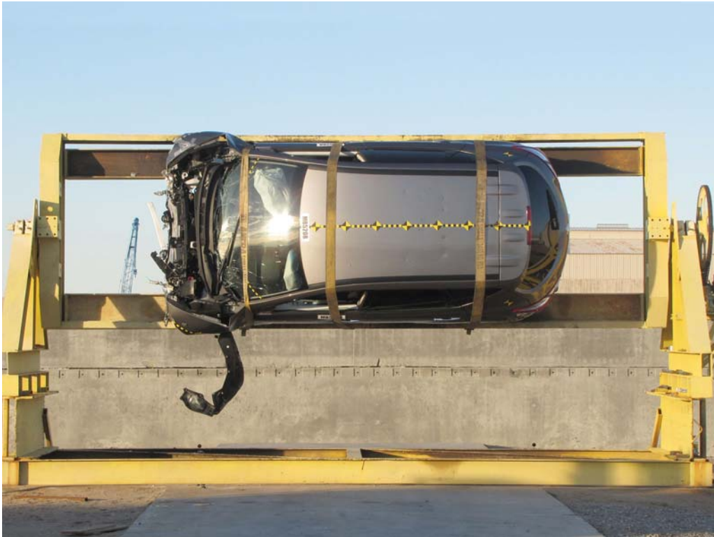
FIGURE 65. Vehicle at 90°on Static Rollover Device
