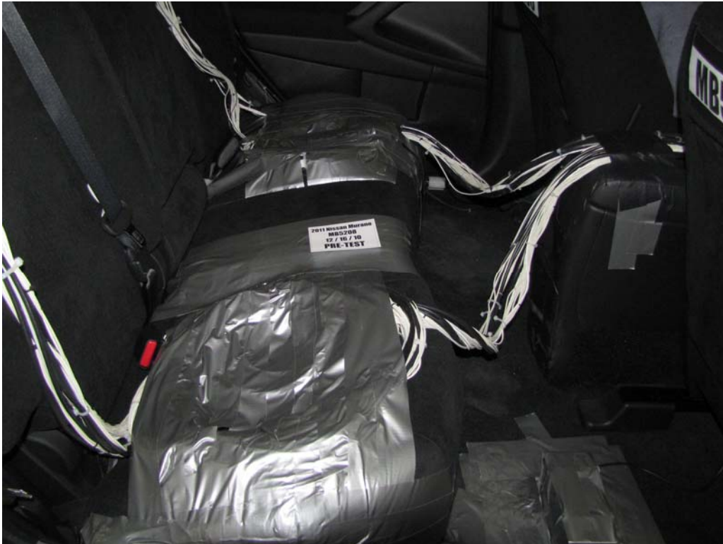
FIGURE 27. Pre-Test Dummy Cable Routing
