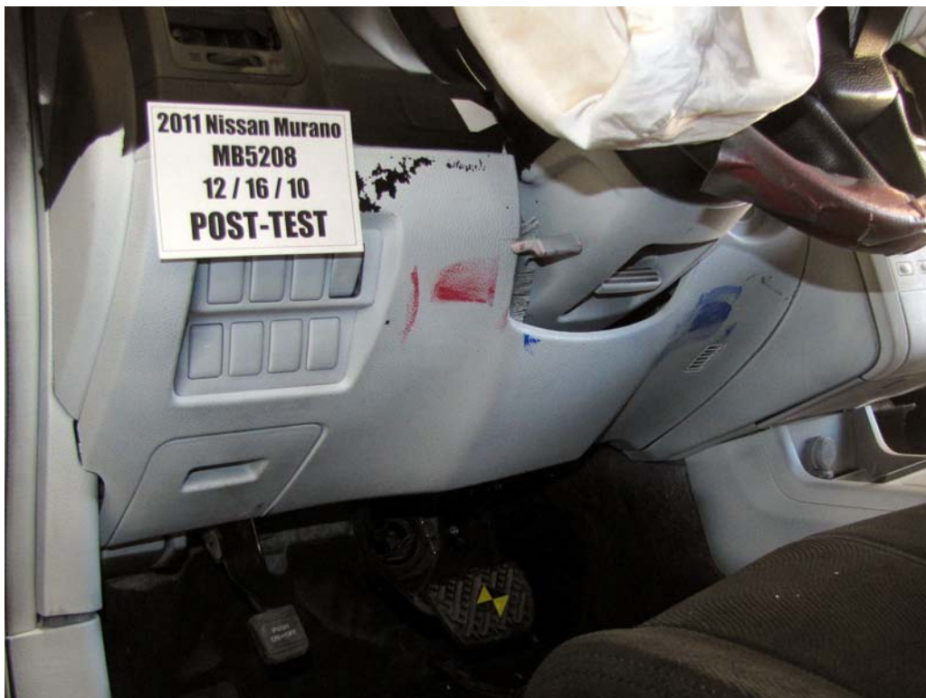
FIGURE 40. Post-Test Driver's Side Knee Bolster
