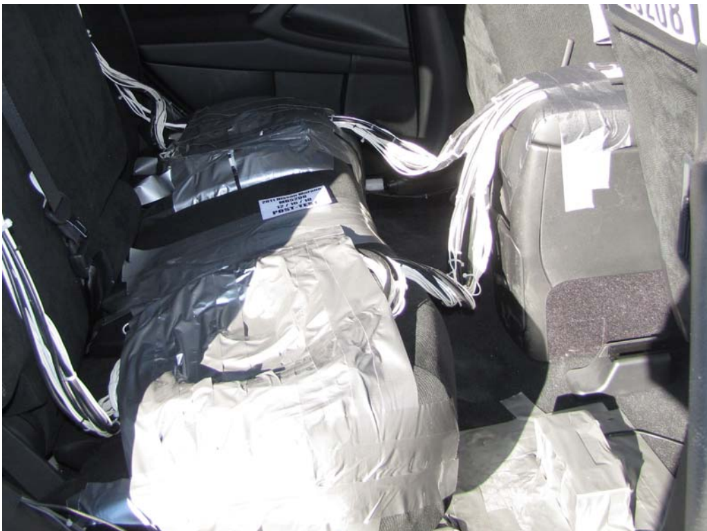
FIGURE 28. Post-Test Dummy Cable Routing
