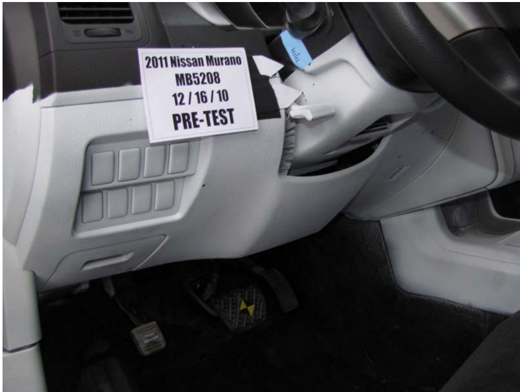
FIGURE 39. Pre-Test Driver's Side Knee Bolster
