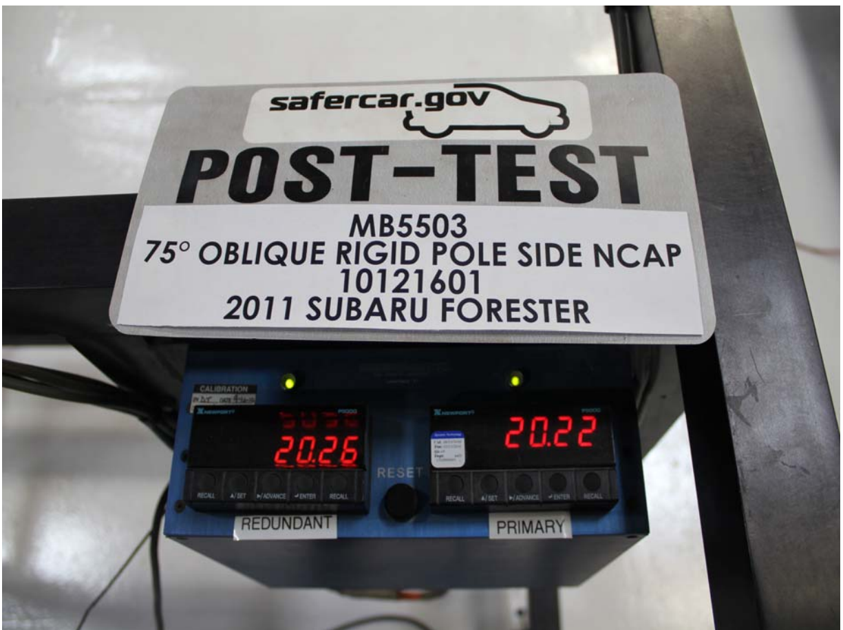
Post-Test Primary and Redundant Speed Trap Read-Out
