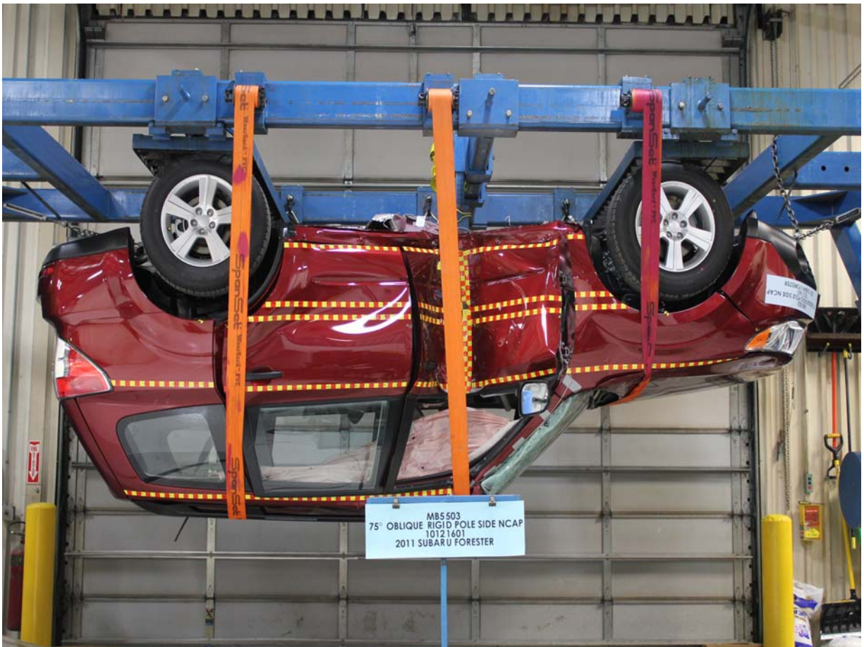
FMVSS No. 301/305 Rollover 180 Degrees
