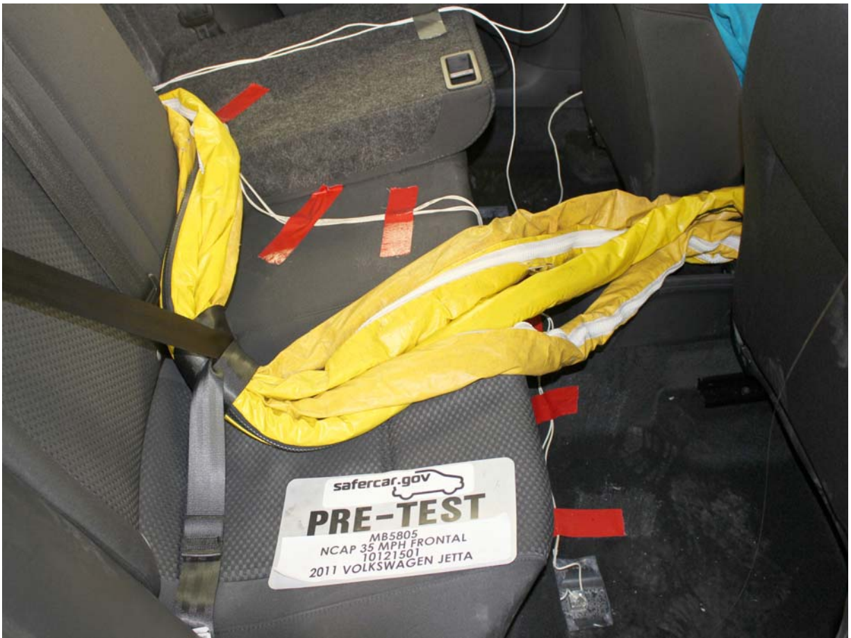
Pre-Test Dummy Cable Routing
