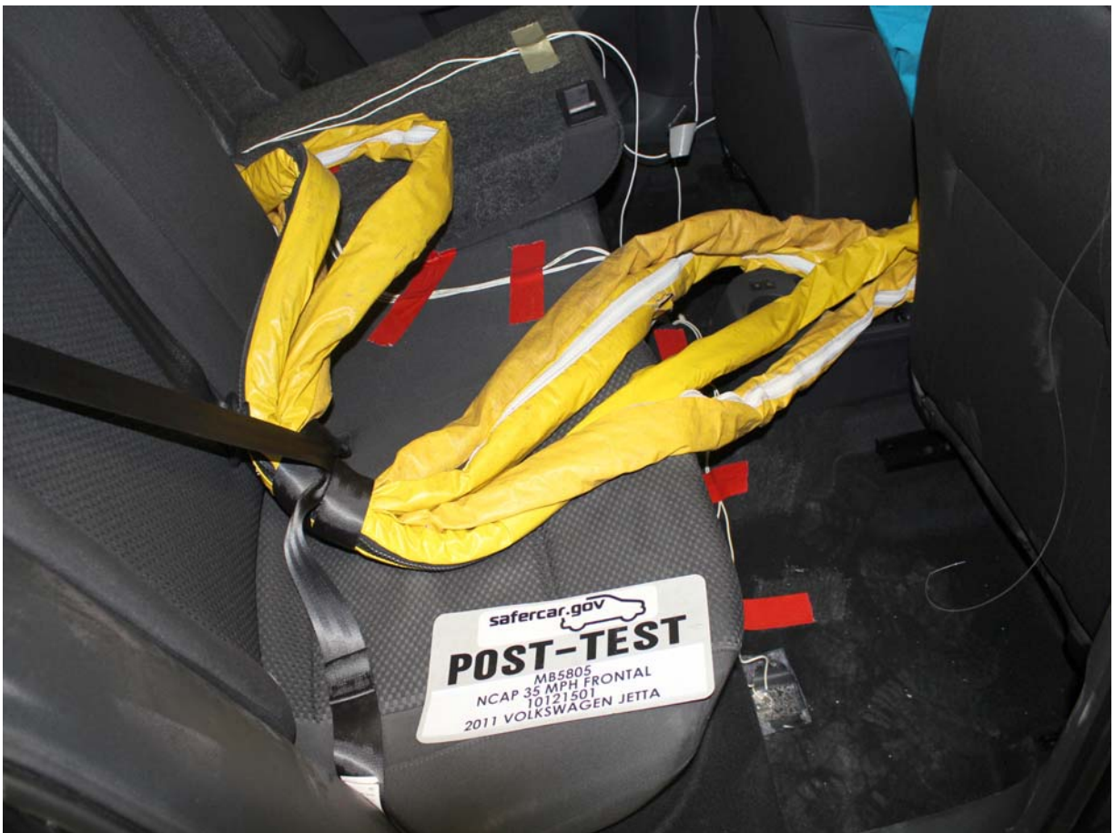
Post-Test Dummy Cable Routing
