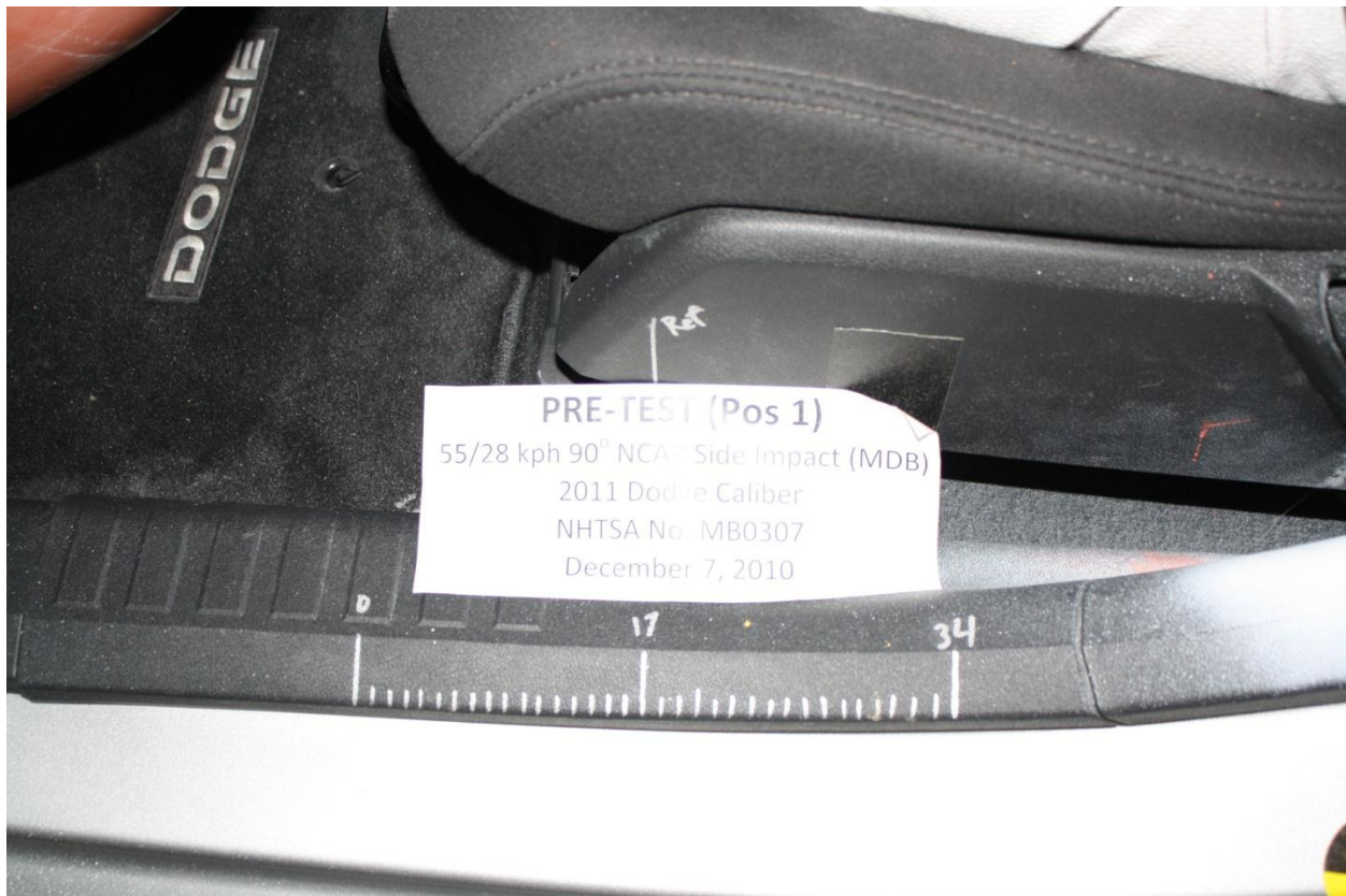
Figure A-38: Pre-test Close-up Left Side View of Driver Seat Track Showing Seat Positioning
