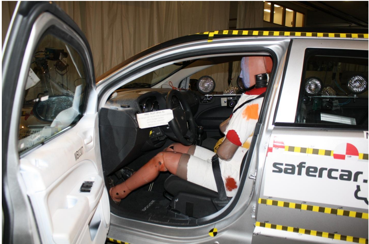
Figure A-27: Pre-Test Left Side View of Driver Dummy Showing Belt, Chalking, and Contact Switches
