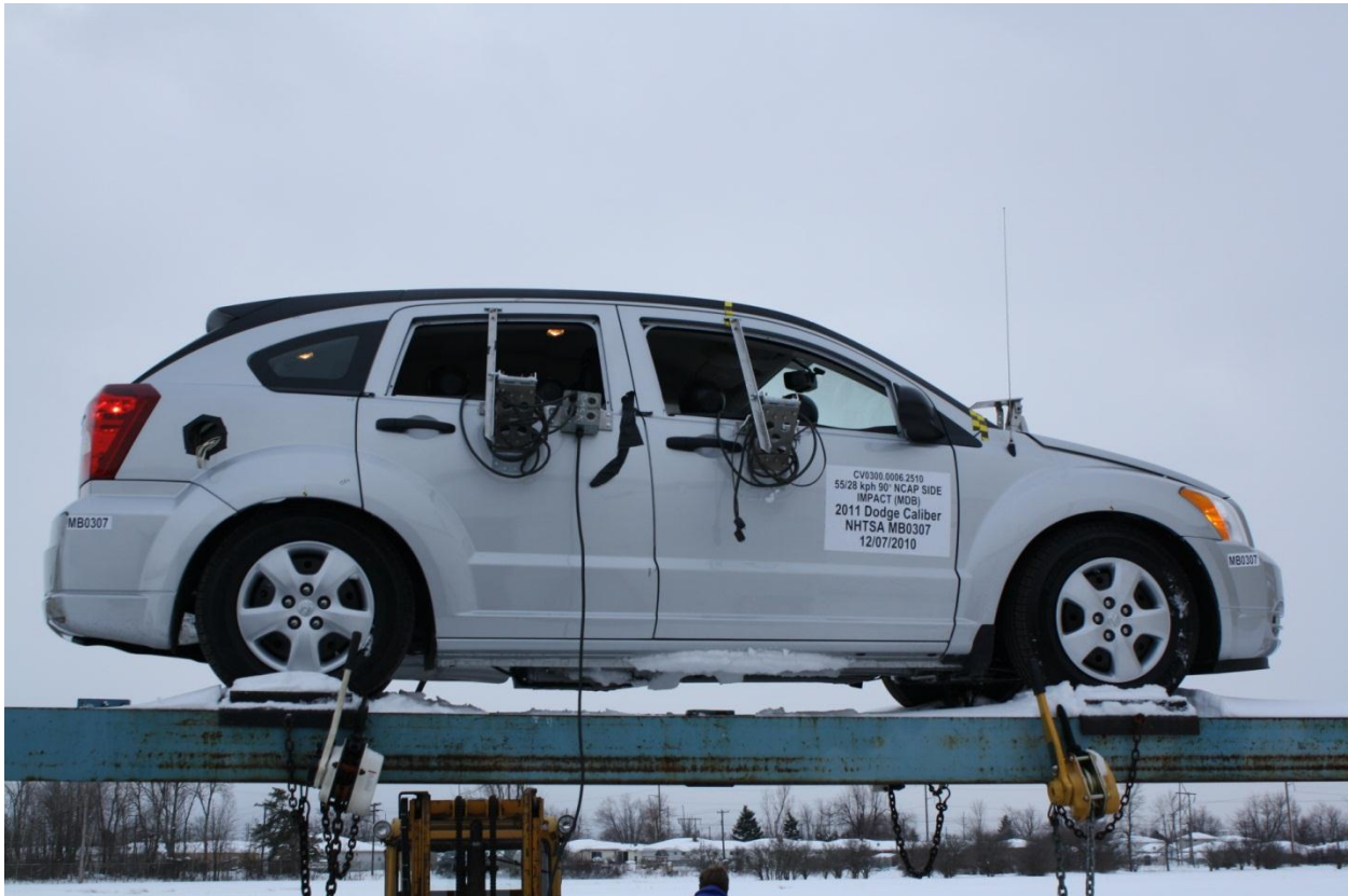
Figure A-93: FMVSS No. 301 Rollover 0°
