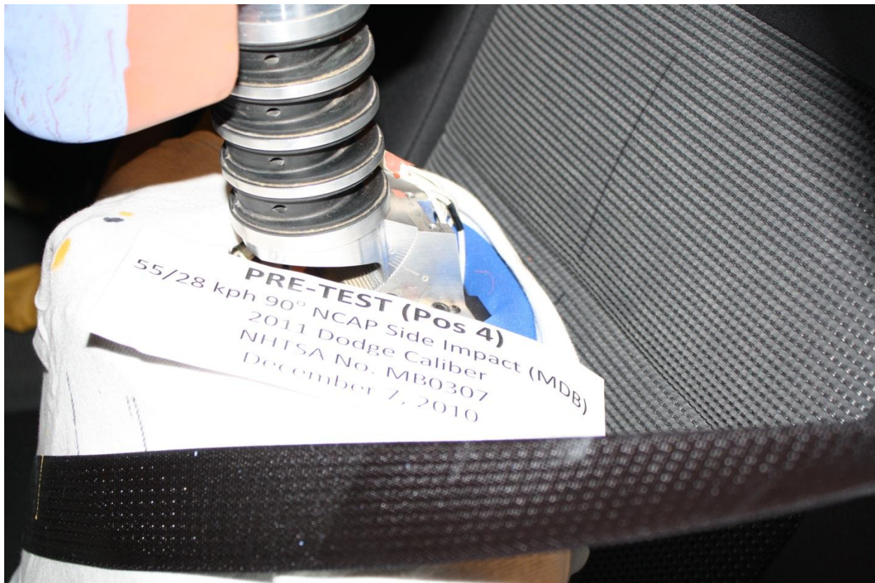
Figure A-60: Pre-Test View of Rear Passenger Dummy's Neck Showing Position of Adjustable Neck Bracket
