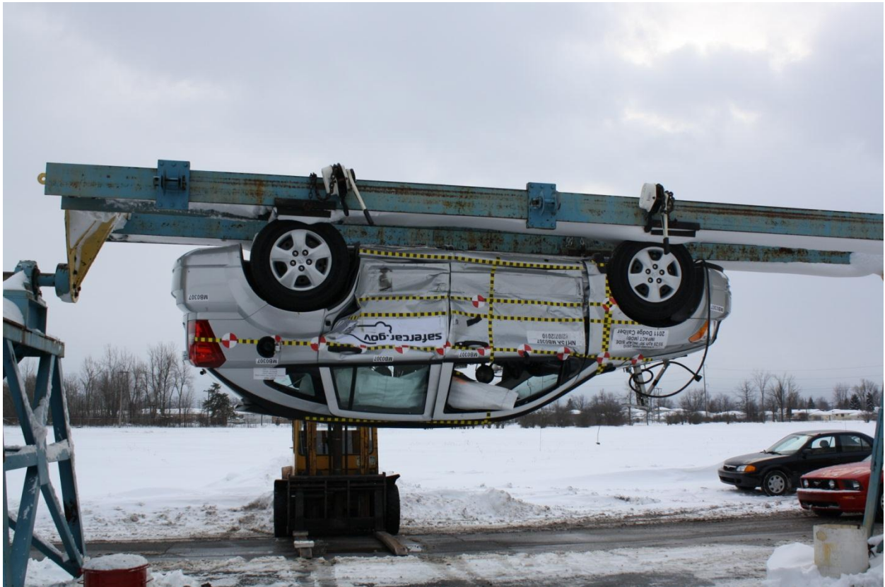
Figure A-95: FMVSS No. 301 Rollover 180°
