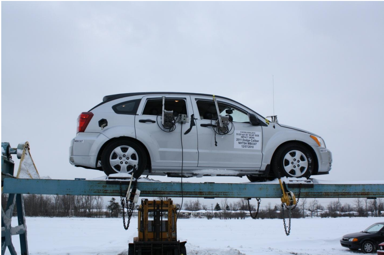
Figure A-97: FMVSS No. 301 Rollover 360°
