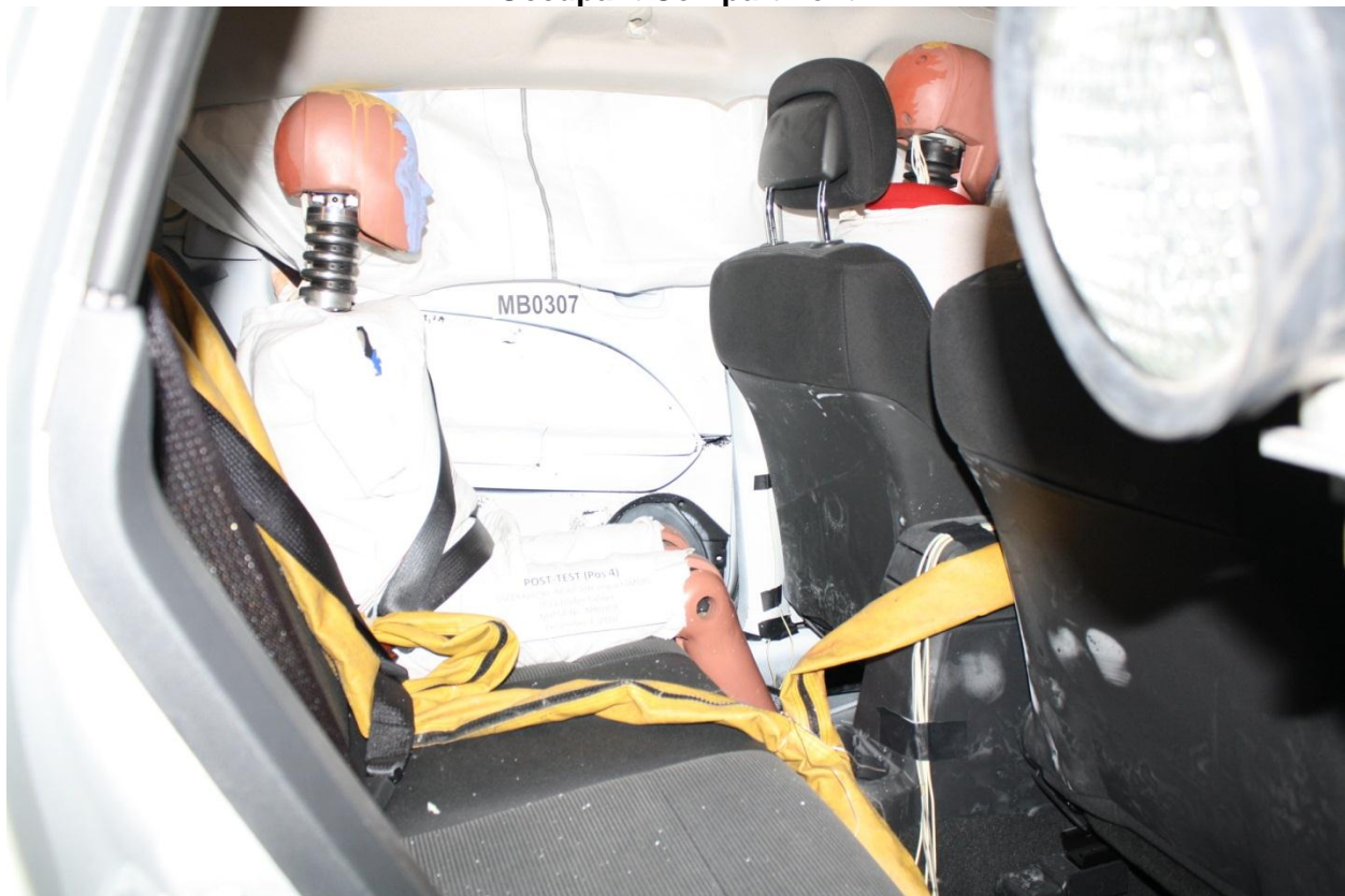
Figure A-70: Post-Test Right Side View of Rear Passenger Dummy and Rear Seat Occupant Compartment
