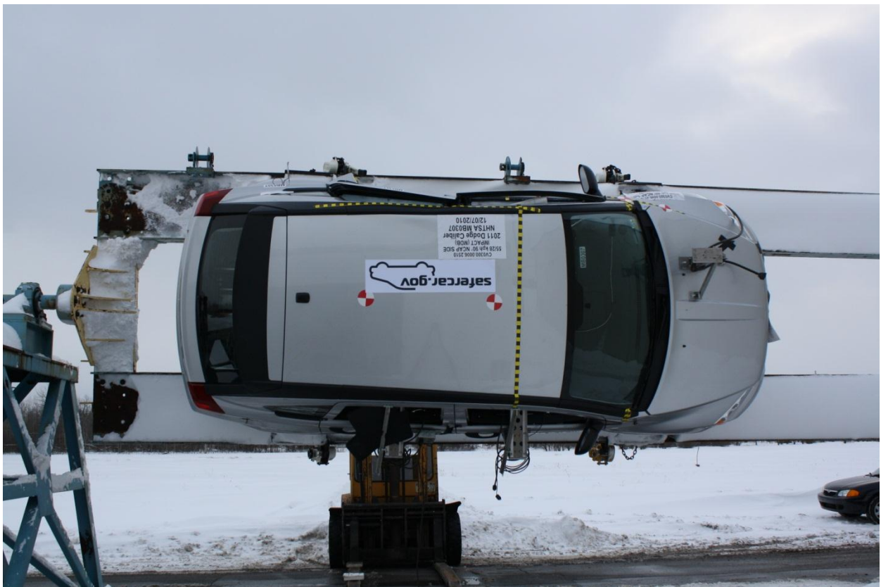
Figure A-96: FMVSS No. 301 Rollover 270°
