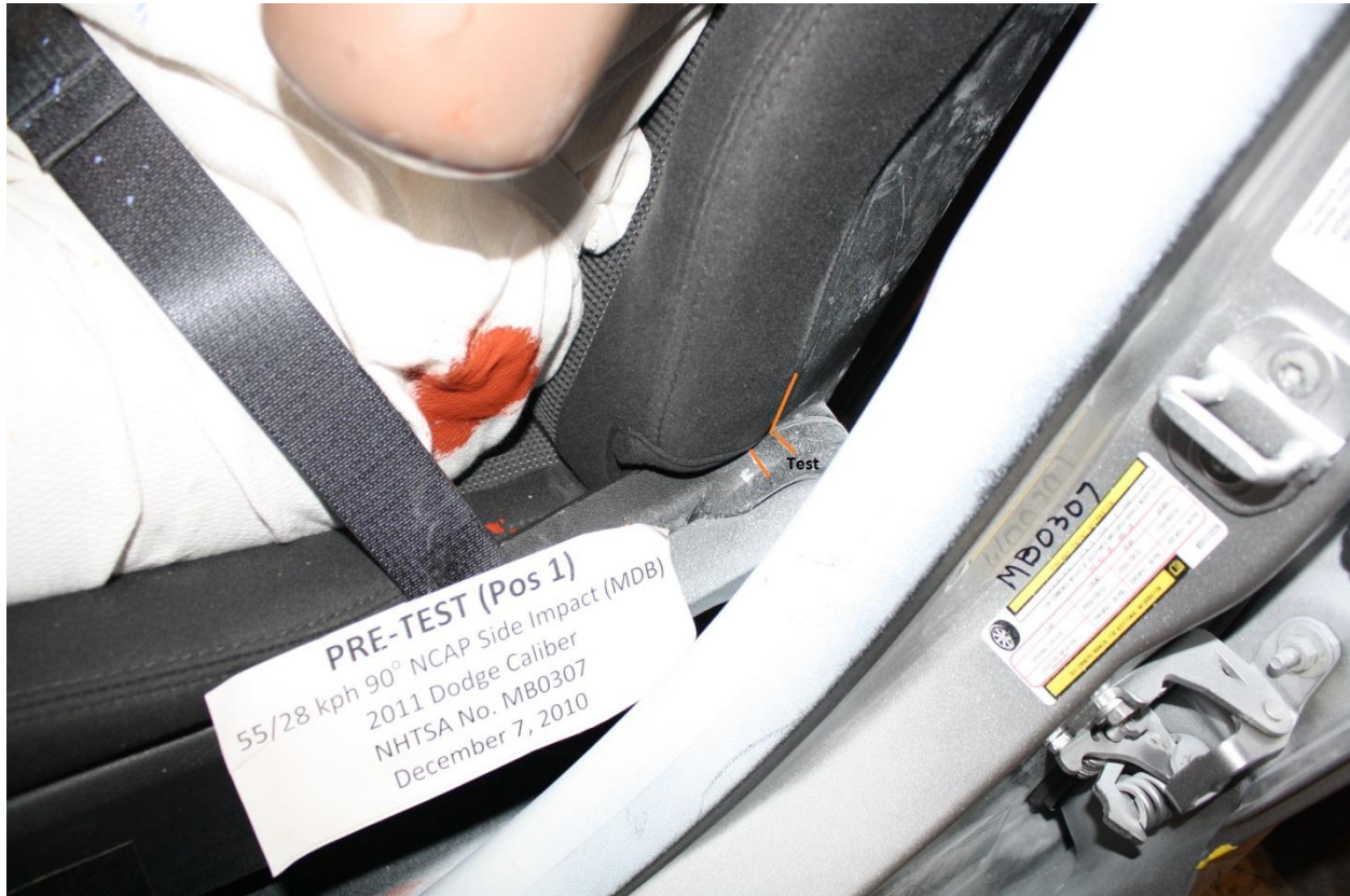
Figure A-39: Pre-test Close-up Left Side View of Driver Seat Back Showing Seat Back Positioning
