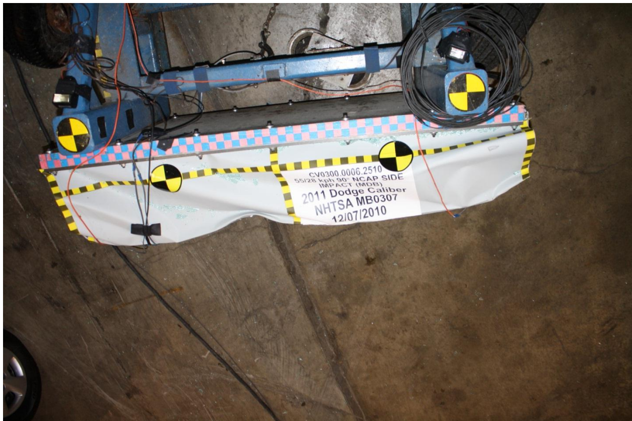
Figure A-84: Post-Test Top View of MDB Impactor Face
