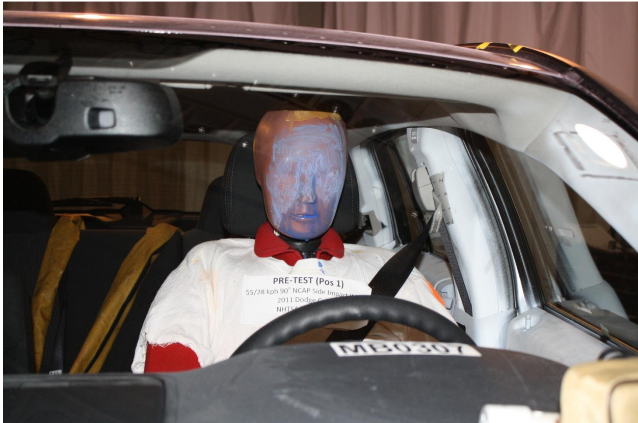
Figure A-31: Pre-Test Frontal View of Driver Dummy Head and Shoulders in Relation to Head Restraint
