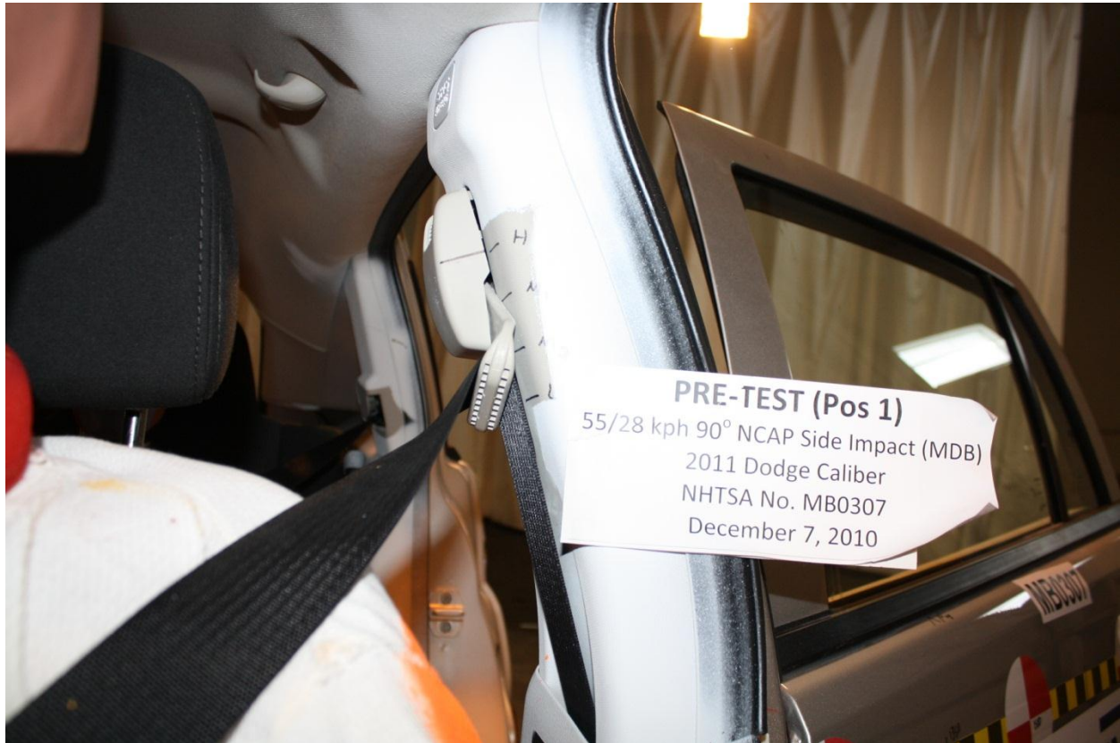
Figure A-35: Pre-Test View of Belt Anchorage for Driver Dummy to Show Position
