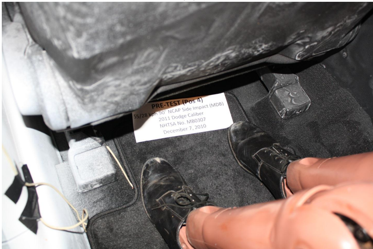
Figure A-62: Pre-Test Placement of Rear Passenger Dummy's Feet
