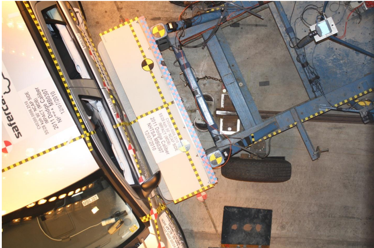
Figure A-15: Pre-Test Overhead View of the Test Vehicle and MDB
