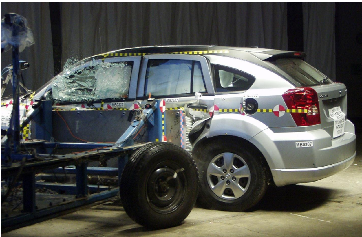
Figure A-98: Impact Event (Impact Side)
