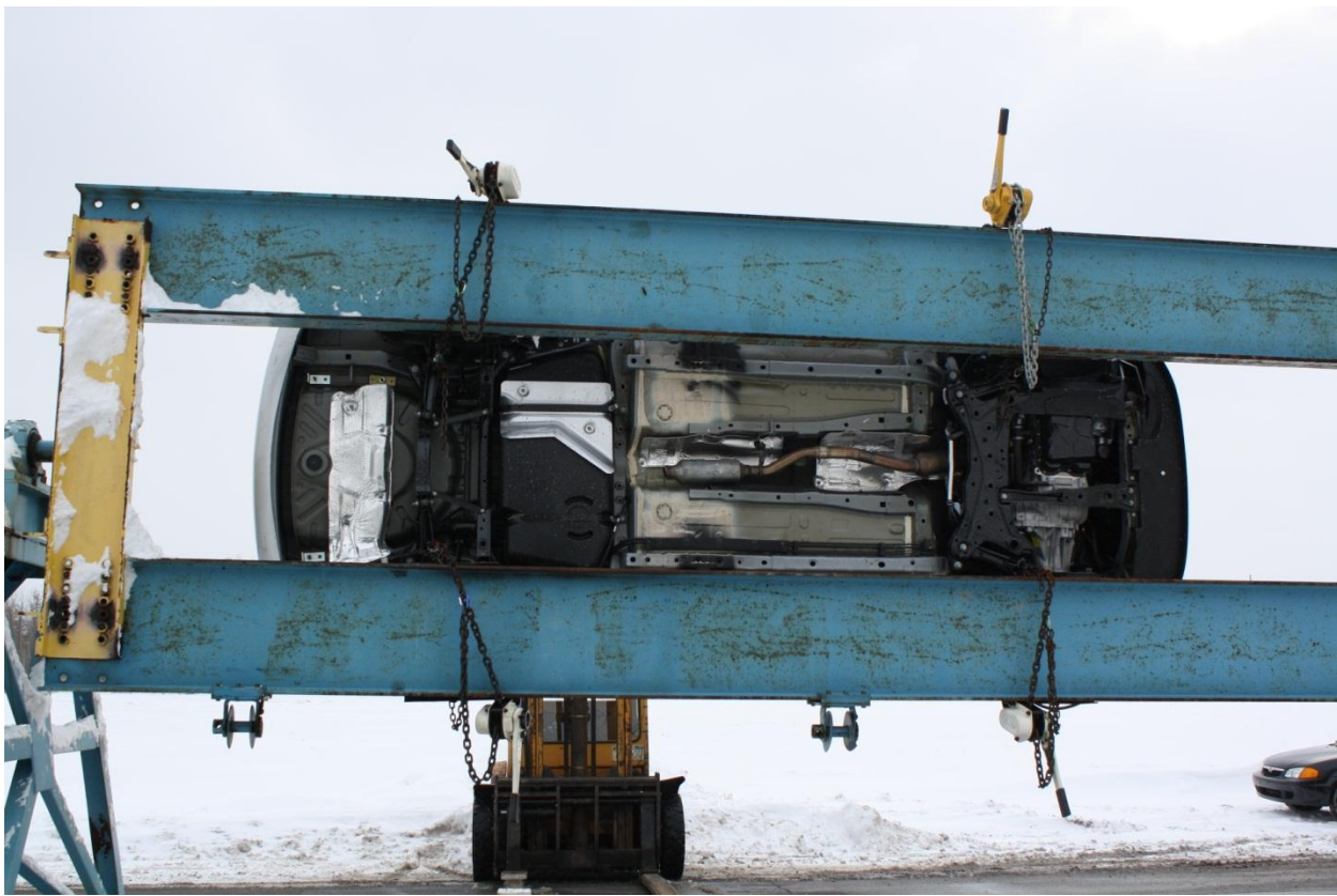
Figure A-94: FMVSS No. 301 Rollover 90°
