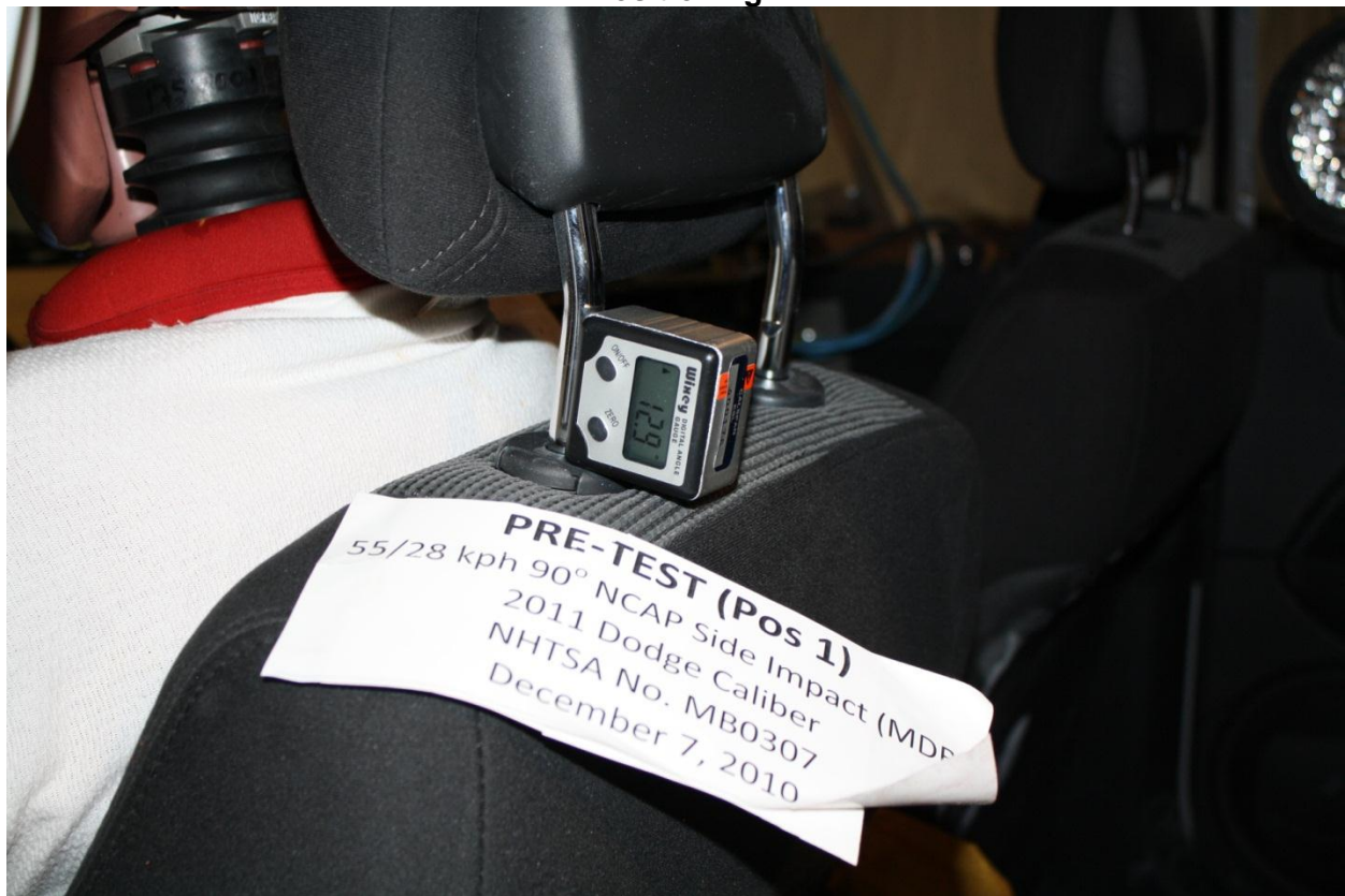
Figure A-40: Pre-Test Close-Up View of Driver Seat Back or Head Restraint Showing Seat Back Test Position
