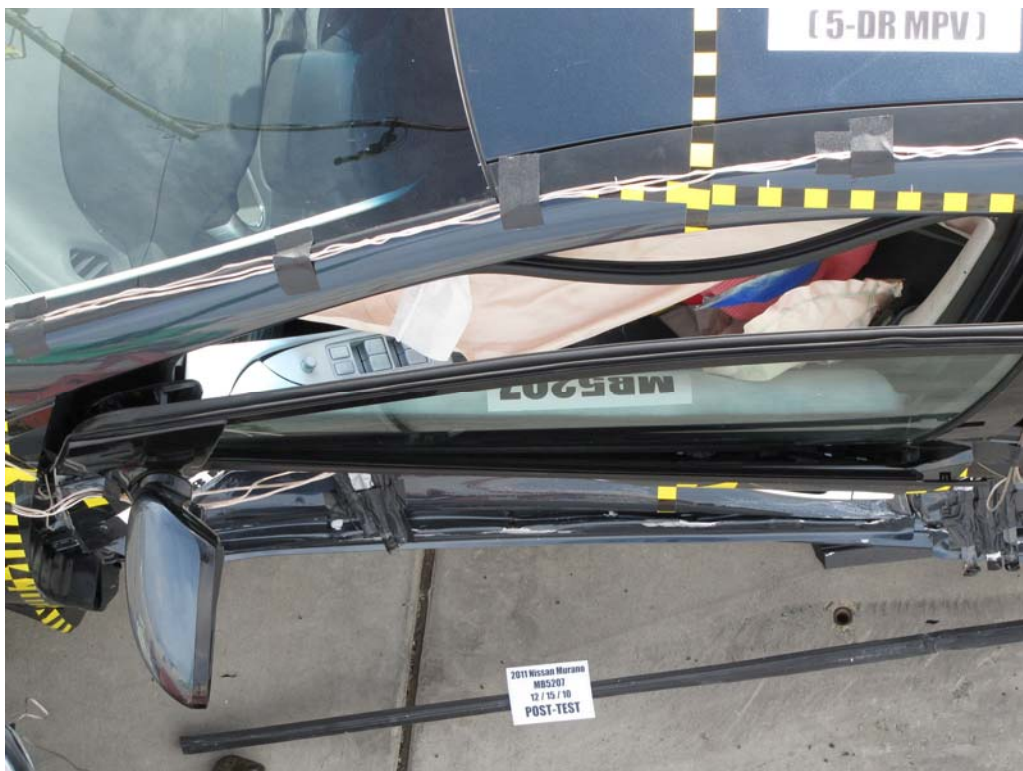
FIGURE 42. Post-Test Driver Dummy and Door Clearance View
