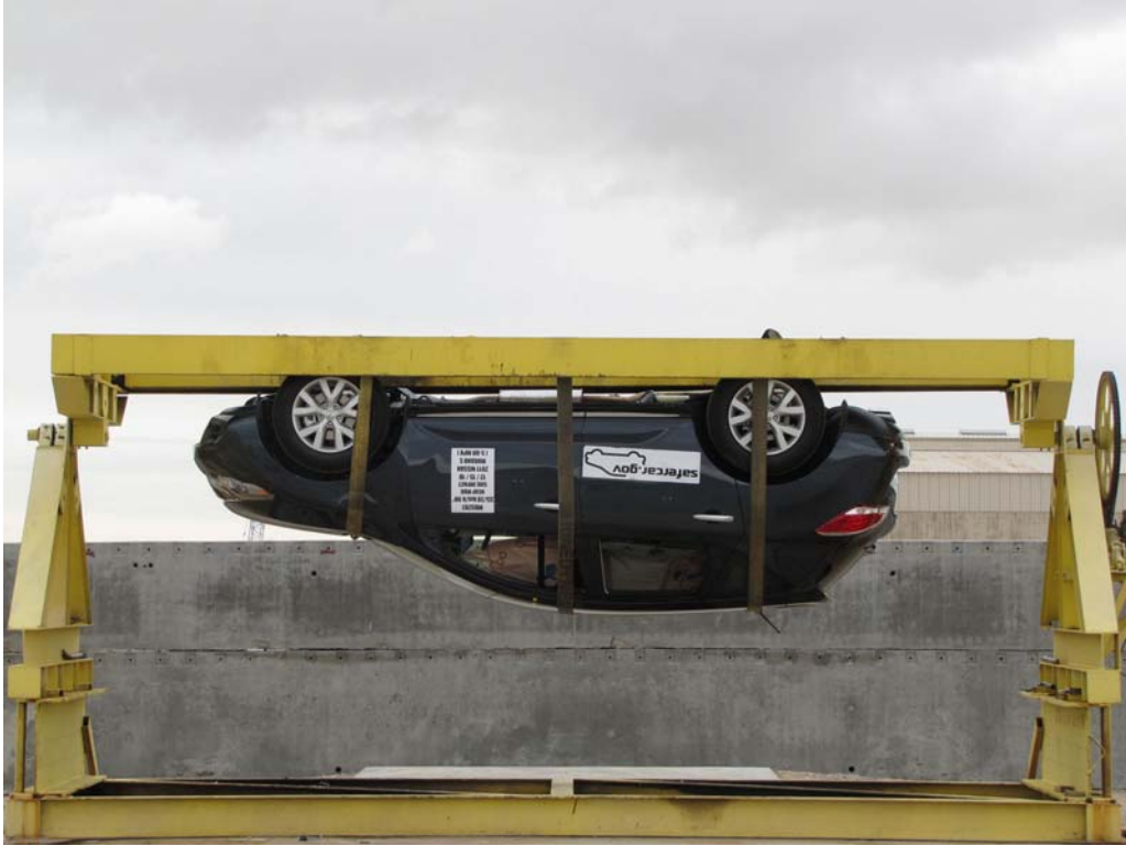
FIGURE 95. FMVSS No. 301/305 Rollover 180 Degrees
