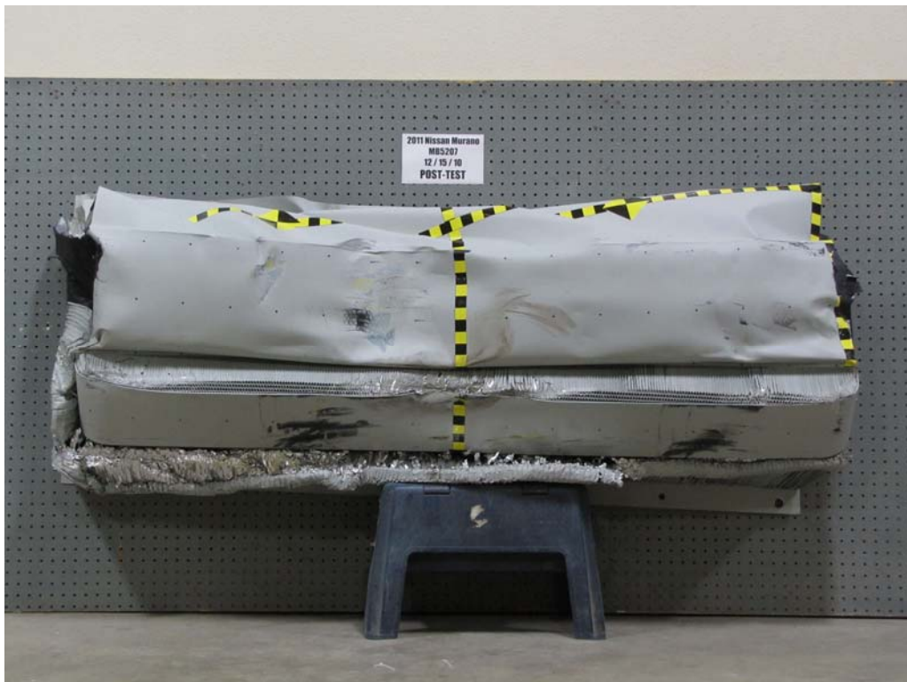
FIGURE 82. Post-Test Front View of MDB Impactor Face
