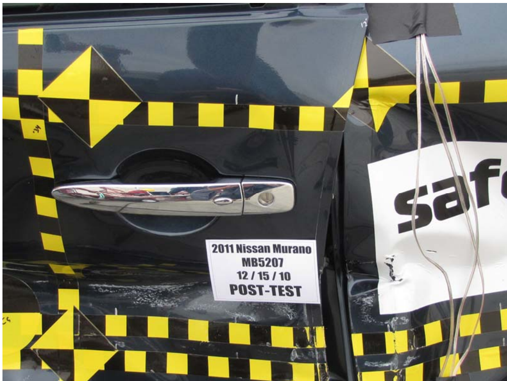
FIGURE 22. Post-Test Left Front Door Latch Close-Up
