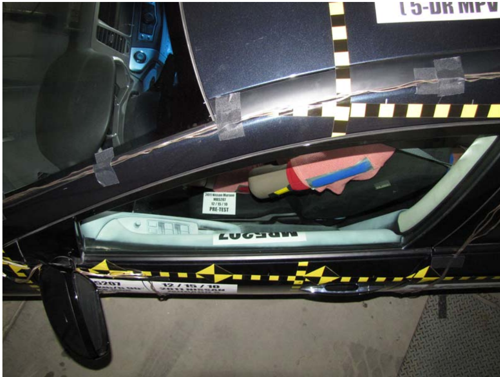
FIGURE 41. Pre-Test Driver Dummy and Door Clearance View
