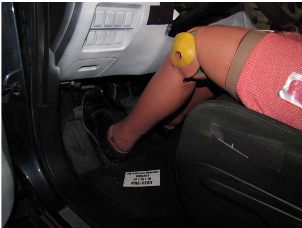
FIGURE 34. Pre-Test Placement of Driver Dummy's Feet
