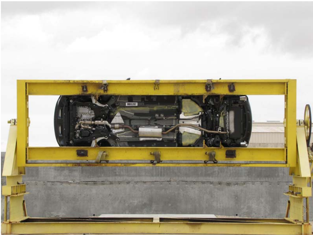
FIGURE 96. FMVSS No. 301/305 Rollover 270 Degrees
