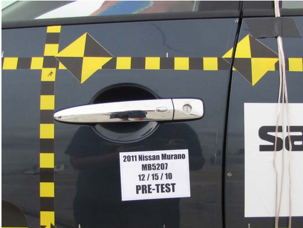
FIGURE 21. Pre-Test Left Front Door Latch Close-Up
