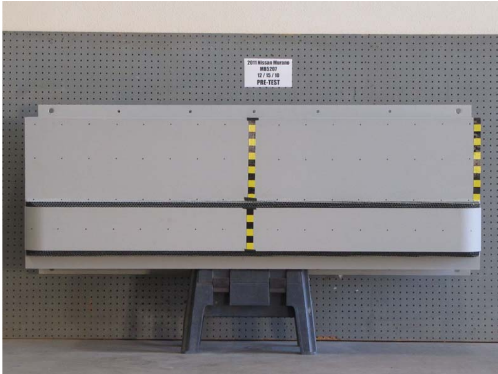
FIGURE 81. Pre-Test Front View of MDB Impactor Face
