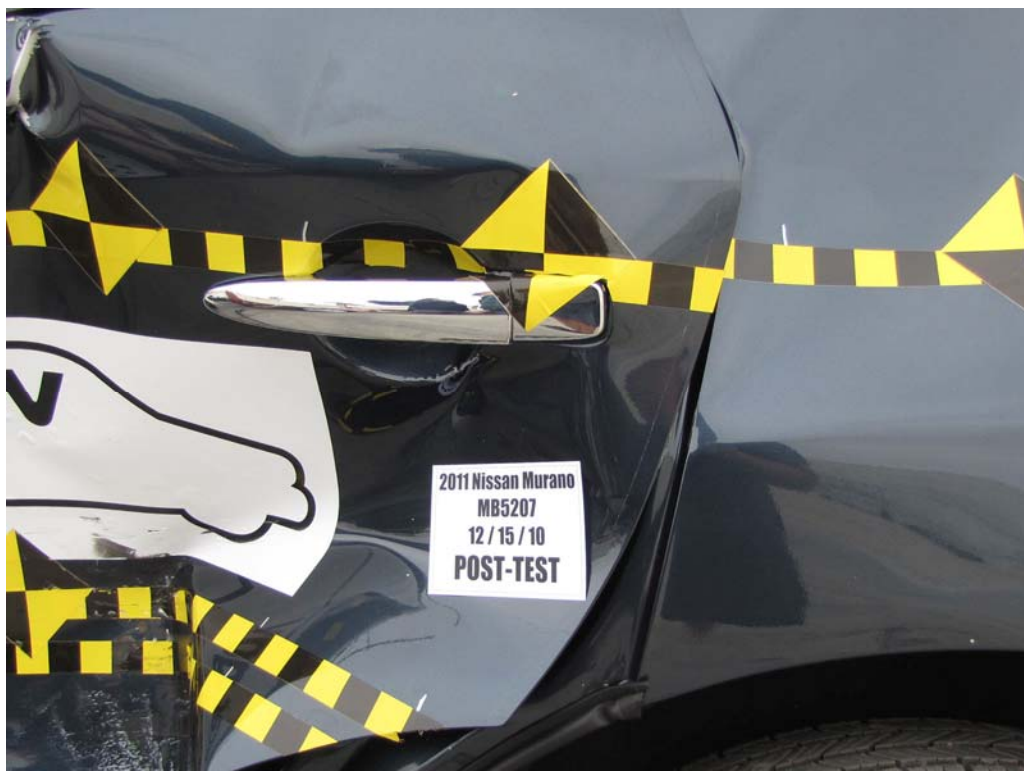
FIGURE 24. Post-Test Left Rear Door Latch Close-Up
