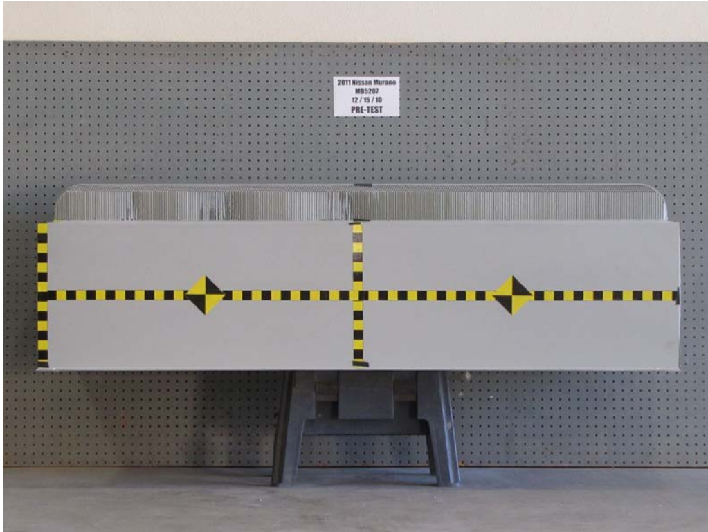
FIGURE 83. Pre-Test Top View of MDB Impactor Face
