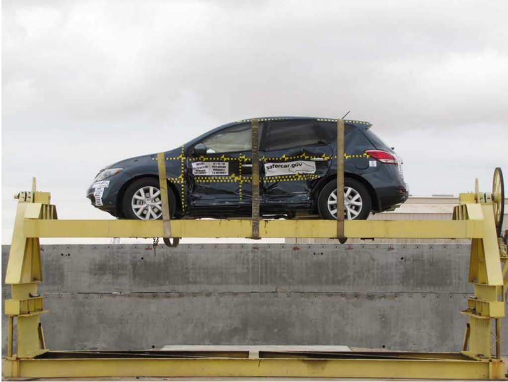
FIGURE 93. FMVSS No. 301/305 Rollover 0 Degrees
