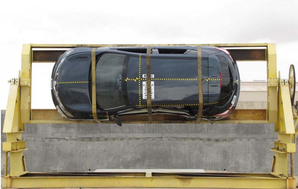
FIGURE 94. FMVSS No. 301/305 Rollover 90 Degrees
