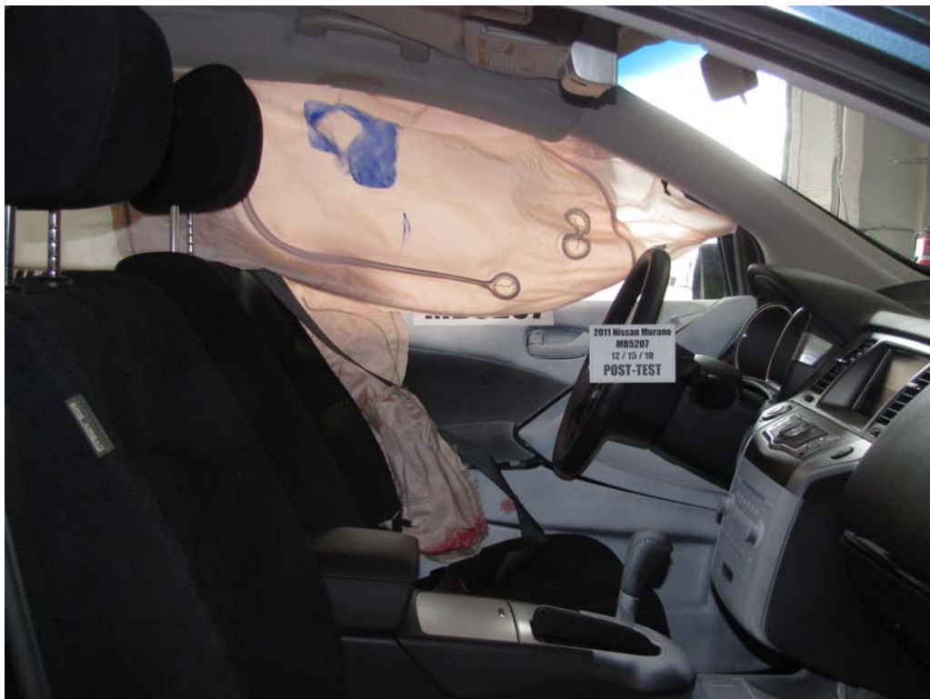
FIGURE 46. Post-Test Driver Dummy Inner Door Panel View Showing Driver Dummy Contact Locations
