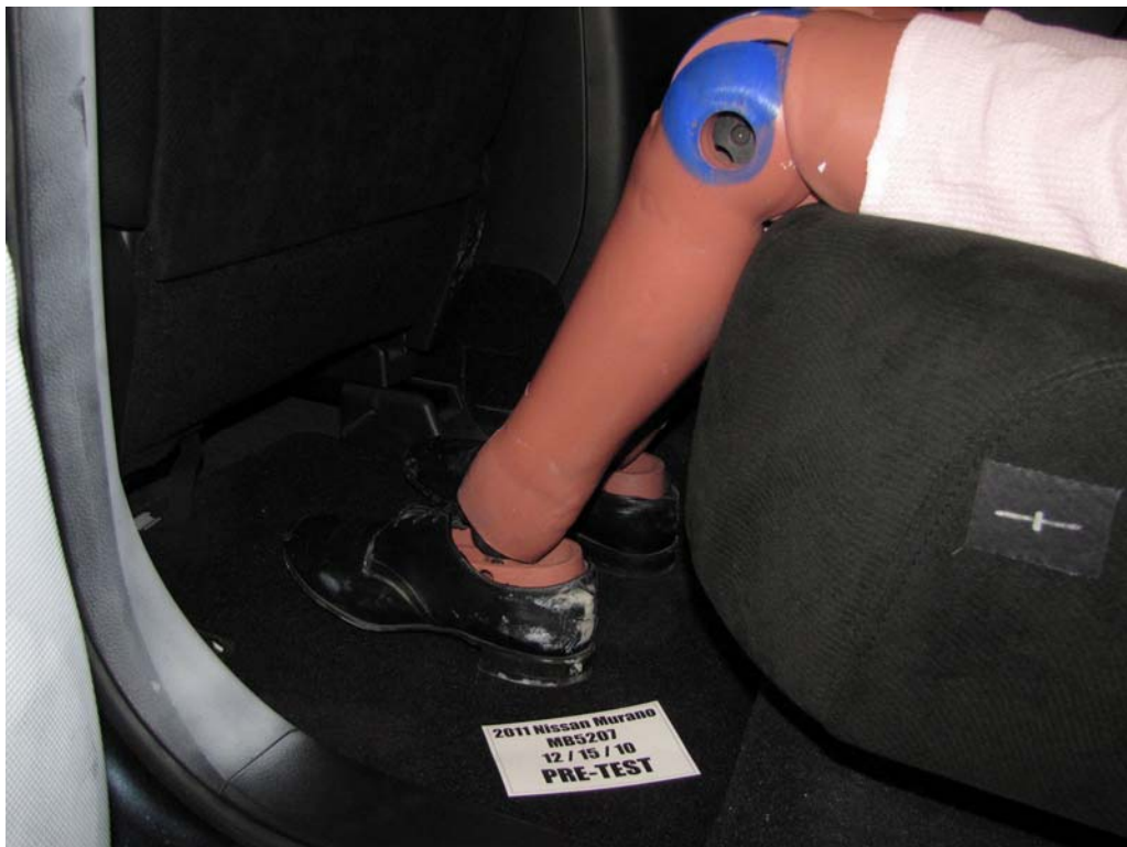
FIGURE 62. Pre-Test Placement of Rear Passenger Dummy's Feet
