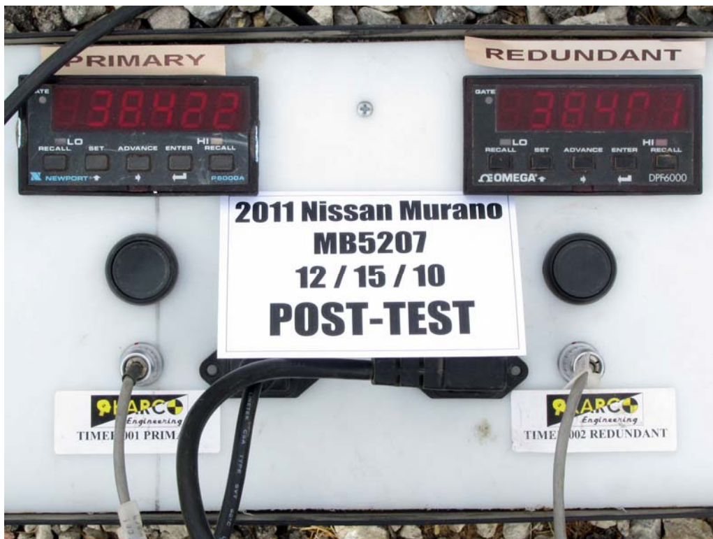
FIGURE 92. Post-Test Primary and Redundant Speed Trap Read-Out
