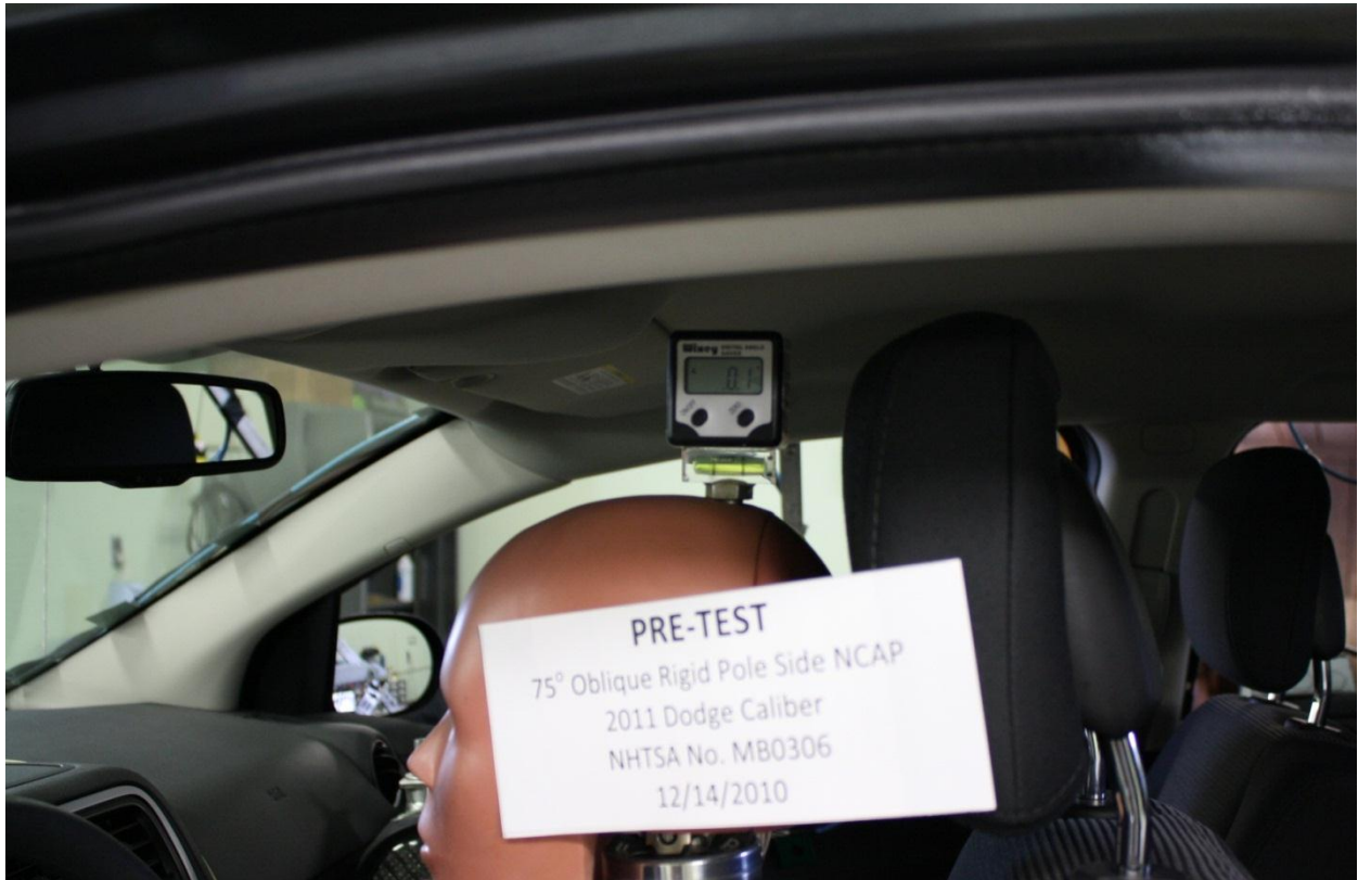
Figure A-31: Pre-Test View of Dummy's Head Showing Dummy's Head is Level
