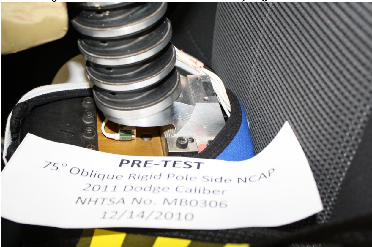
Figure A-30: Pre-Test View of Dummy's Neck Showing Position of Adjustable Neck Bracket
