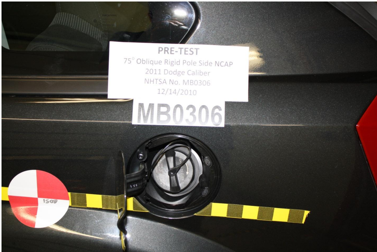
Figure A-51: Pre-Test View of Fuel Filler Cap or Fuel Filler Neck
