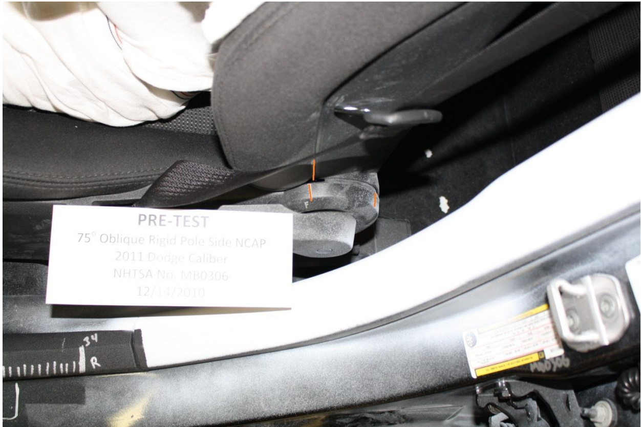
Figure A-37: Pre-Test Close-Up Left Side View of Driver Seat Back Showing Test Position
