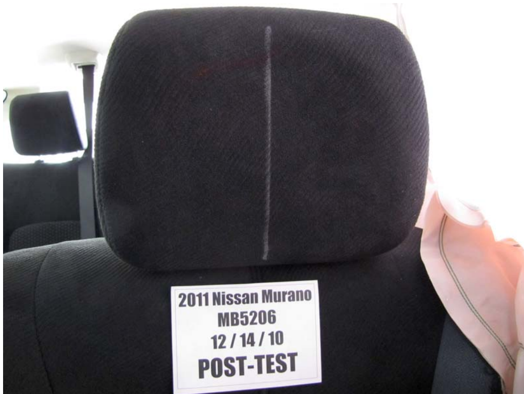
FIGURE 45. Post-Test Dummy Close-Up Head Contact with Vehicle Interior View
