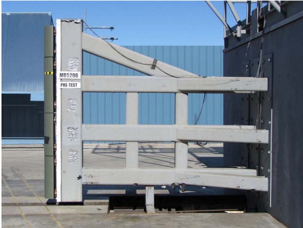
FIGURE 55. Pre-Test Pole Barrier Front View
