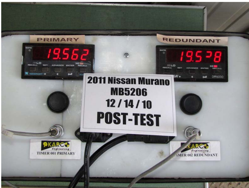
FIGURE 60. Post-Test Primary and Redundant Speed Trap Read-Out
