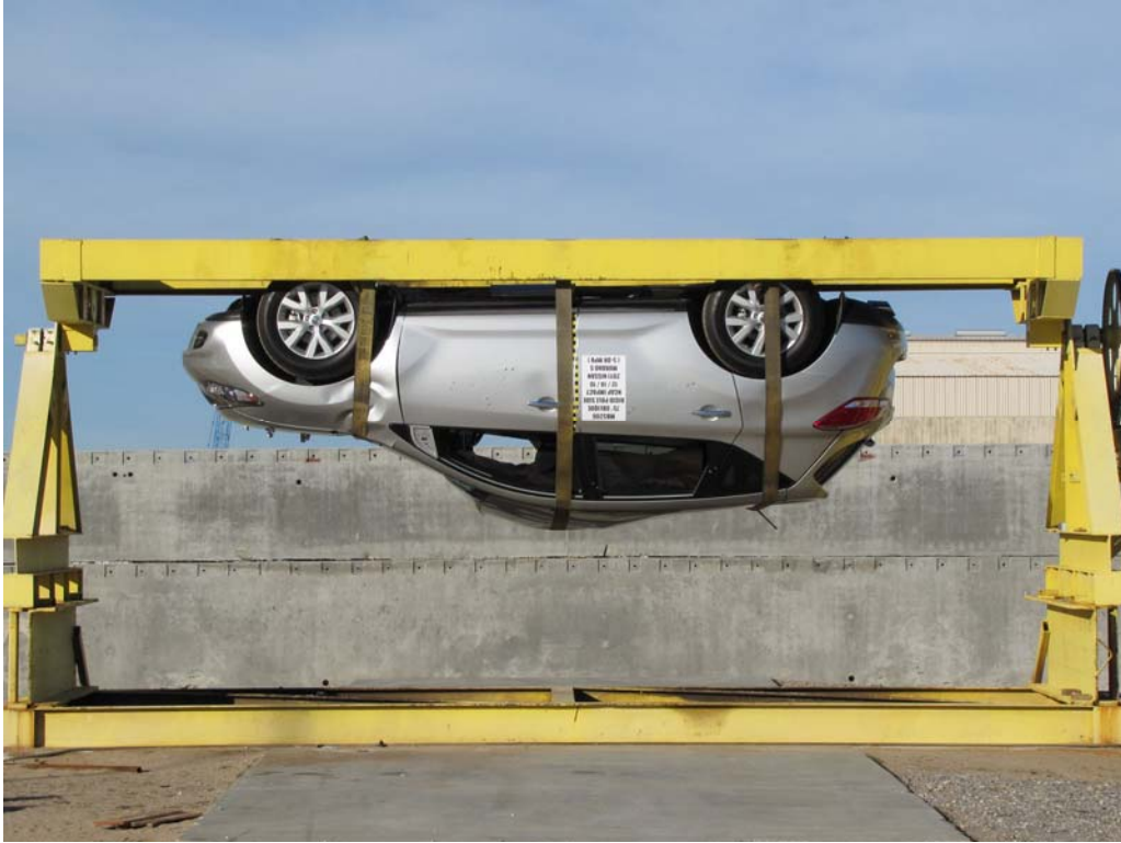
FIGURE 63. FMVSS No. 301-305 Rollover 180 Degrees
