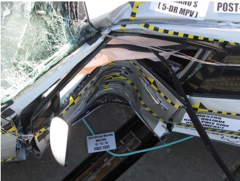
FIGURE 40. Post-Test Driver Dummy and Door Clearance
