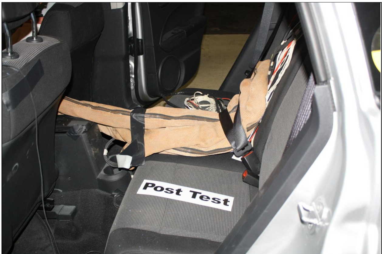
Figure A-28: Post-Test Dummy Cable Routing
