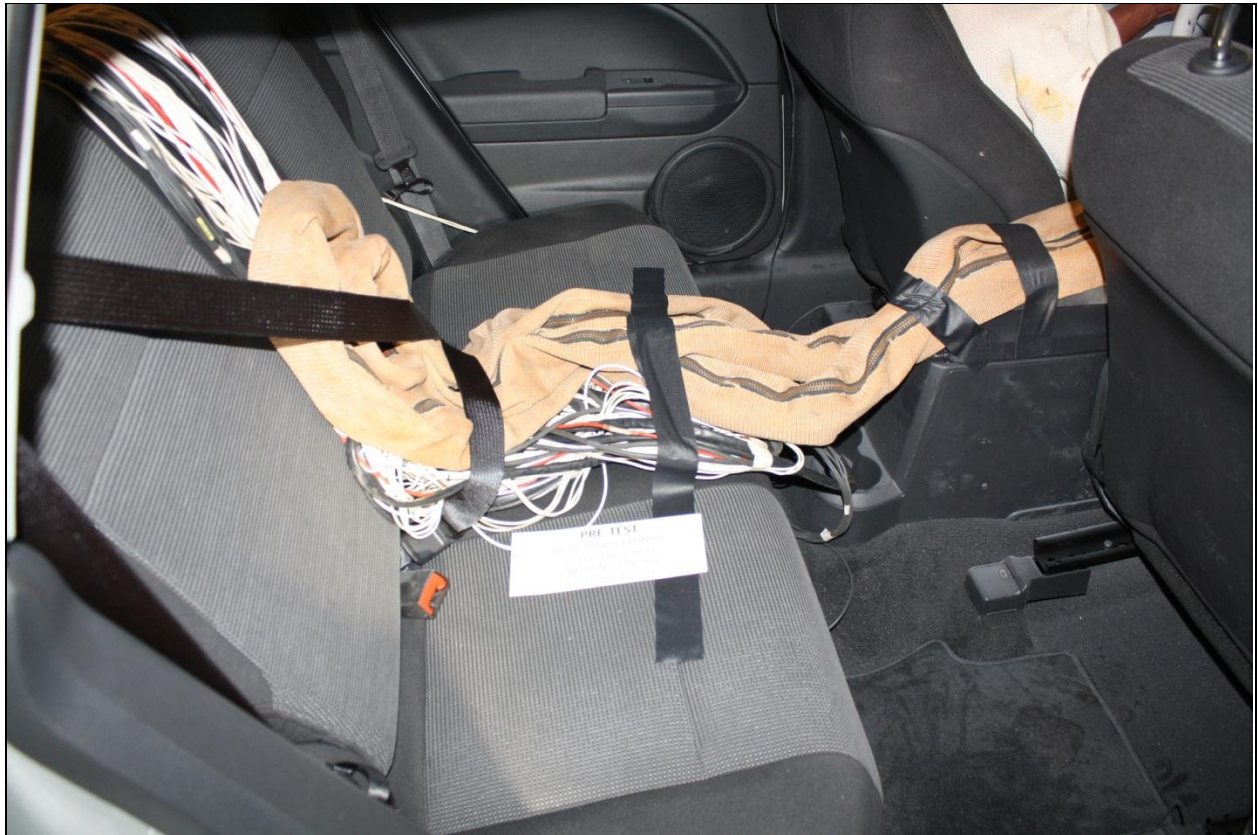
Figure A-27: Pre-Test Dummy Cable Routing
