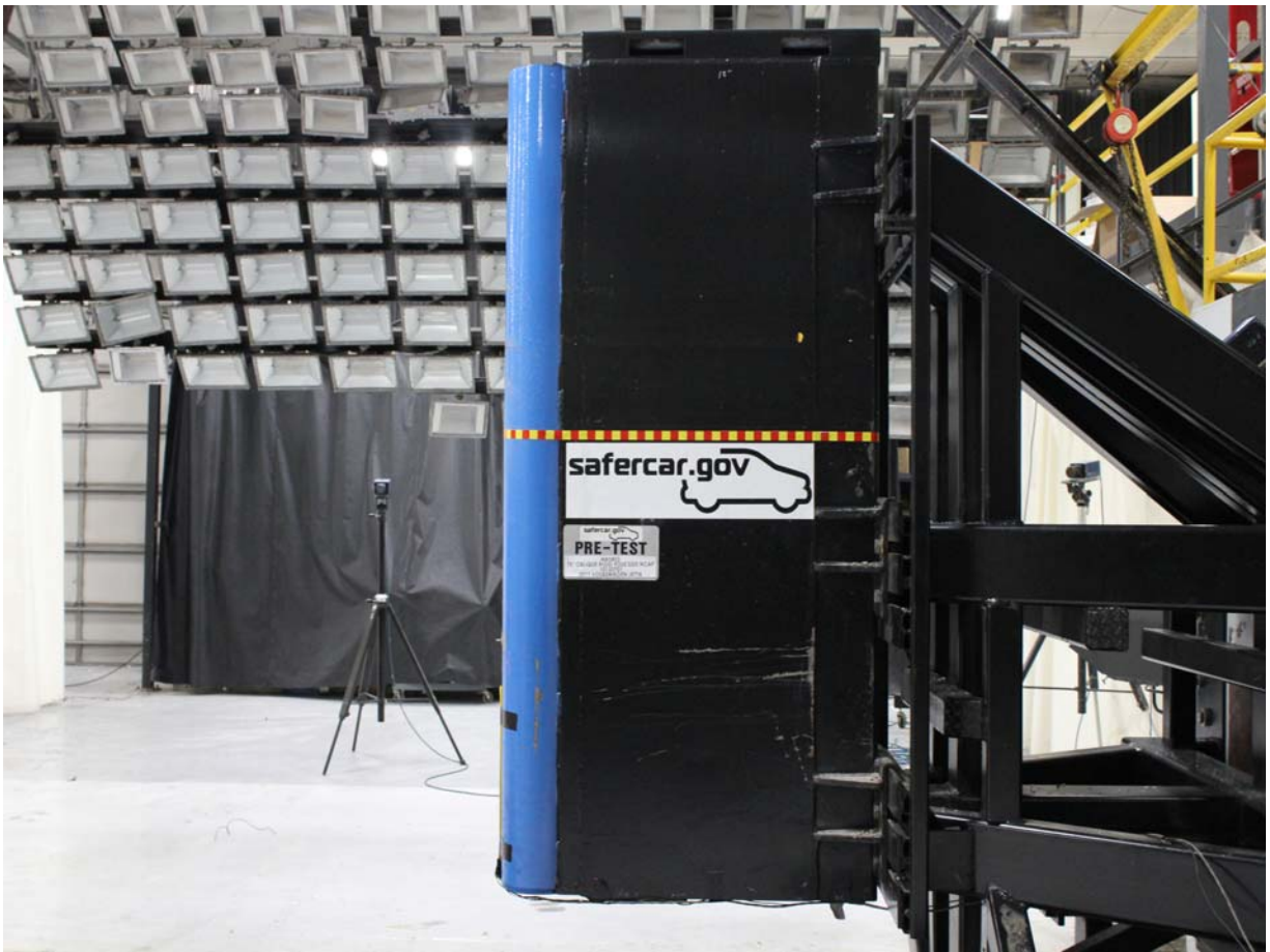
Pre-Test Pole Barrier Side View
