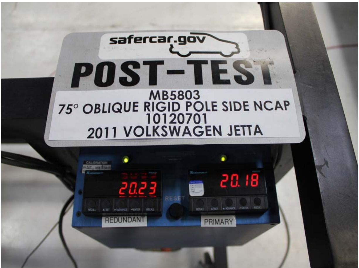
Post-Test Primary and Redundant Speed Trap Read-Out
