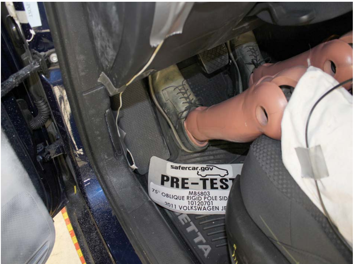
Pre-Test Placement of Dummy's Feet
