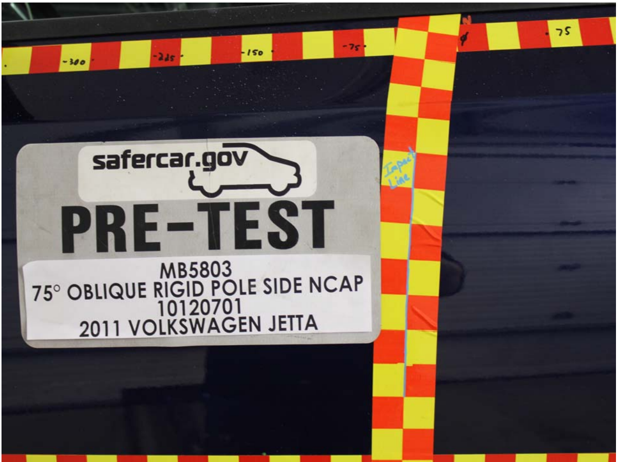
Pre-Test Close-Up View of Impact Point Target
