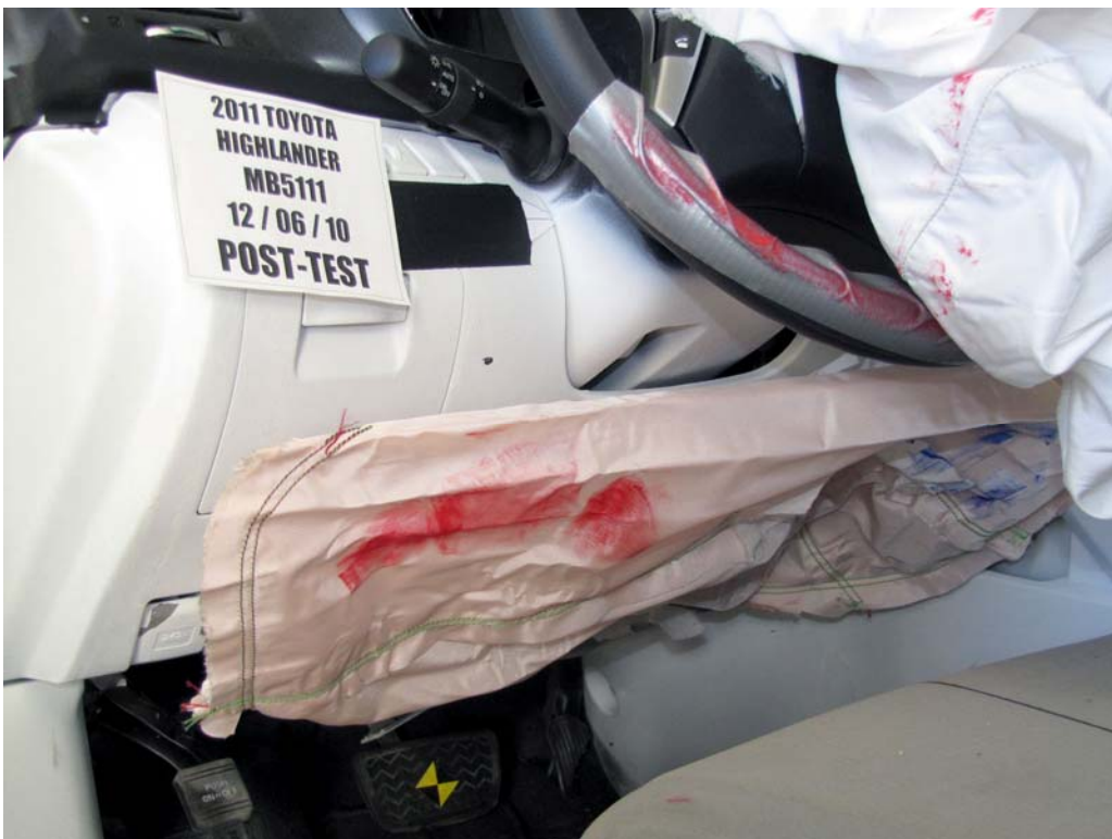
FIGURE 40. Post-Test Driver's Side Knee Bolster
