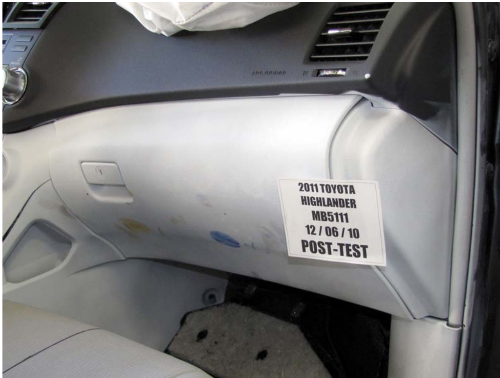
FIGURE 57. Post-Test Passenger's Side Knee Bolster
