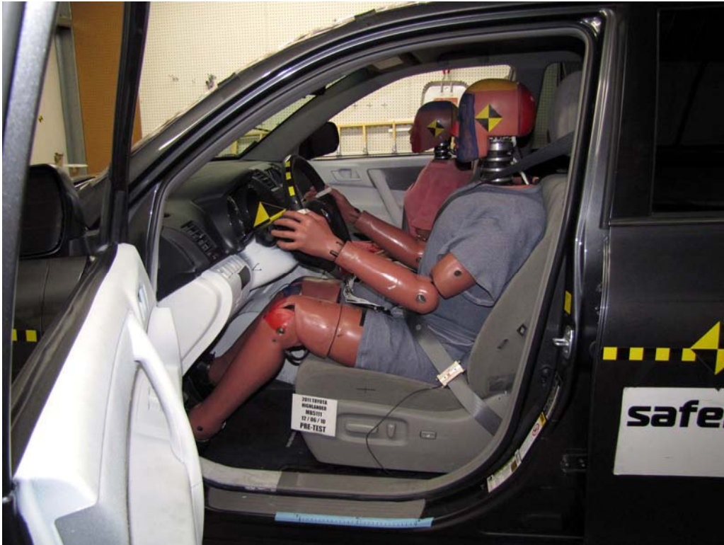
FIGURE 33. Pre-Test Driver Dummy and Vehicle Interior View
