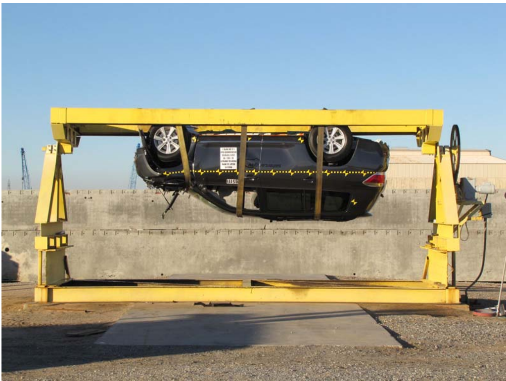
FIGURE 66. Vehicle at 180° on Static Rollover Device
