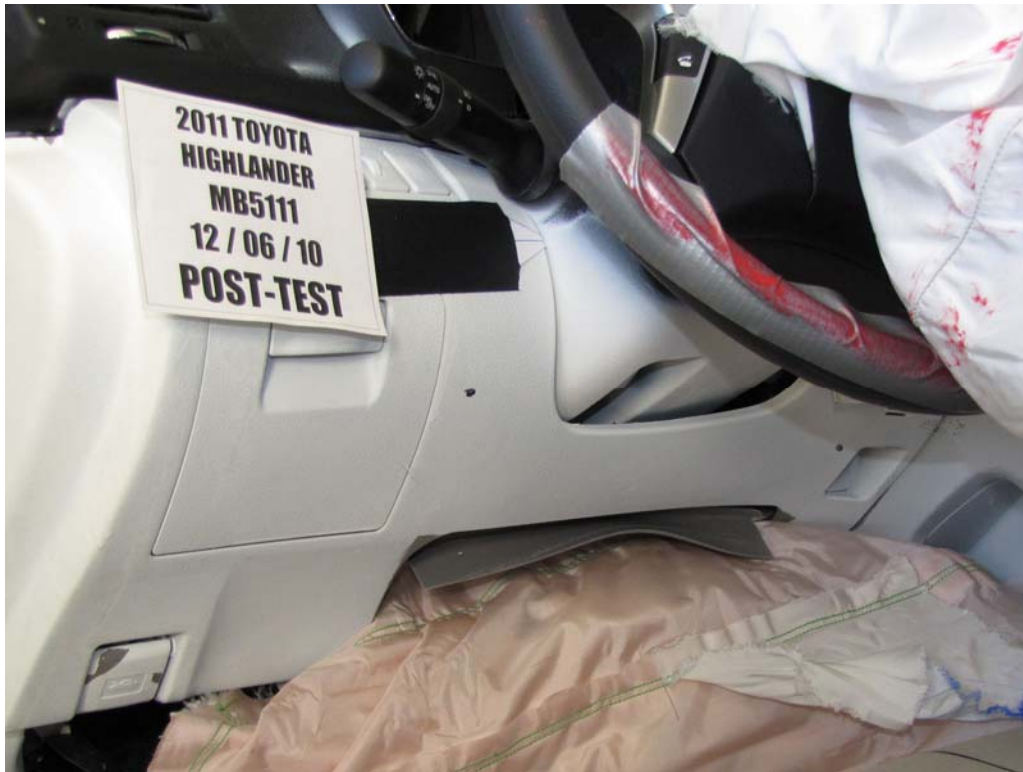
FIGURE 45. Post-Test View of Steering Column Shear Capsule
