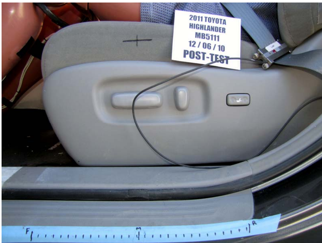
FIGURE 36. Post-Test Driver's Seat Fore-Aft Markings
