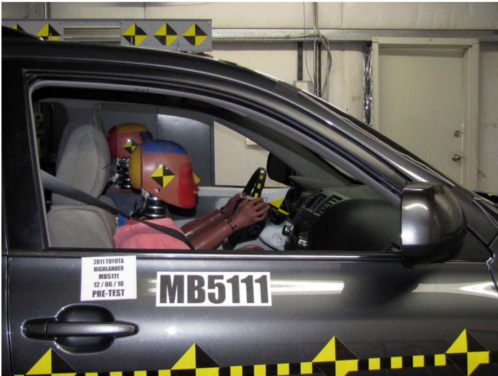
FIGURE 48. Pre-Test Passenger Dummy Window View
