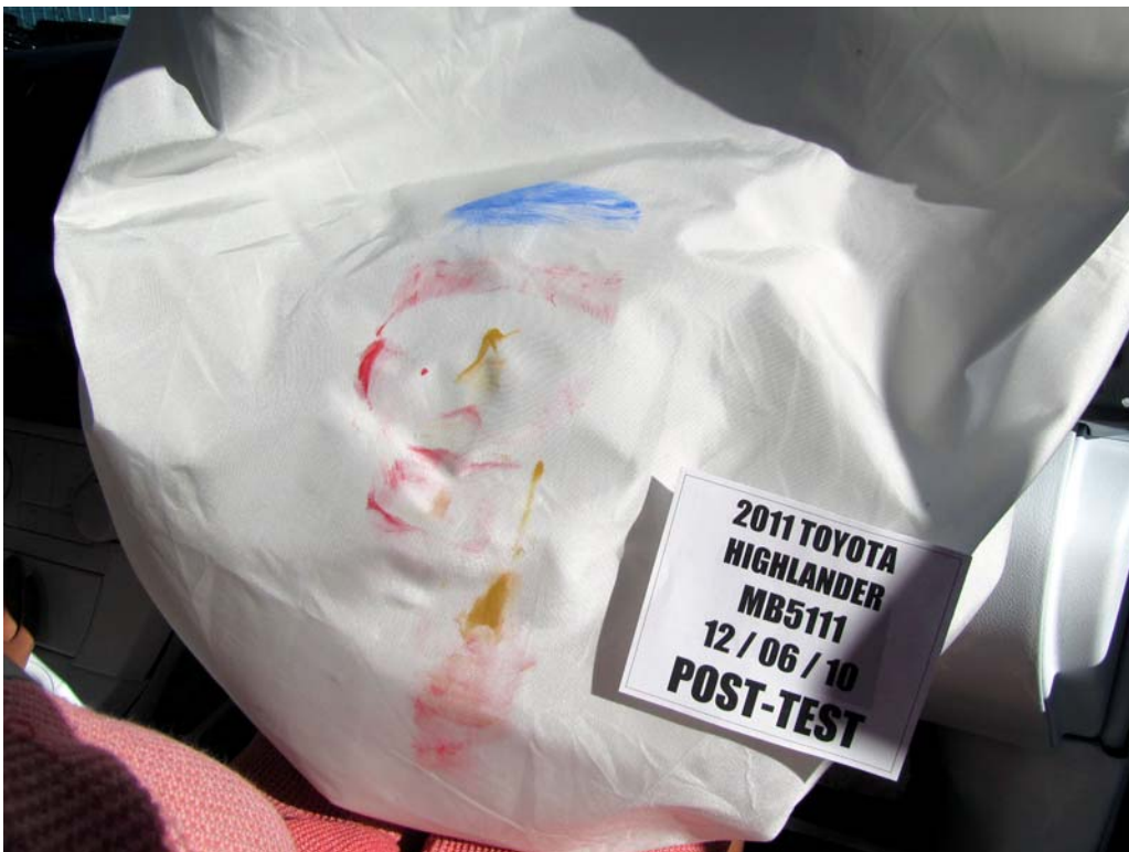
FIGURE 60. Post-Test Passenger Dummy Contact With Airbag
