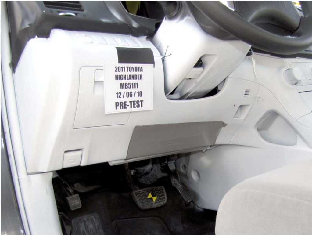
FIGURE 39. Pre-Test Driver's Side Knee Bolster
