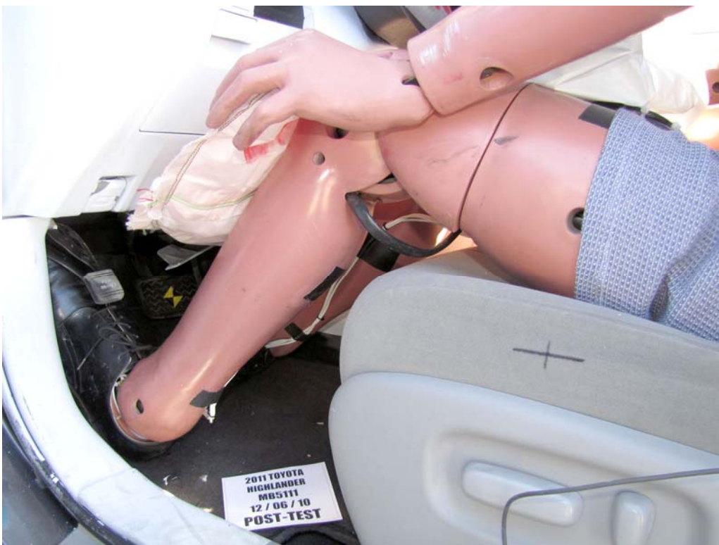
FIGURE 38. Post-Test Driver Dummy Feet
