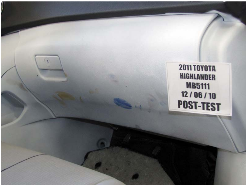
FIGURE 60b. Post-Test Passenger Dummy Contact With Glovebox
