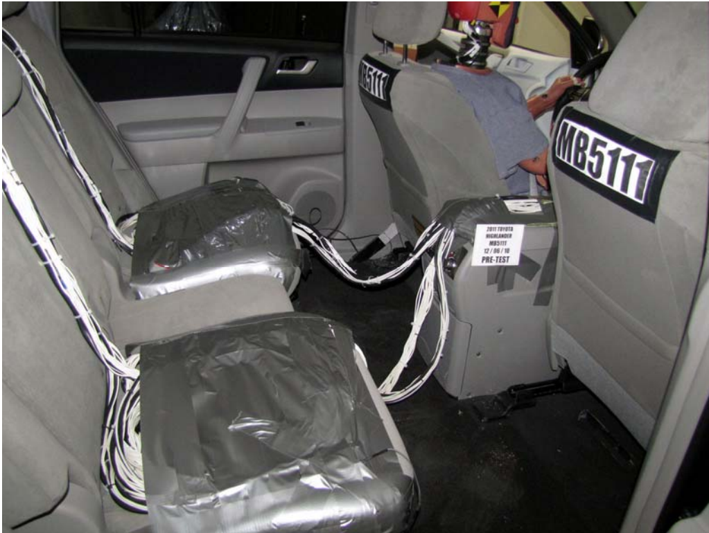
FIGURE 27. Pre-Test Dummy Cable Routing
