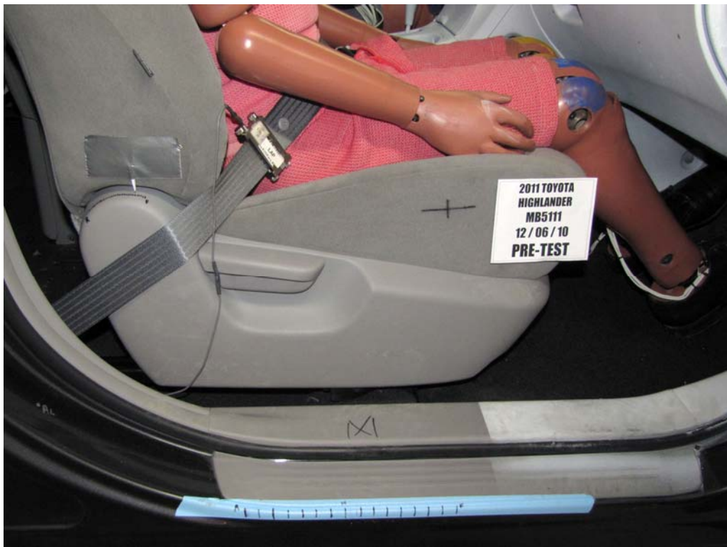
FIGURE 52. Pre-Test Passenger's Seat Fore-Aft Markings
