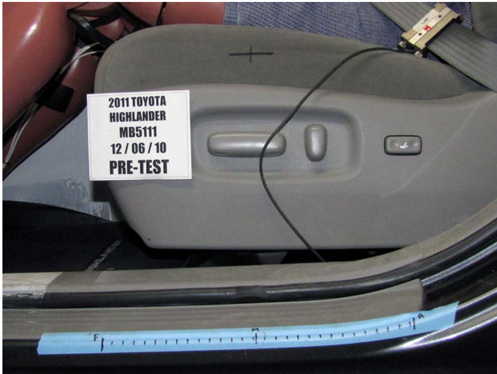
FIGURE 35. Pre-Test Driver's Seat Fore-Aft Markings
