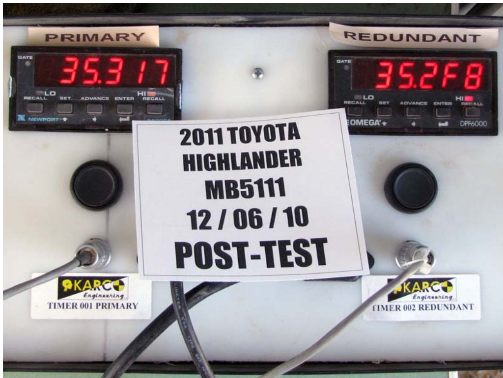
FIGURE 63. Post-Test Speed Trap Read Out
