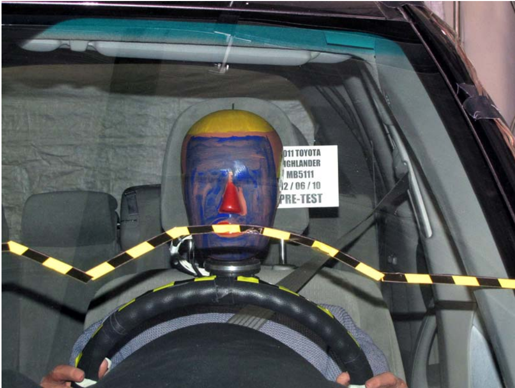
FIGURE 29. Pre-Test Driver Dummy Front View
