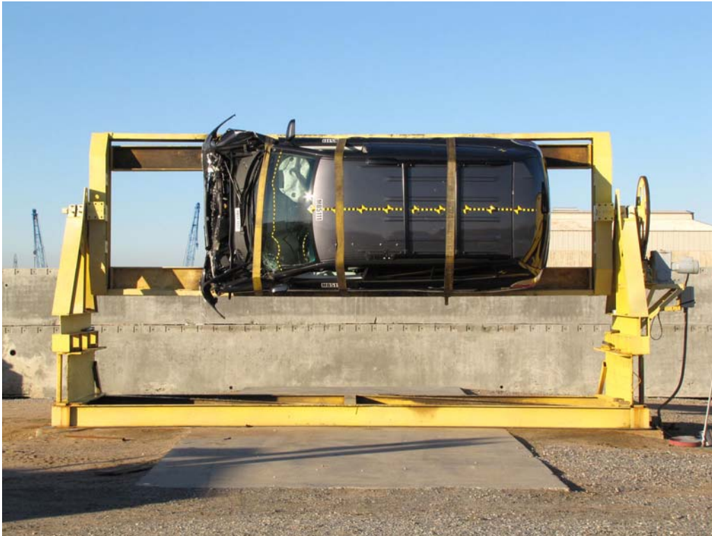
FIGURE 65. Vehicle at 90° on Static Rollover Device
