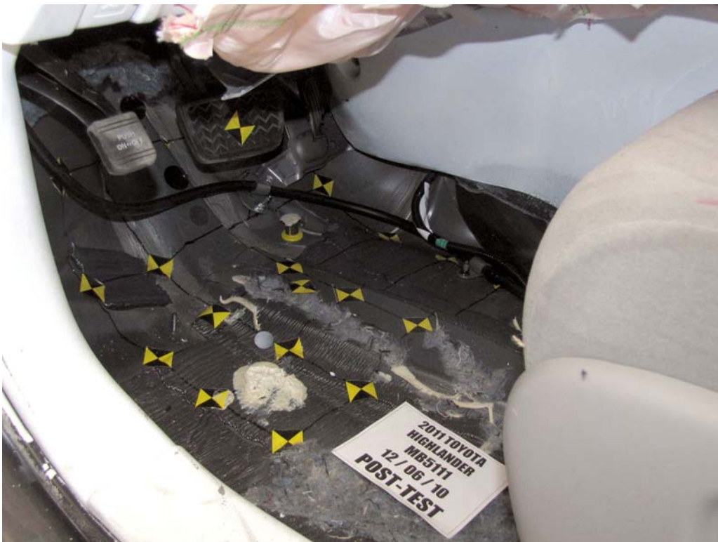
FIGURE 42. Post-Test Driver's Side Floorpan
