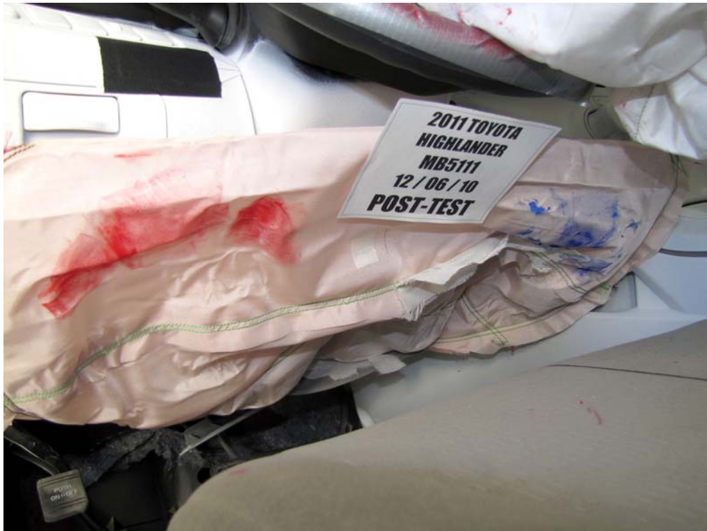
FIGURE 43b. Post-Test Driver Dummy Contact With Knee Airbag
