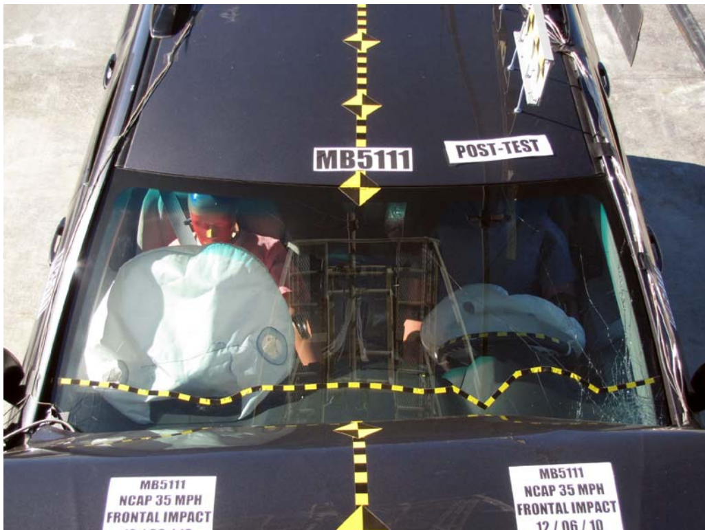
FIGURE 18. Post-Test Windshield View
