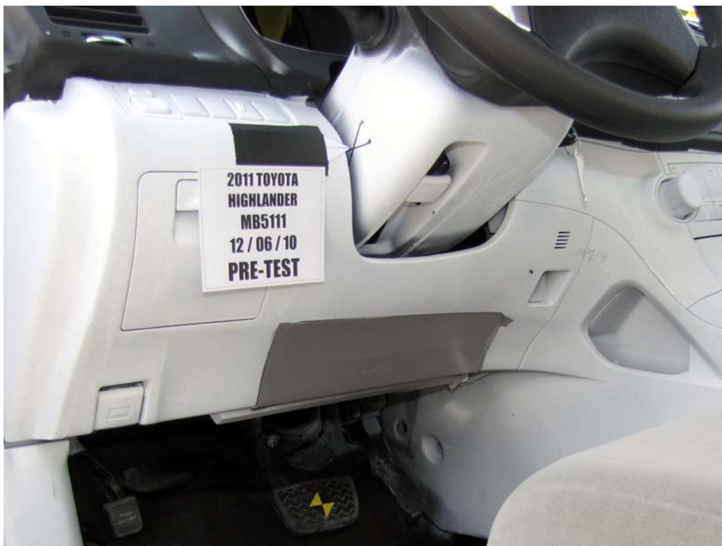
FIGURE 44. Pre-Test View of Steering Column Shear Capsule
