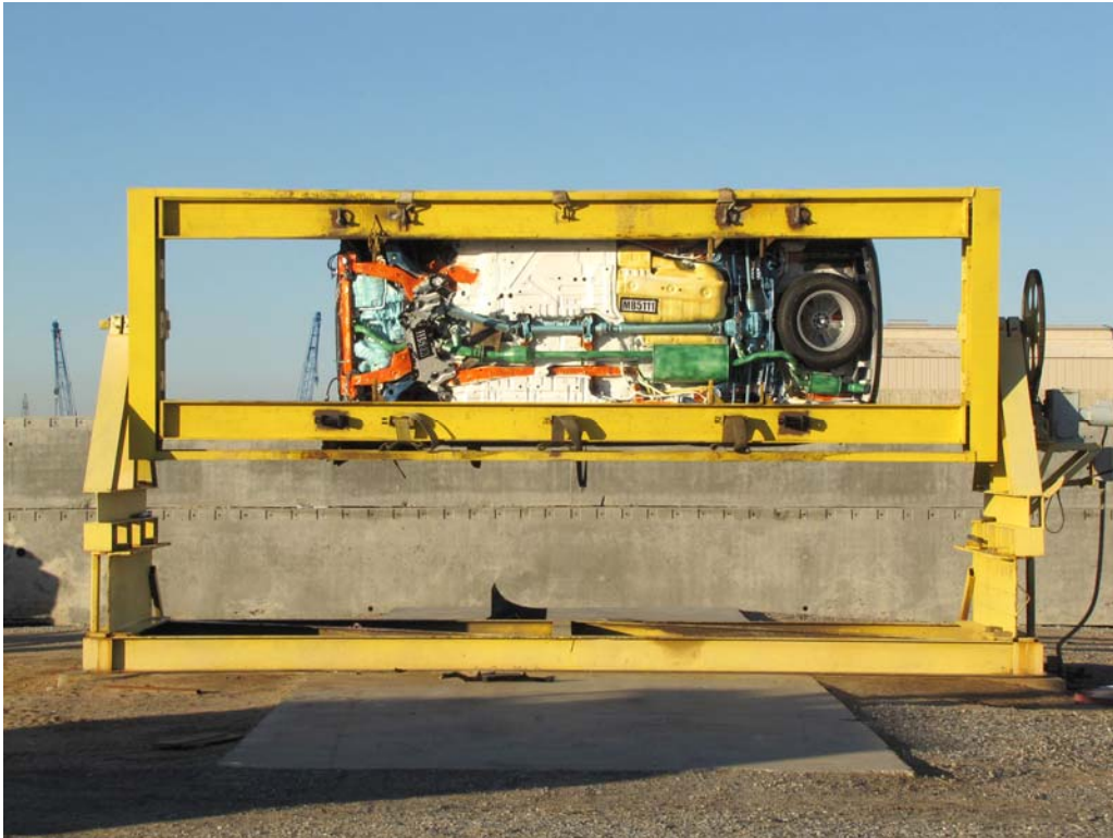
FIGURE 67. Vehicle at 270° on Static Rollover Device
