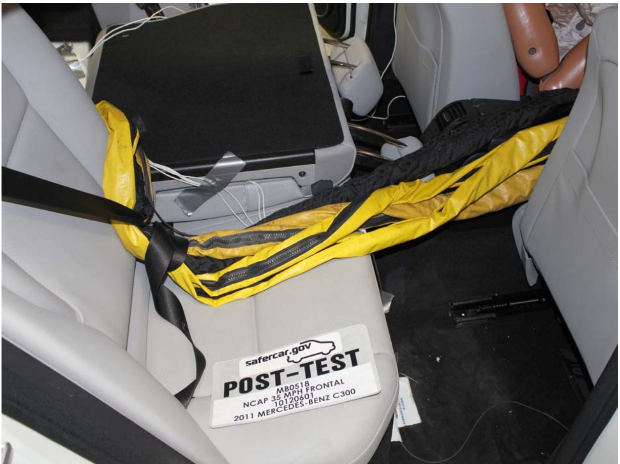
Post-Test Dummy Cable Routing
