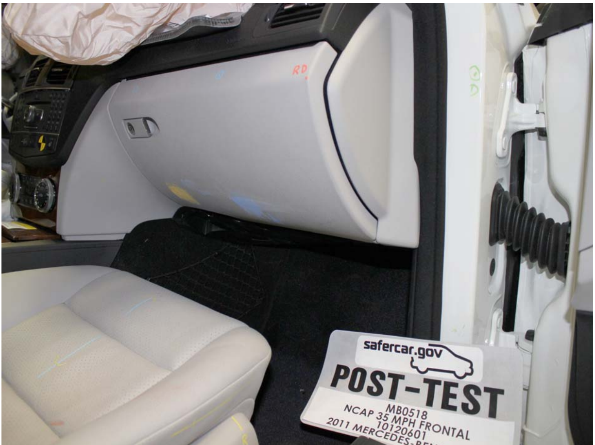
Post-Test Passenger's Side Knee Bolster (without dummy)
