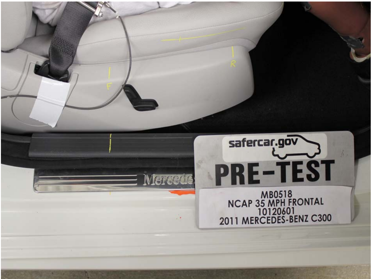
Pre-Test Passenger's Seat Fore-Aft Markings
