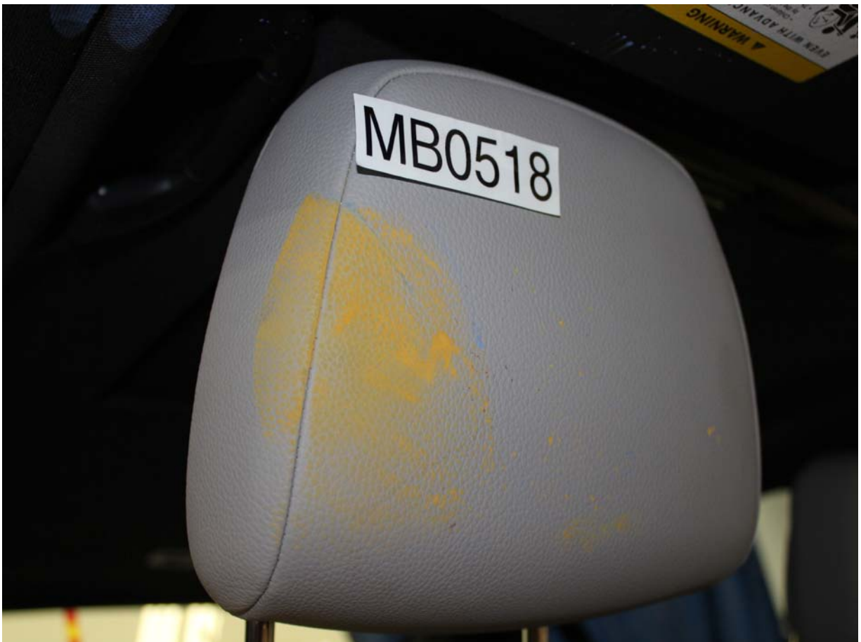
Post-Test Passenger Dummy Contact with Headrest
