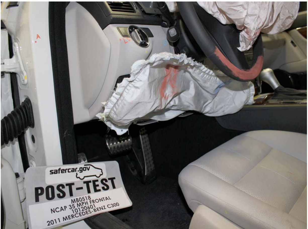
Post-Test Driver's Side Knee Bolster (without dummy)
