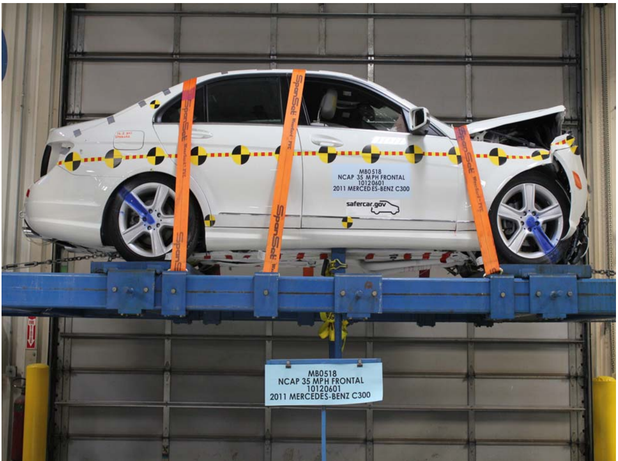
Vehicle at 360 Degrees on Static Rollover Device
