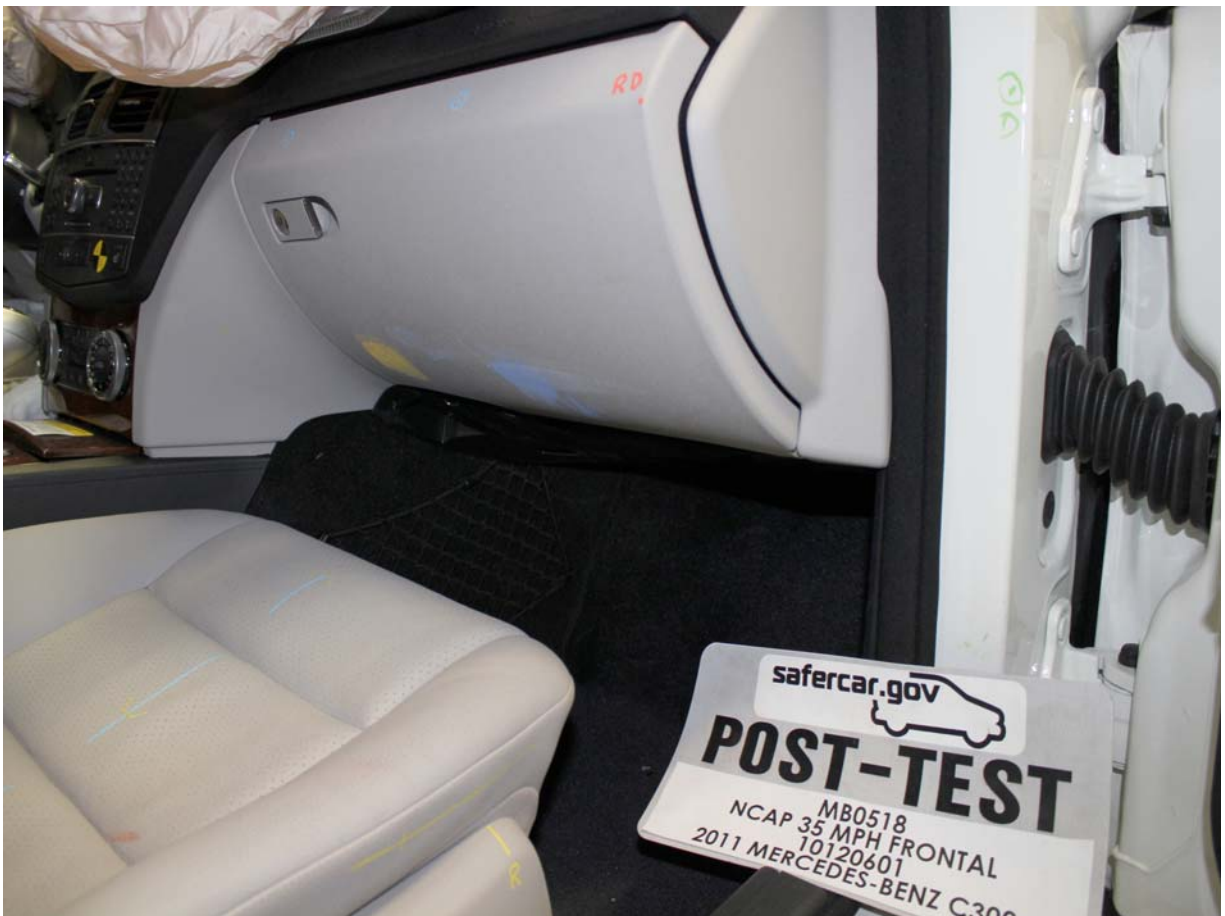
Post-Test Passenger Dummy Contact with Glovebox
