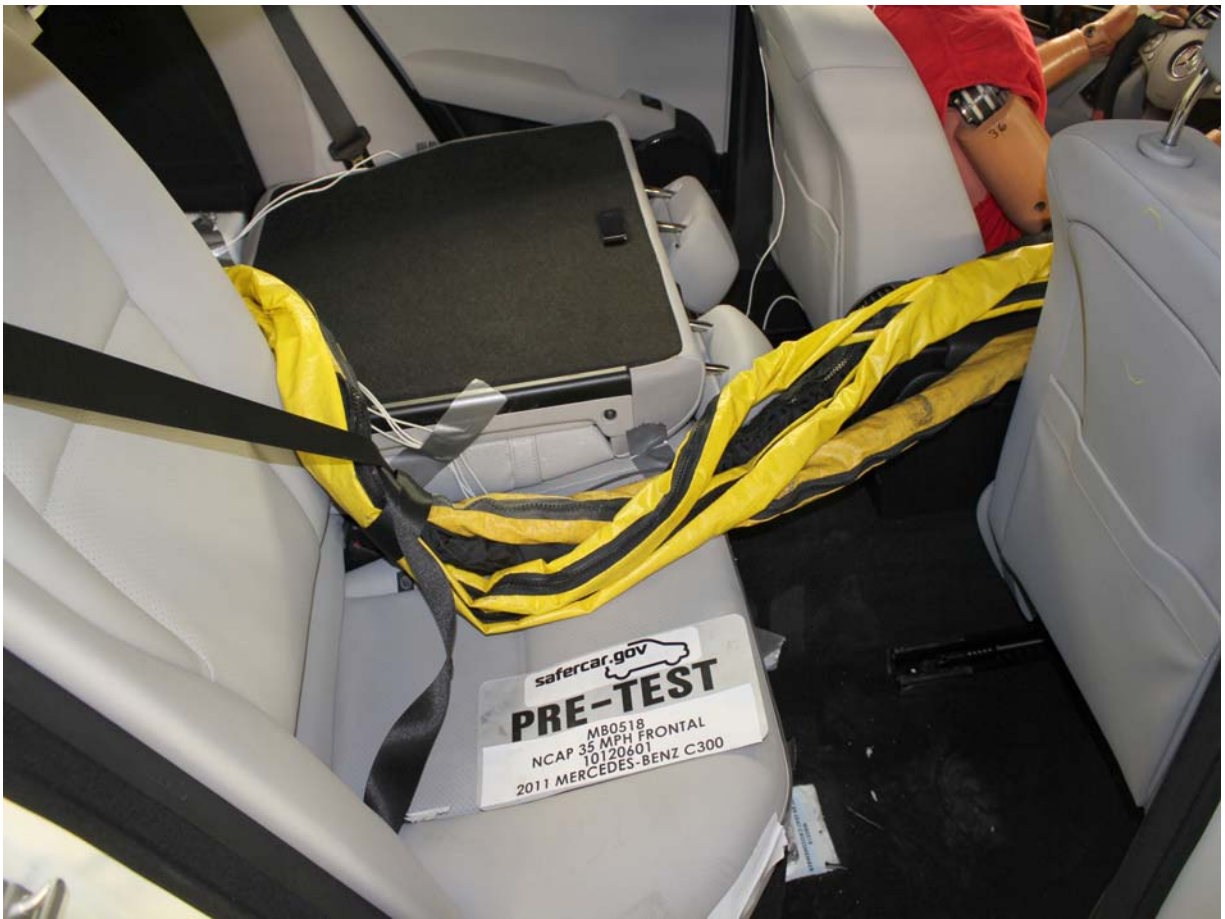
Pre-Test Dummy Cable Routing
