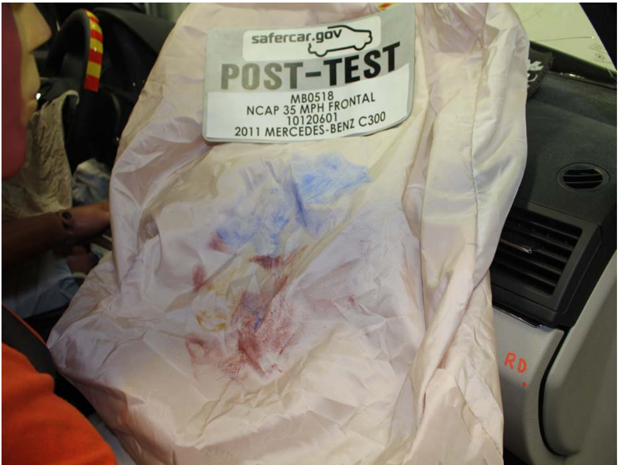
Post-Test Passenger Dummy Contact with Airbag
