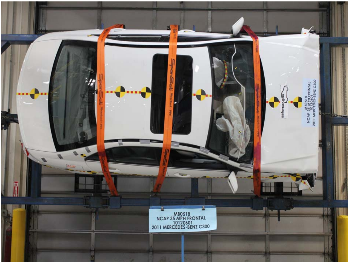
Vehicle at 90 Degrees on Static Rollover Device
