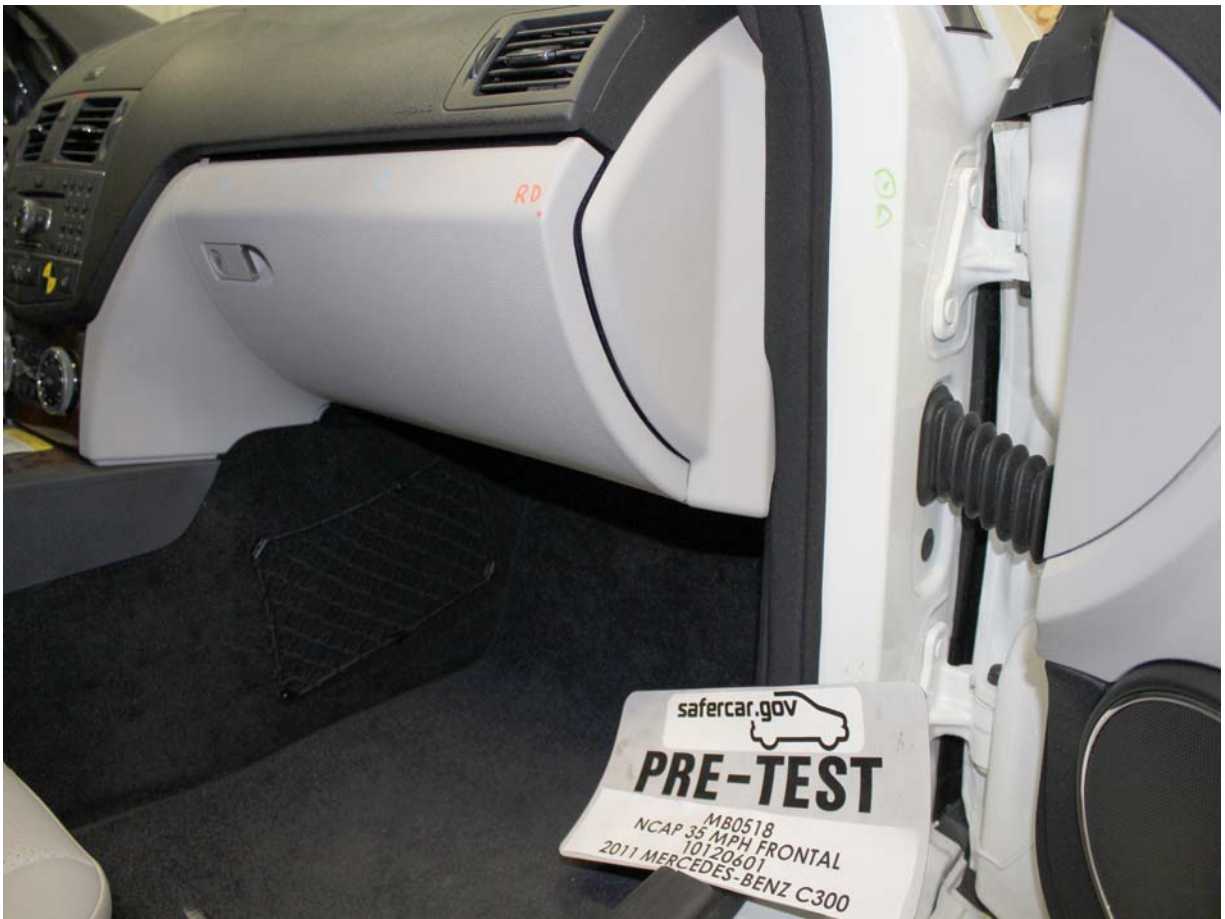
Pre-Test Passenger's Side Knee Bolster (without dummy)
