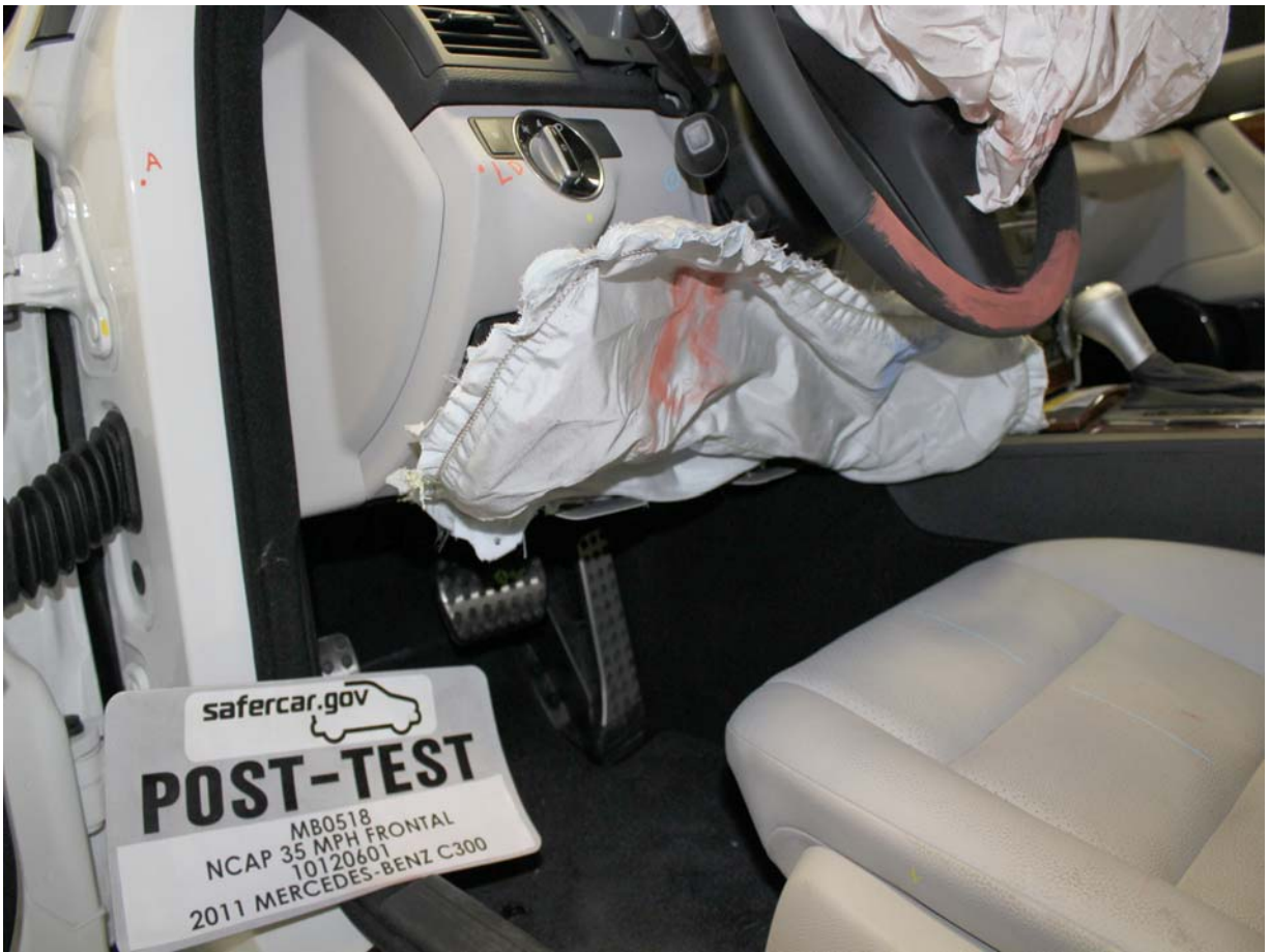
Post-Test Driver Dummy Contact with Knee Airbag
