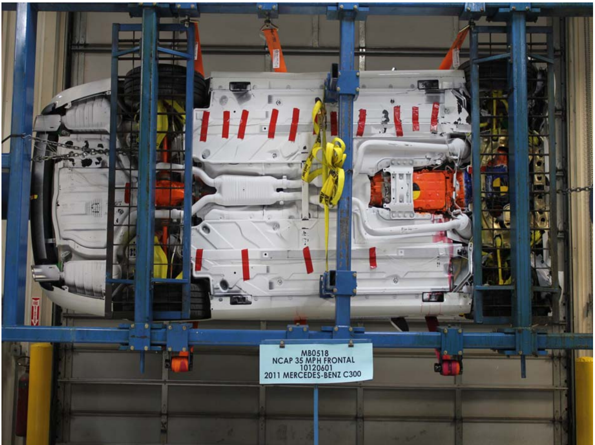
Vehicle at 270 Degrees on Static Rollover Device
