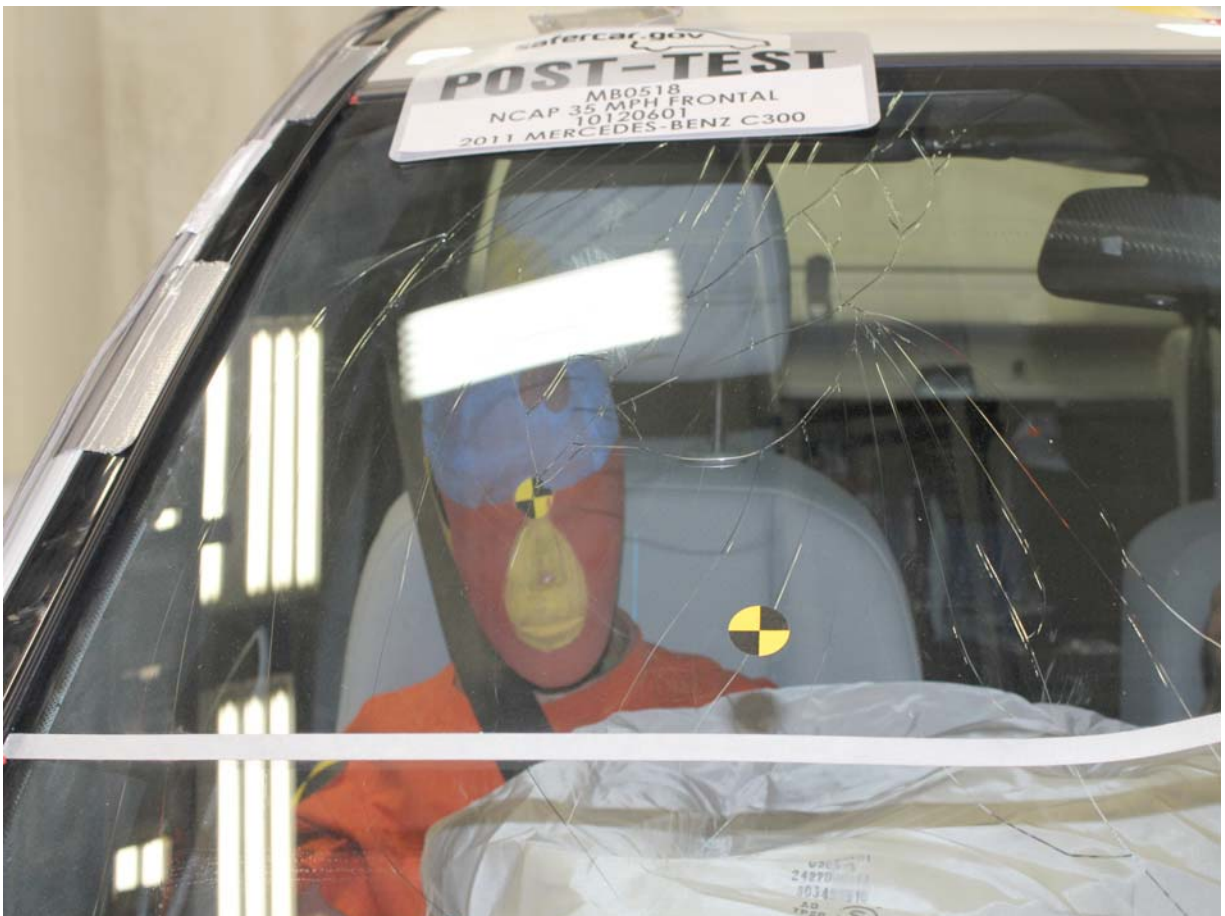
Post-Test Passenger Dummy Front View
