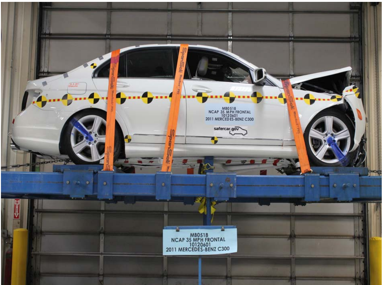
Vehicle at 0 Degrees on Static Rollover Device
