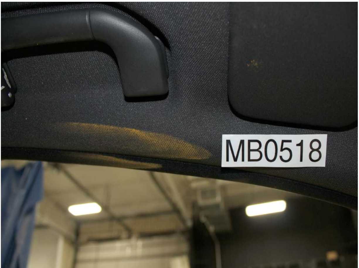
Post-Test Driver Dummy Contact with Side Header
