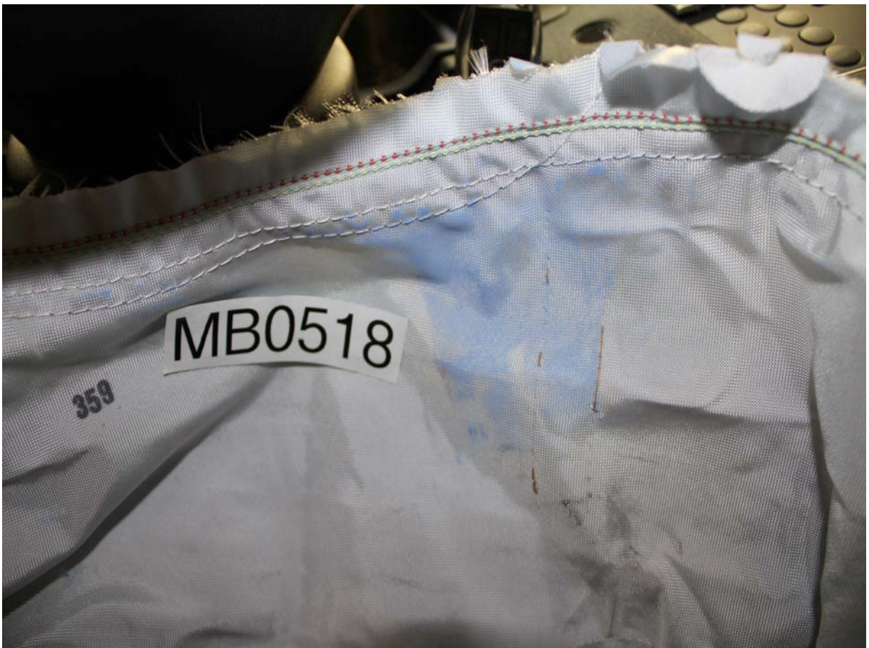
Post-Test Driver Dummy Contact with Knee Airbag
