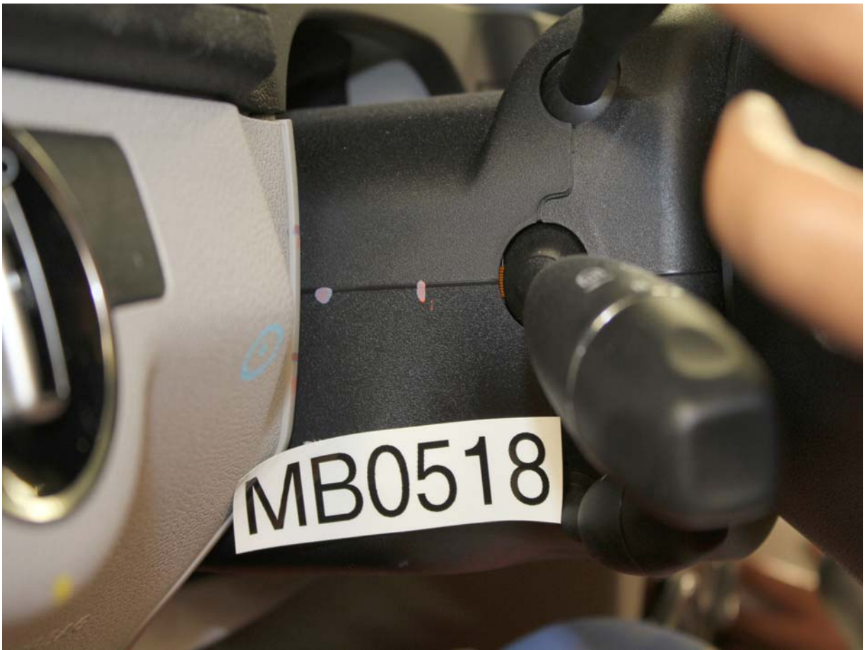
Pre-Test View of Steering Column Shear Capsule
