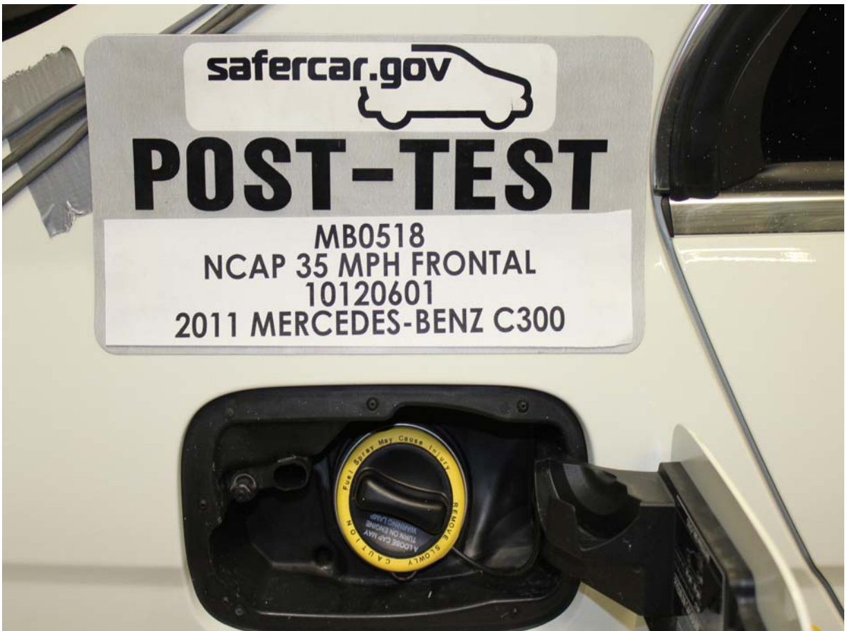
Post-Test Fuel Cap View
