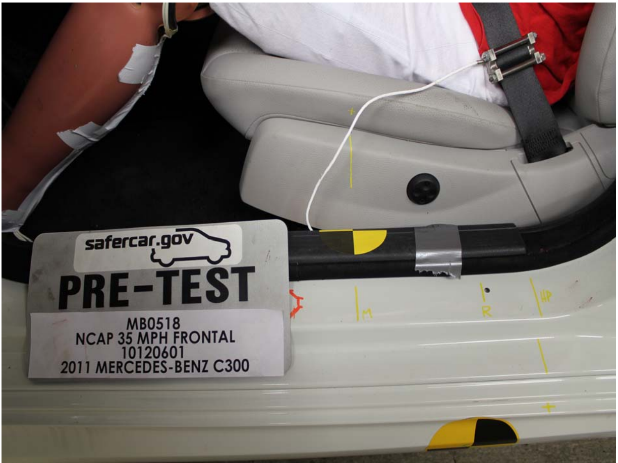
Pre-Test Driver's Seat Fore-Aft Markings
