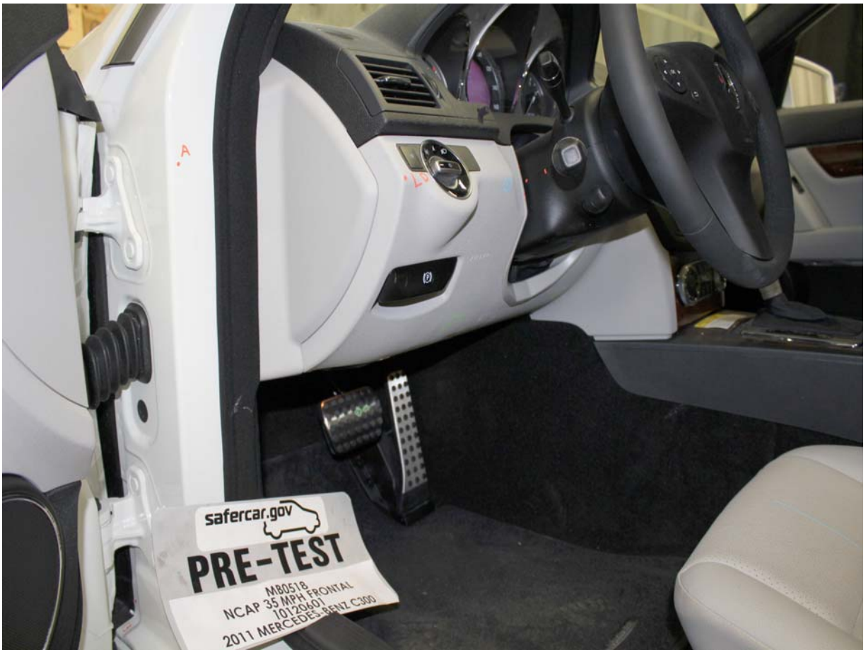
Pre-Test Driver's Side Knee Bolster (without dummy)
