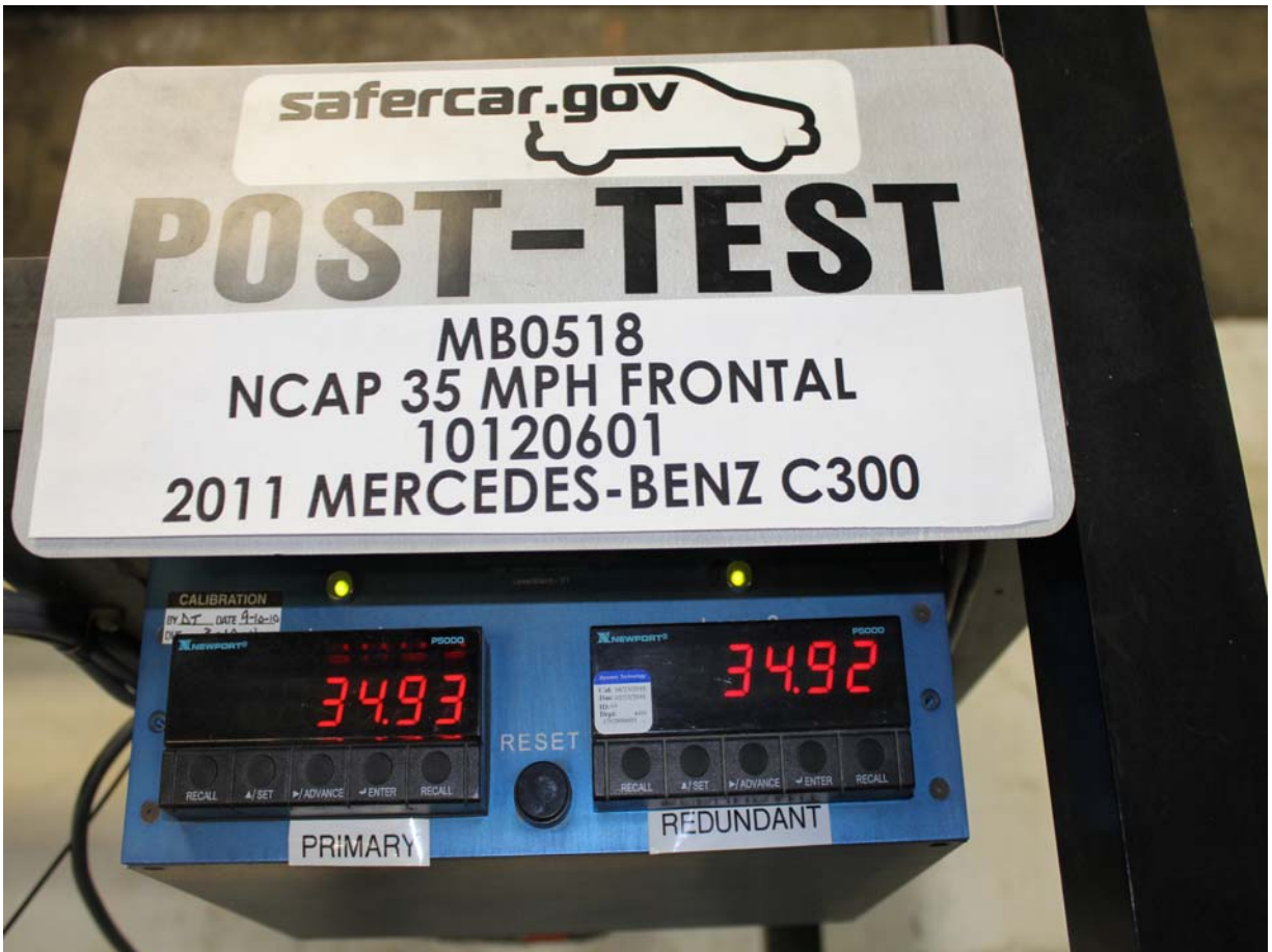
Post-Test Speed Trap Read-Out
