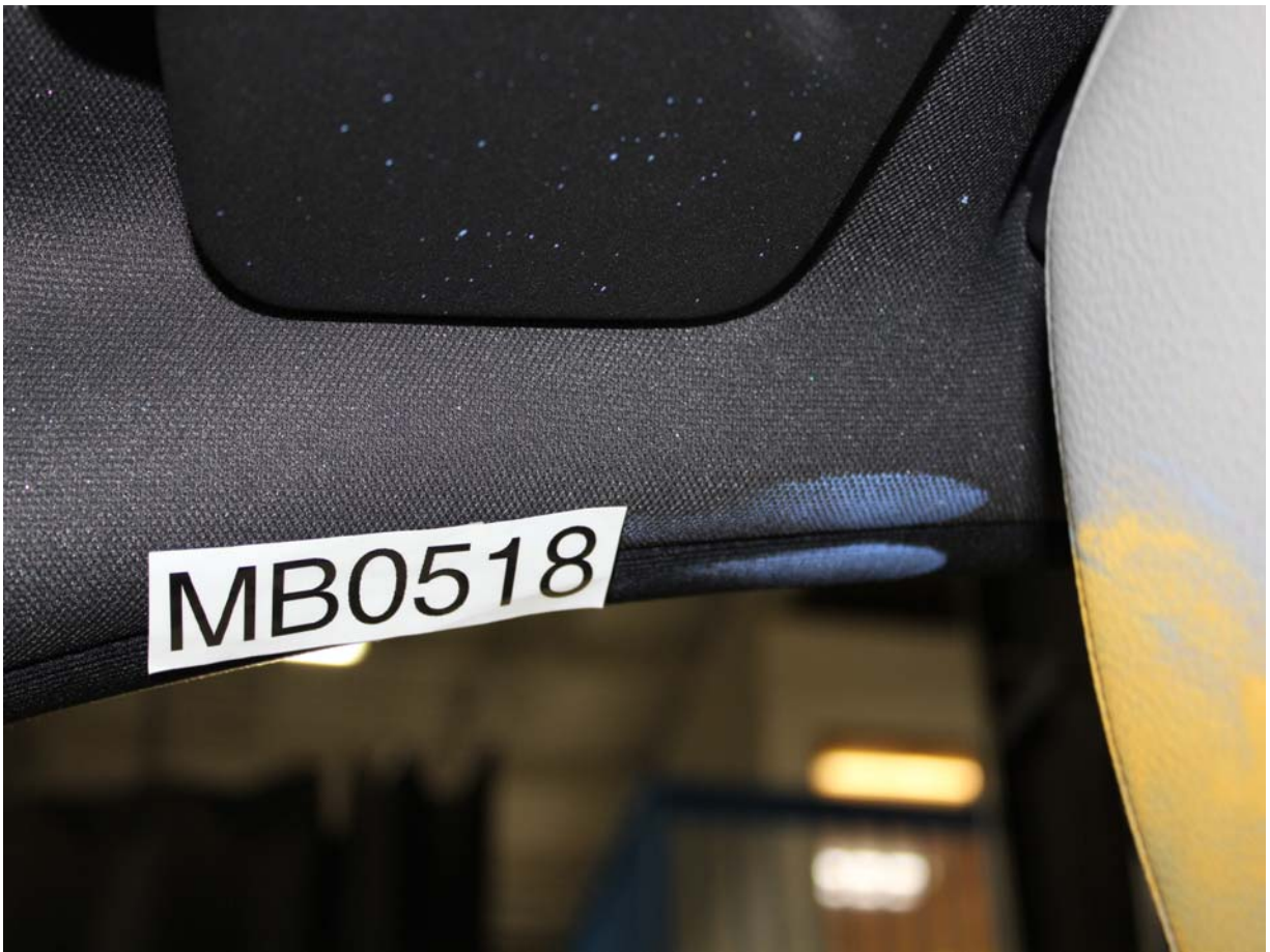
Post-Test Passenger Dummy Contact with Side Header
