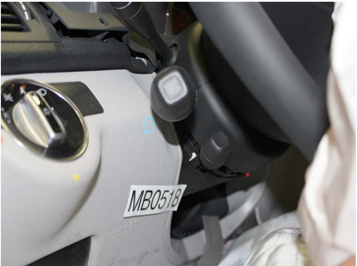
Post-Test View of Steering Column Shear Capsule
