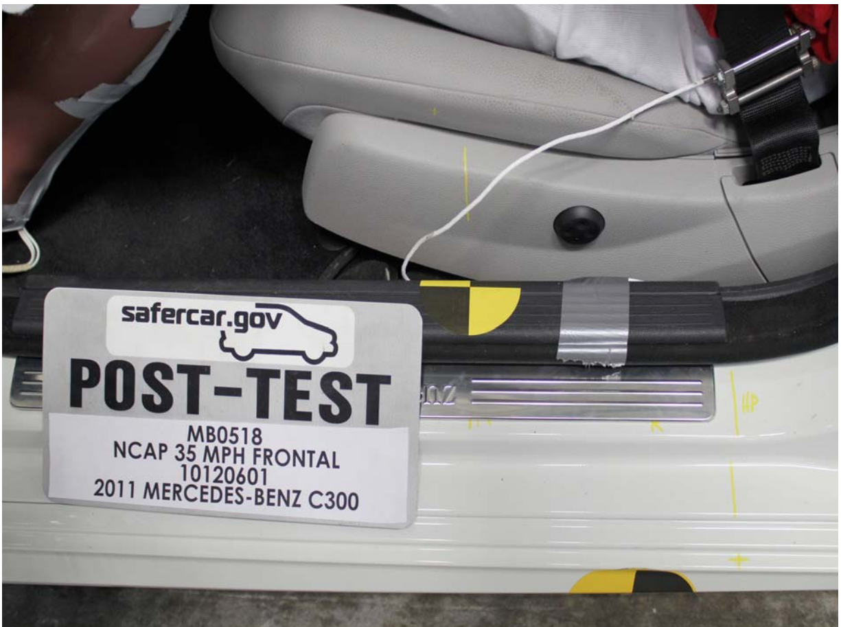
Post-Test Driver's Seat Fore-Aft Markings
