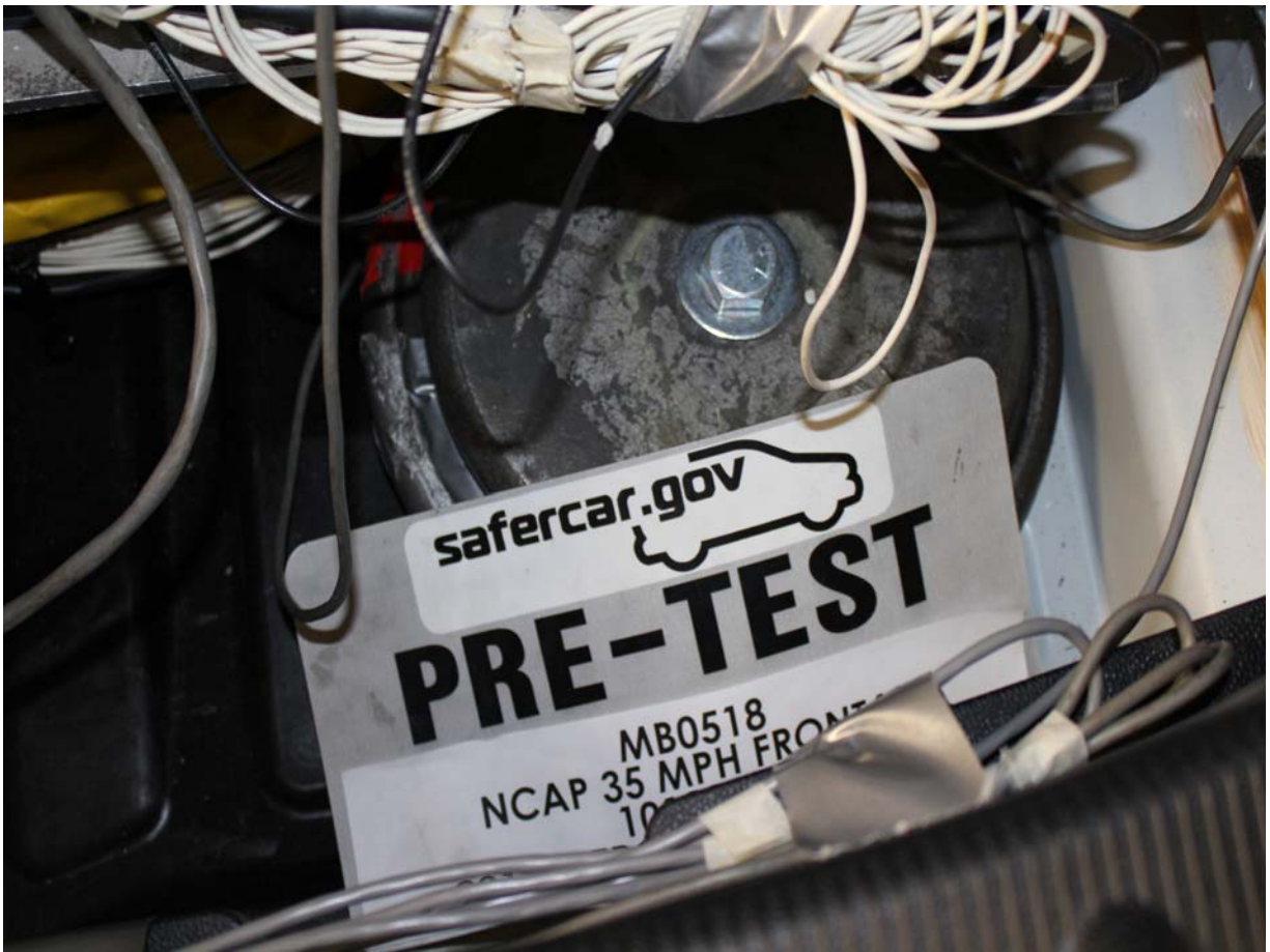
Ballast Installed in Vehicle
