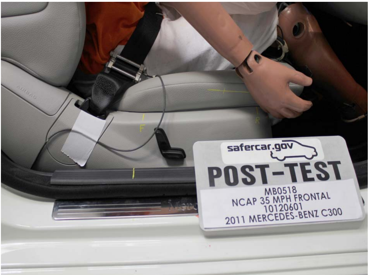
Post-Test Passenger's Seat Fore-Aft Markings
