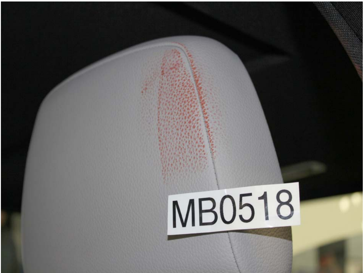
Post-Test Driver Dummy Contact with Headrest
