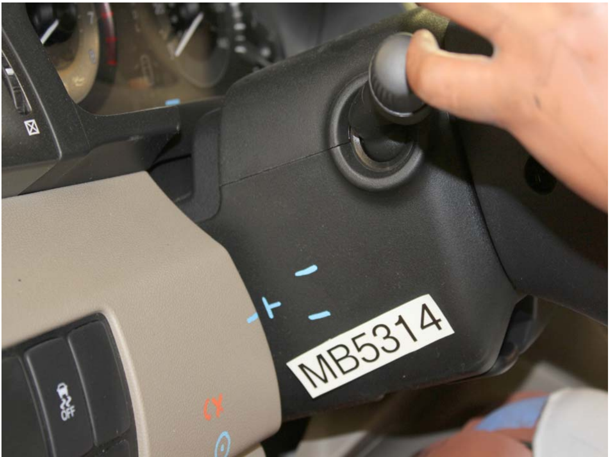
Pre-Test View of Steering Column Shear Capsule
