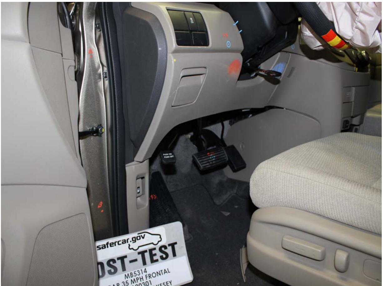
Post-Test Driver Dummy Contact with Knee Bolster
