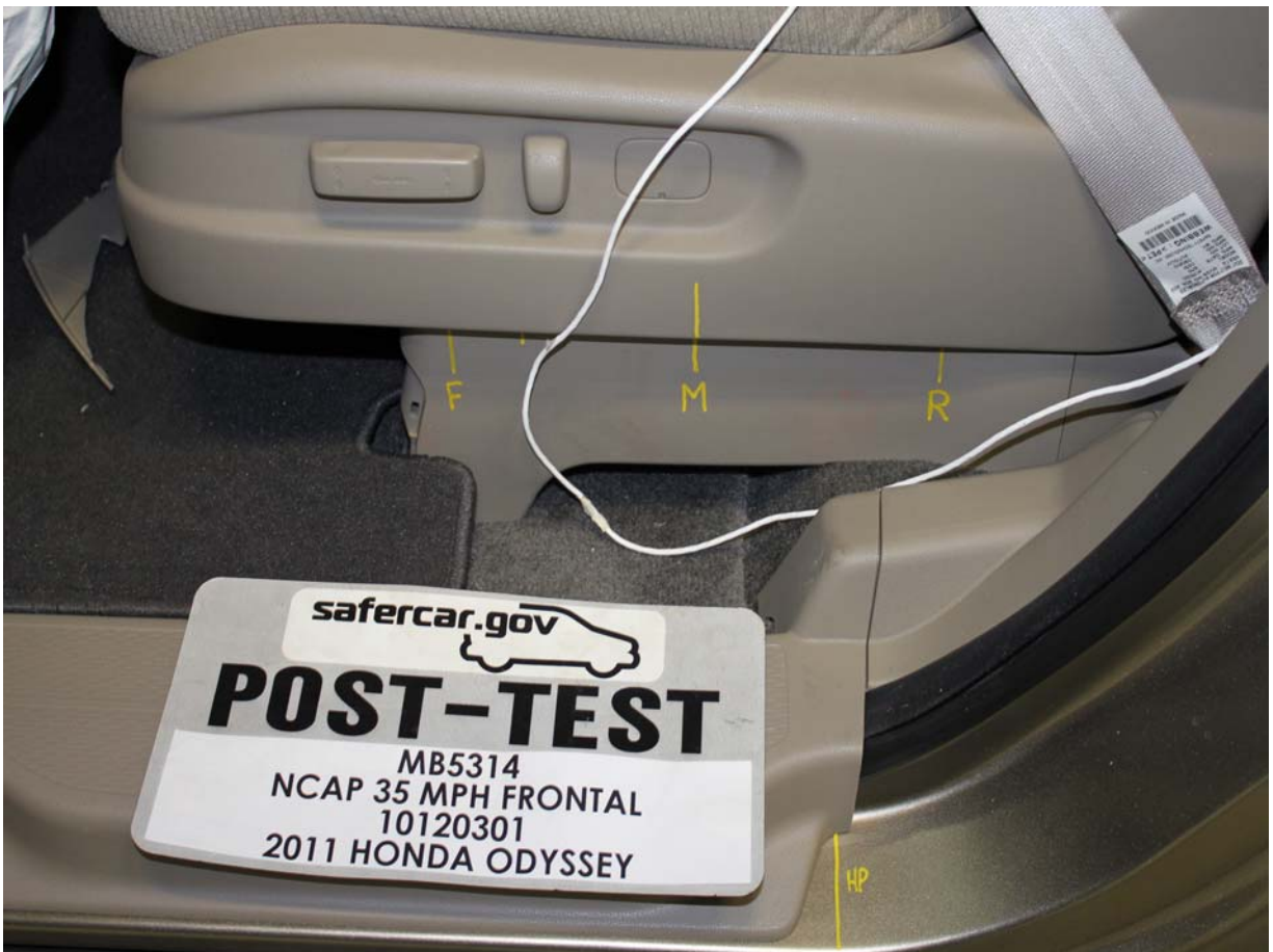
Post-Test Driver's Seat Fore-Aft Markings
