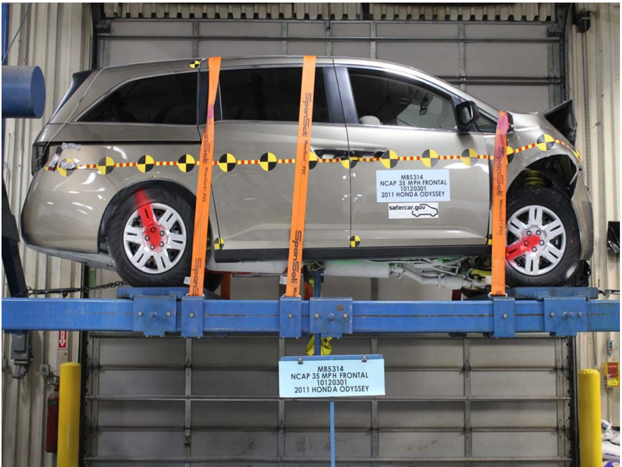
Vehicle at 0 Degrees on Static Rollover Device
