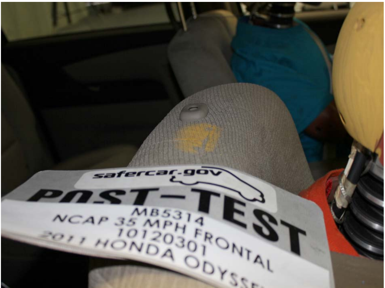
Post-Test Passenger Dummy Contact with Seatback
