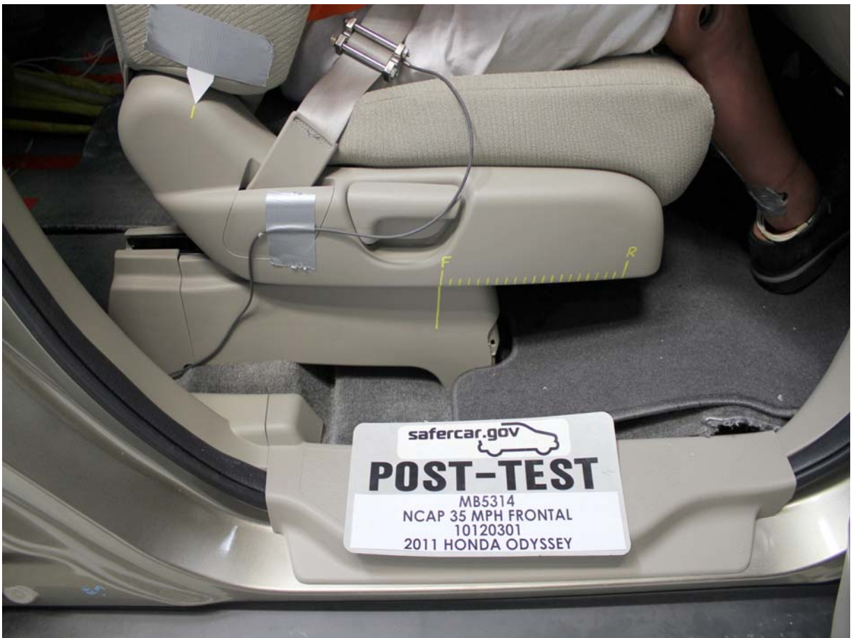
Post-Test Passenger's Seat Fore-Aft Markings
