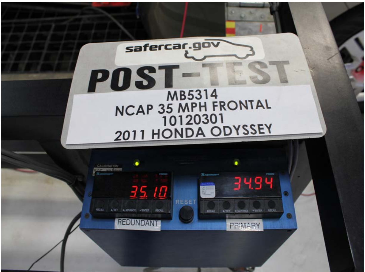
Post-Test Speed Trap Read-Out
