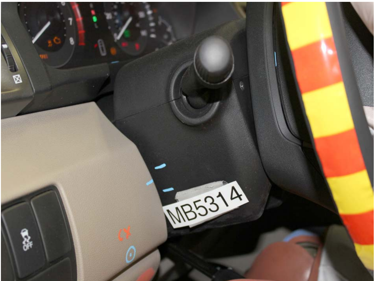
Post-Test View of Steering Column Shear Capsule
