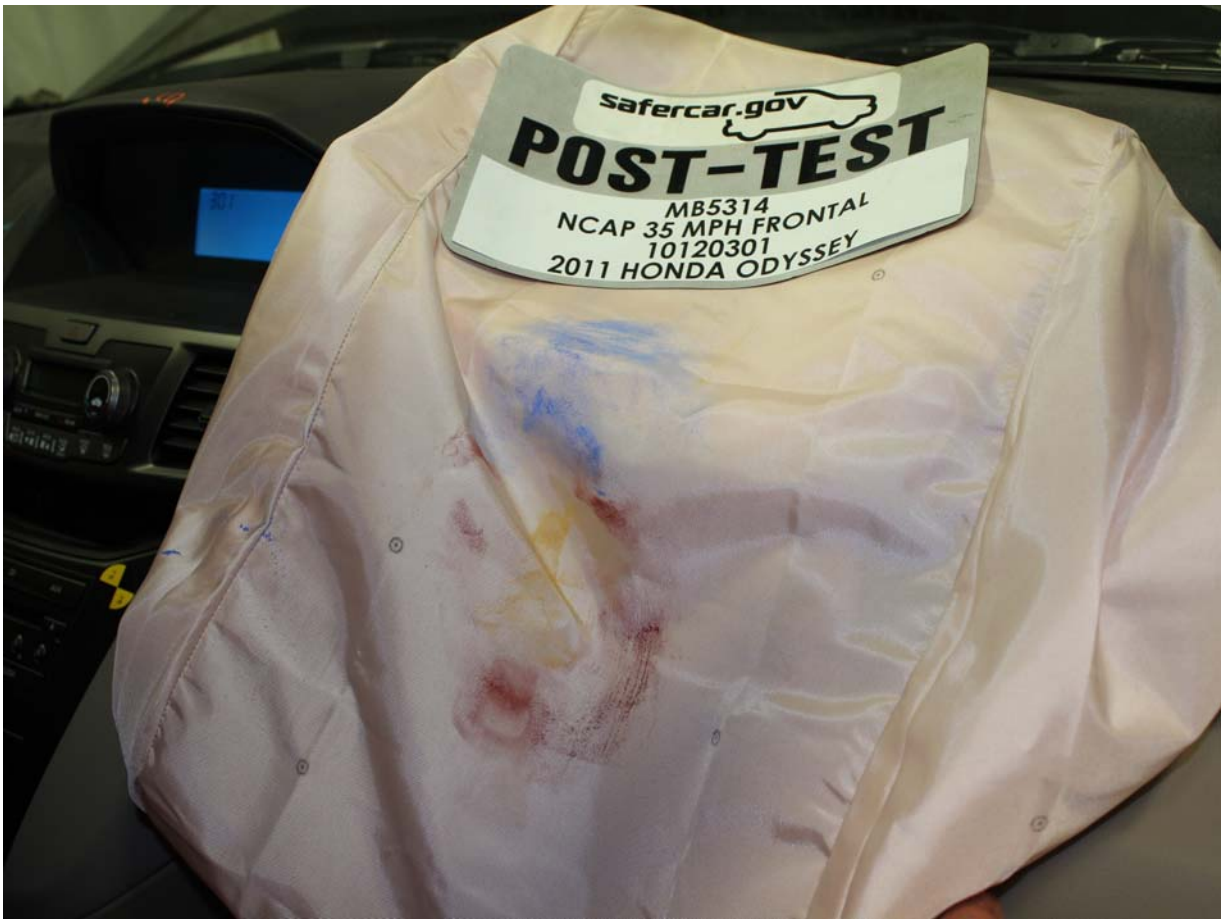
Post-Test Passenger Dummy Contact with Airbag
