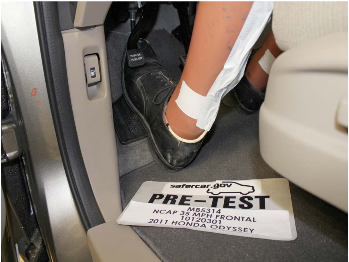
Pre-Test Driver Dummy Feet
