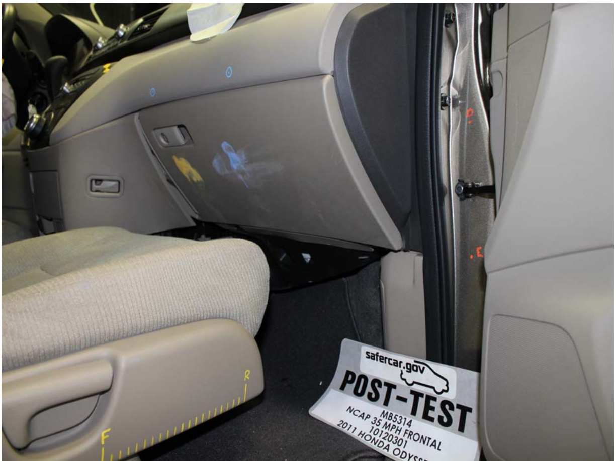
Post-Test Passenger's Side Knee Bolster (without dummy)
