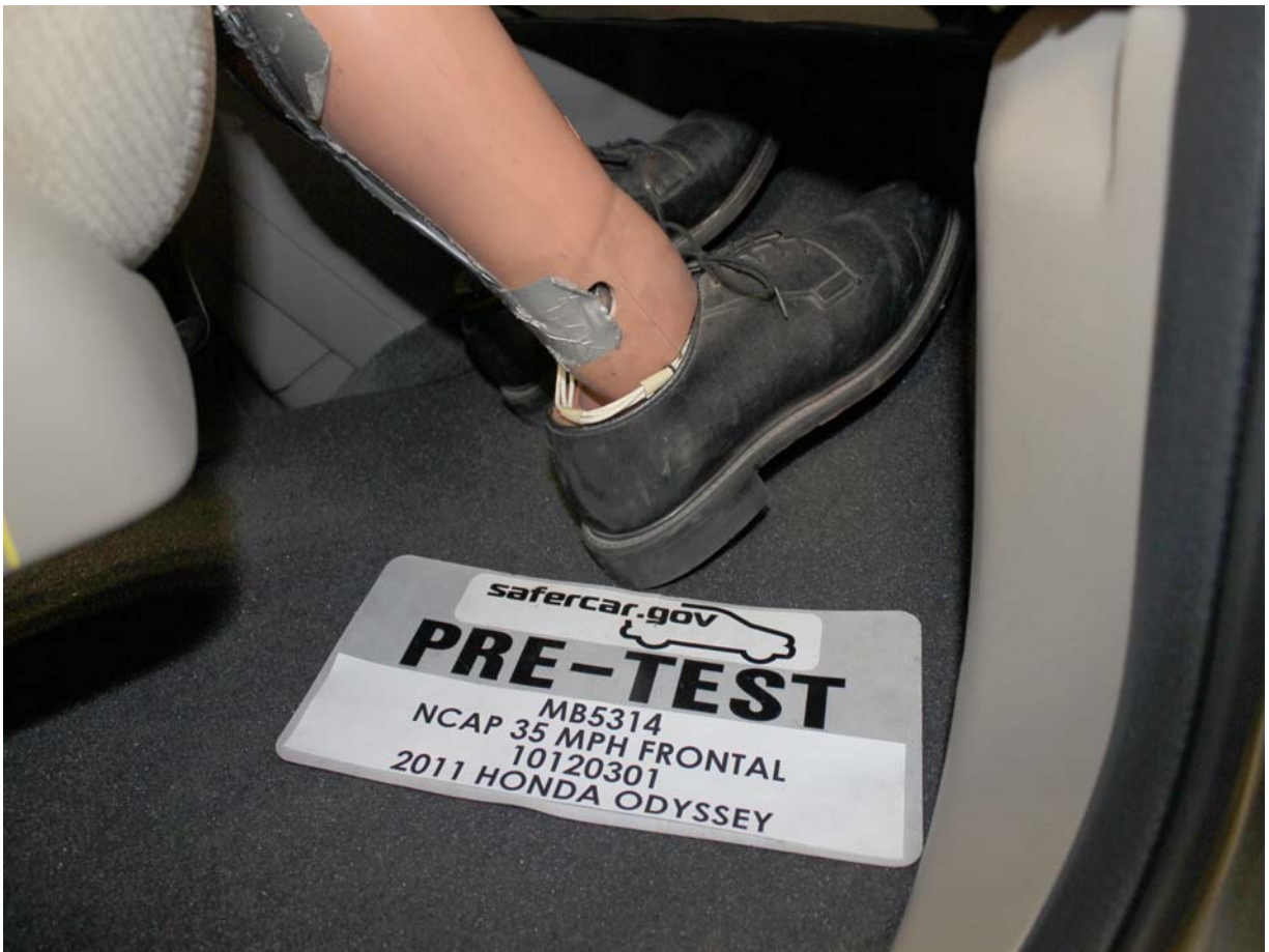
Pre-Test Passenger Dummy Feet
