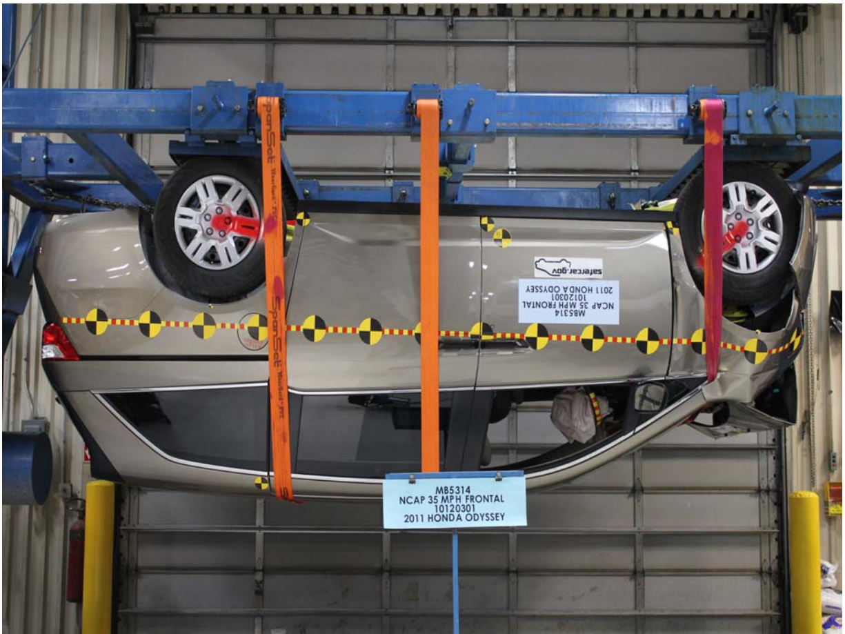
Vehicle at 180 Degrees on Static Rollover Device
