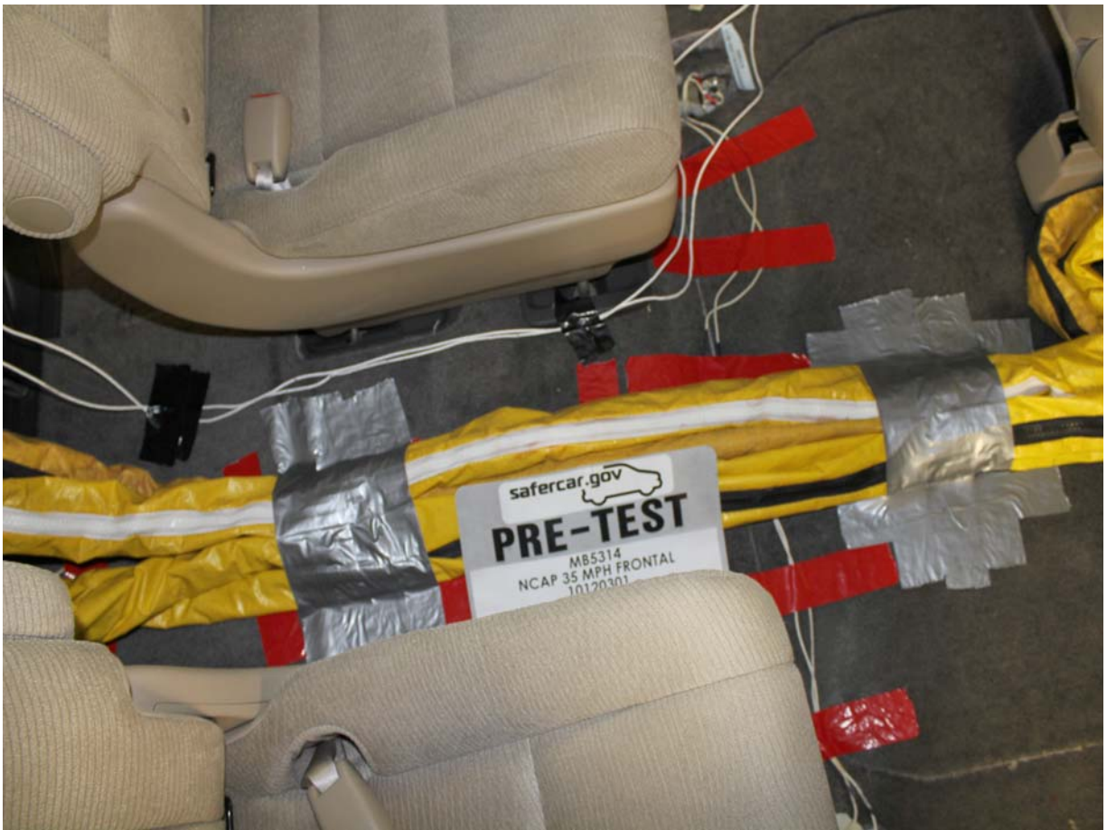
Pre-Test Dummy Cable Routing
