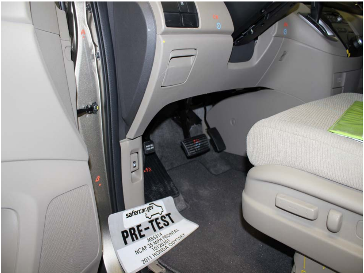
Pre-Test Driver's Side Knee Bolster (without dummy)
