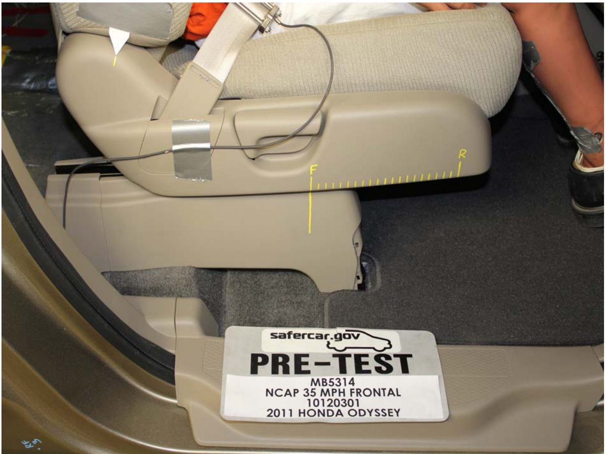
Pre-Test Passenger's Seat Fore-Aft Markings
