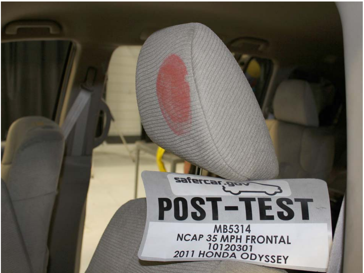
Post-Test Driver Dummy Contact with Headrest
