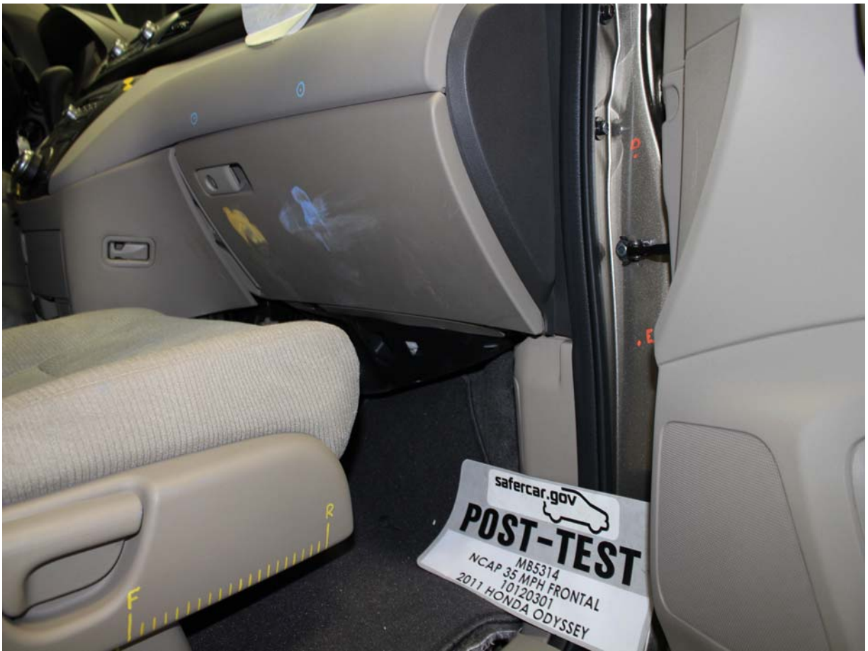
Post-Test Passenger Dummy Contact with Glovebox
