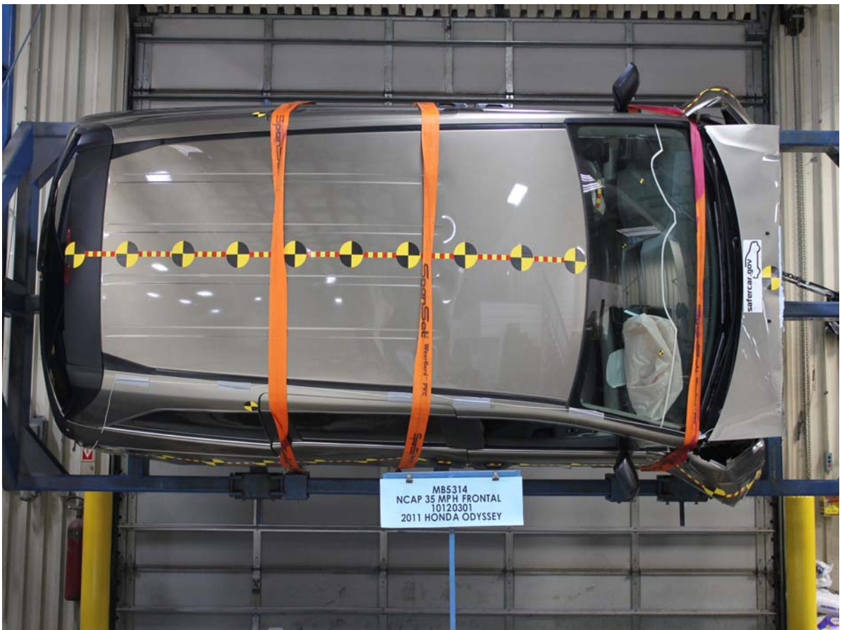
Vehicle at 270 Degrees on Static Rollover Device
