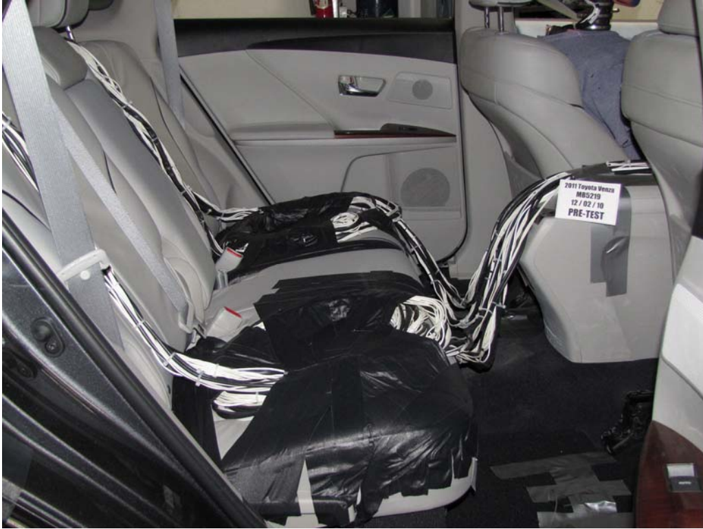
FIGURE 27. Pre-Test Dummy Cable Routing
