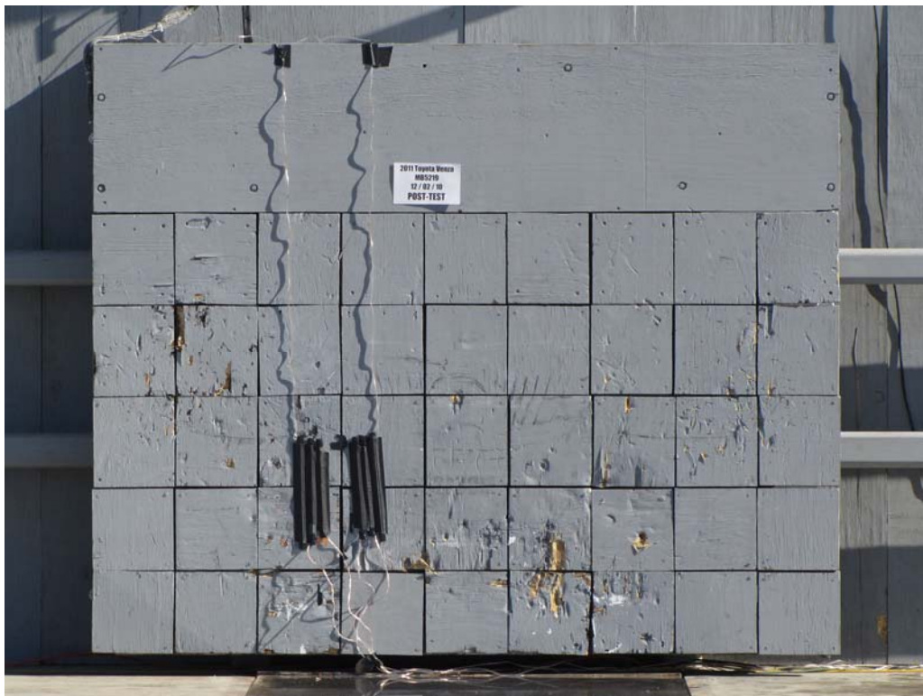
FIGURE 2. Load Cell Wall
