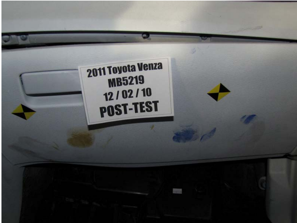
FIGURE 60c. Post-Test Passenger Dummy Contact With Glove Box
