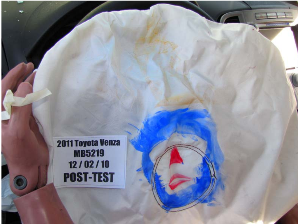
FIGURE 43. Post-Test Driver Dummy Contact With Airbag
