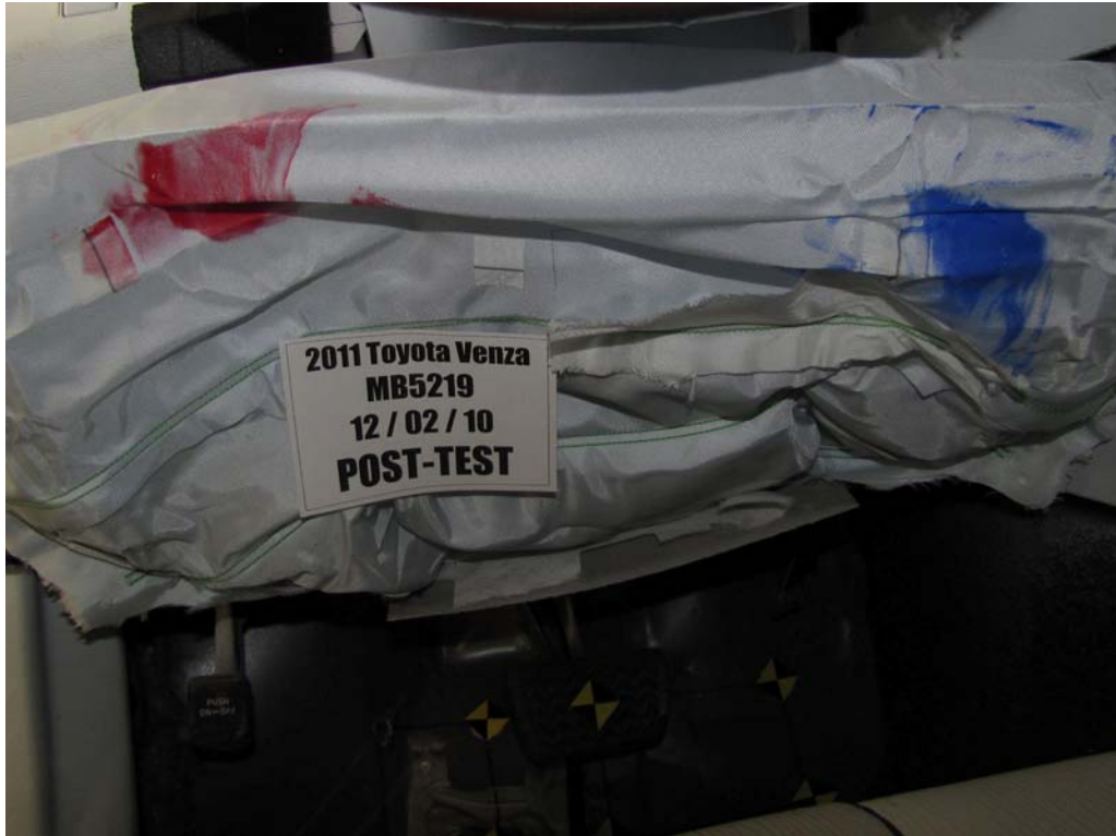
FIGURE 43d. Post-Test Driver Dummy Contact With Knee Airbag
