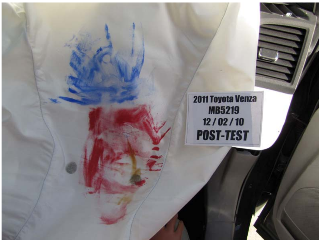
FIGURE 60. Post-Test Passenger Dummy Contact With Airbag
