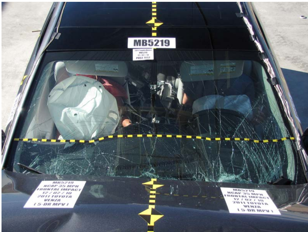
FIGURE 18. Post-Test Windshield View
