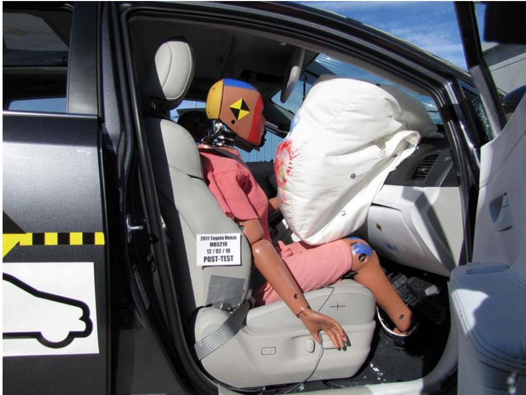
FIGURE 51. Post-Test Passenger Dummy and Vehicle Interior View
