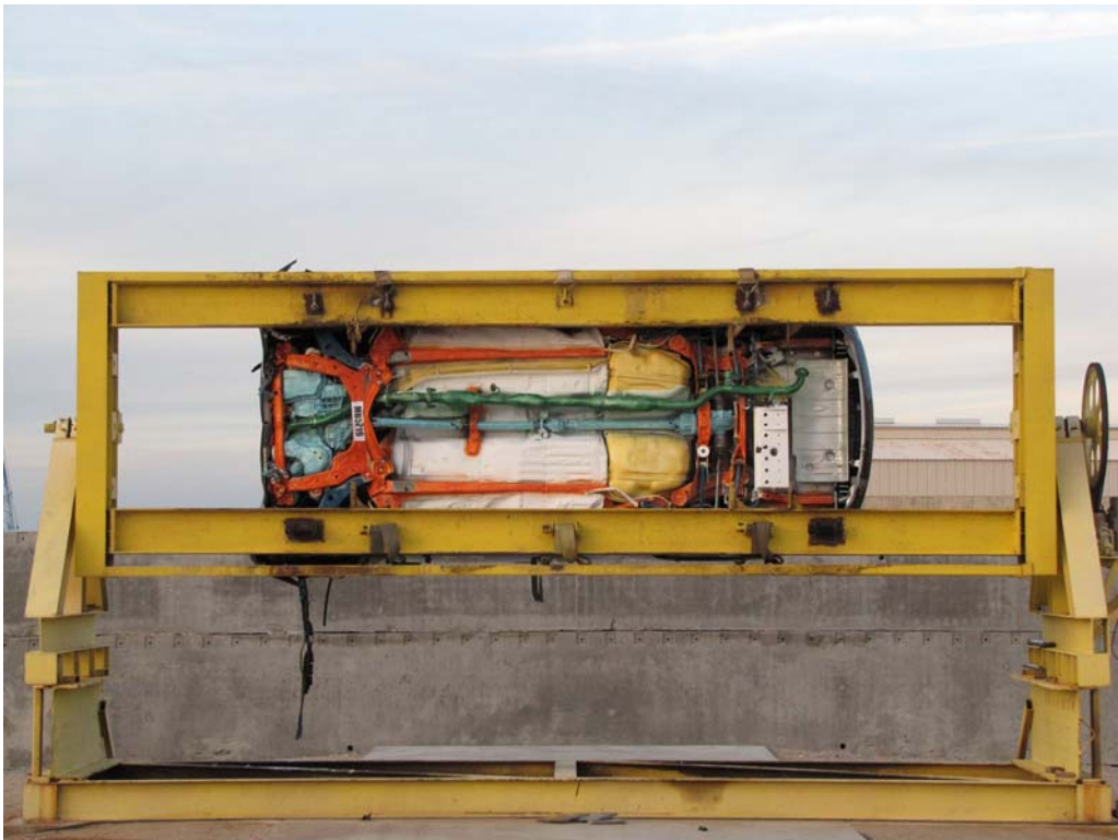
FIGURE 67. Vehicle at 270 Degrees on Static Rollover Device
