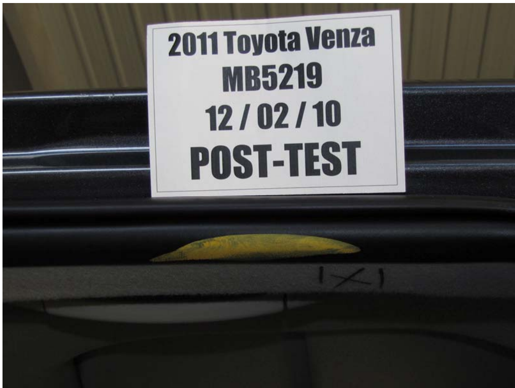
FIGURE 43c. Post-Test Driver Dummy Contact With Side Header
