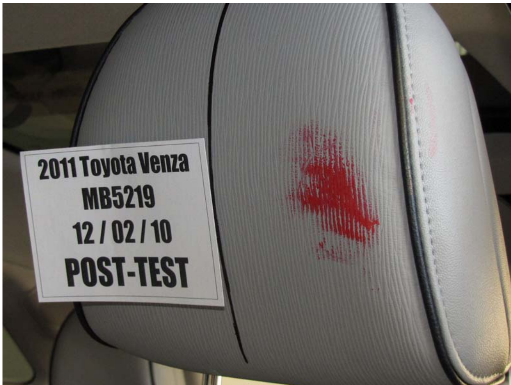
FIGURE 43a. Post-Test Driver Dummy Contact With Head Restraint
