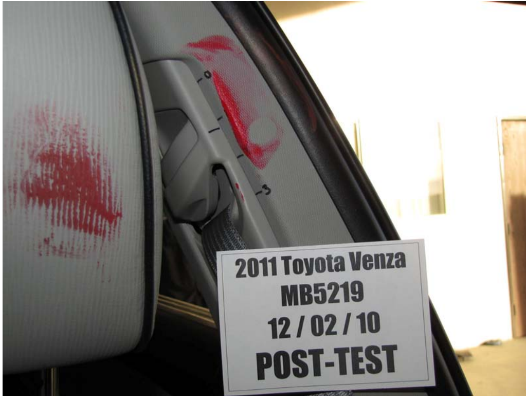
FIGURE 43b. Post-Test Driver Dummy Contact With B-Pillar
