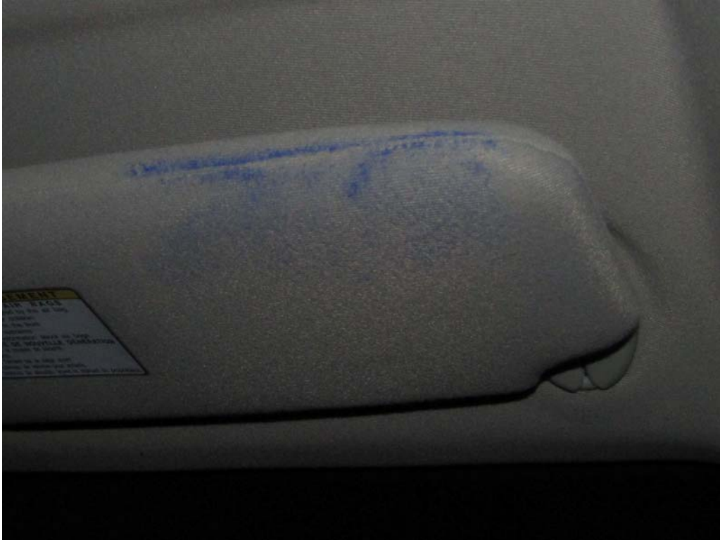
FIGURE 60a. Post-Test Passenger Dummy Contact With Sun Visor
