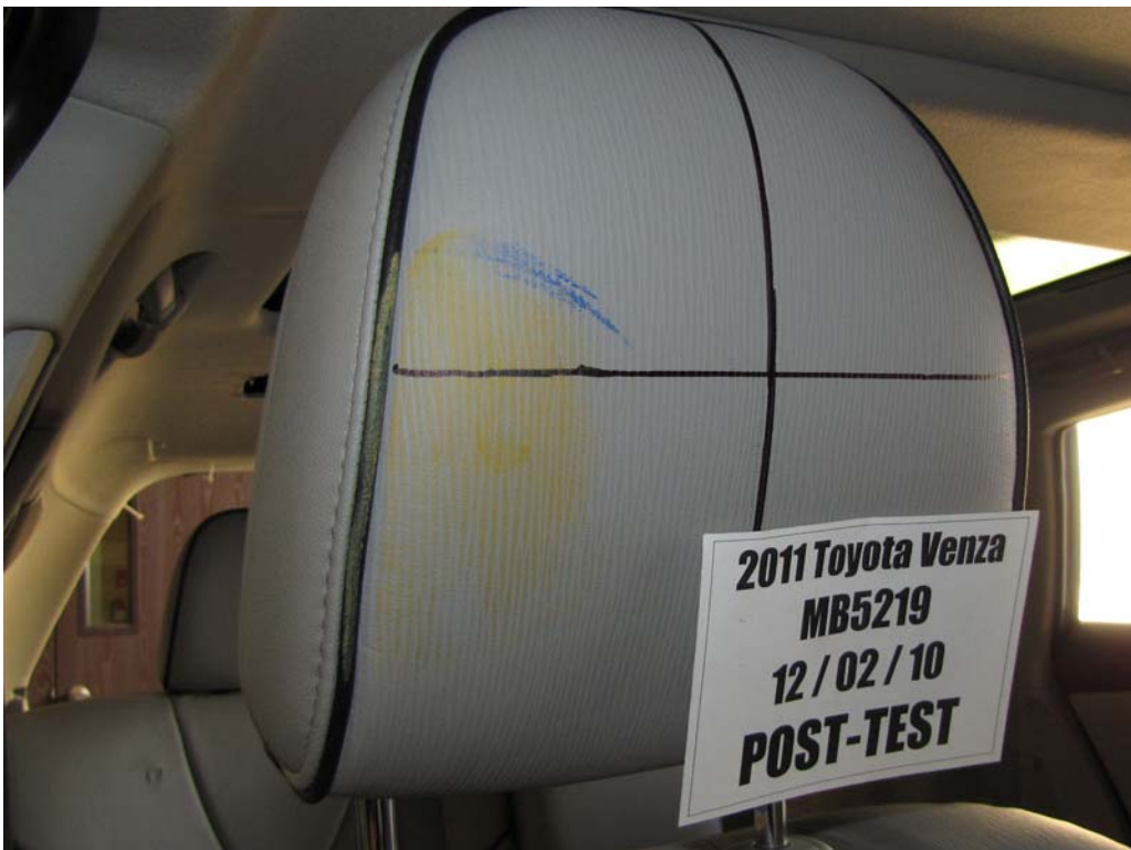
FIGURE 60b. Post-Test Passenger Dummy Contact With Head Restraint
