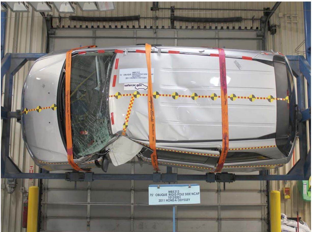
FMVSS No. 301/305 Rollover 90 Degrees
