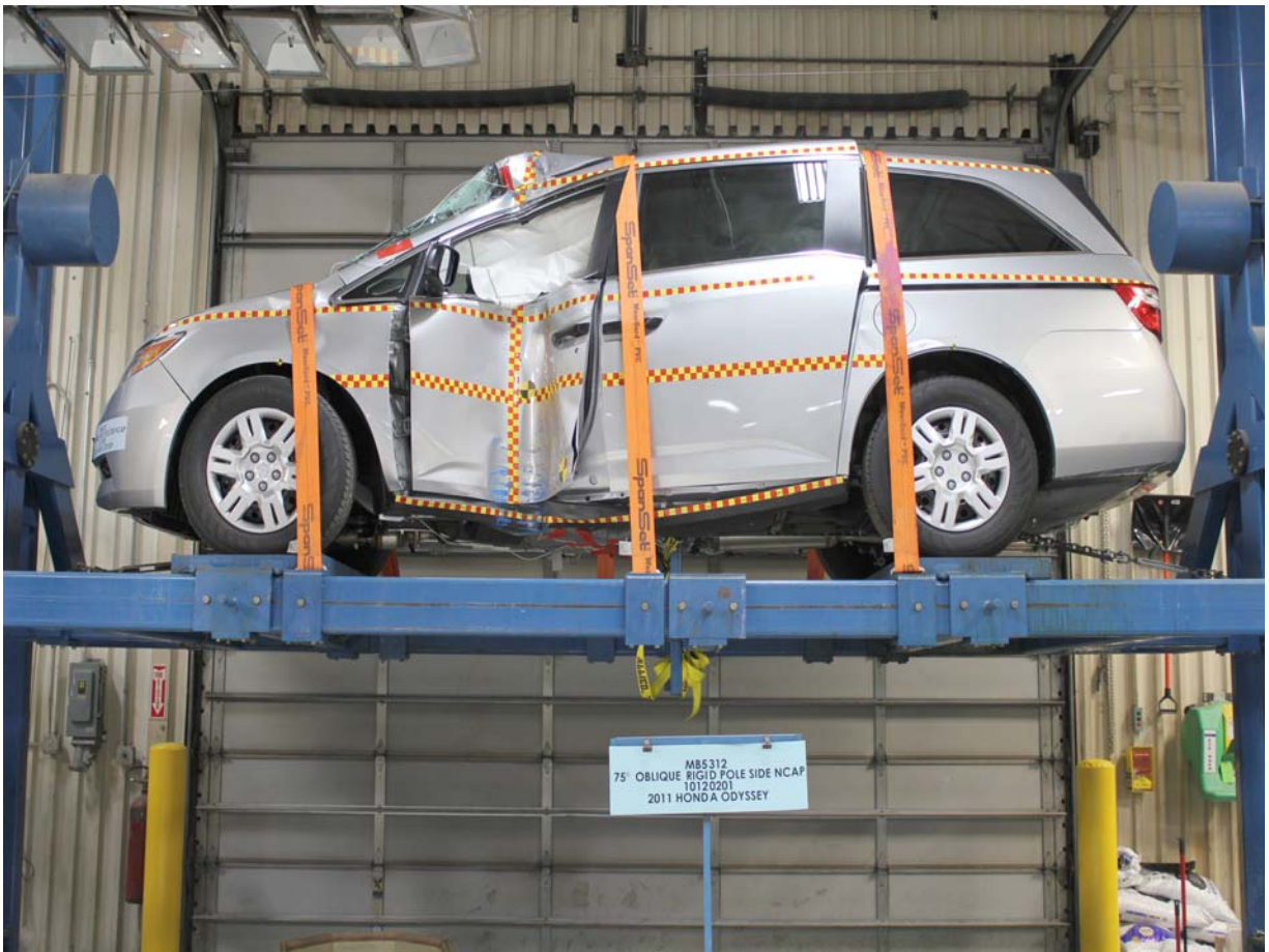
FMVSS No. 301/305 Rollover 360 Degrees
