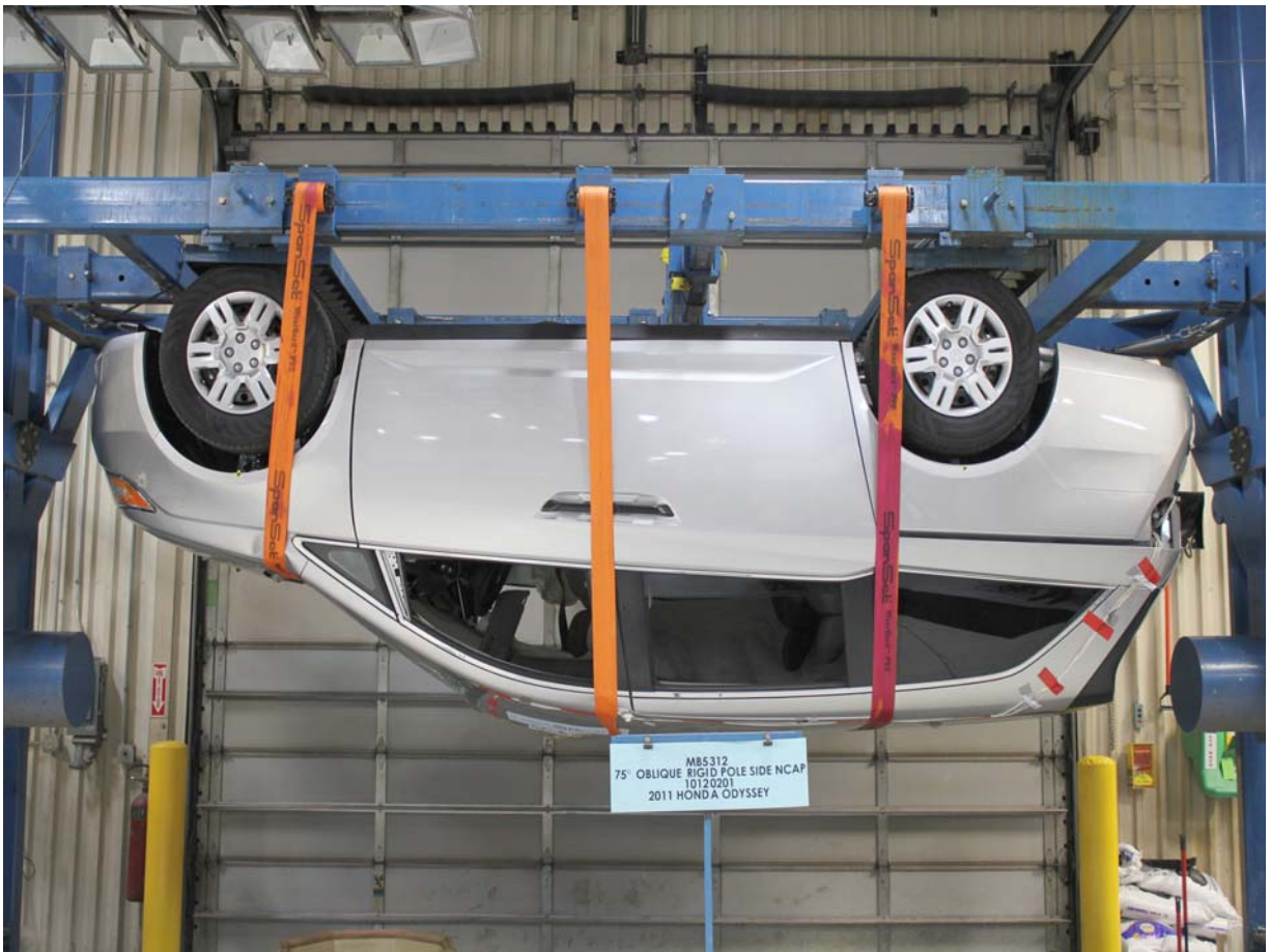
FMVSS No. 301/305 Rollover 180 Degrees
