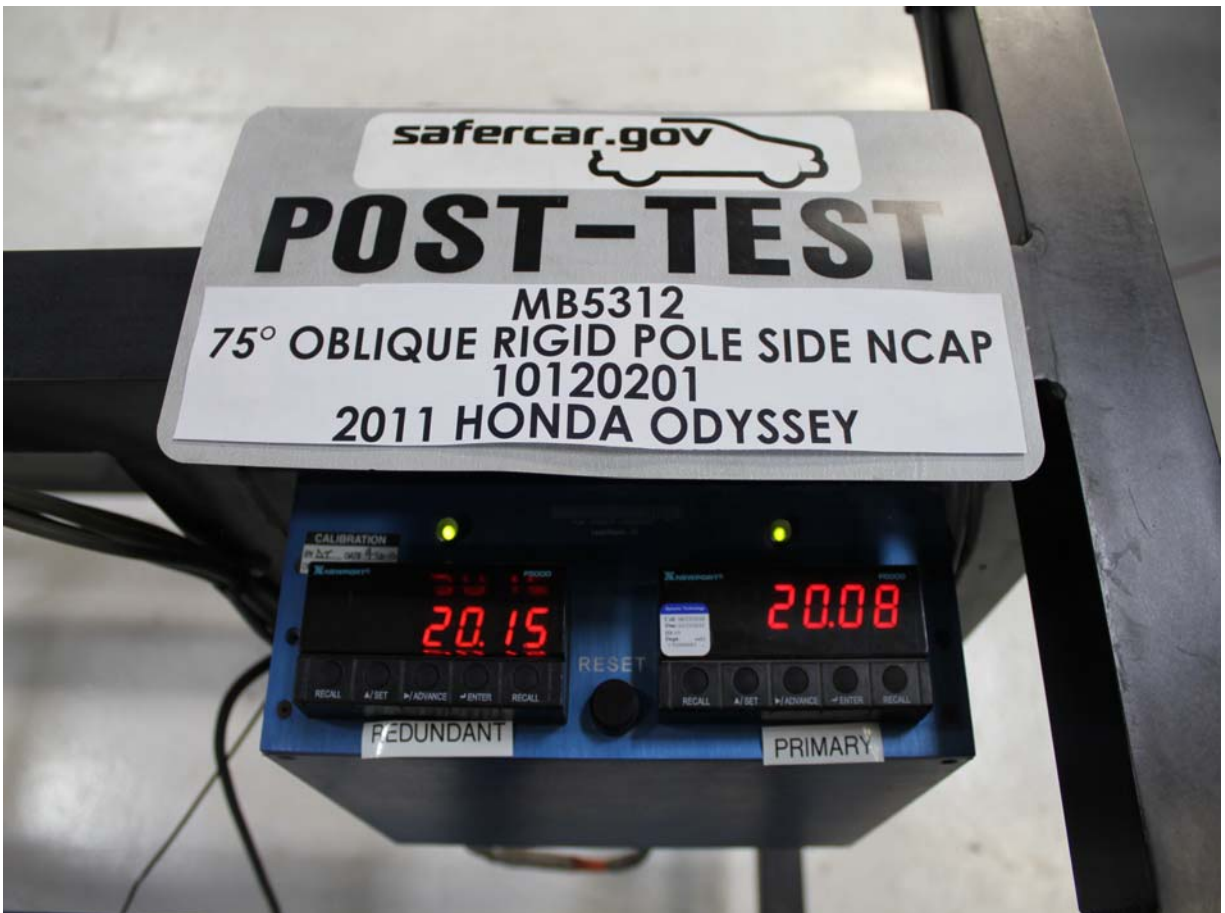
Post-Test Primary and Redundant Speed Trap Read-Out
