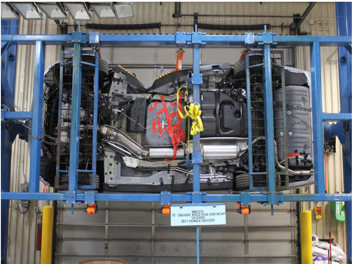
FMVSS No. 301/305 Rollover 270 Degrees
