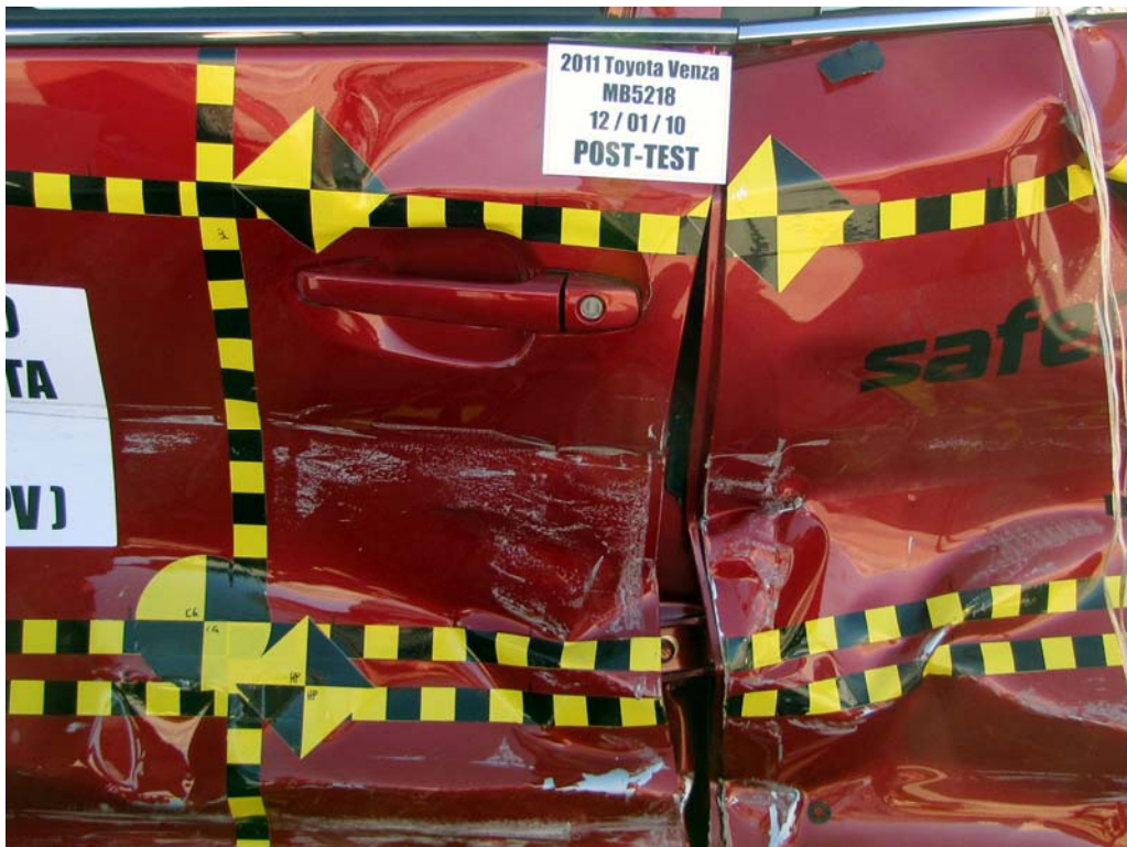
FIGURE 22. Post-Test Left Front Door Latch Close-Up
