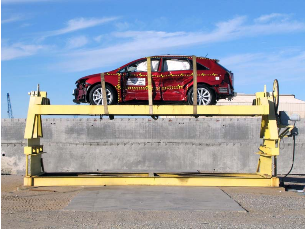
FIGURE 93. FMVSS No. 301/305 Rollover 0 Degrees
