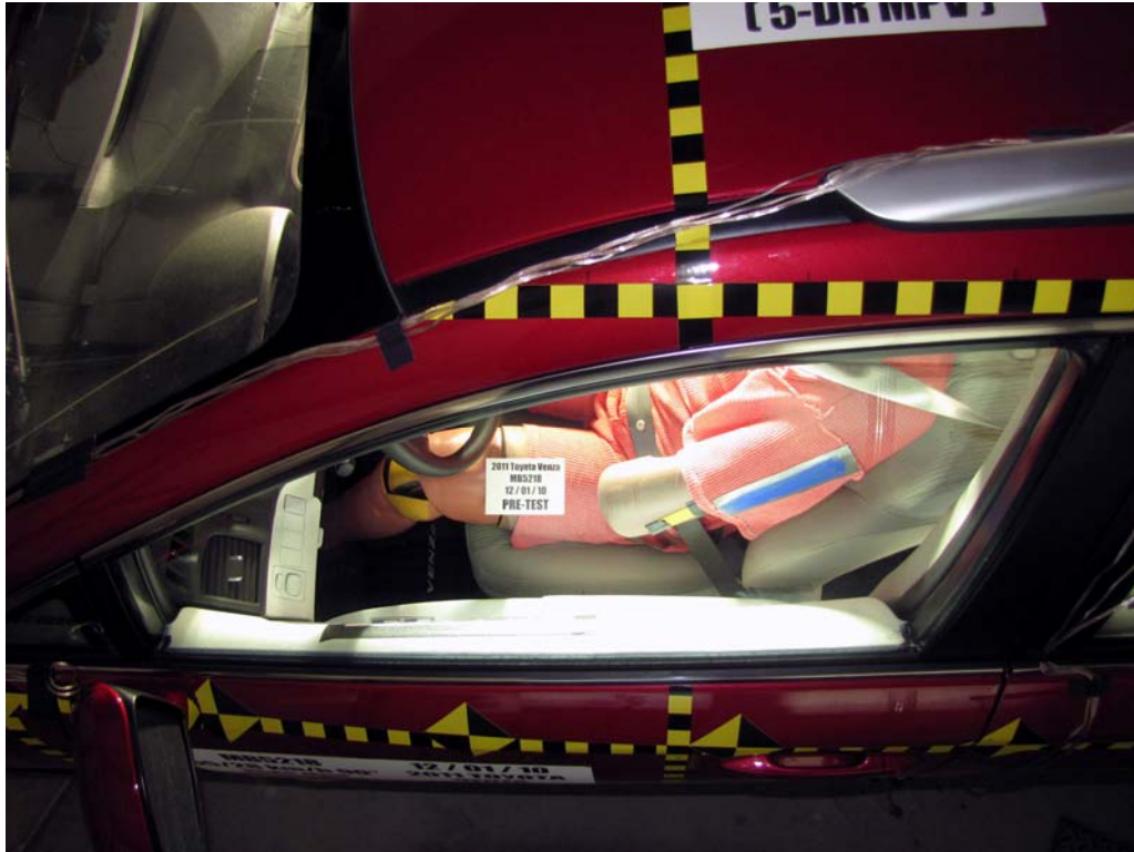
FIGURE 41. Pre-Test Driver Dummy and Door Clearance View
