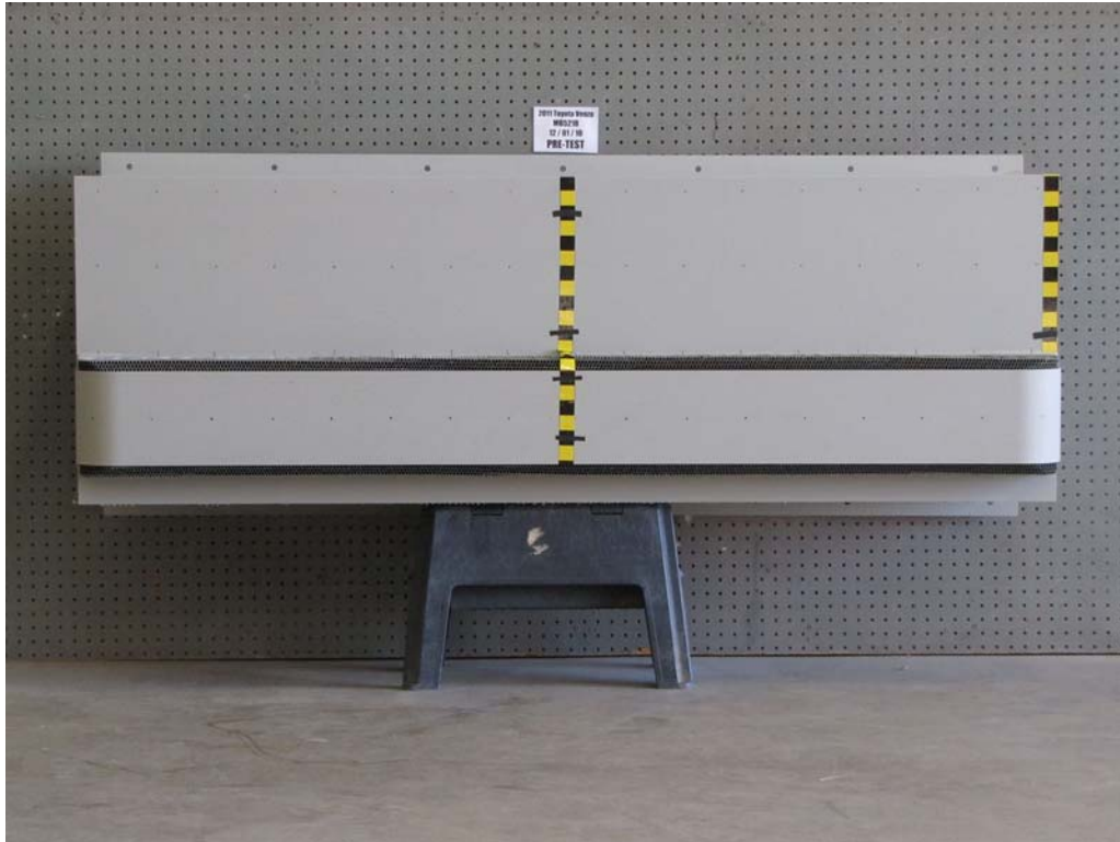
FIGURE 81. Pre-Test Front View of MDB Impactor Face
