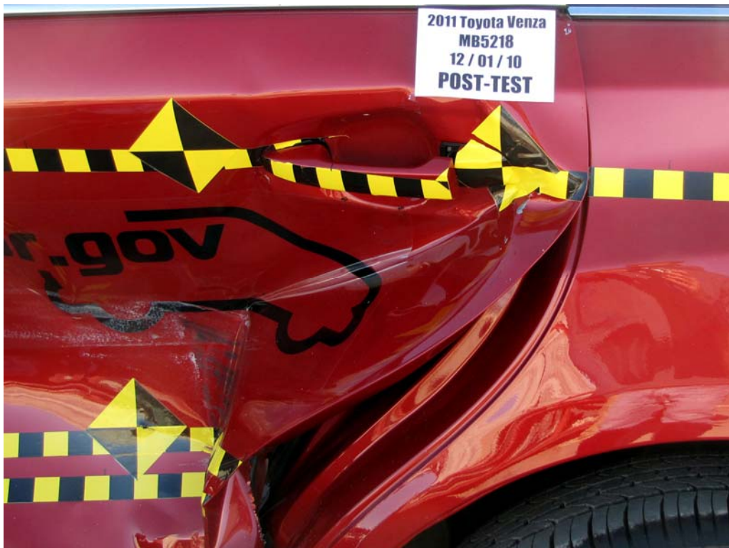
FIGURE 24. Post-Test Left Rear Door Latch Close-Up
