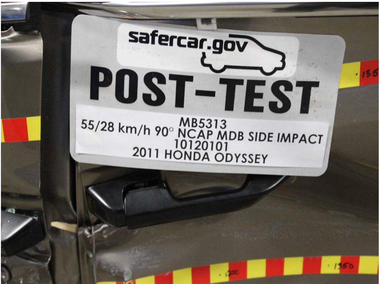
Post-Test Left Rear Door Latch Close-Up
