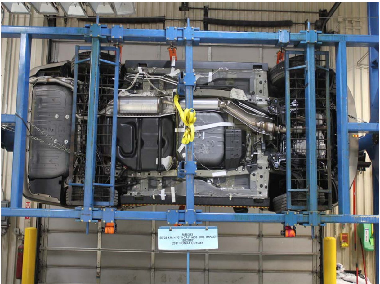
FMVSS No. 301/305 Rollover 90 Degrees
