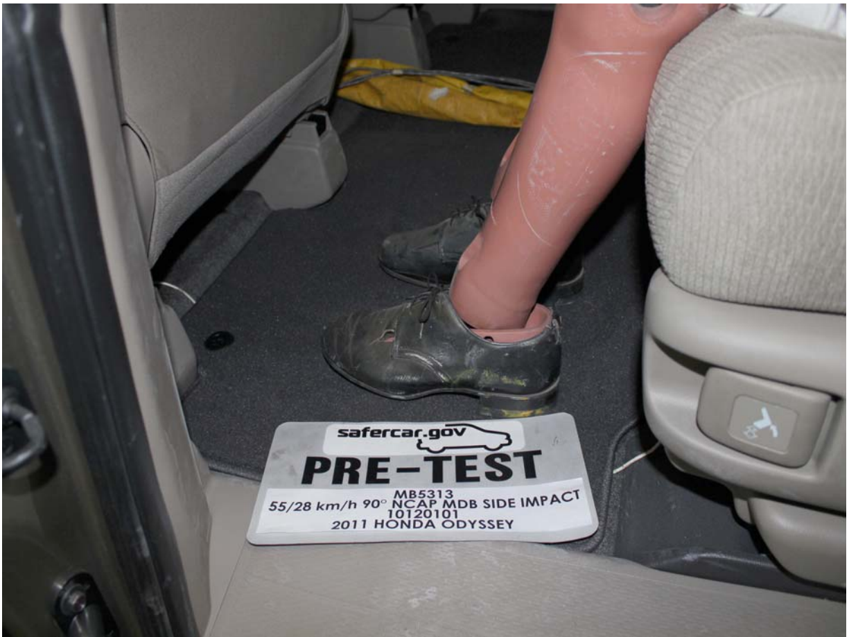
Pre-Test Placement of Rear Passenger Dummy's Feet
