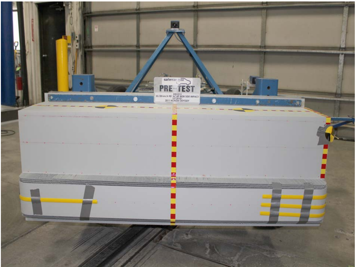
Pre-Test Front View of MDB Impactor Face
