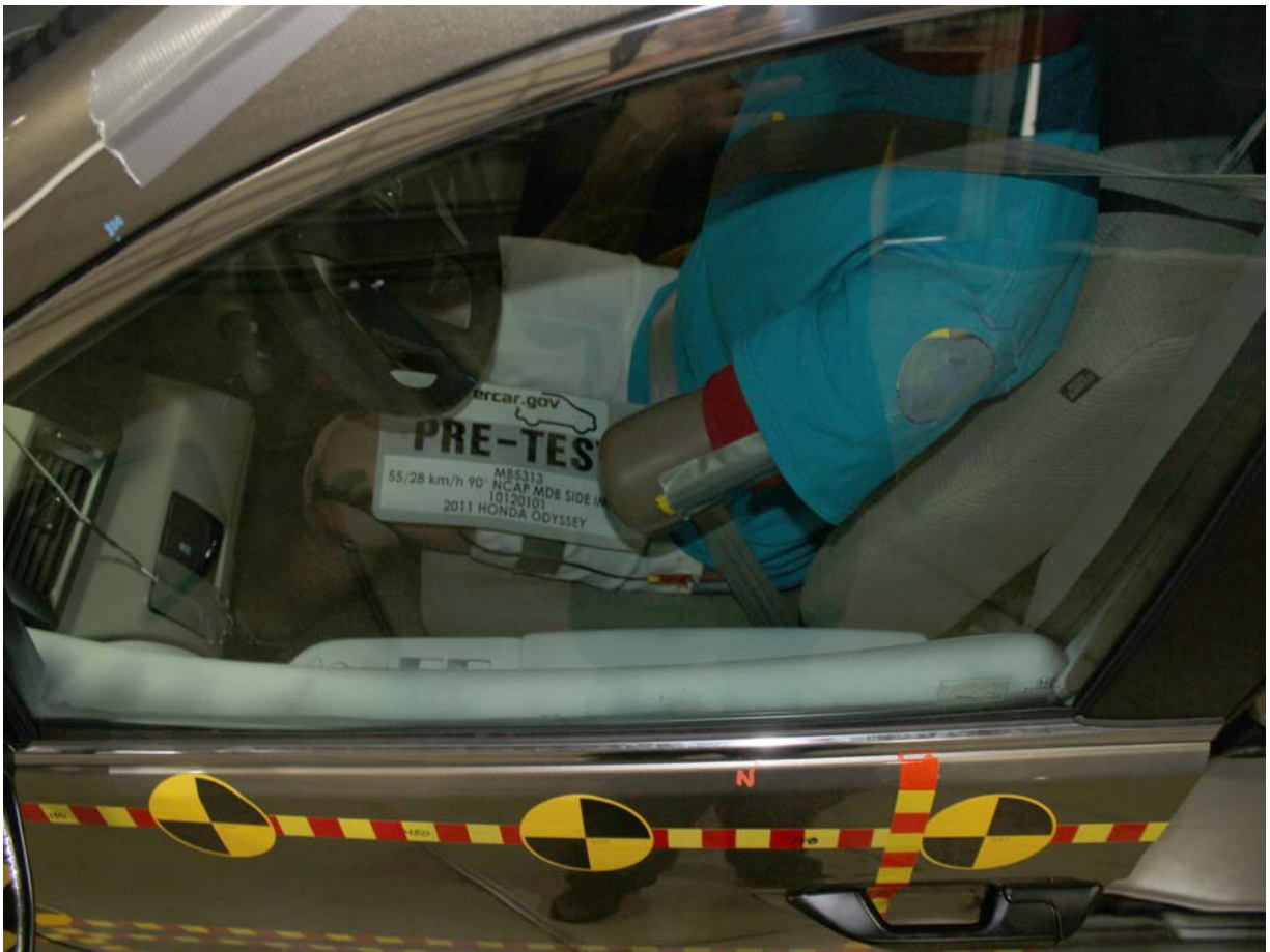
Pre-Test Driver Dummy and Door Clearance View
