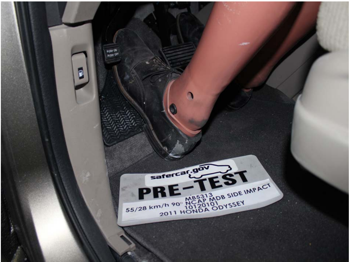
Pre-Test Placement of Driver Dummy's Feet
