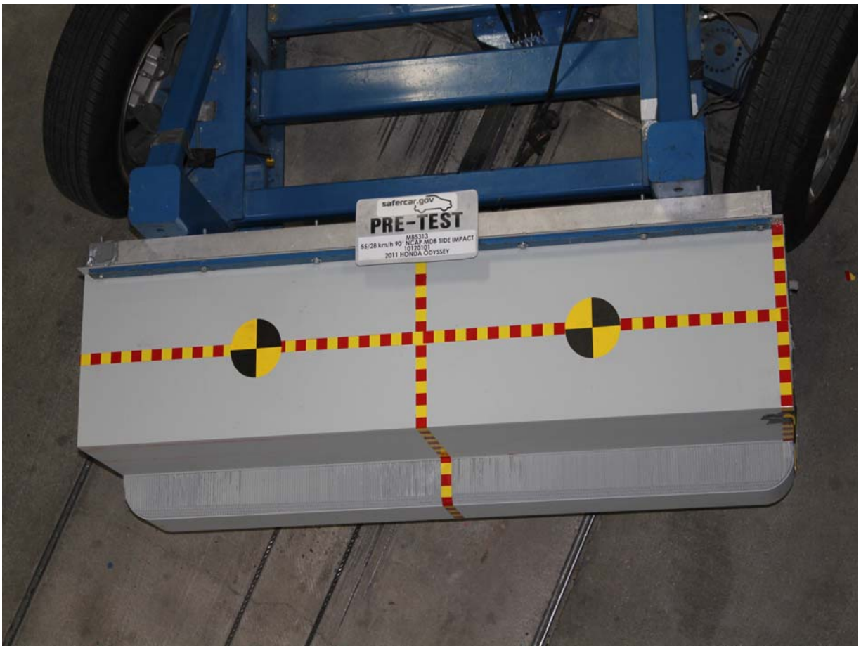
Pre-Test Top View of MDB Impactor Face
