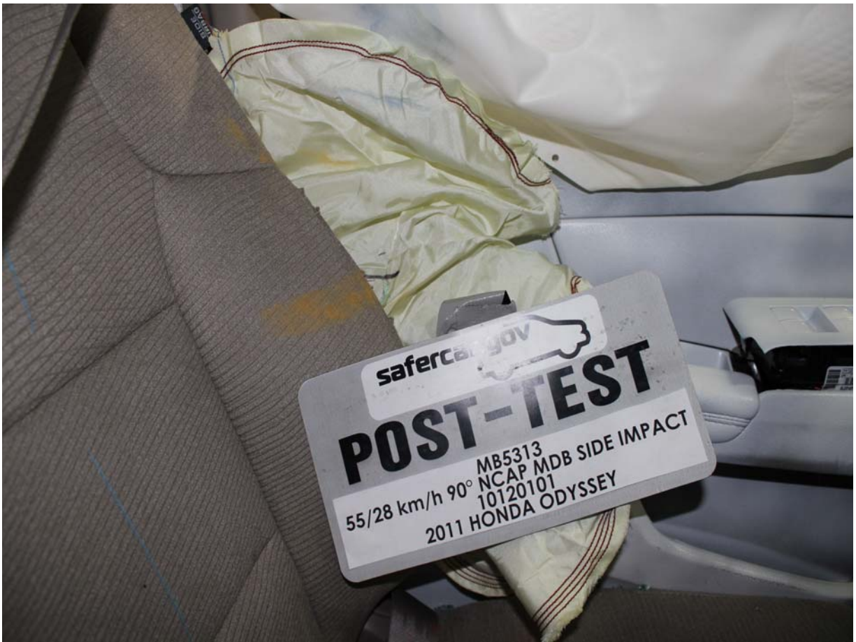
Post-Test Driver Dummy Close-up Torso Contact with Vehicle Interior View
