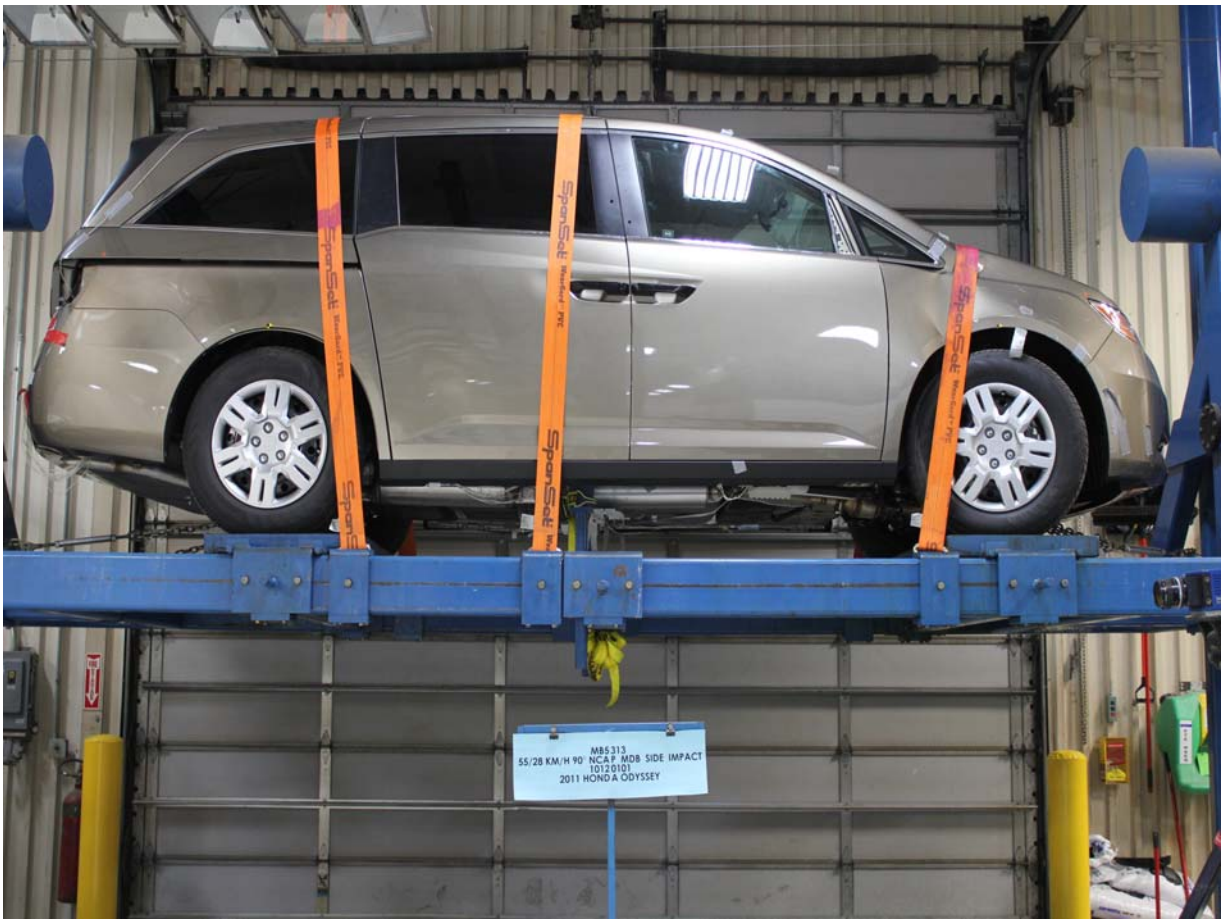
FMVSS No. 301/305 Rollover 360 Degrees
