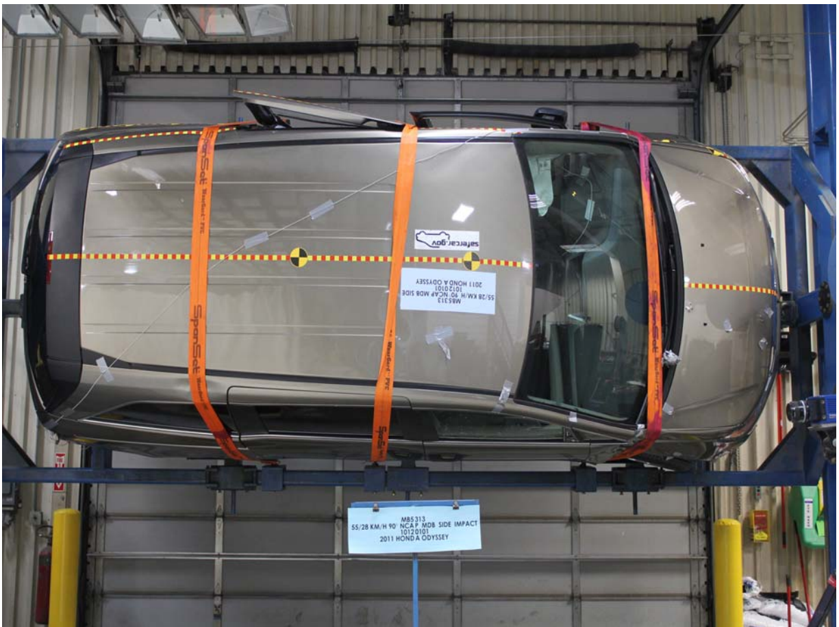
FMVSS No. 301/305 Rollover 270 Degrees
