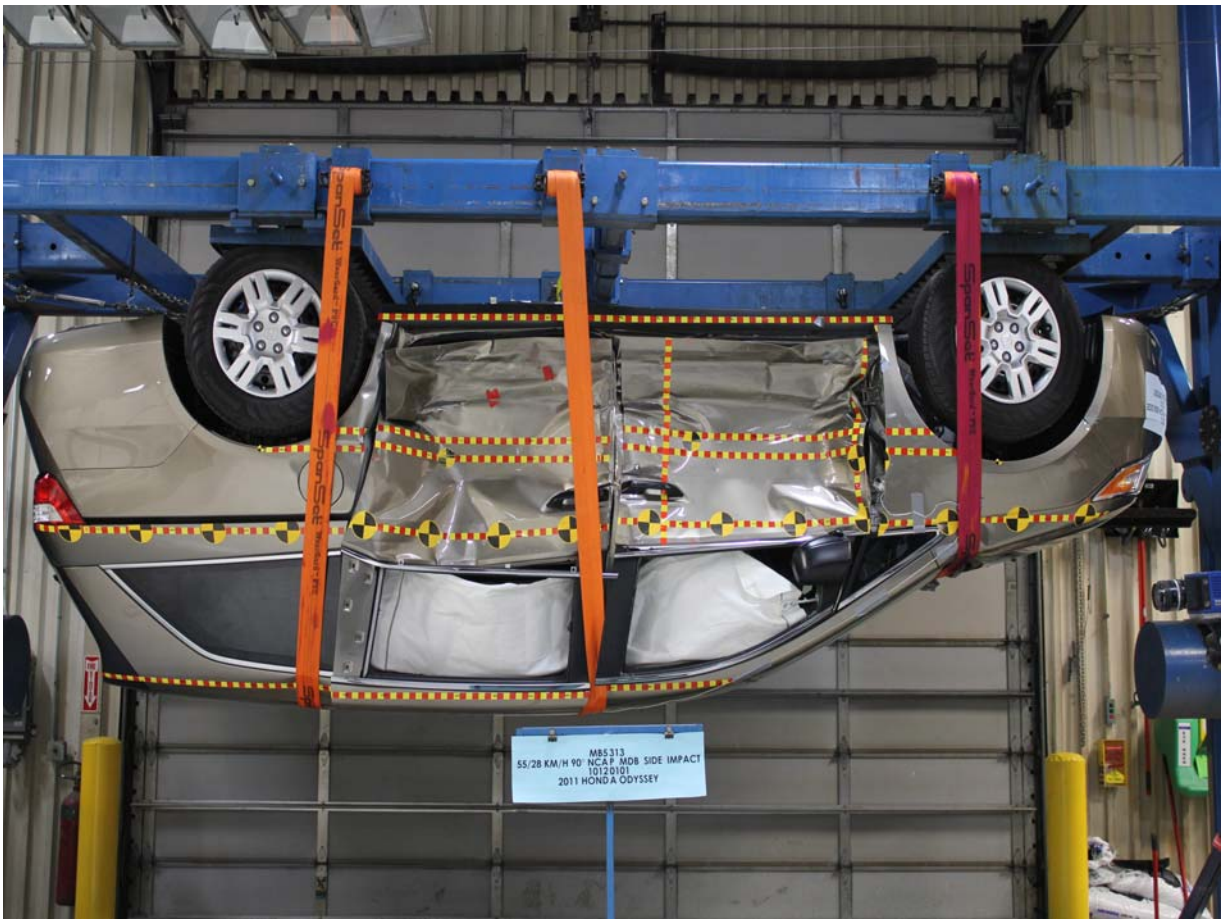
FMVSS No. 301/305 Rollover 180 Degrees
