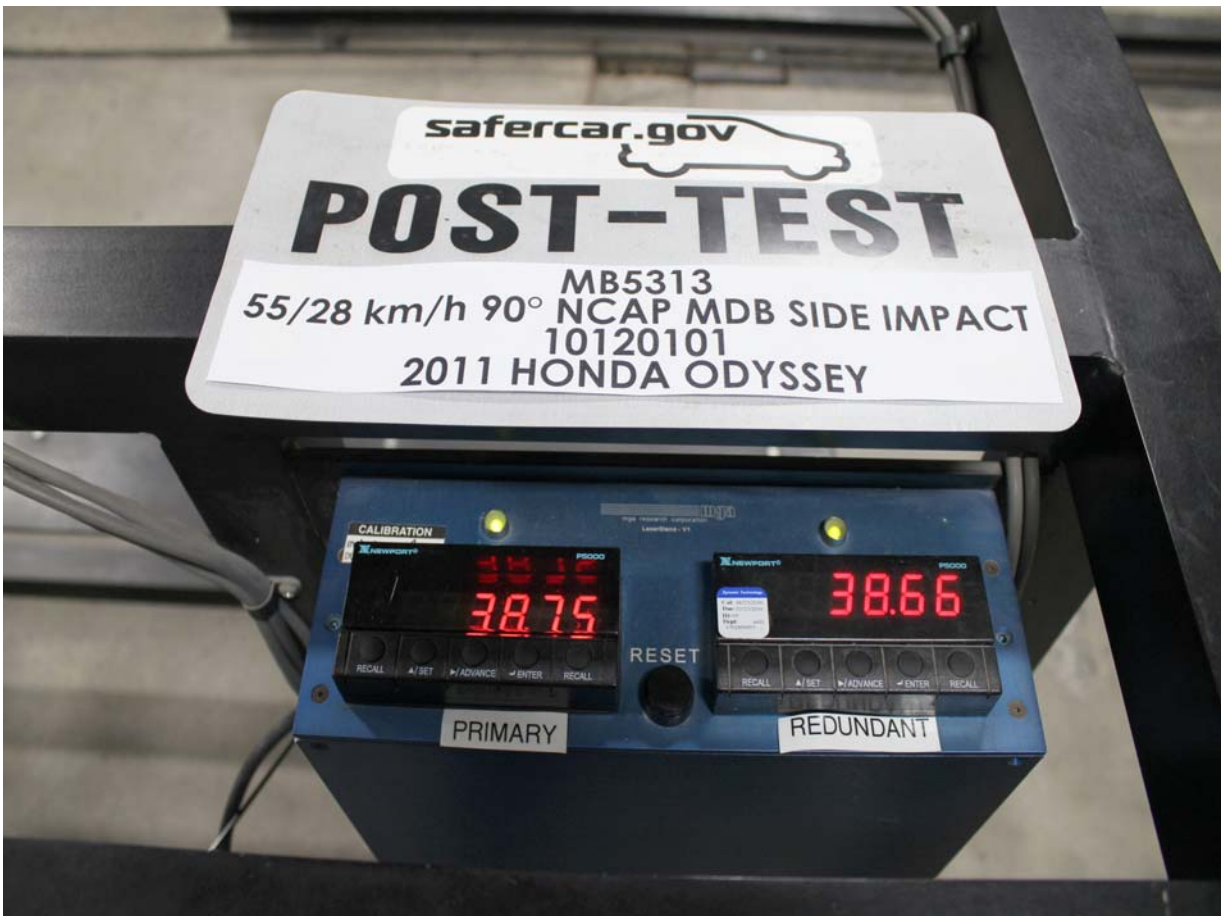
Post-Test Primary and Redundant Speed Trap Read-Out
