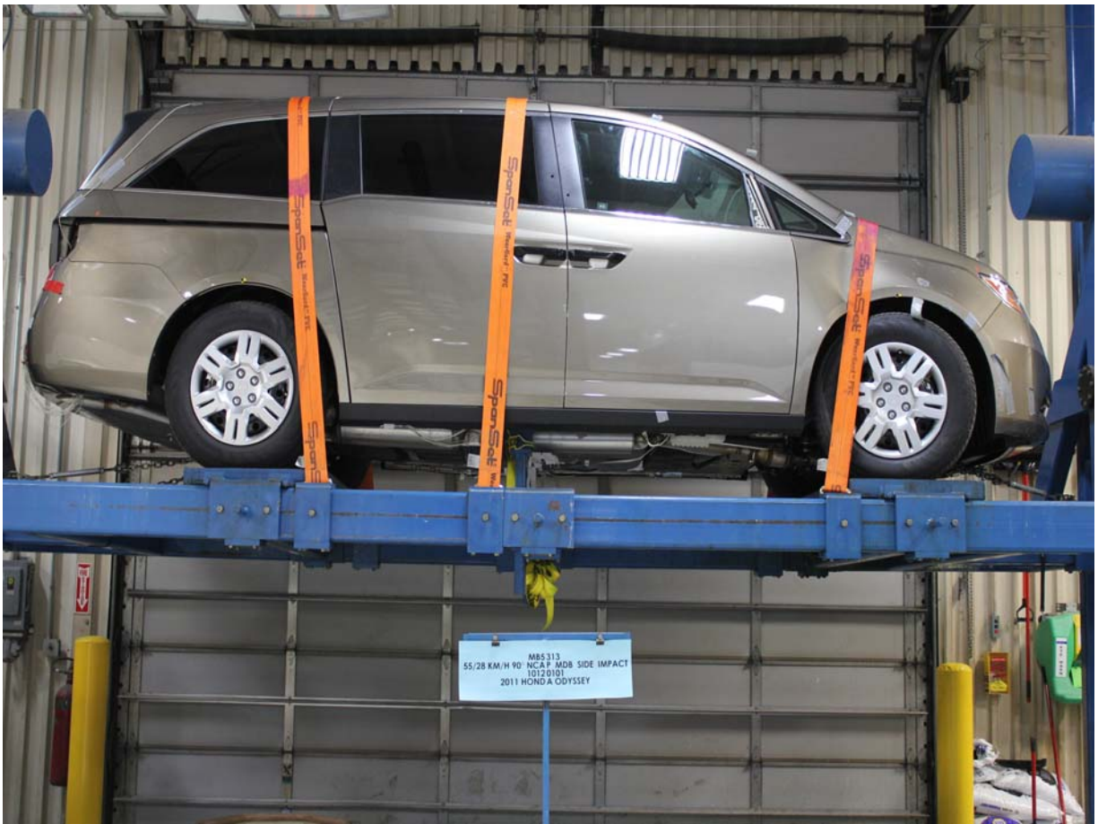
FMVSS No. 301/305 Rollover 0 Degrees
