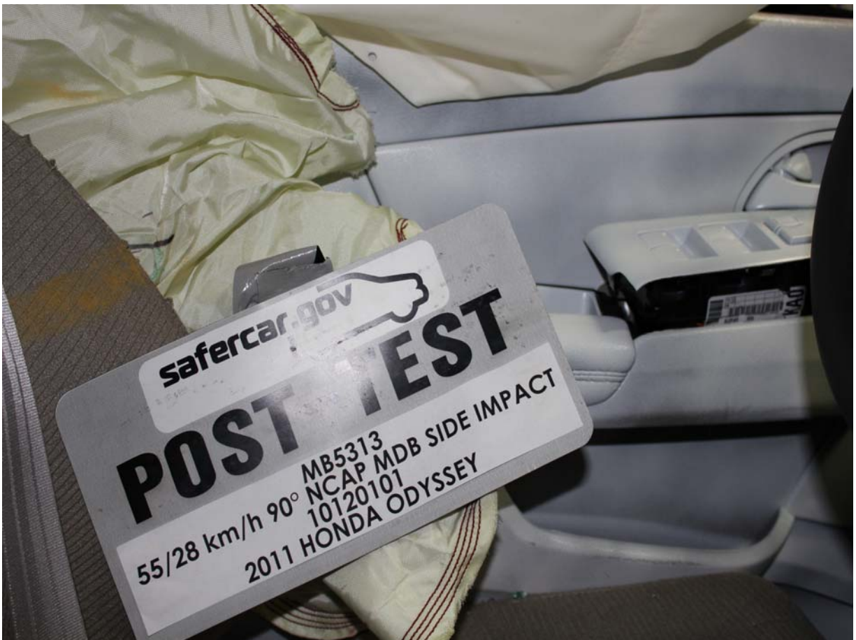
Post-Test Driver Dummy Close-up Torso Contact with Side Airbag View
