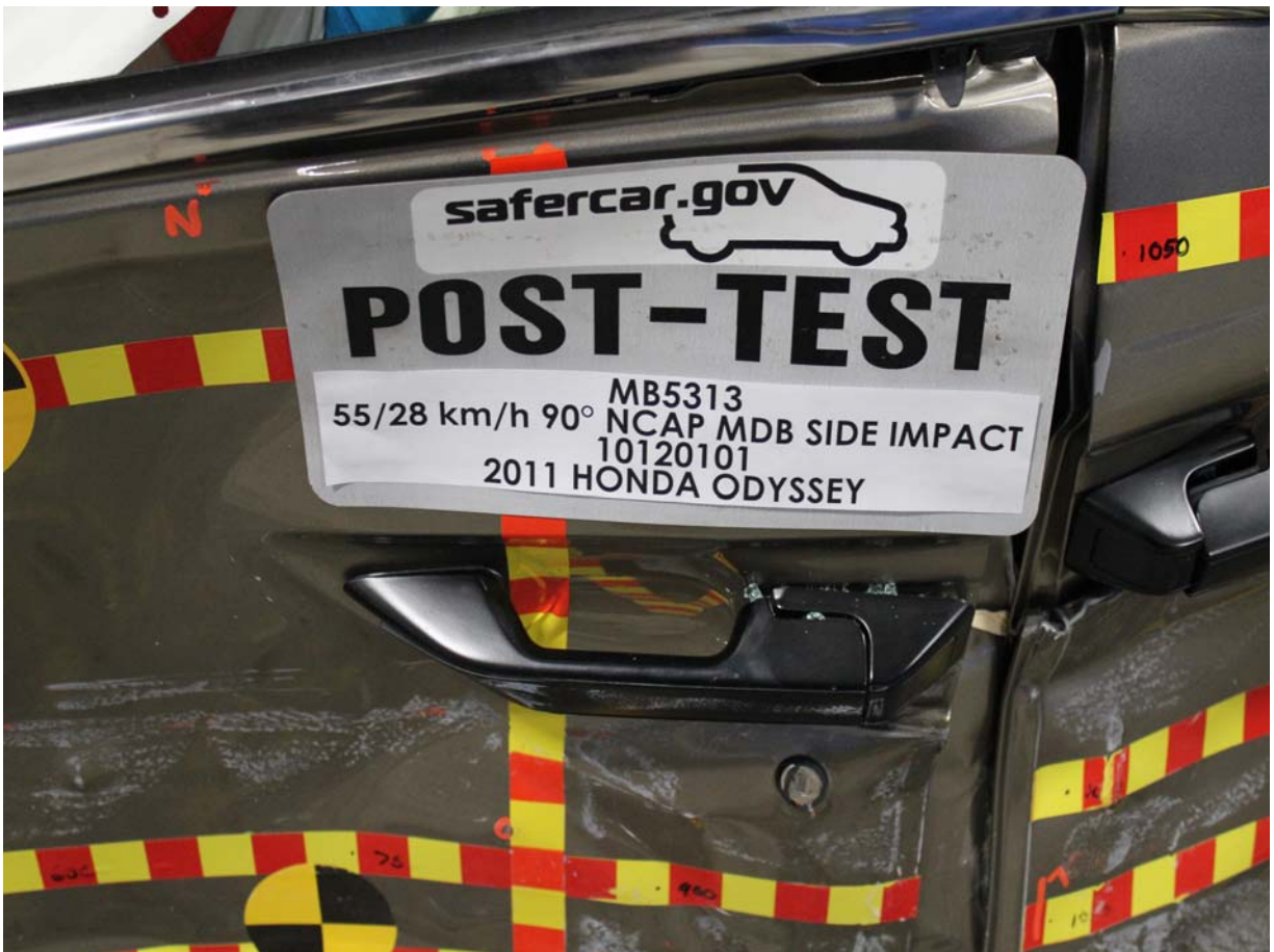
Post-Test Left Front Door Latch Close-Up
