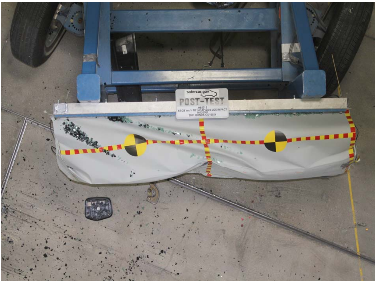
Post-Test Top View of MDB Impactor Face
