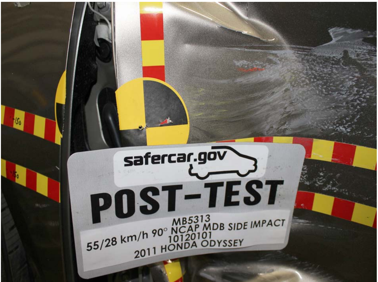
Post-Test Close-Up View of Impact Point Target
