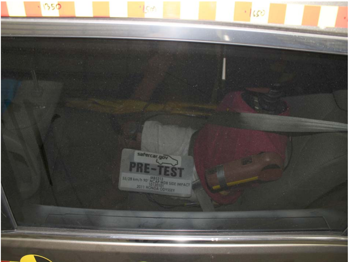
Pre-Test Rear Passenger Dummy and Door Clearance View
