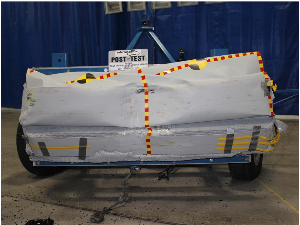
Post-Test Front View of MDB Impactor Face
