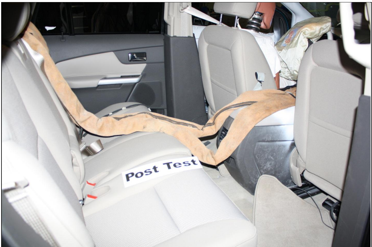
Figure A-28: Post-Test Dummy Cable Routing
