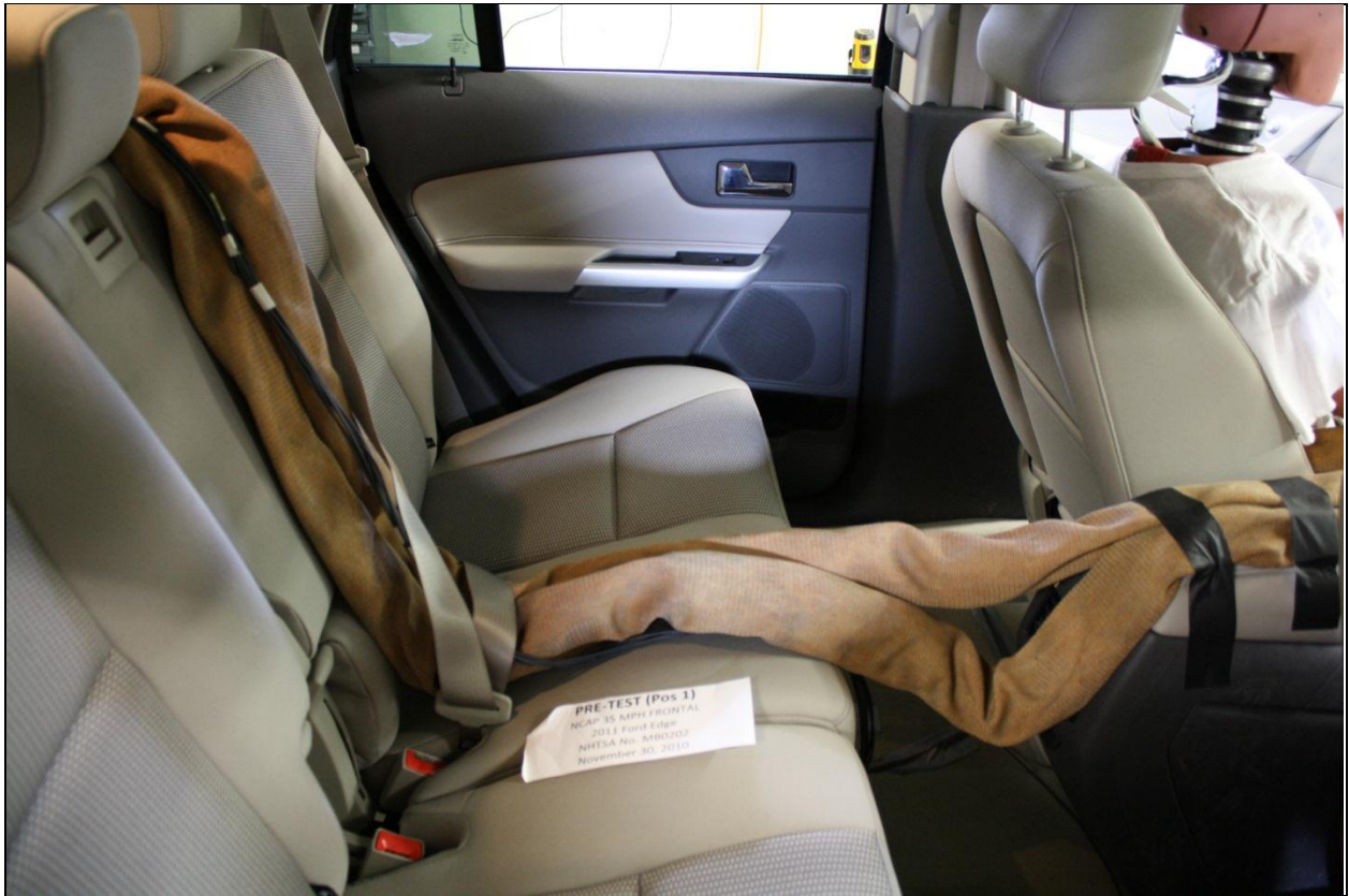
Figure A-27: Pre-Test Dummy Cable Routing
