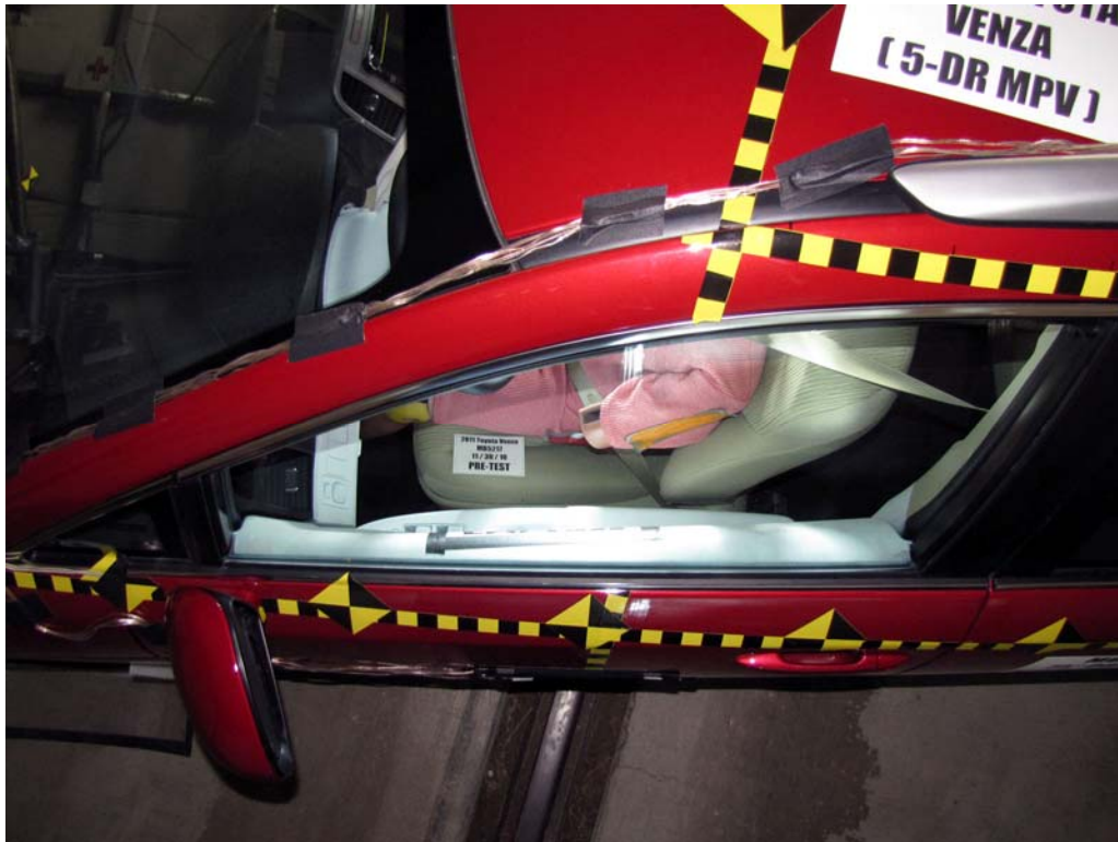
FIGURE 39. Pre-Test Driver Dummy and Door Clearance
