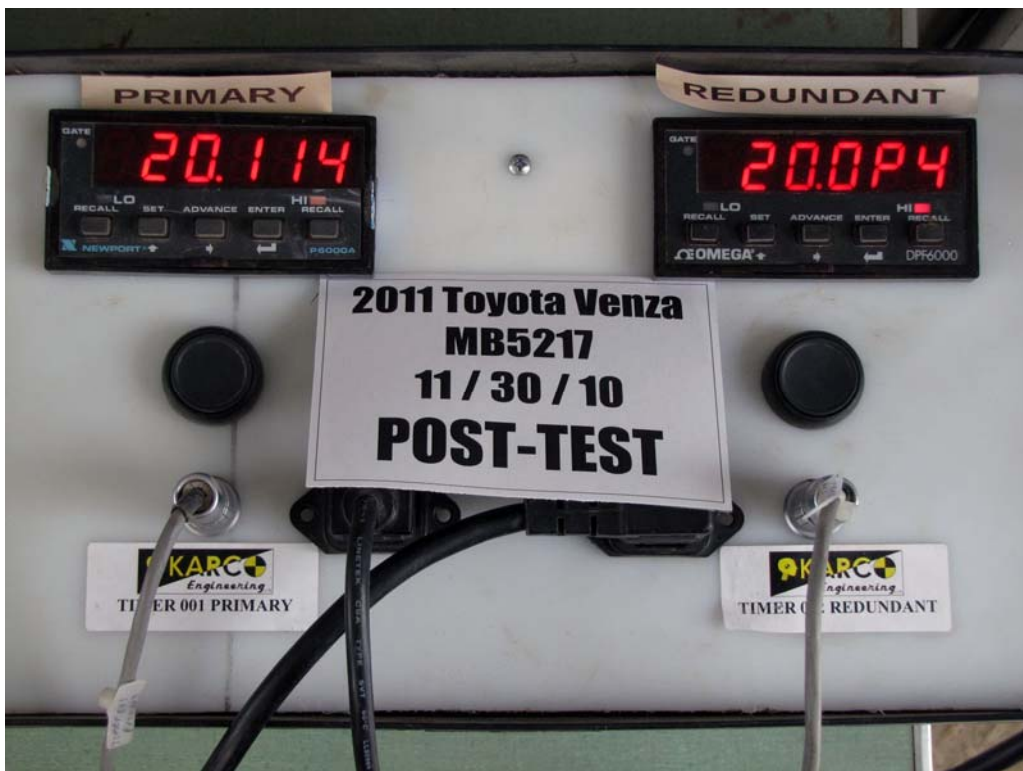
FIGURE 60. Post-Test Primary and Redundant Speed Trap Read-Out
