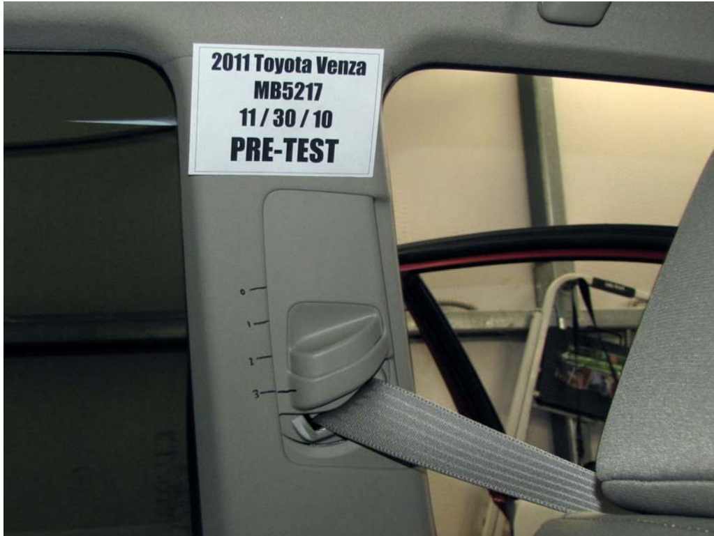
FIGURE 33. Pre-Test View of Belt Anchorage for Dummy
