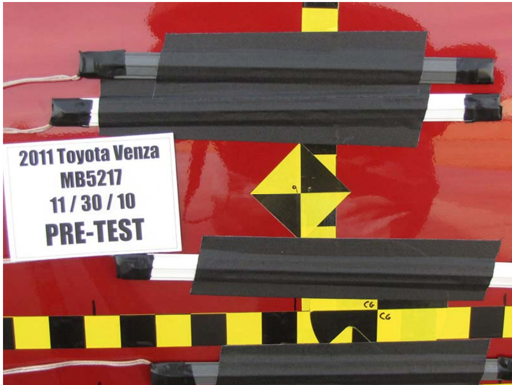
FIGURE 19. Pre-Test Close-Up View of Impact Point Target
