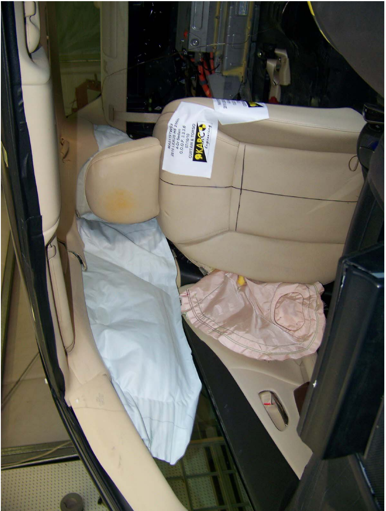
Figure A-10: Post-Test Airbags, Left Front ¾ View
