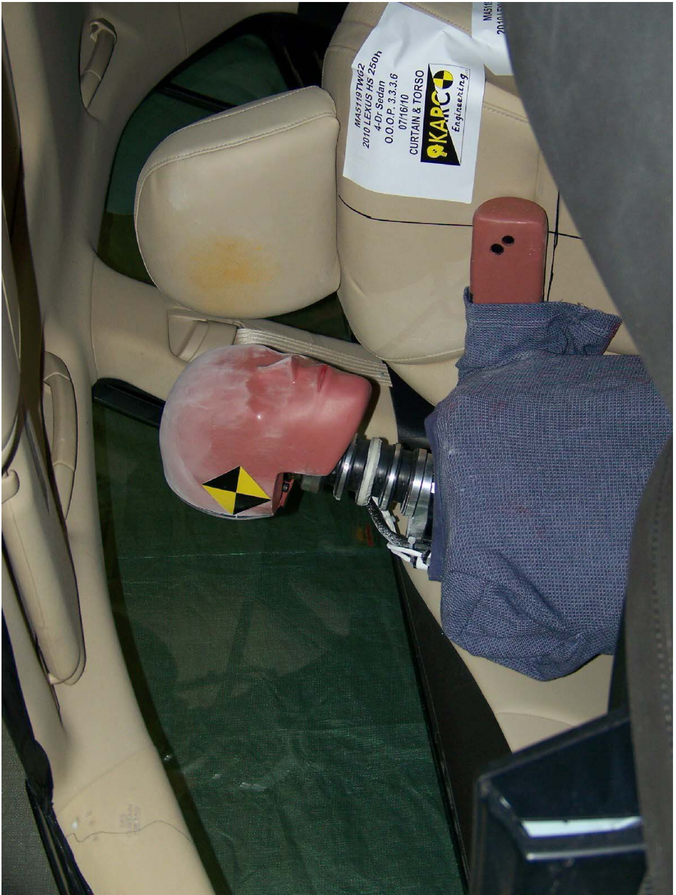
Figure A-6: Pre-Test Dummy Position, \frac{3}{4} View
