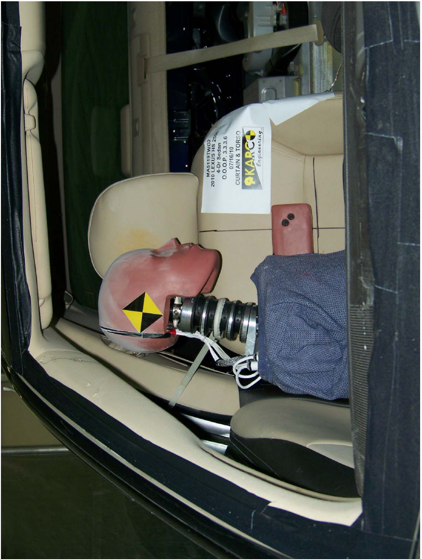
Figure A-7: Pre-Test Dummy Position, Front View
