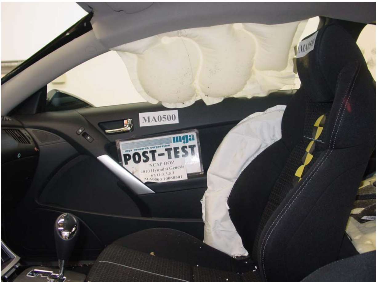
Post-Test Curtain and Torso/Pelvis Airbag Left View
