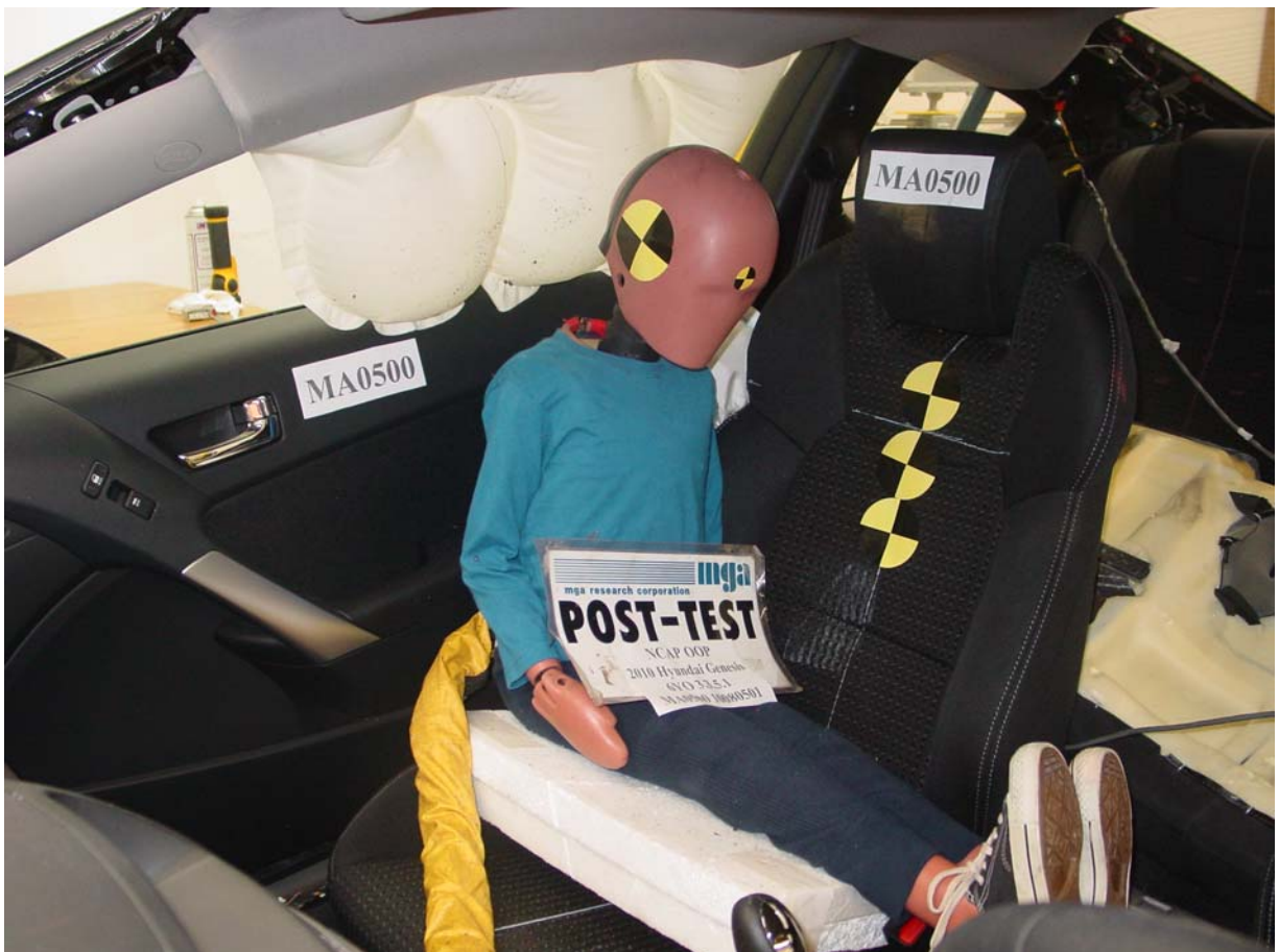
Post-Test 6-Year-Old Child Dummy Left ¾ Front View
