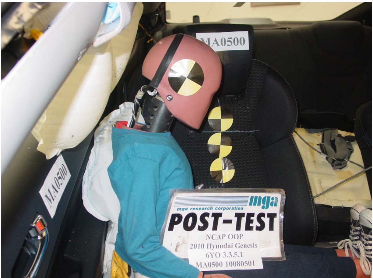
Post-Test 6-Year-Old Child Dummy Front Closeup View
