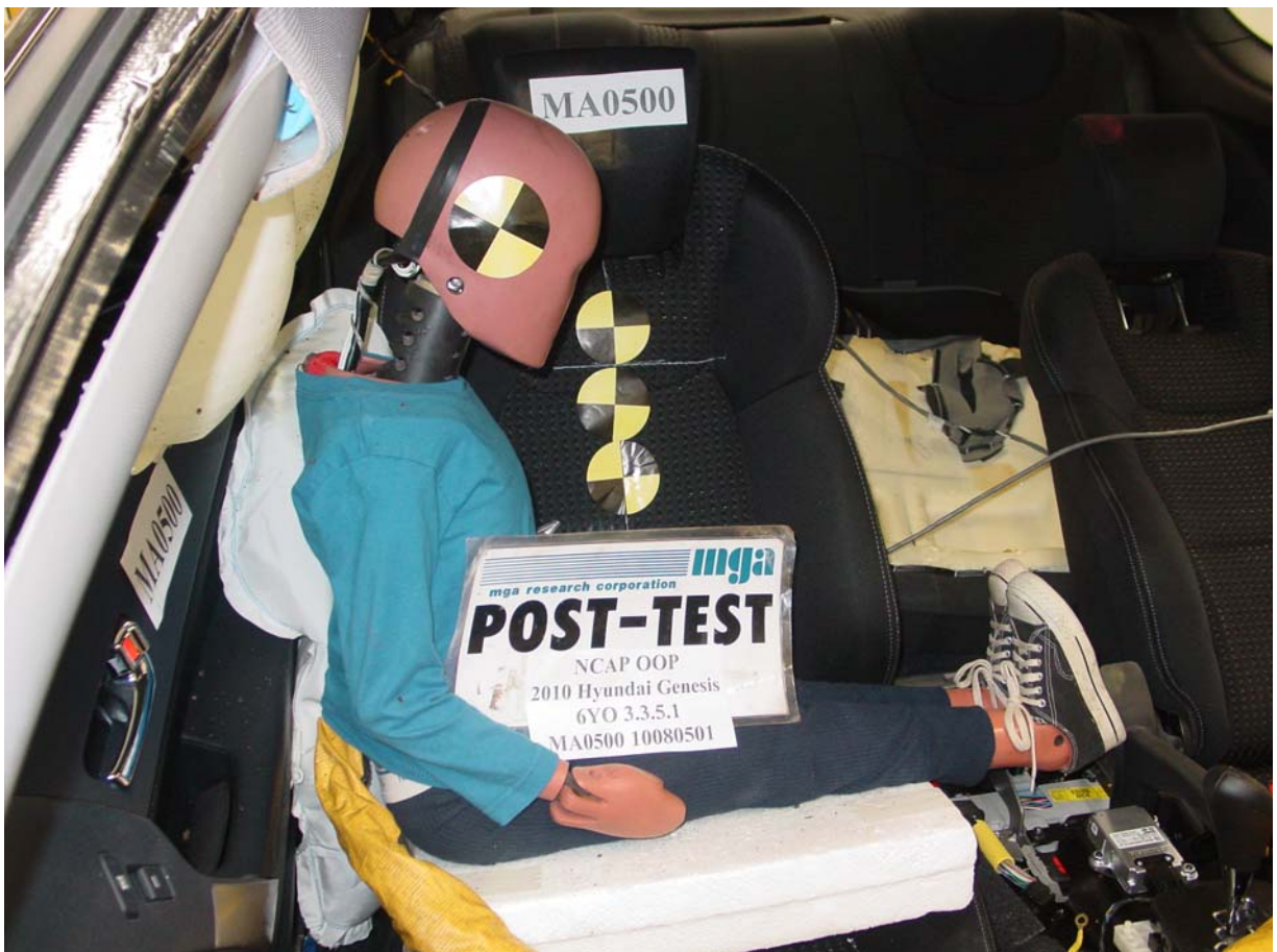
Post-Test 6-Year-Old Child Dummy Front View
