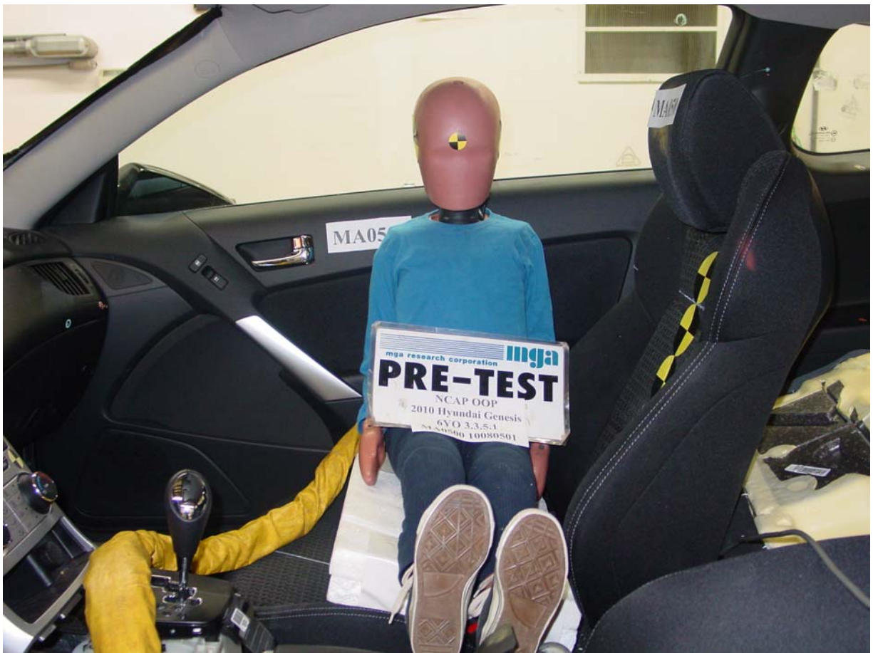
Pre-Test 6-Year-Old Child Dummy Left Side View
