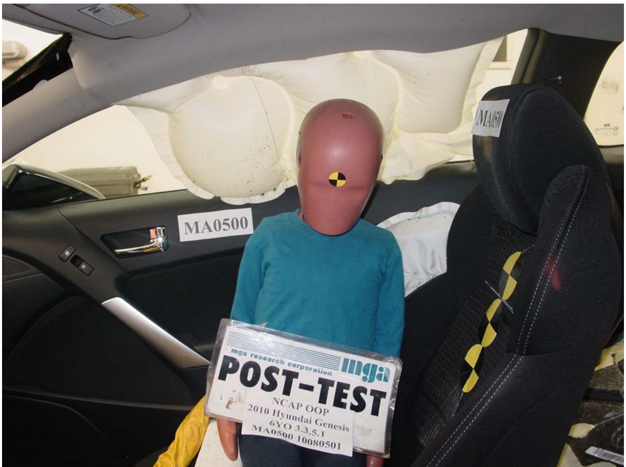
Post-Test 6-Year-Old Child Dummy Left Side Closeup View
