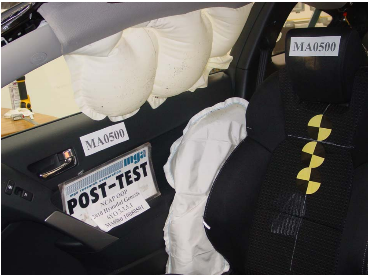
Post-Test Curtain and Torso/Pelvis Airbag Left ¾ Front View
