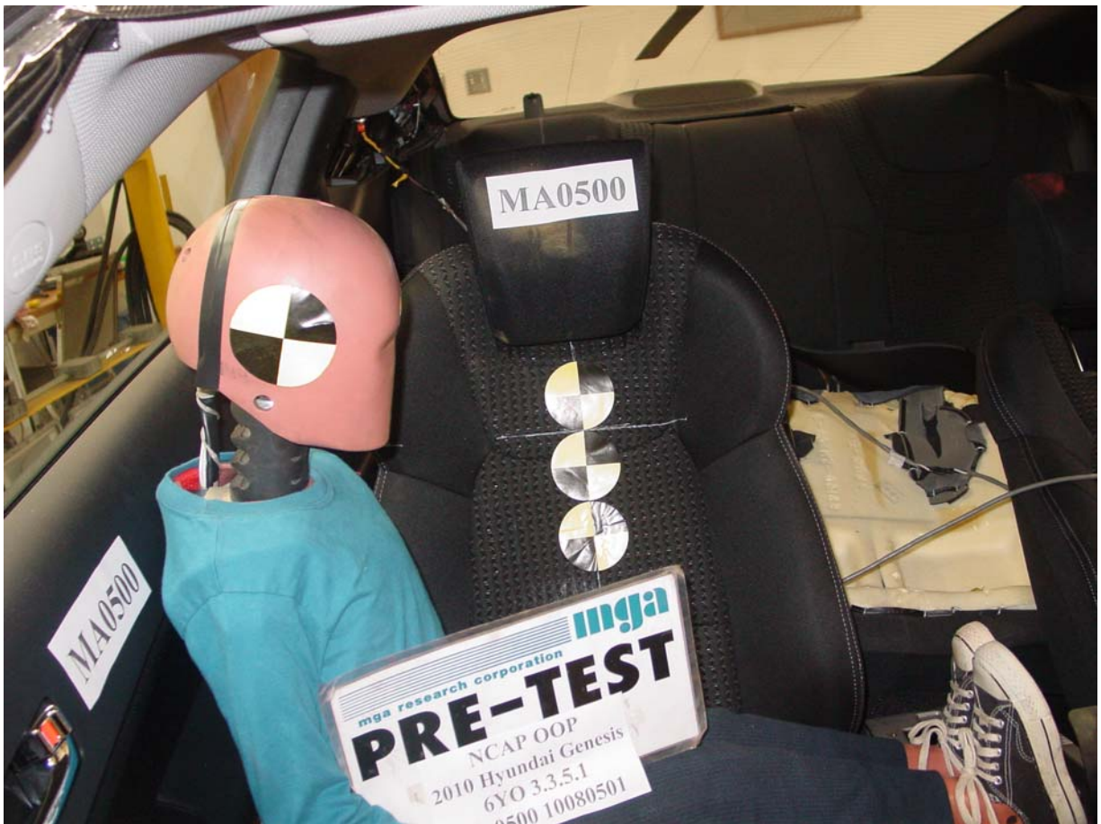
Pre-Test 6-Year-Old Child Dummy Front Closeup View
