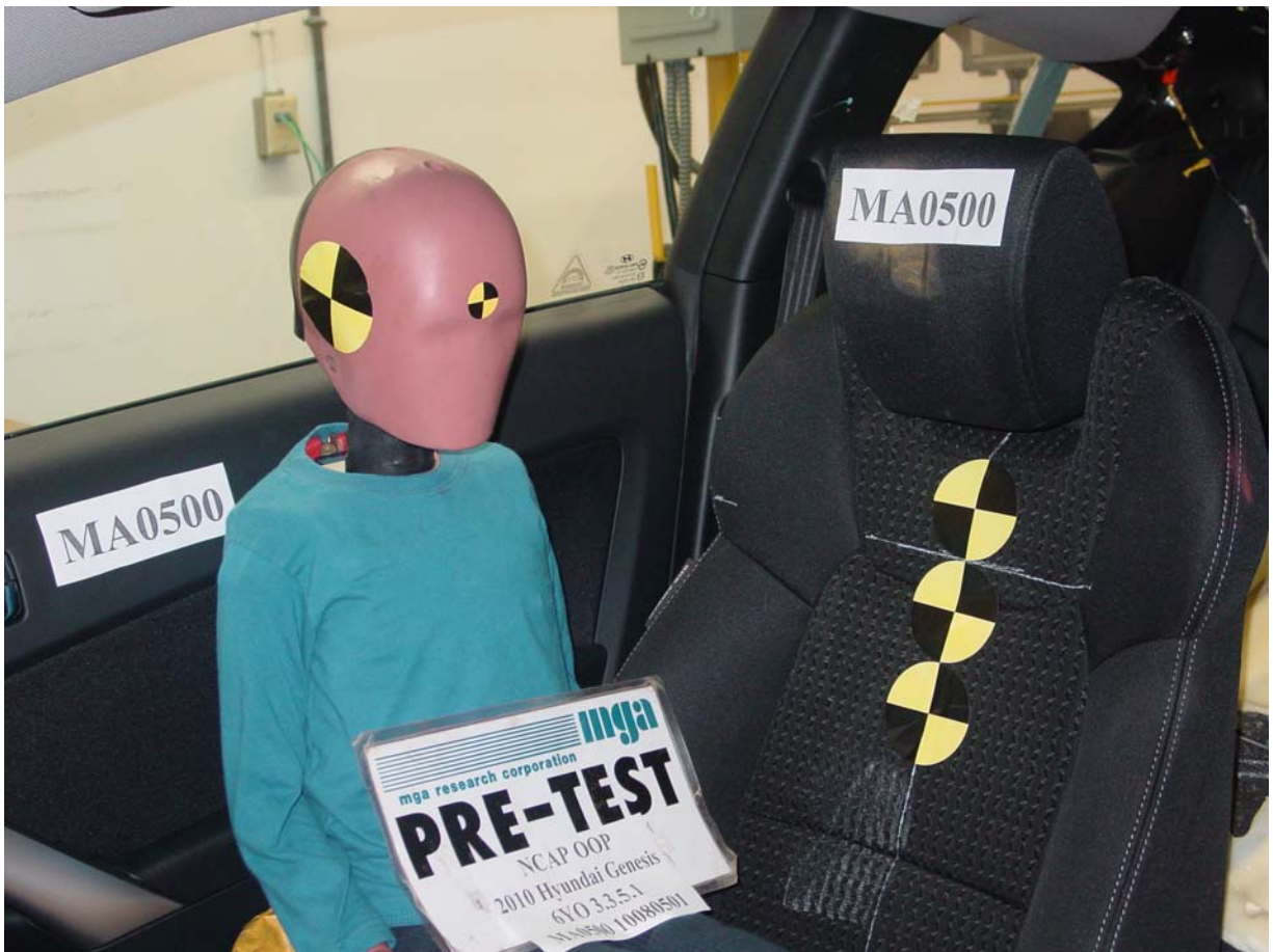
Pre-Test 6-Year-Old Child Dummy Left 3/4 Front Closeup View
