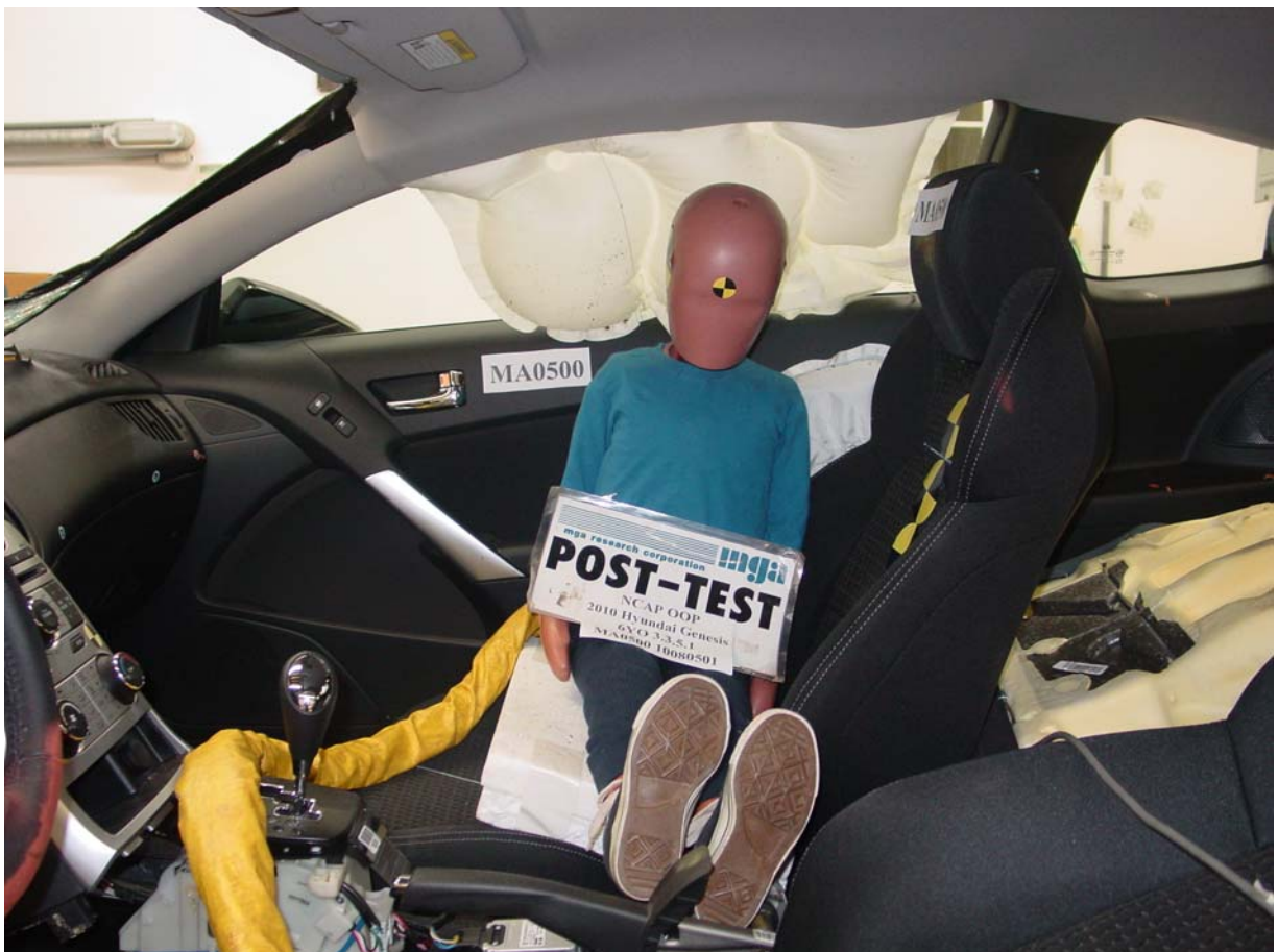
Post-Test 6-Year-Old Child Dummy Left Side View
