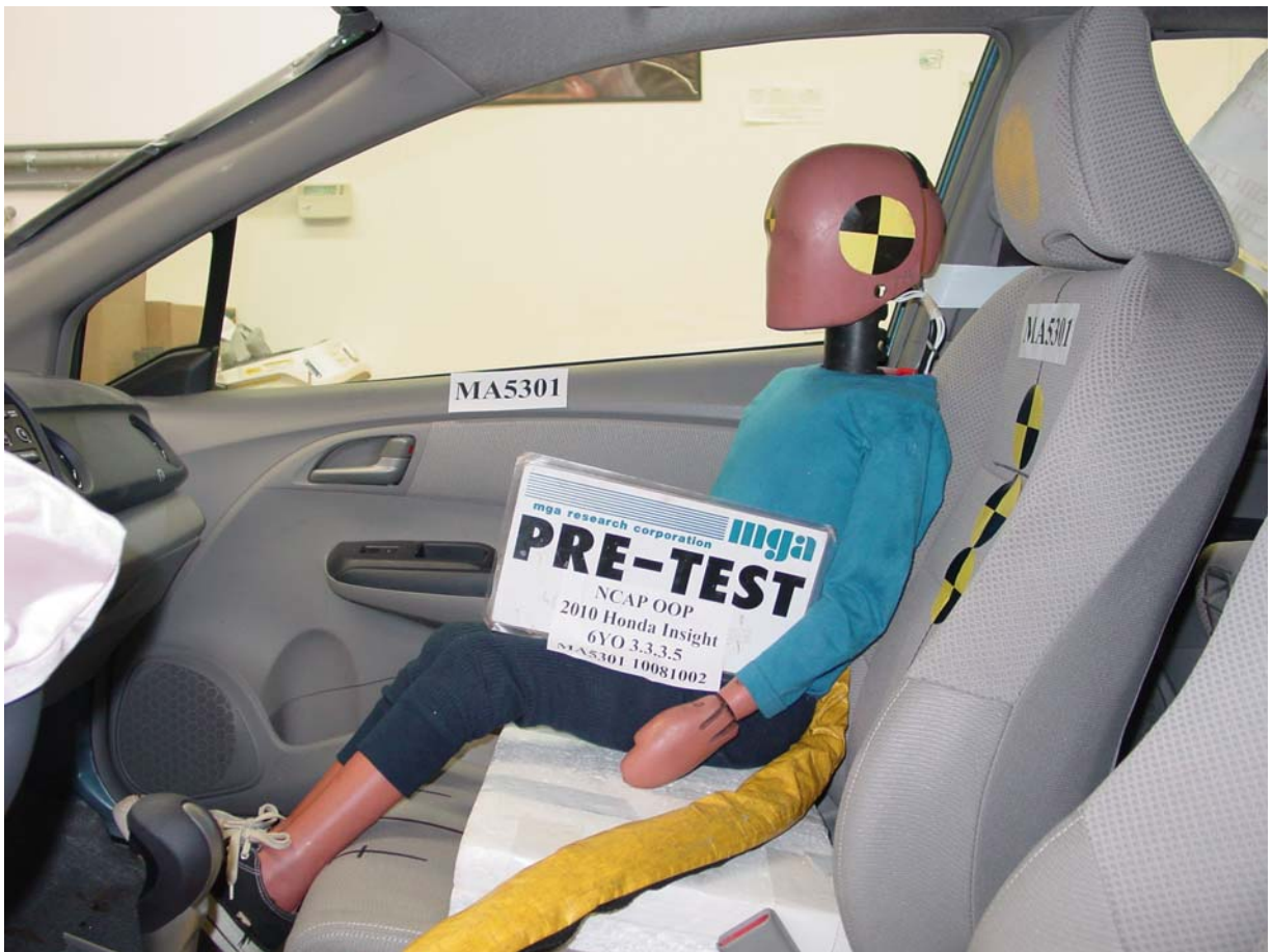
Pre-Test 6-Year-Old Child Dummy Left Side View
