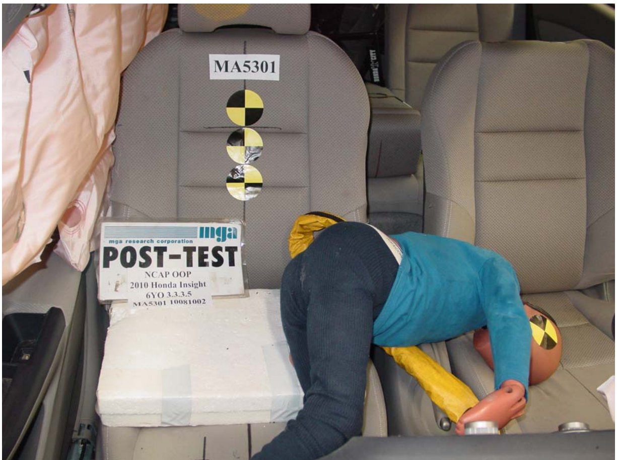
Post-Test 6-Year-Old Child Dummy Front View
