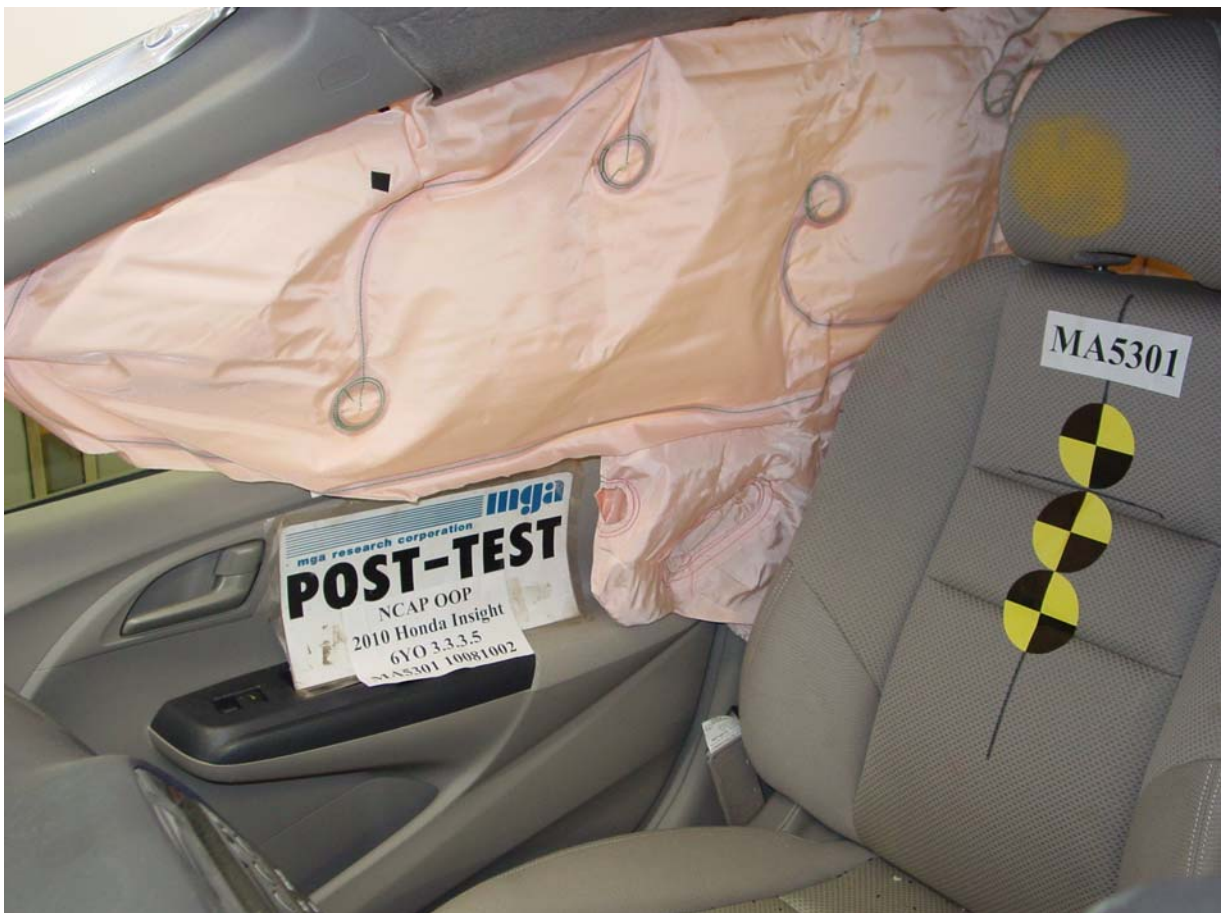
Post-Test Curtain and Torso Airbag Left \frac{3}{4} Front View
