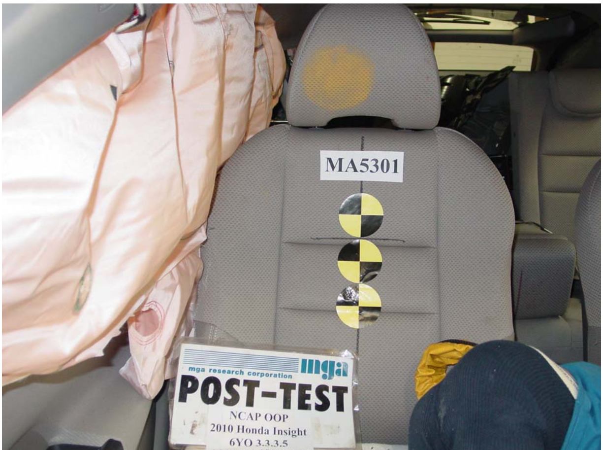
Post-Test 6-Year-Old Child Dummy Front Closeup View
