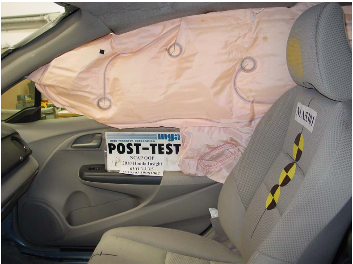
Post-Test Curtain and Torso Airbag Left View
