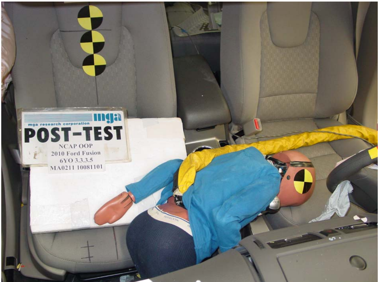
Post-Test 6-Year-Old Child Dummy Front Closeup View
