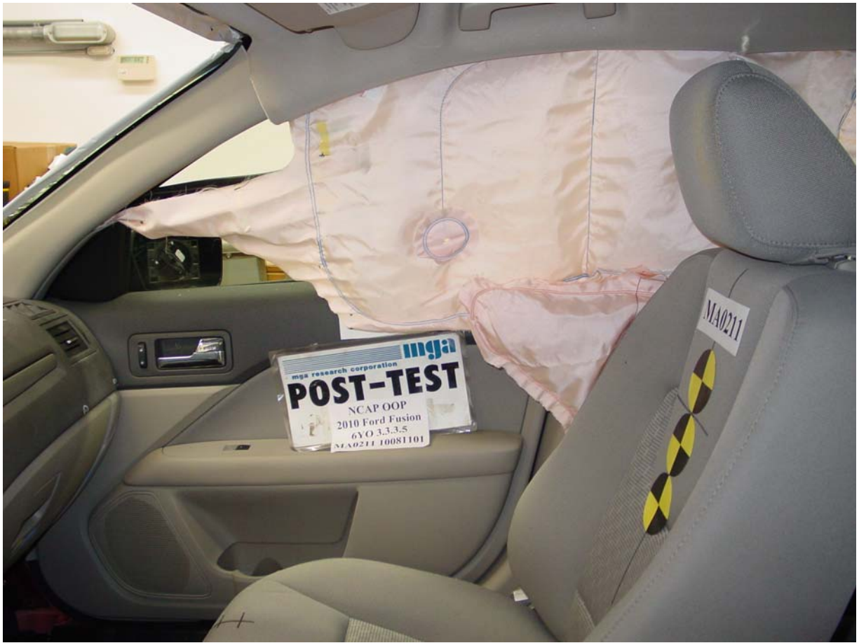
Post-Test Curtain and Torso Airbag Left View
