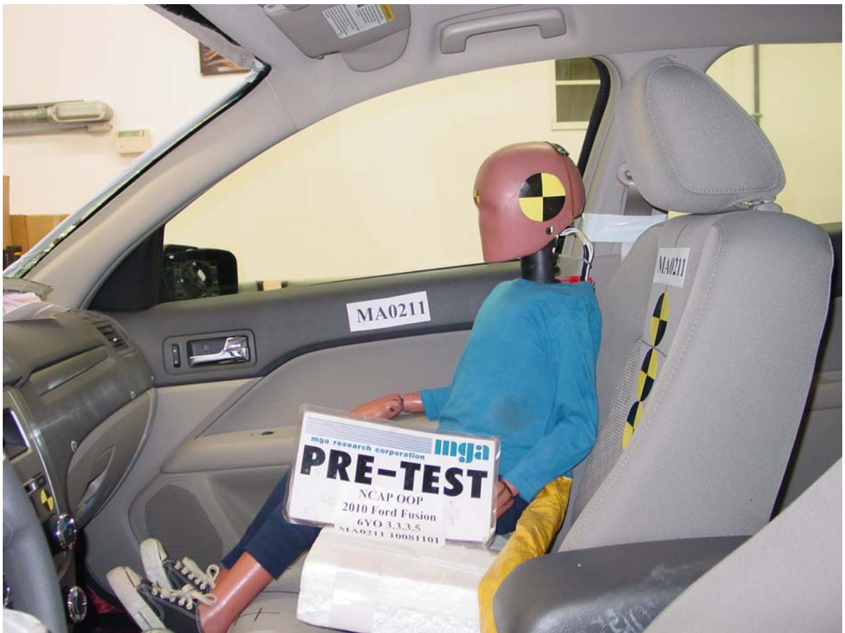
Pre-Test 6-Year-Old Child Dummy Left Side View
