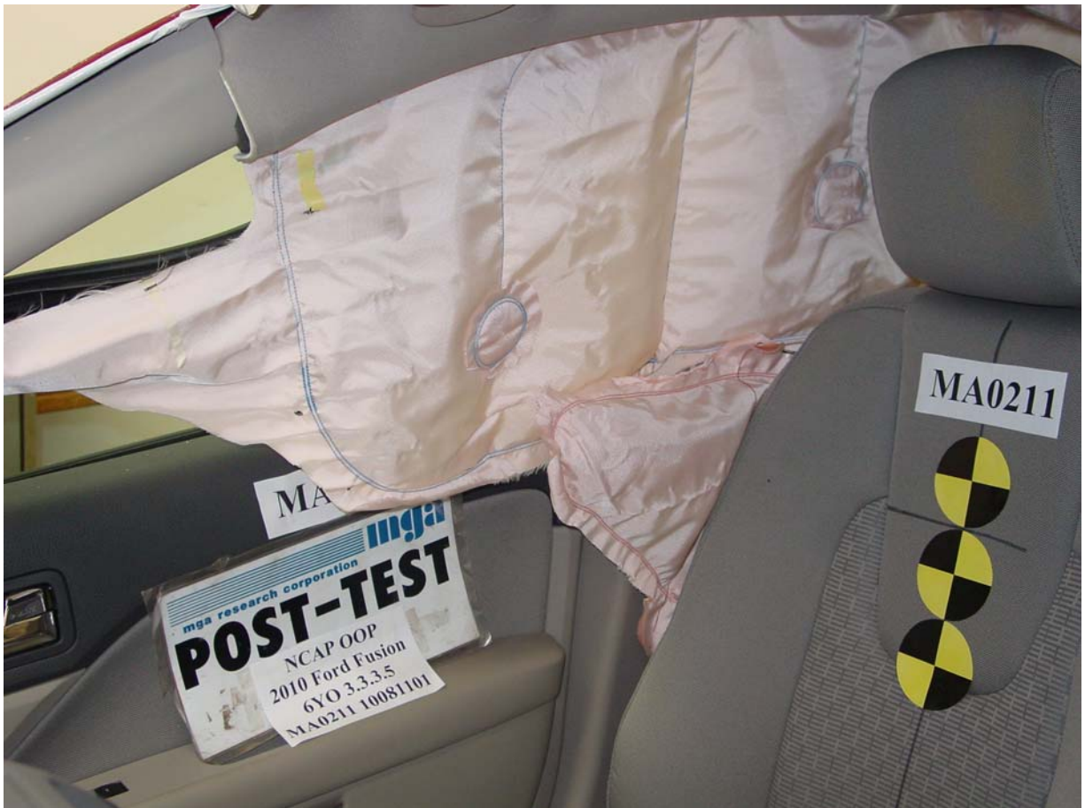
Post-Test Curtain and Torso Airbag Left ¾ Front View
