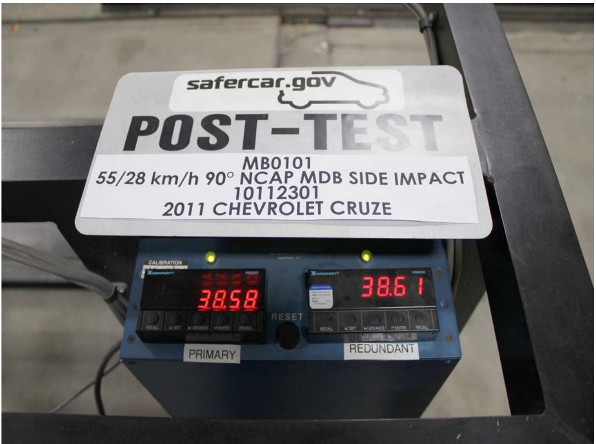
Post-Test Primary and Redundant Speed Trap Read-Out
