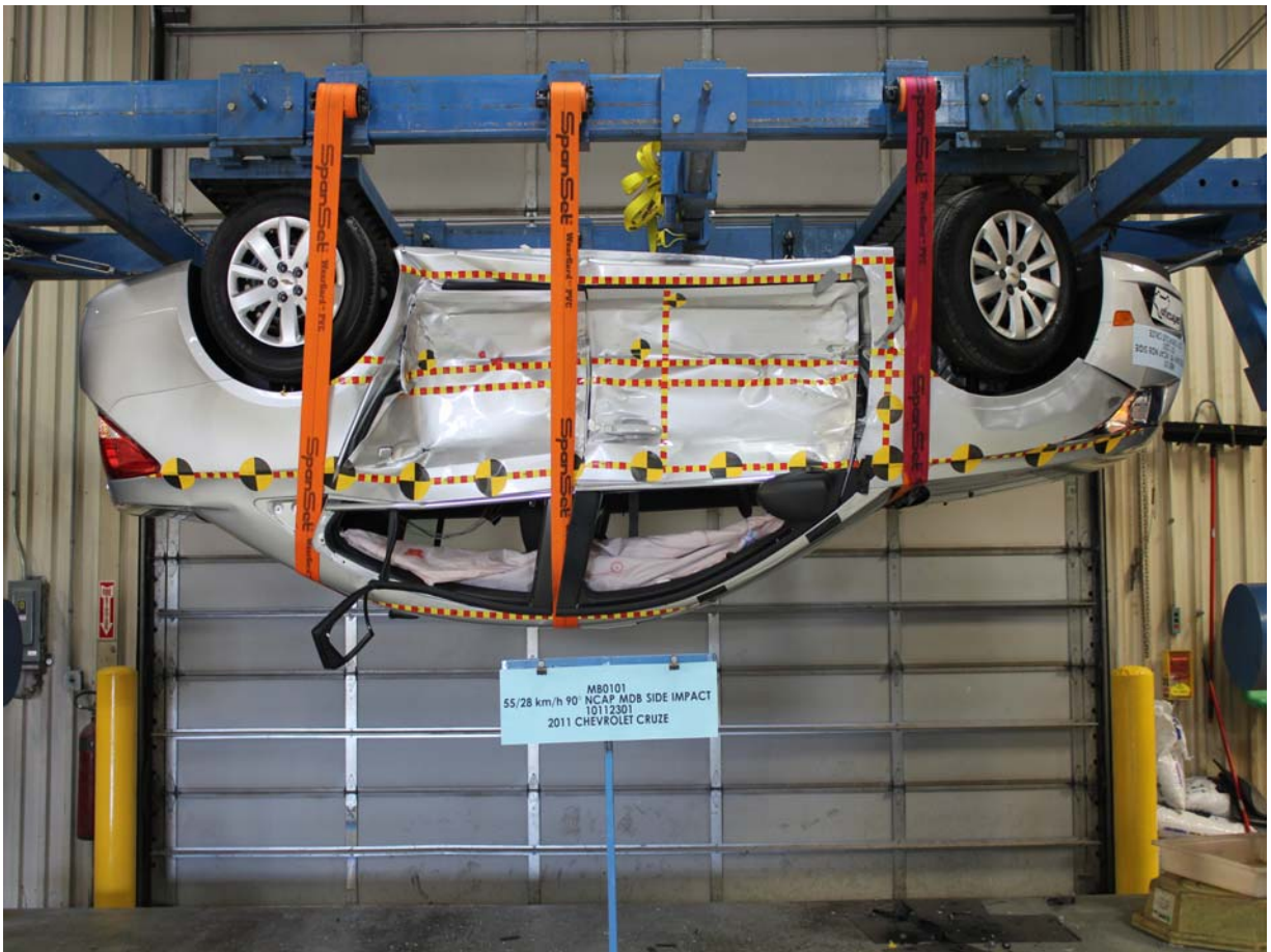
FMVSS No. 301/305 Rollover 180 Degrees
