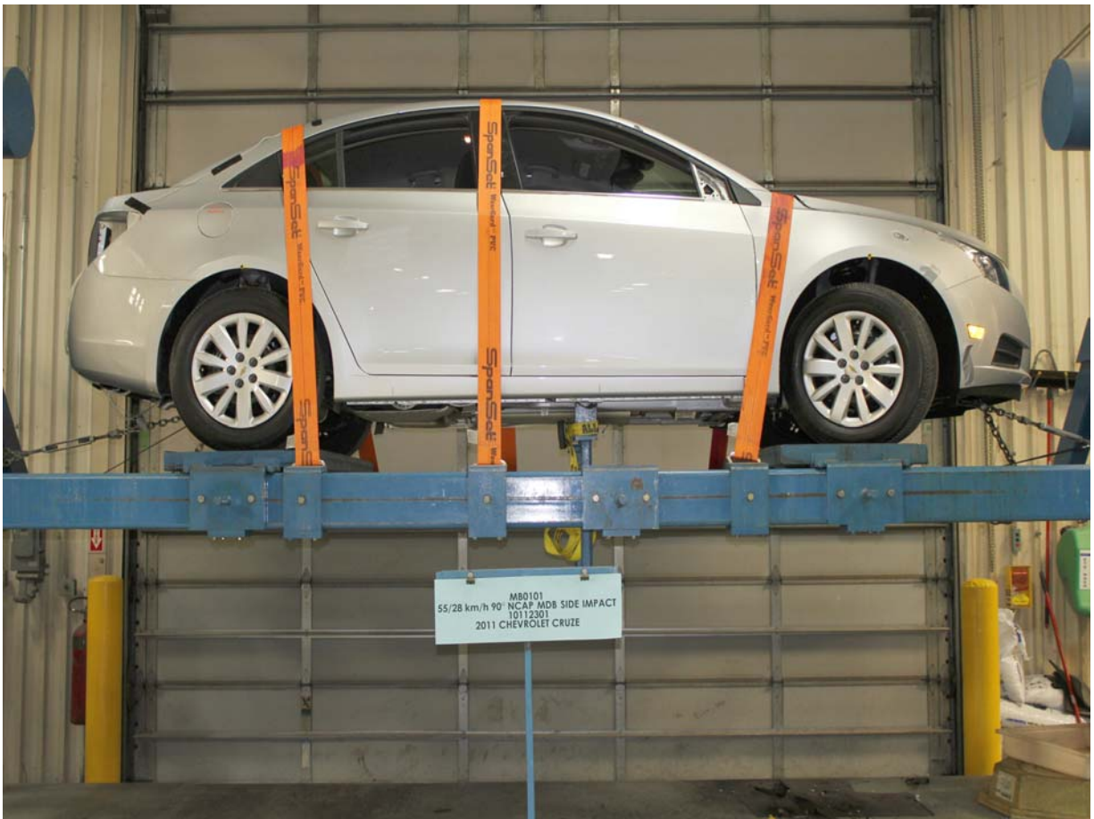
FMVSS No. 301/305 Rollover 0 Degrees
