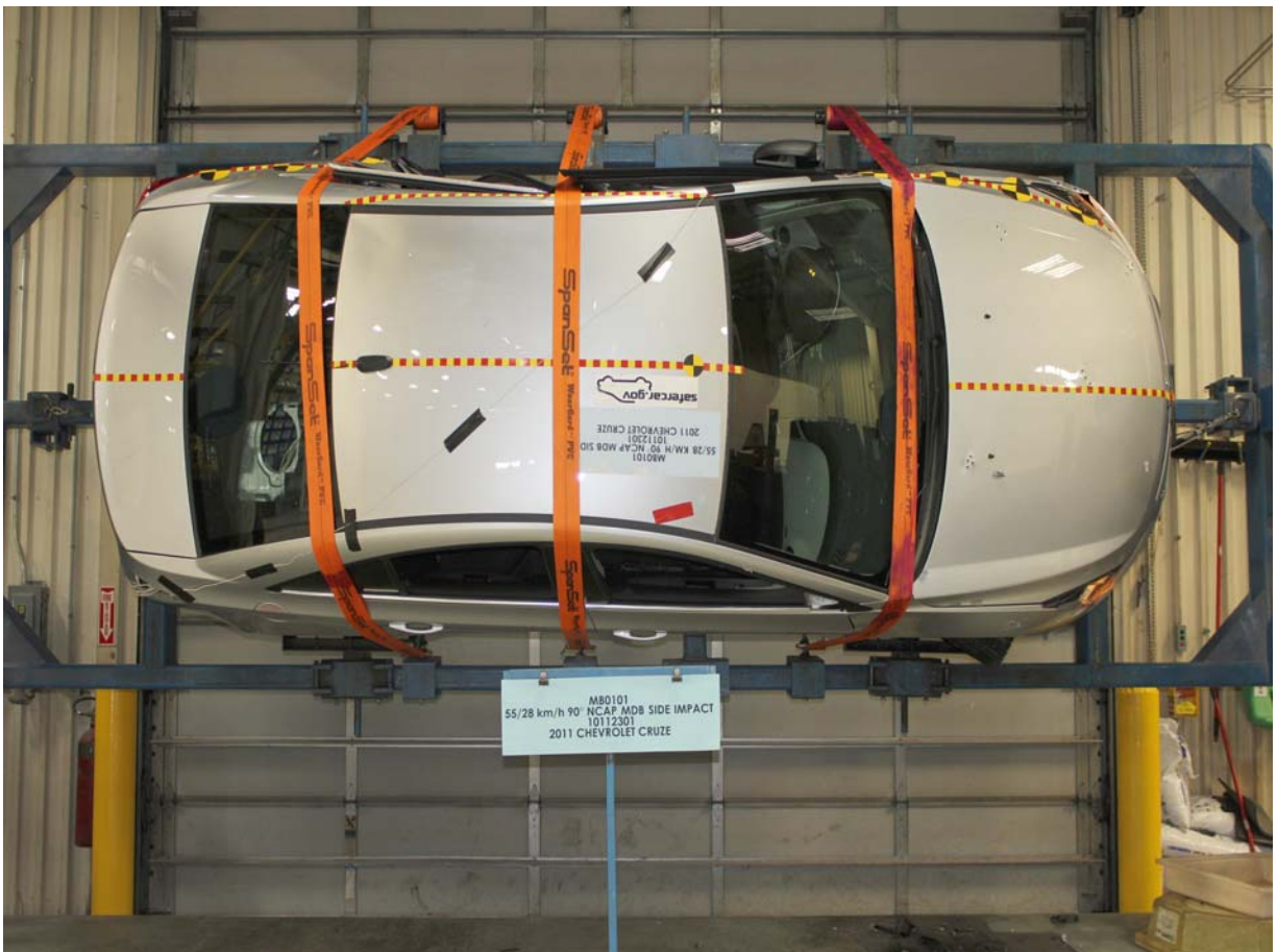
FMVSS No. 301/305 Rollover 90 Degrees
