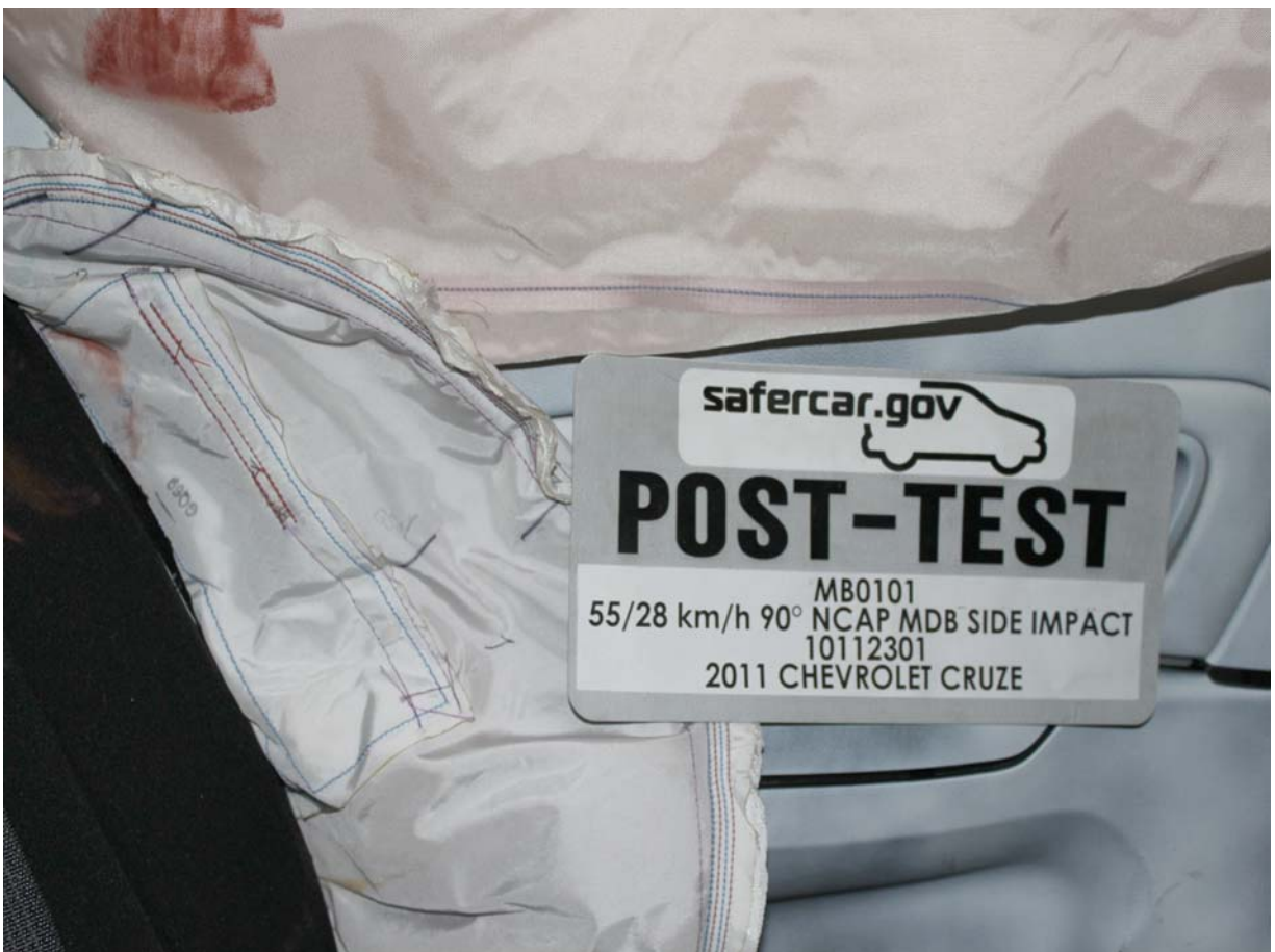
Post-Test Rear Passenger Dummy Close-up Torso Contact with Side Airbag View
