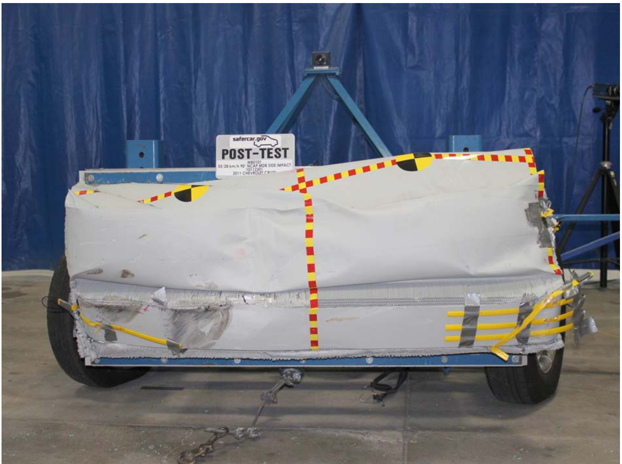
Post-Test Front View of MDB Impactor Face
