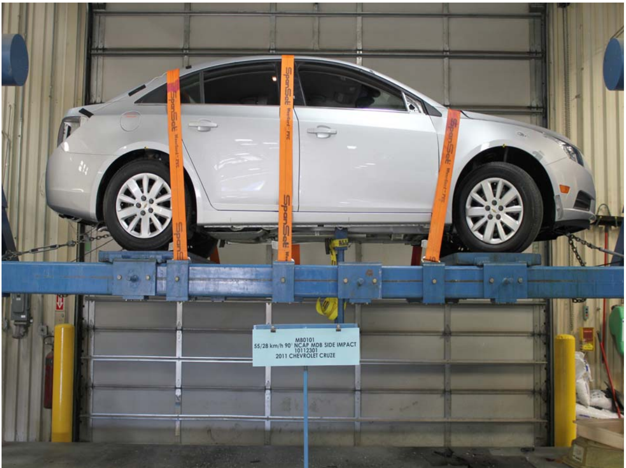
FMVSS No. 301/305 Rollover 360 Degrees
