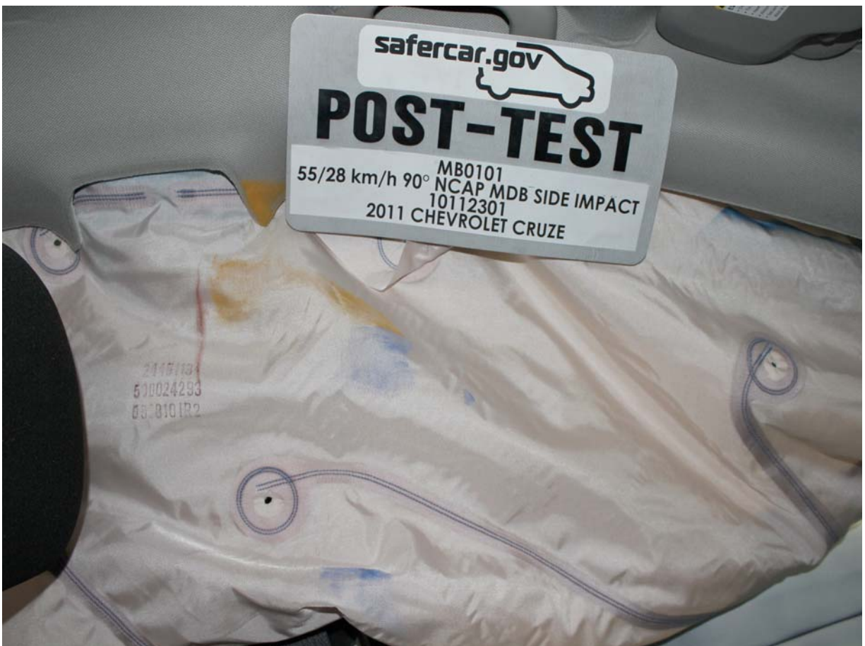
Post-Test Driver Dummy Close-up Head Contact with Side Airbag View
