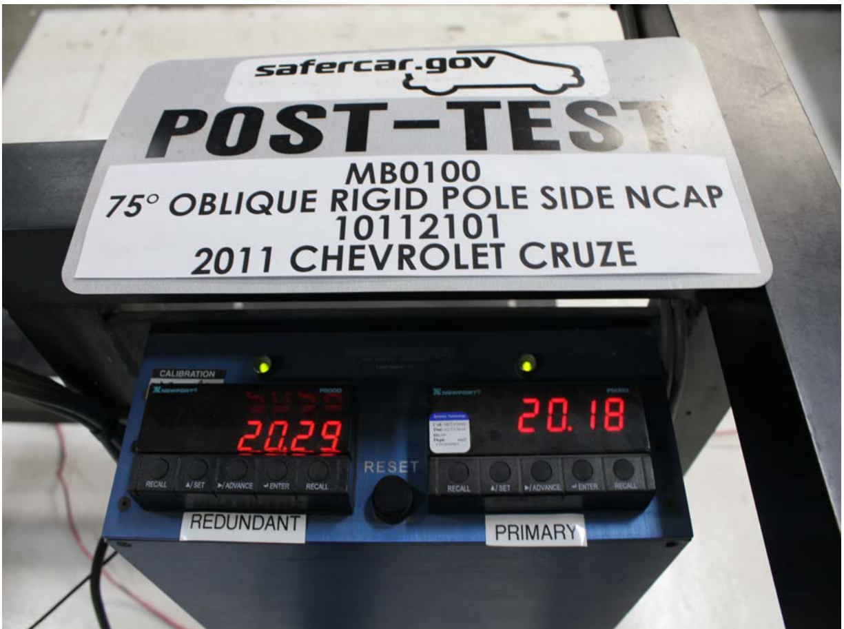
Post-Test Primary and Redundant Speed Trap Read-Out
