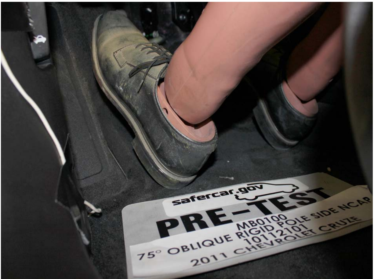
Pre-Test Placement of Dummy's Feet
