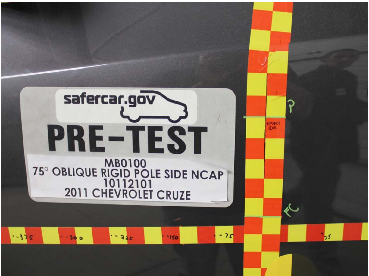
Pre-Test Close-Up View of Impact Point Target
