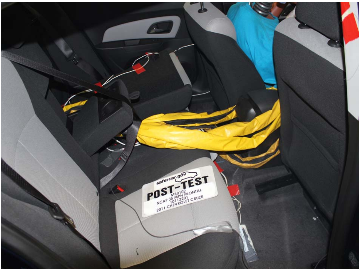
Post-Test Dummy Cable Routing
