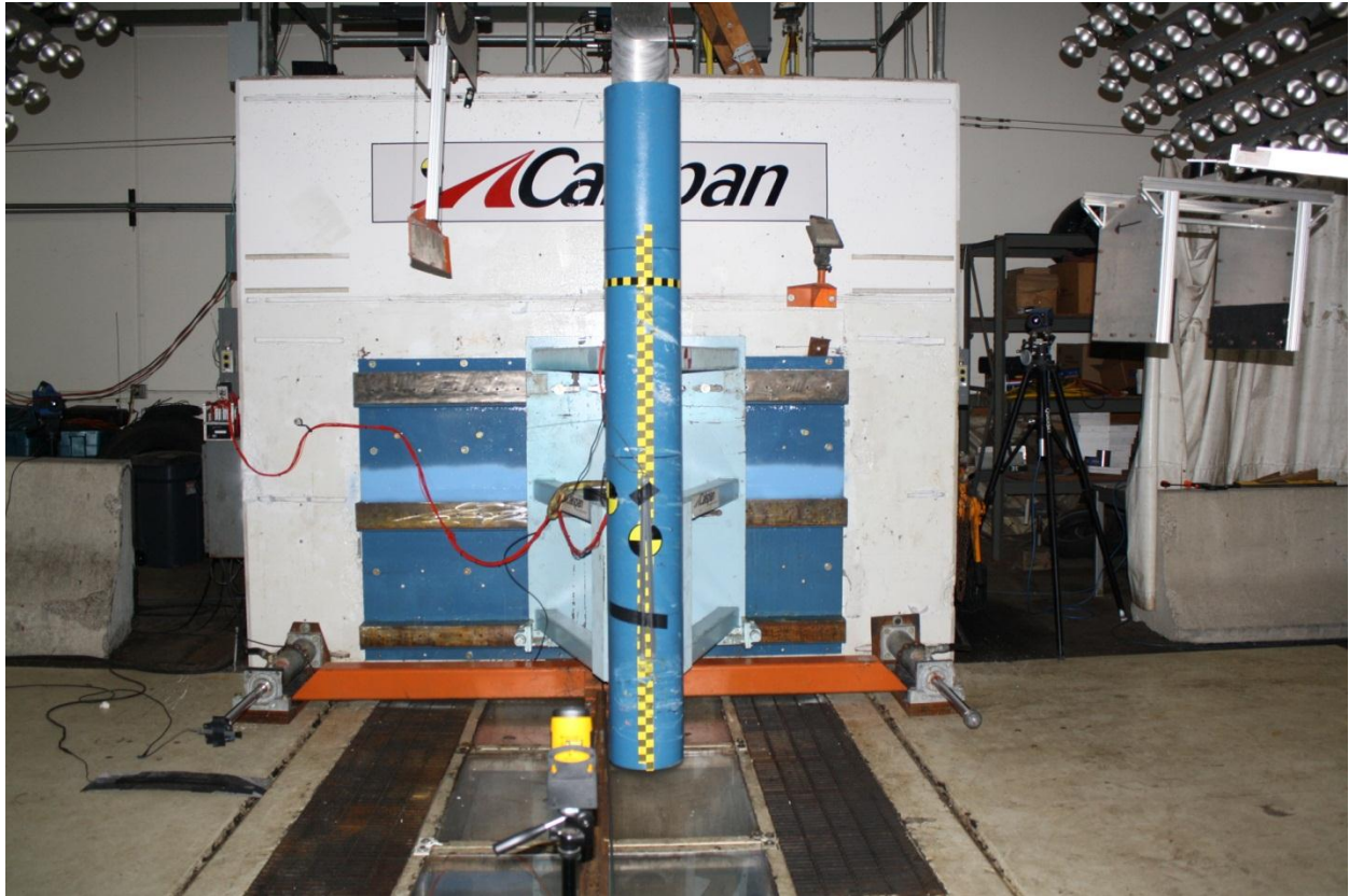
Figure A-55: Pre-Test Pole Barrier Front View
