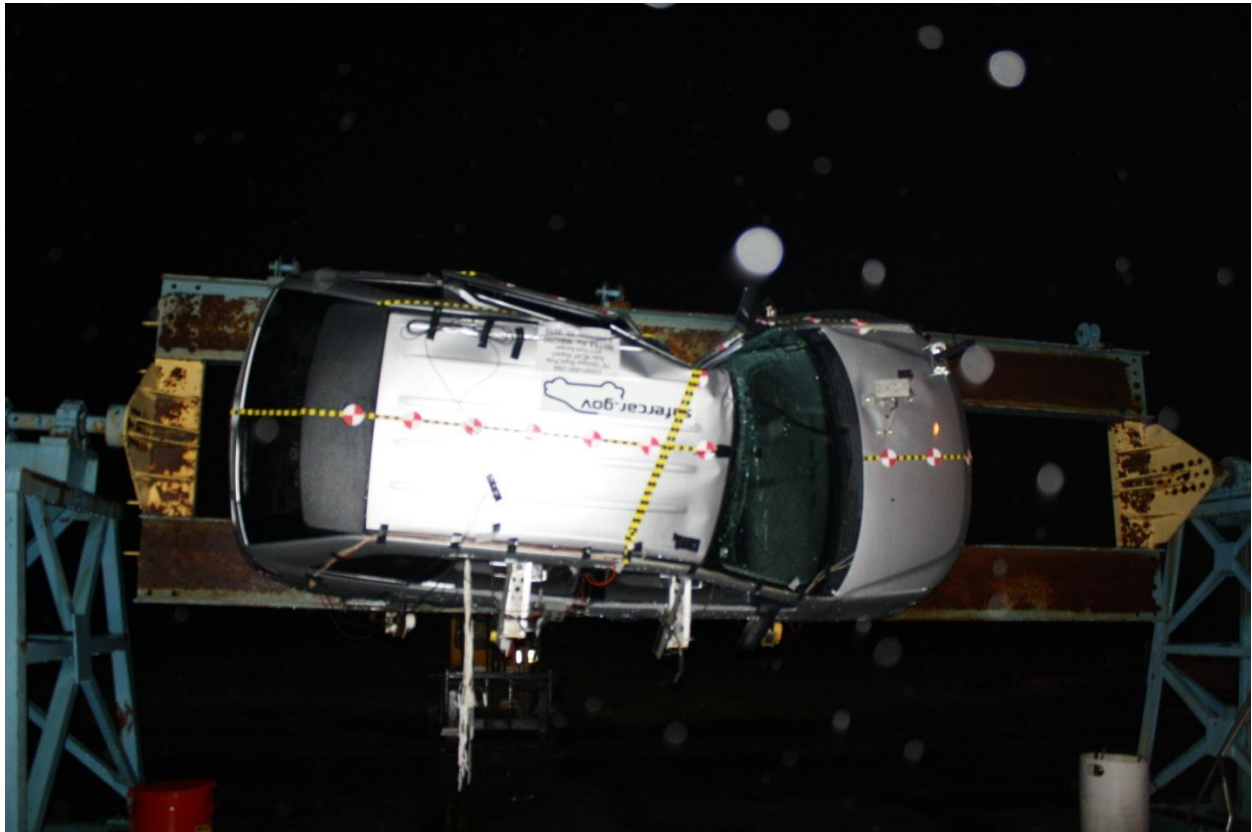
Figure A-64: FMVSS No. 301 Rollover 270°
