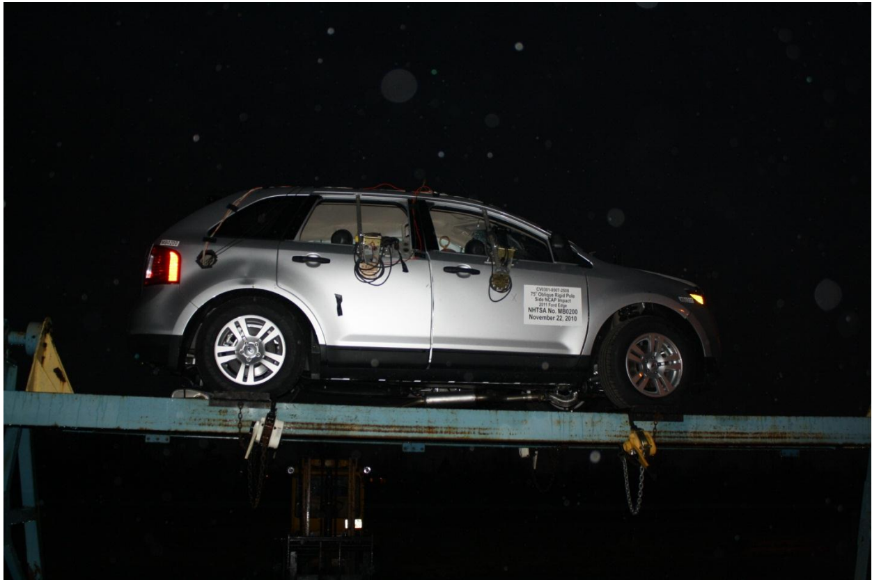
Figure A-61: FMVSS No. 301 Rollover 0°
