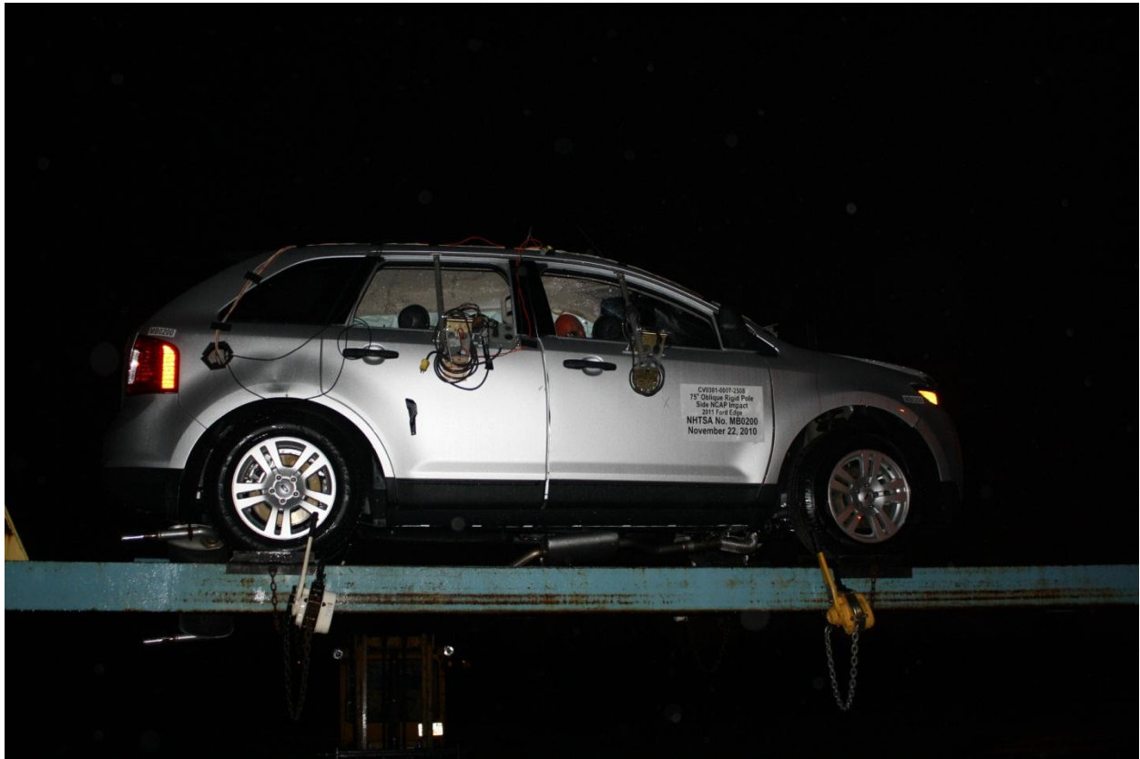
Figure A-65: FMVSS No. 301 Rollover 360°
