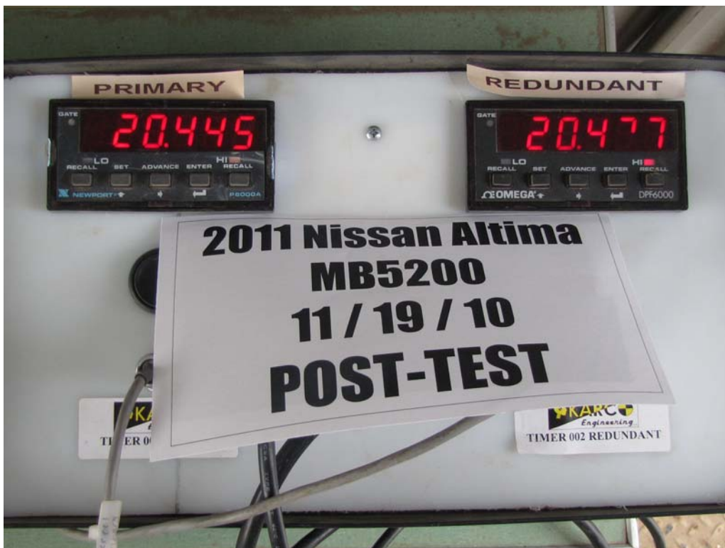
FIGURE 60. Post-Test Primary and Redundant Speed Trap Read-Out
