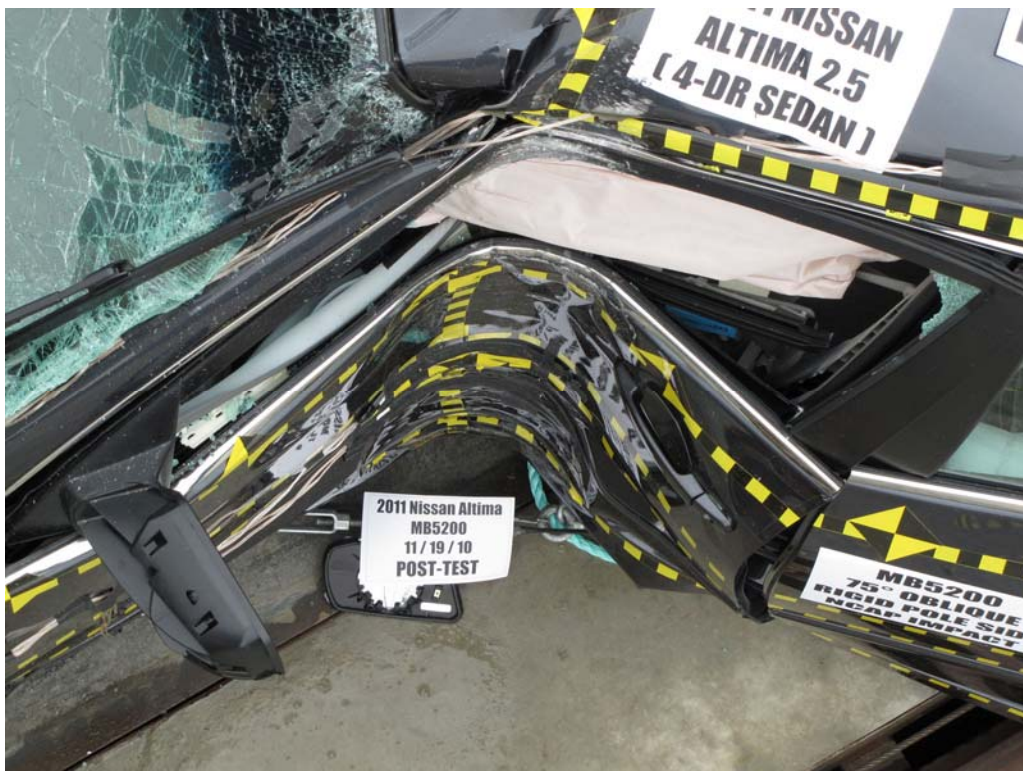
FIGURE 40. Post-Test Driver Dummy and Door Clearance
