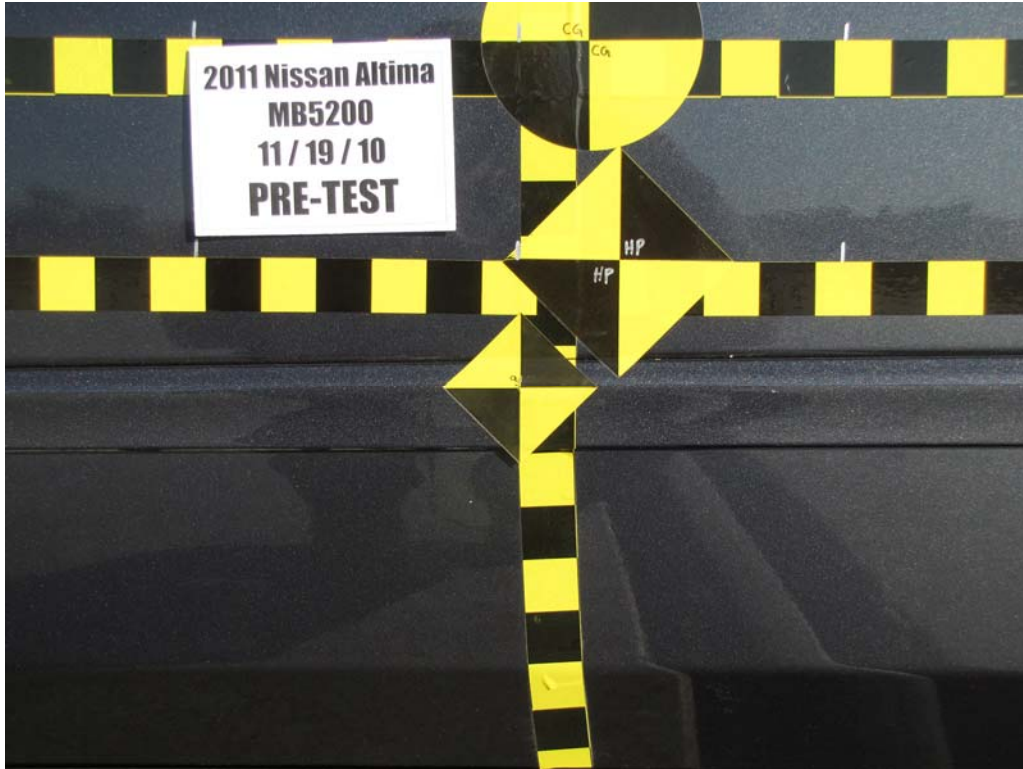
FIGURE 19. Pre-Test Close-Up View of Impact Point Target
