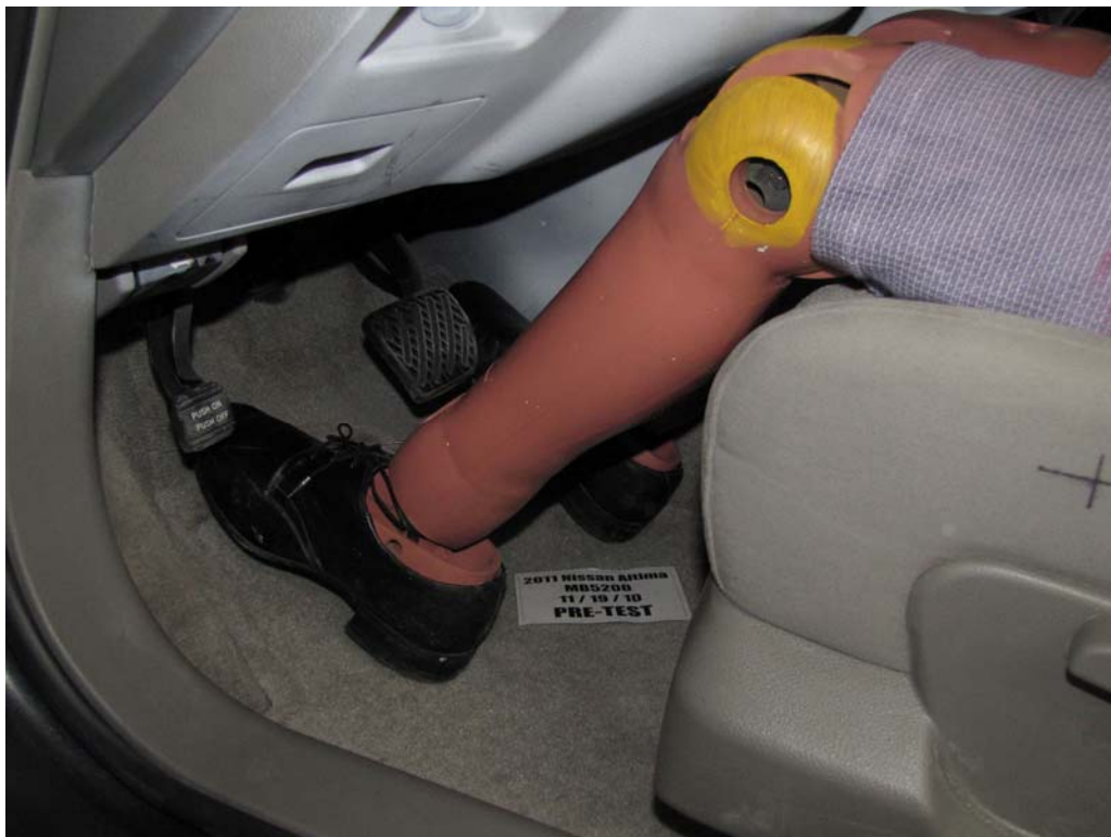
FIGURE 32. Pre-Test Placement of Dummy's Feet
