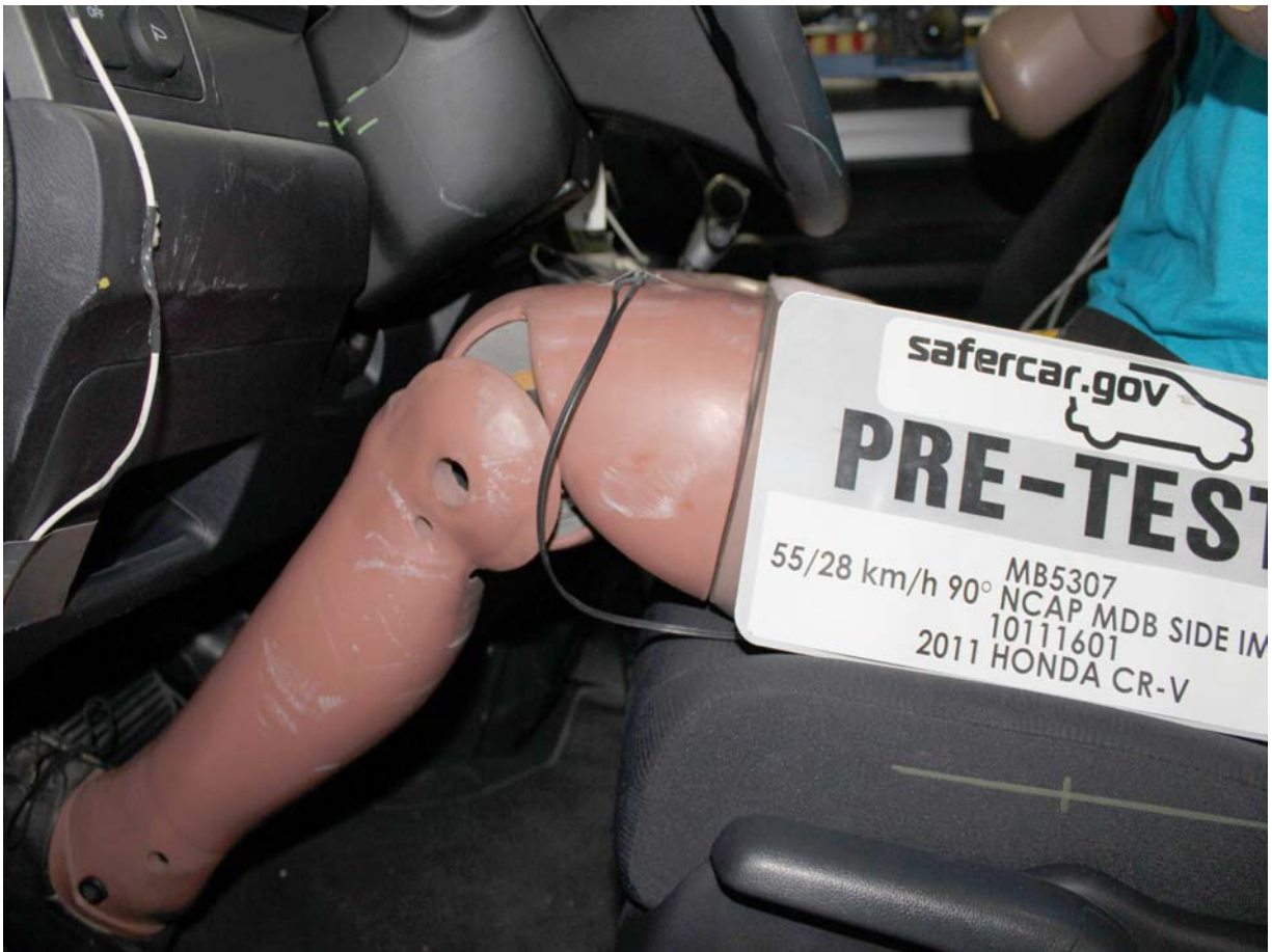
Pre-Test Placement of Driver Dummy's Feet
