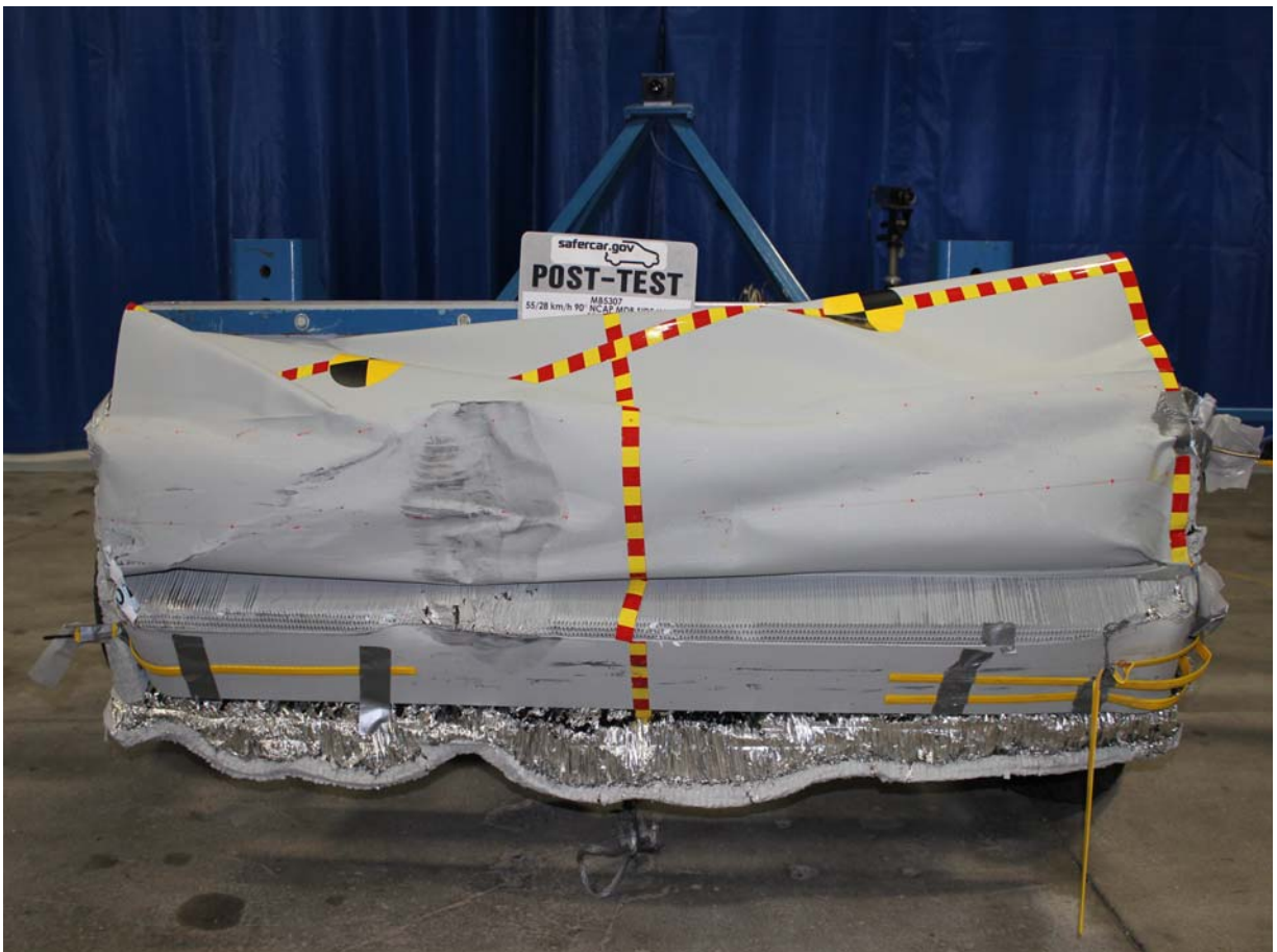
Post-Test Front View of MDB Impactor Face
