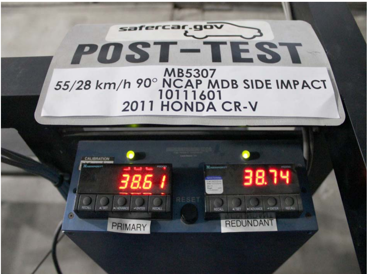
Post-Test Primary and Redundant Speed Trap Read-Out
