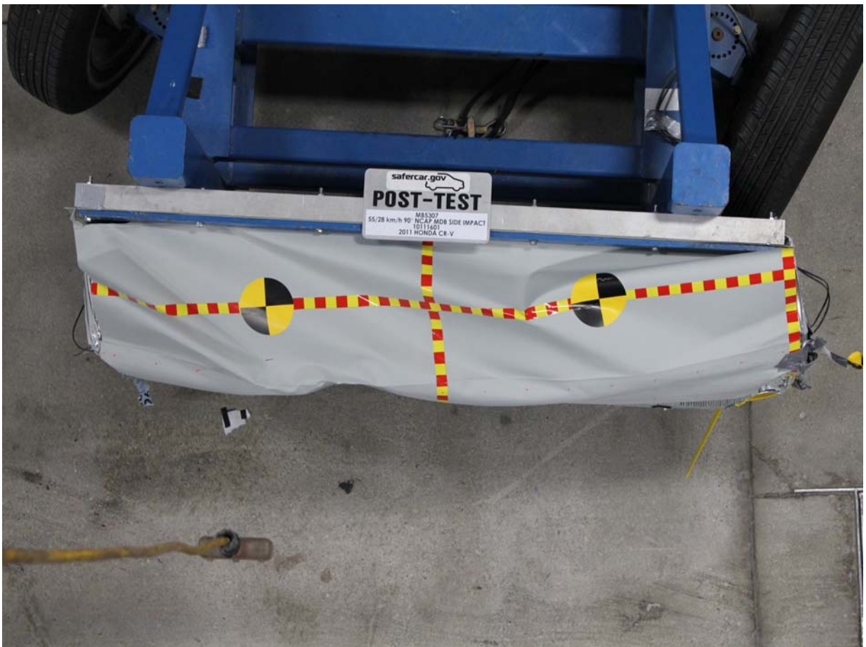
Post-Test Top View of MDB Impactor Face
