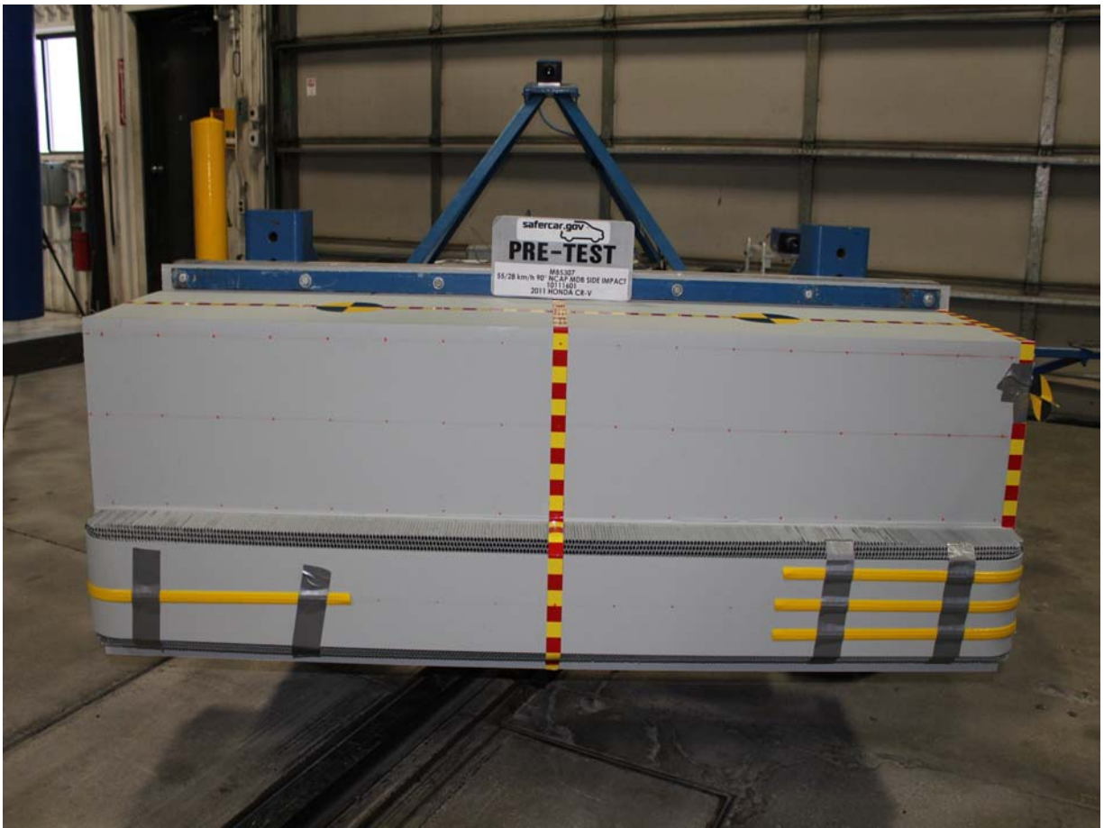
Pre-Test Front View of MDB Impactor Face
