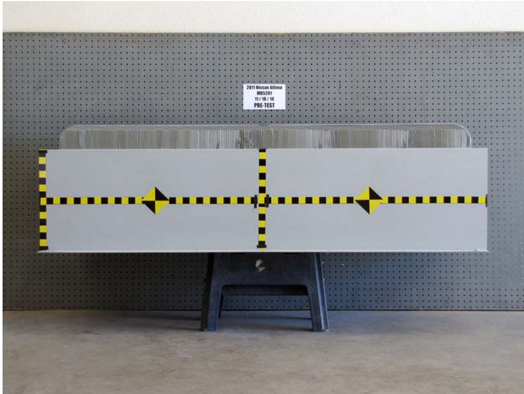
FIGURE 83. Pre-Test Top View of MDB Impactor Face
