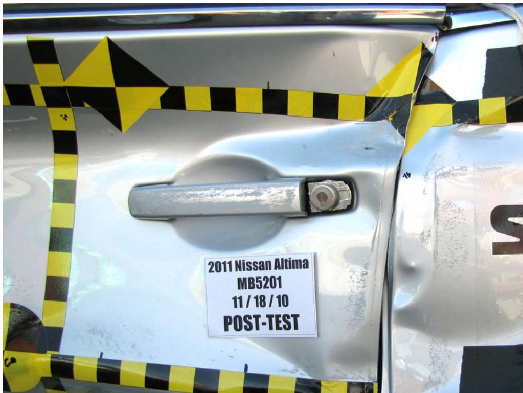
FIGURE 22. Post-Test Left Front Door Latch Close-Up
