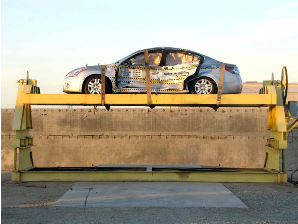
FIGURE 97. FMVSS No. 301/305 Rollover 360 Degrees
