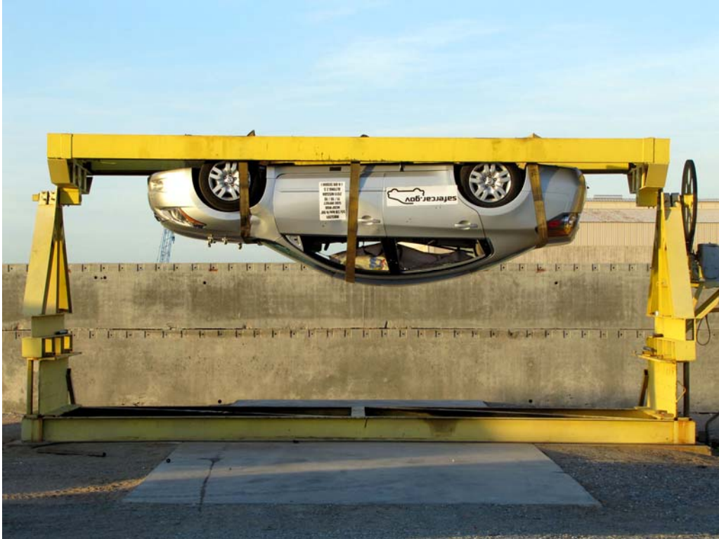
FIGURE 95. FMVSS No. 301/305 Rollover 180 Degrees
