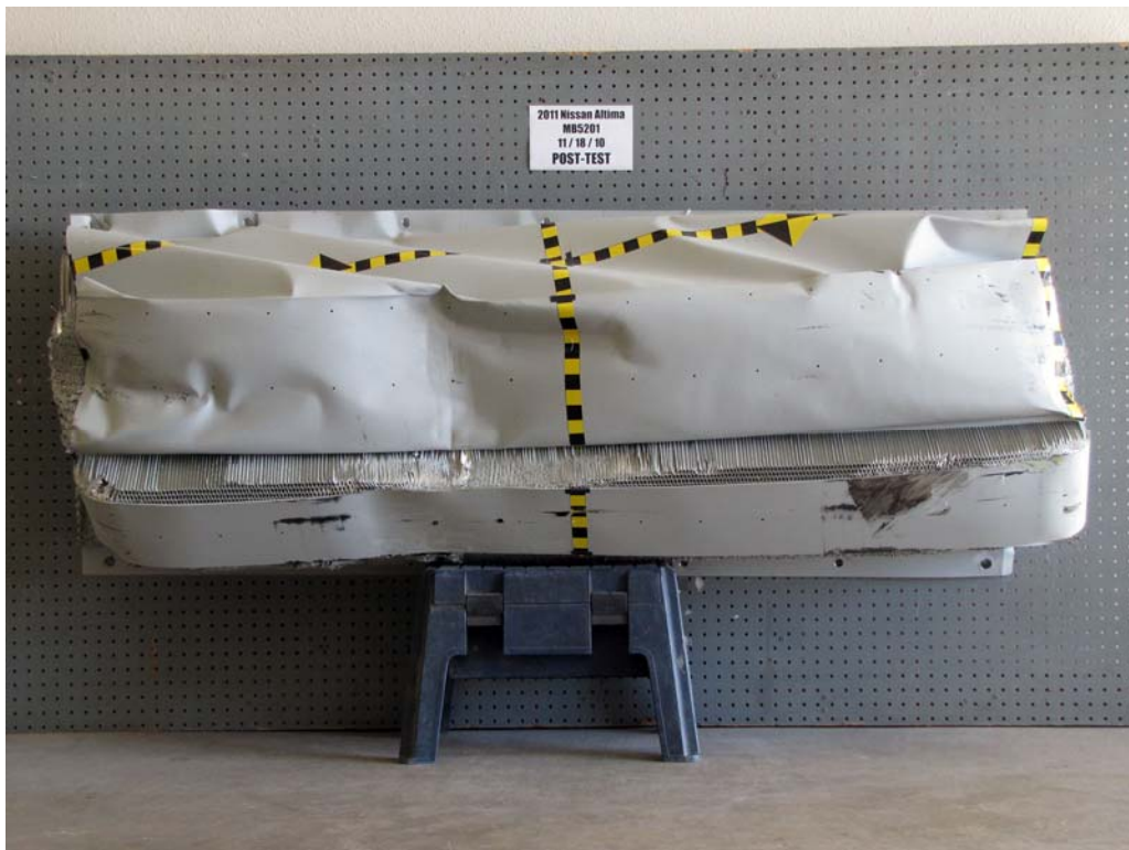
FIGURE 82. Post-Test Front View of MDB Impactor Face
