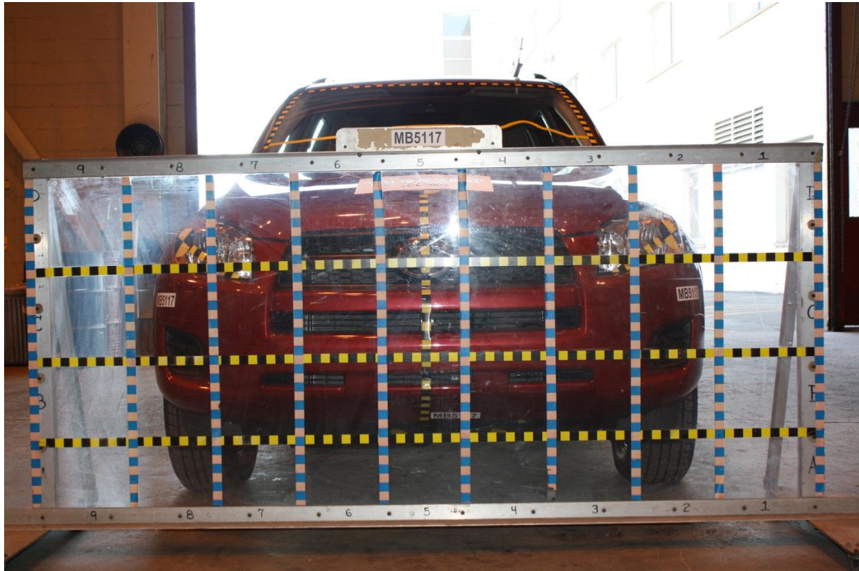
Figure A-1: Load Cell Location
