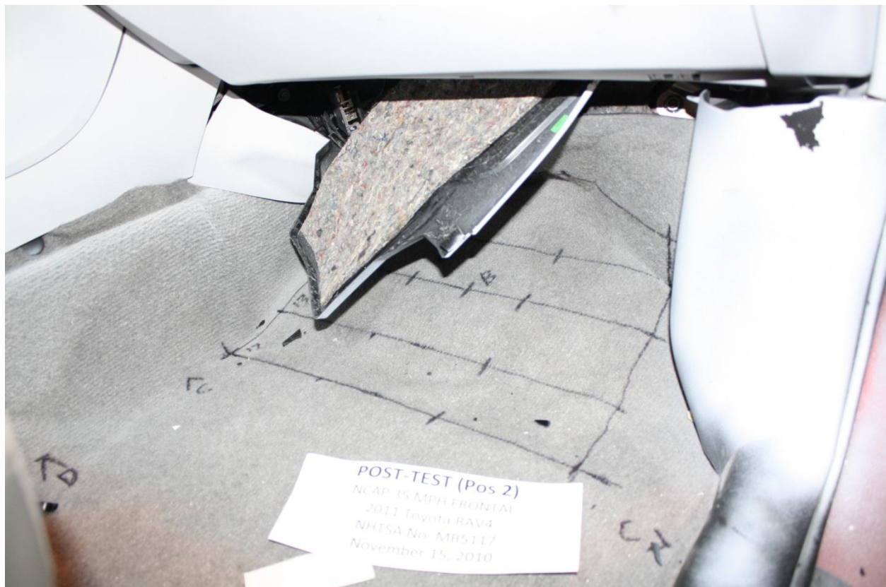
Figure A-59: Post-Test Passenger's Floorpan
