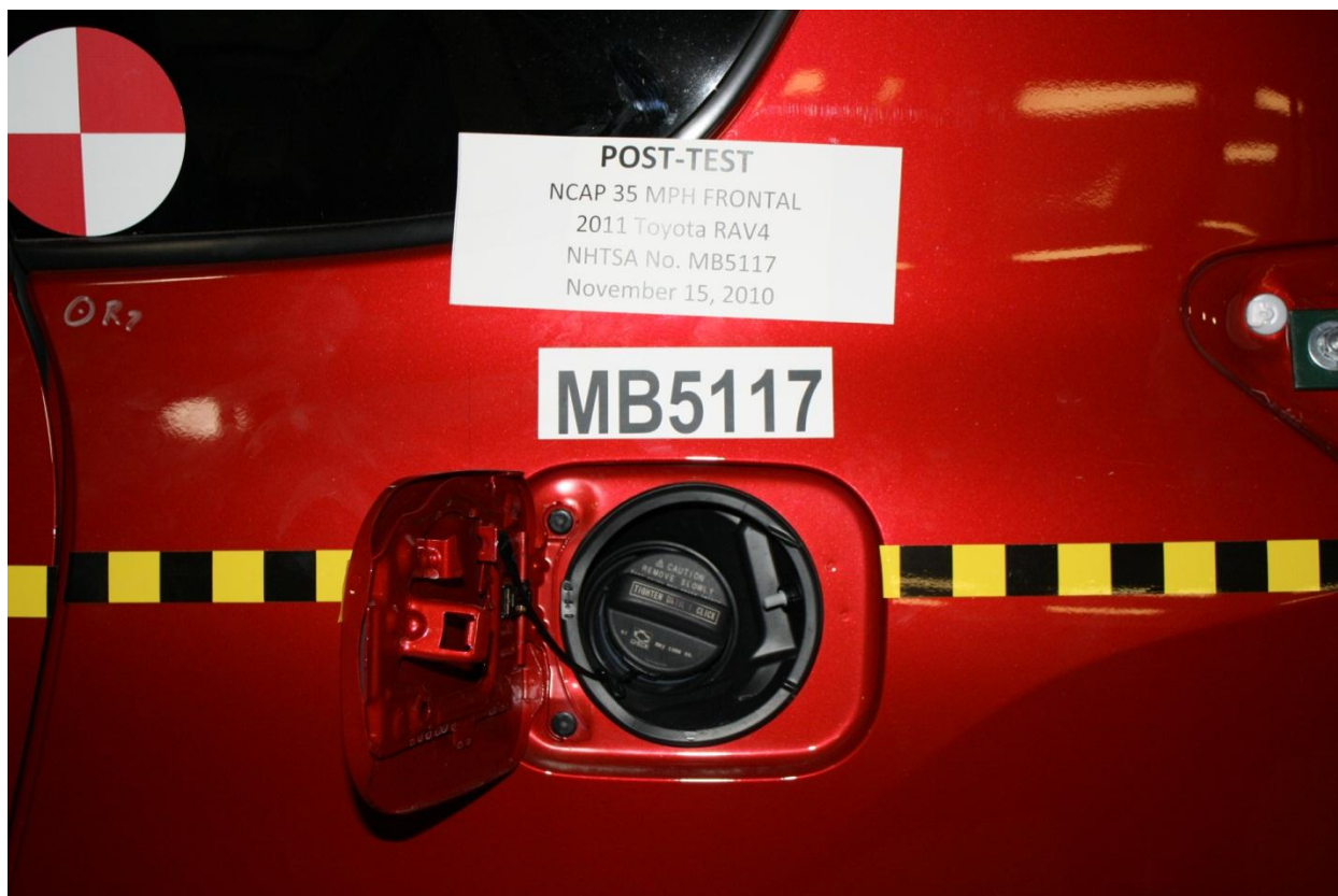
Figure A-22: Post-Test Fuel Filler Cap View
