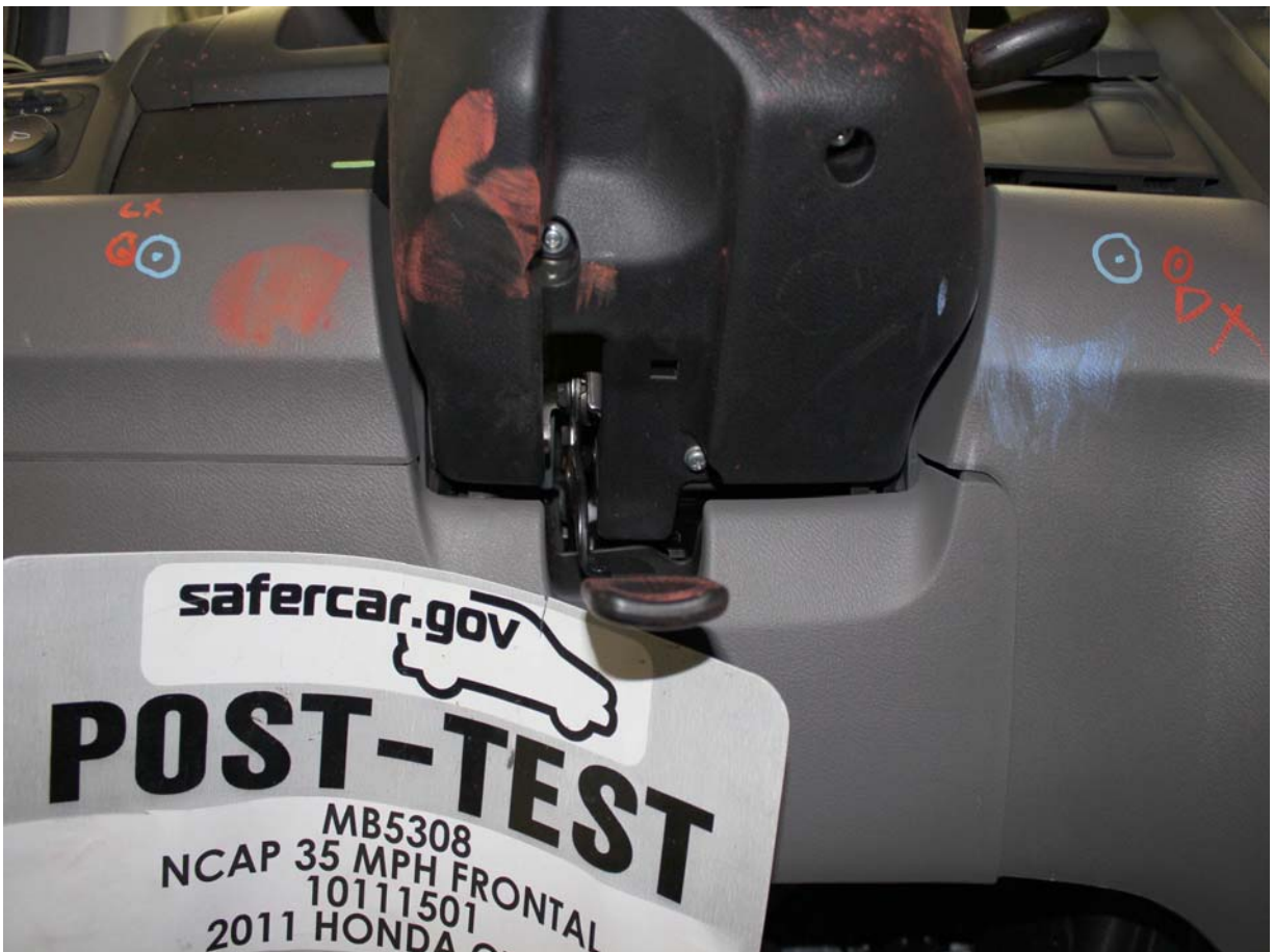
Post-Test Driver Dummy Contact with Knee Bolster
