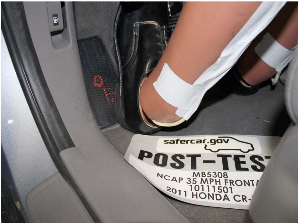
Post-Test Driver Dummy Feet
