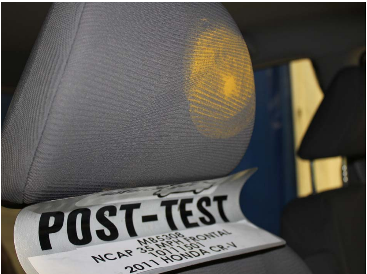
Post-Test Passenger Dummy Contact with Headrest
