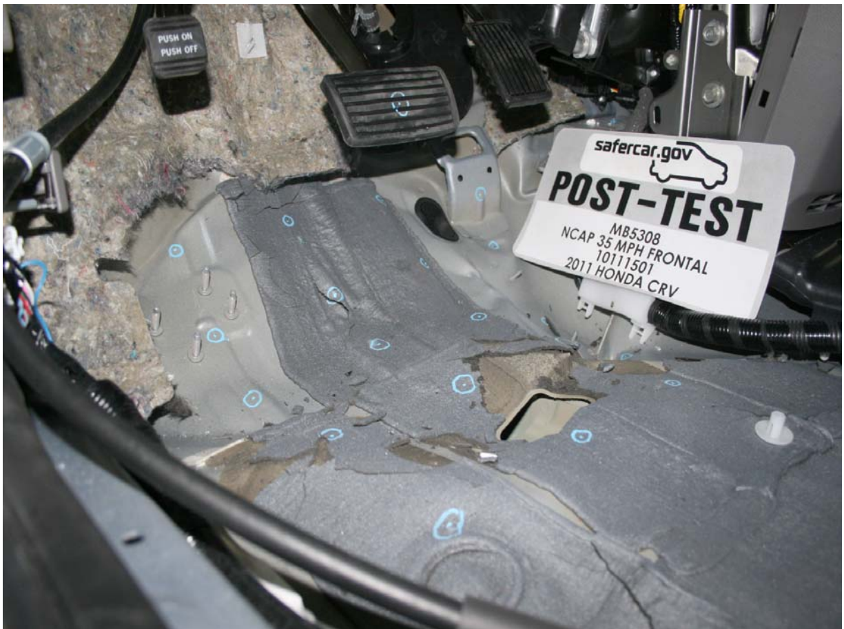
Post-Test Driver's Side Floorpan
