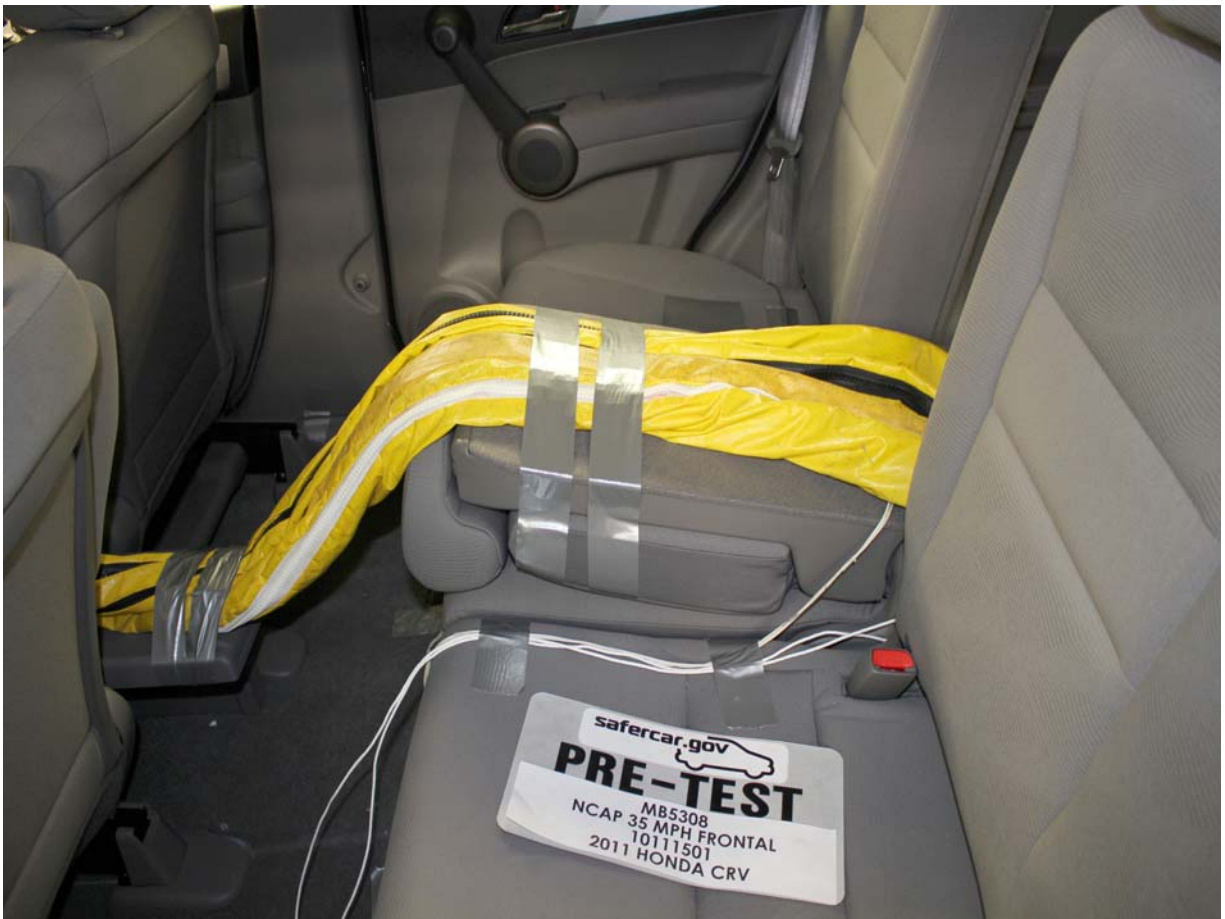
Pre-Test Dummy Cable Routing
