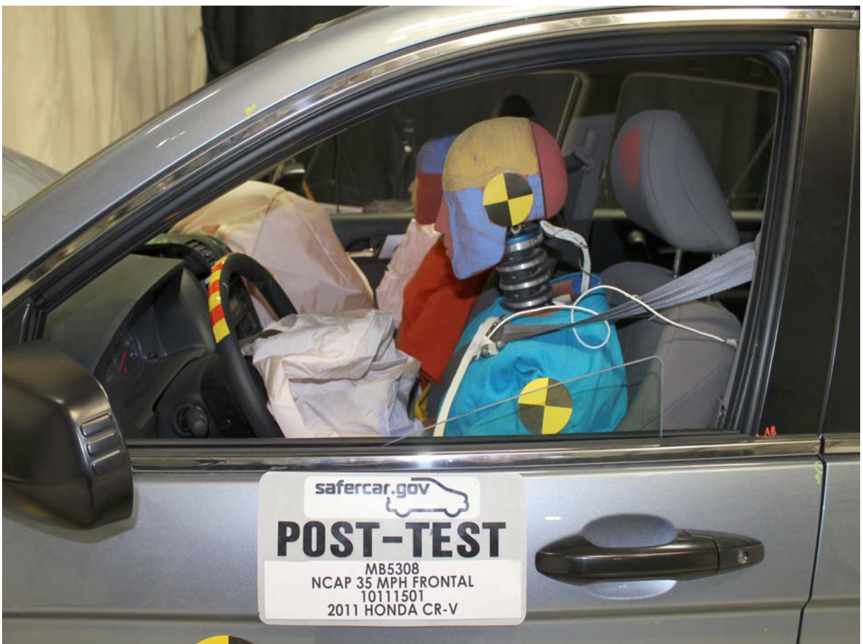
Post-Test Driver Dummy Window View
