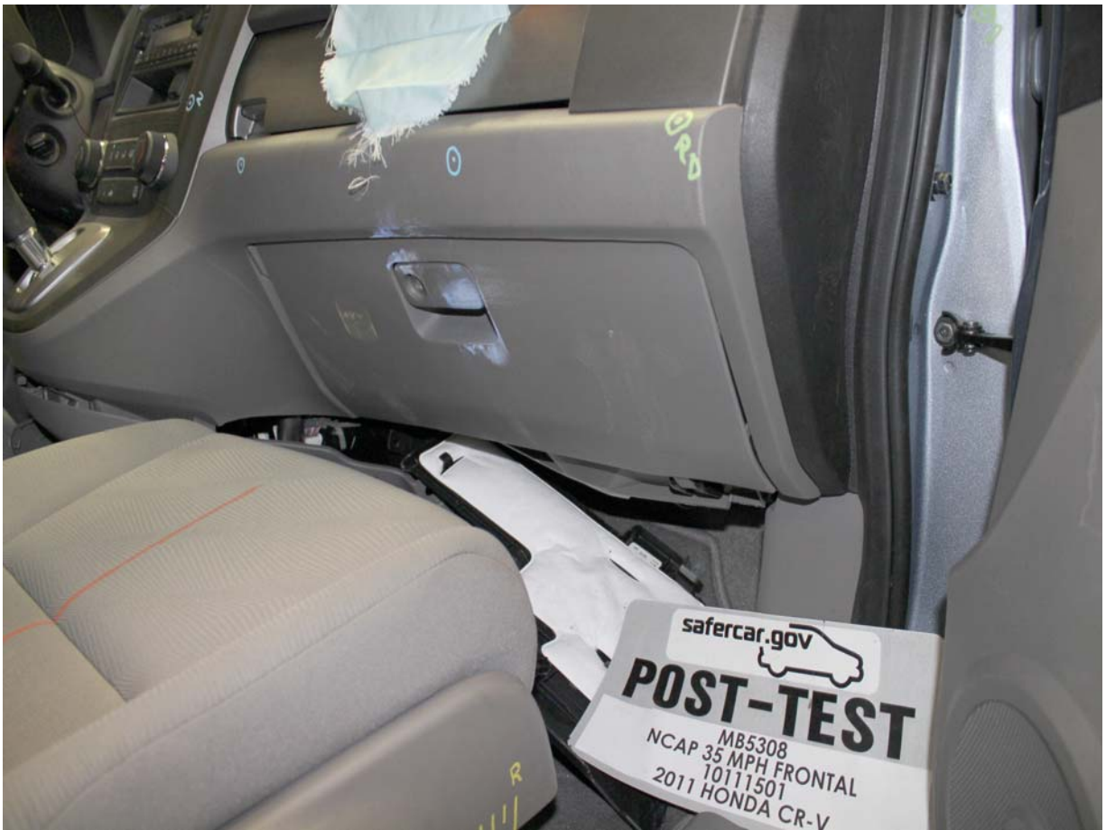
Post-Test Passenger Dummy Contact with Glovebox
