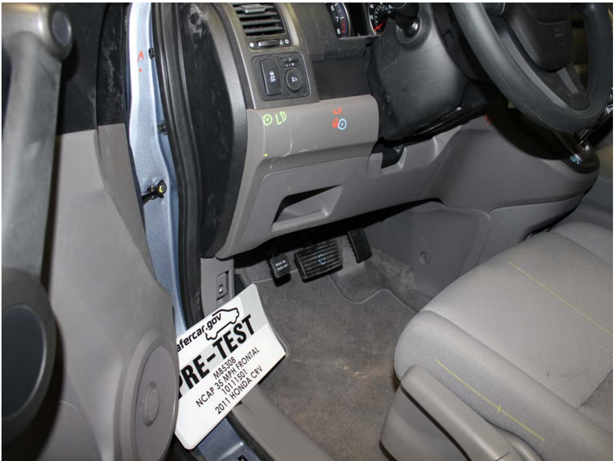
Pre-Test Driver's Side Knee Bolster (without dummy)
