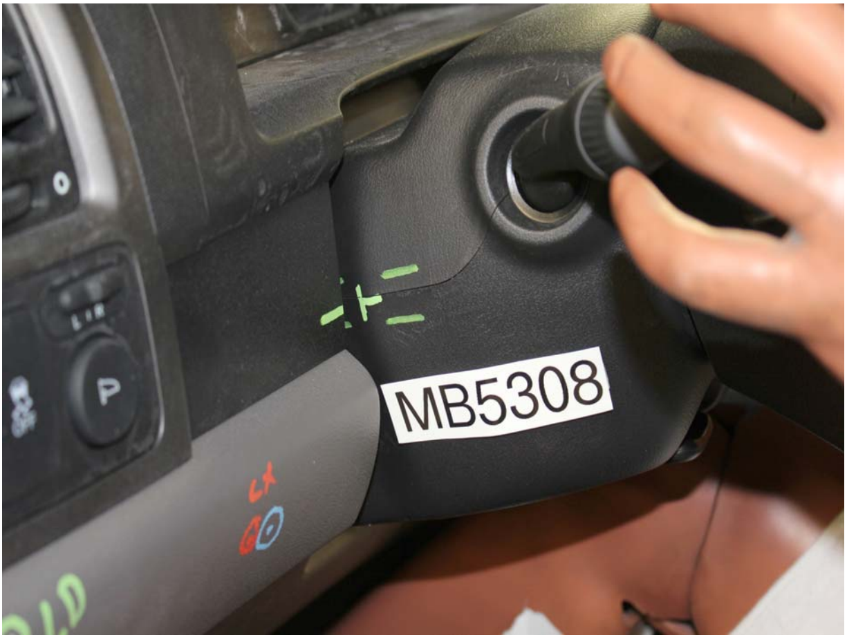
Pre-Test View of Steering Column Shear Capsule
