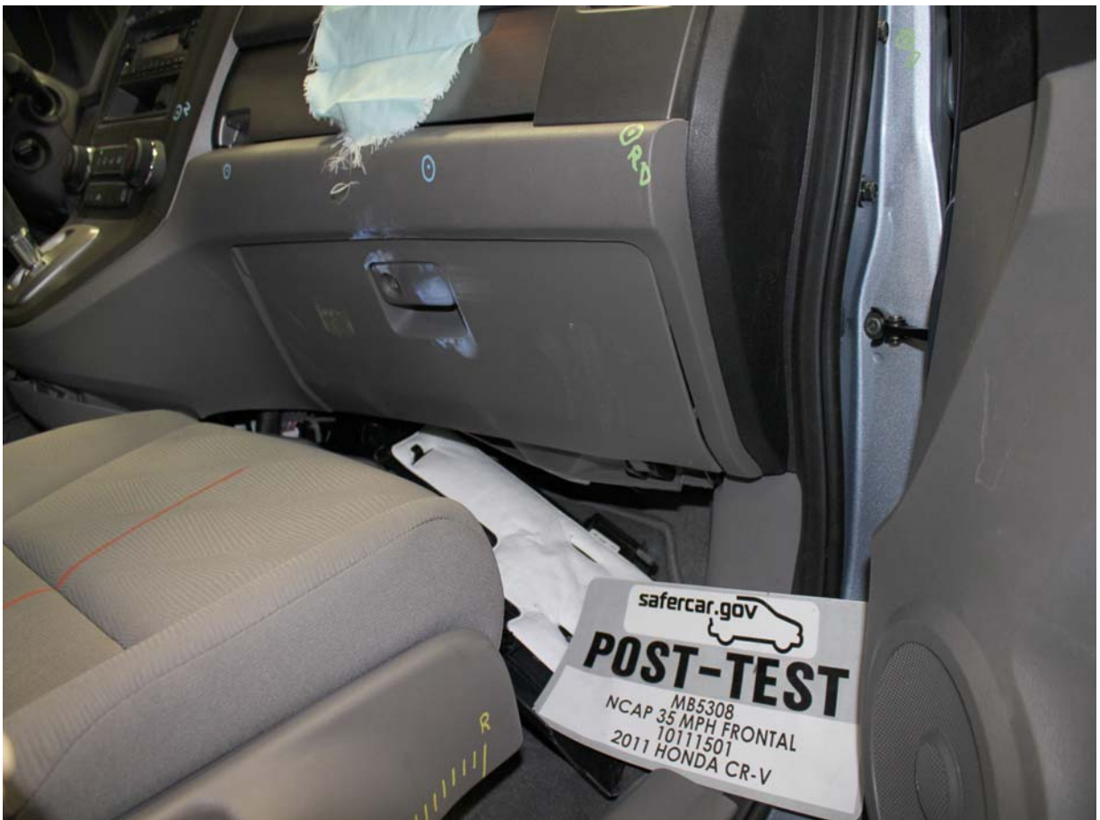
Post-Test Passenger's Side Knee Bolster (without dummy)
