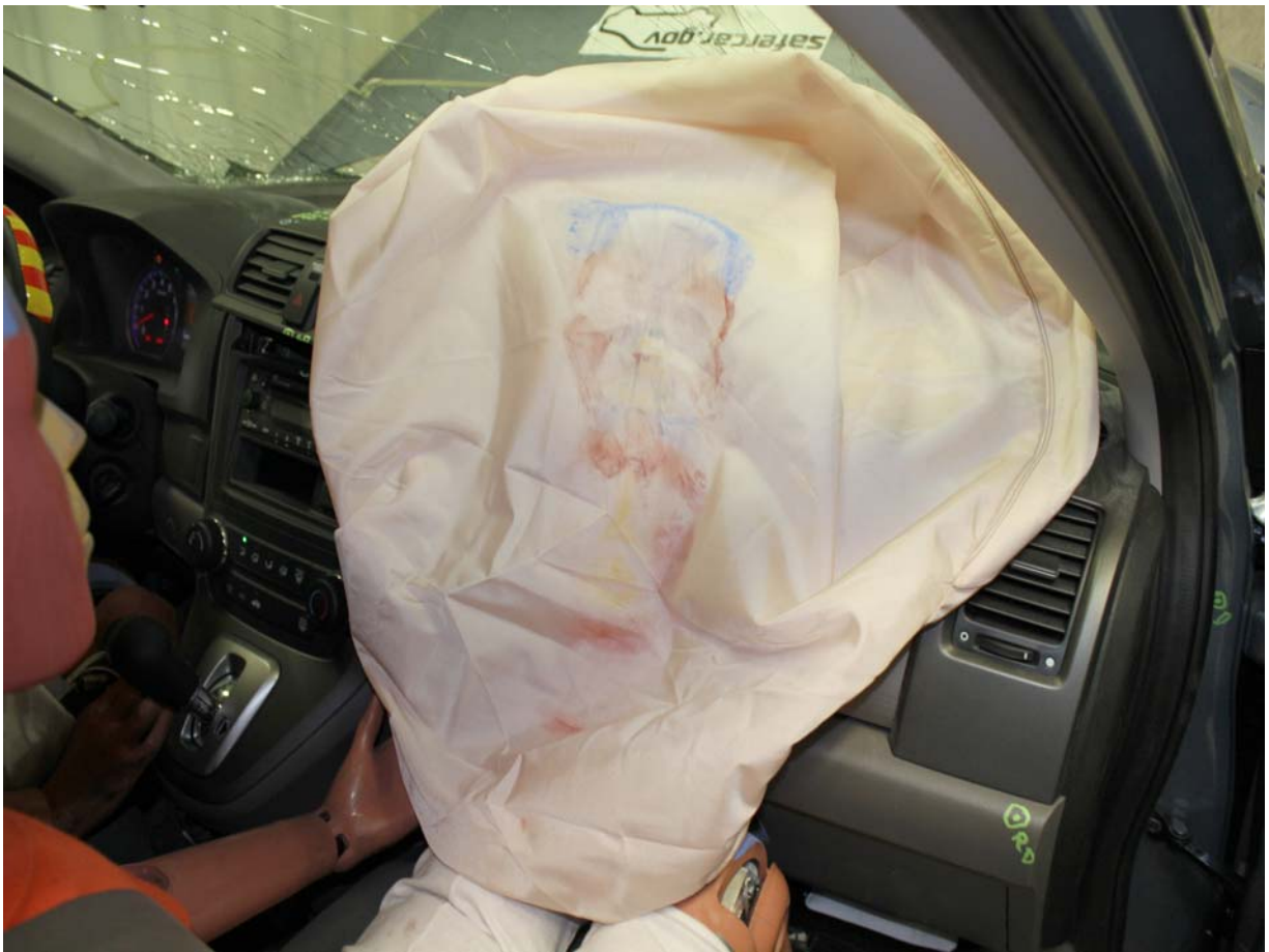
Post-Test Passenger Dummy Contact with Airbag
