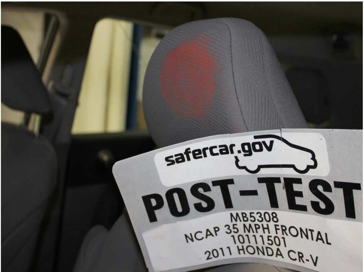
Post-Test Driver Dummy Contact with Headrest
