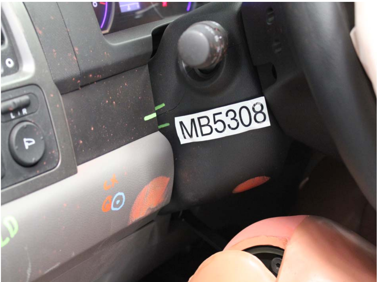
Post-Test View of Steering Column Shear Capsule
