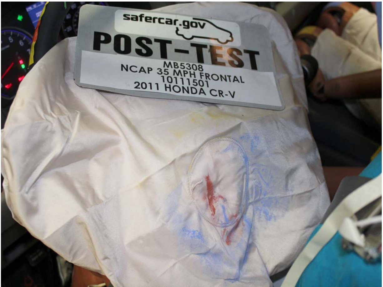
Post-Test Driver Dummy Contact with Airbag
