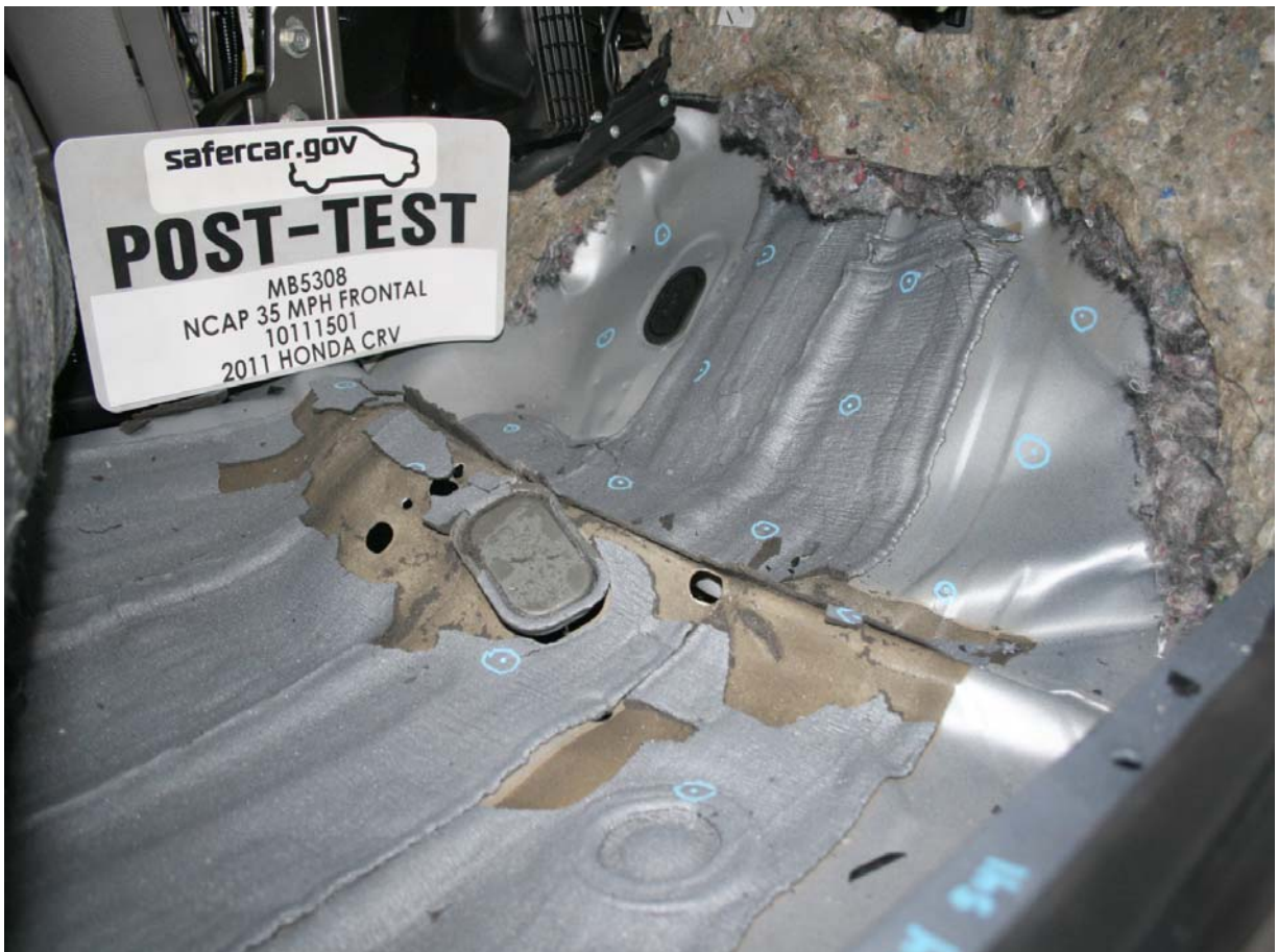
Post-Test Passenger's Side Floorpan
