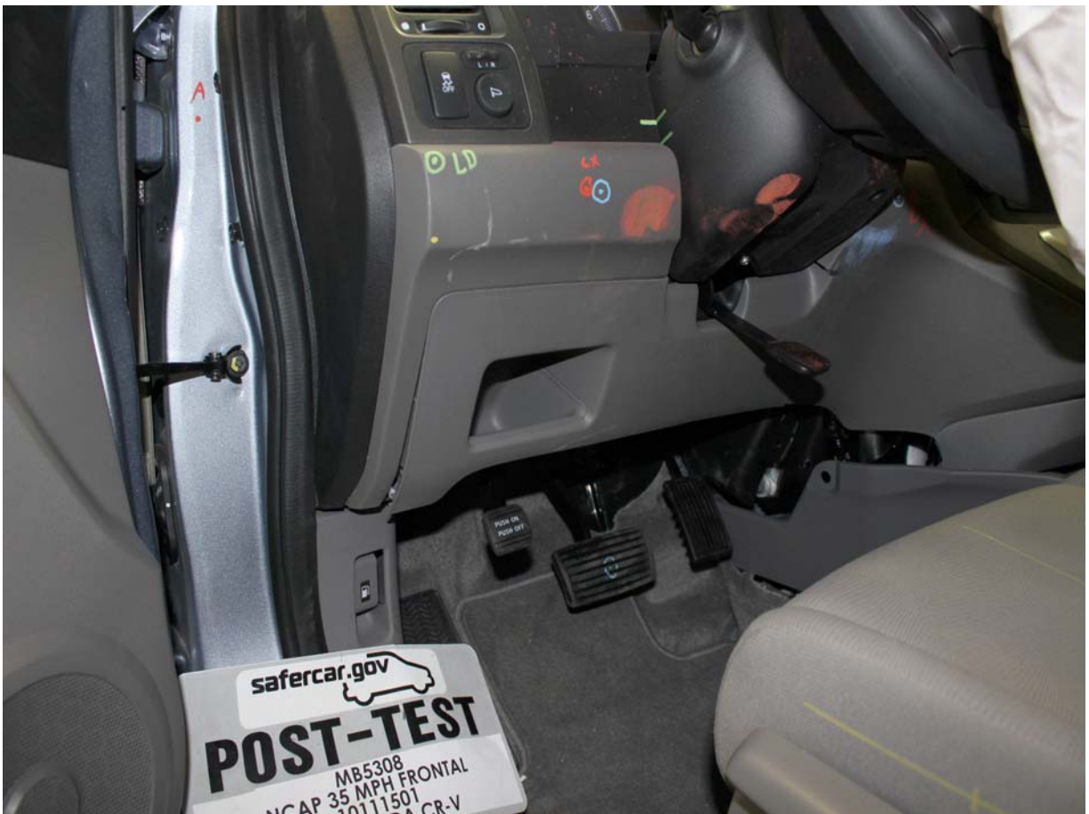
Post-Test Driver's Side Knee Bolster (without dummy)
