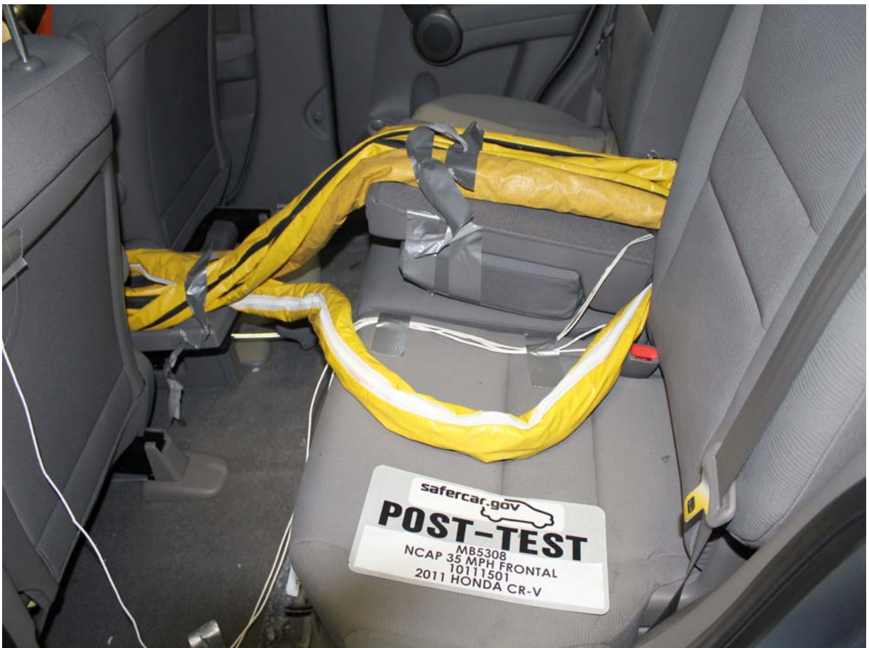
Post-Test Dummy Cable Routing
