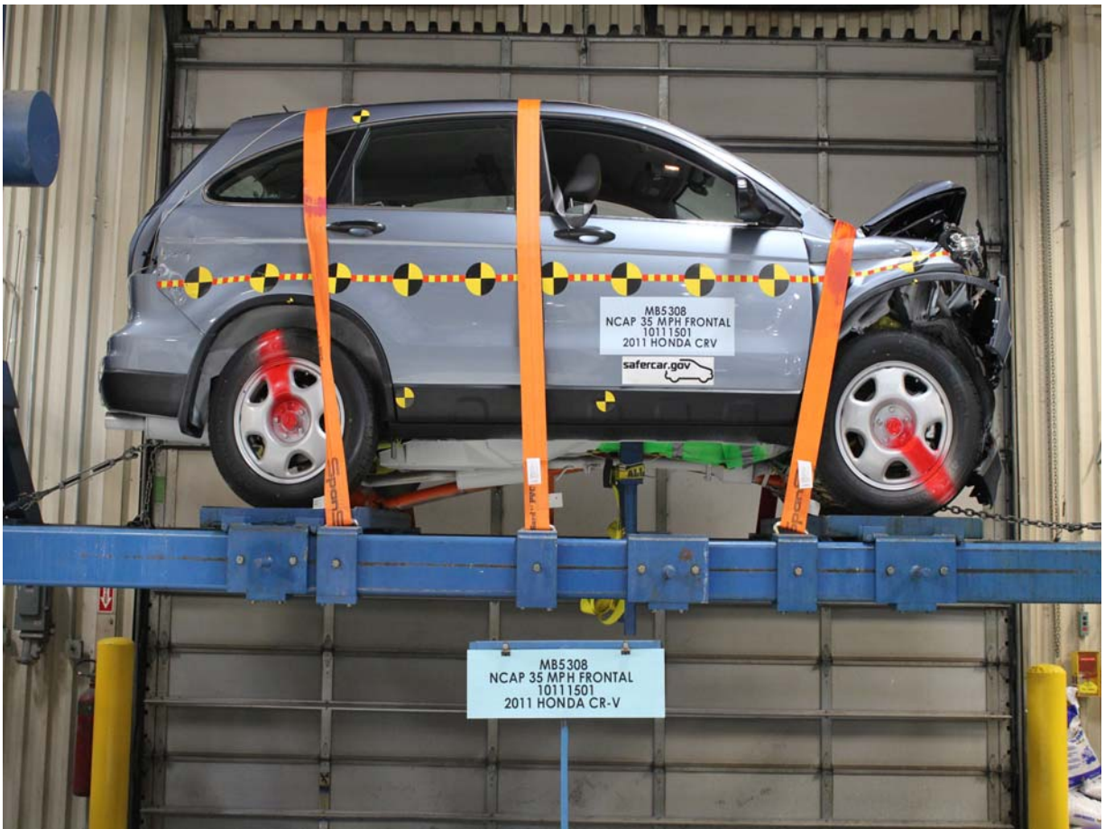
Vehicle at 360 Degrees on Static Rollover Device
