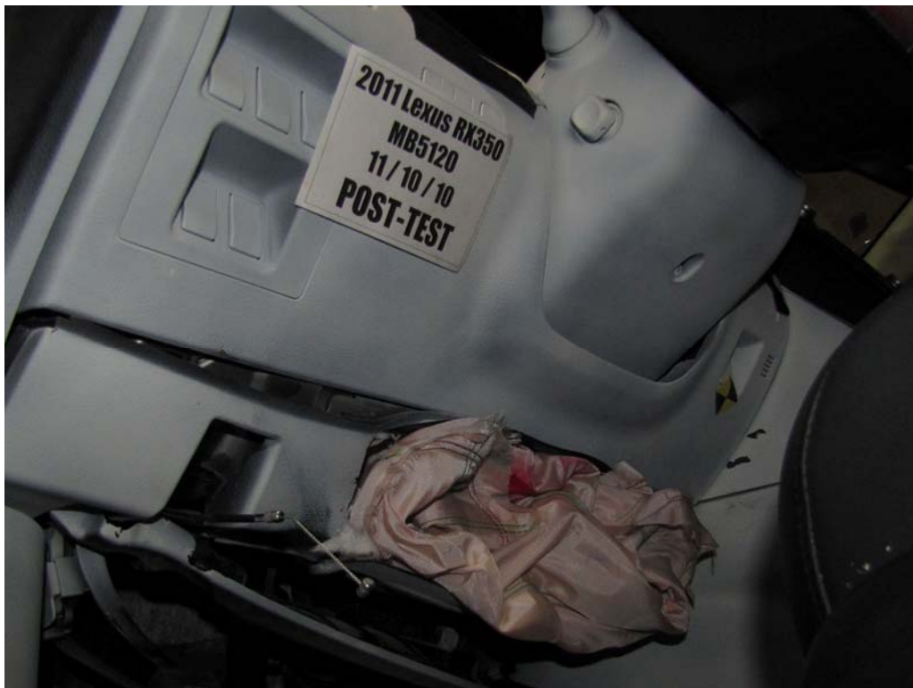
FIGURE 45. Post-Test View of Steering Column Shear Capsule
