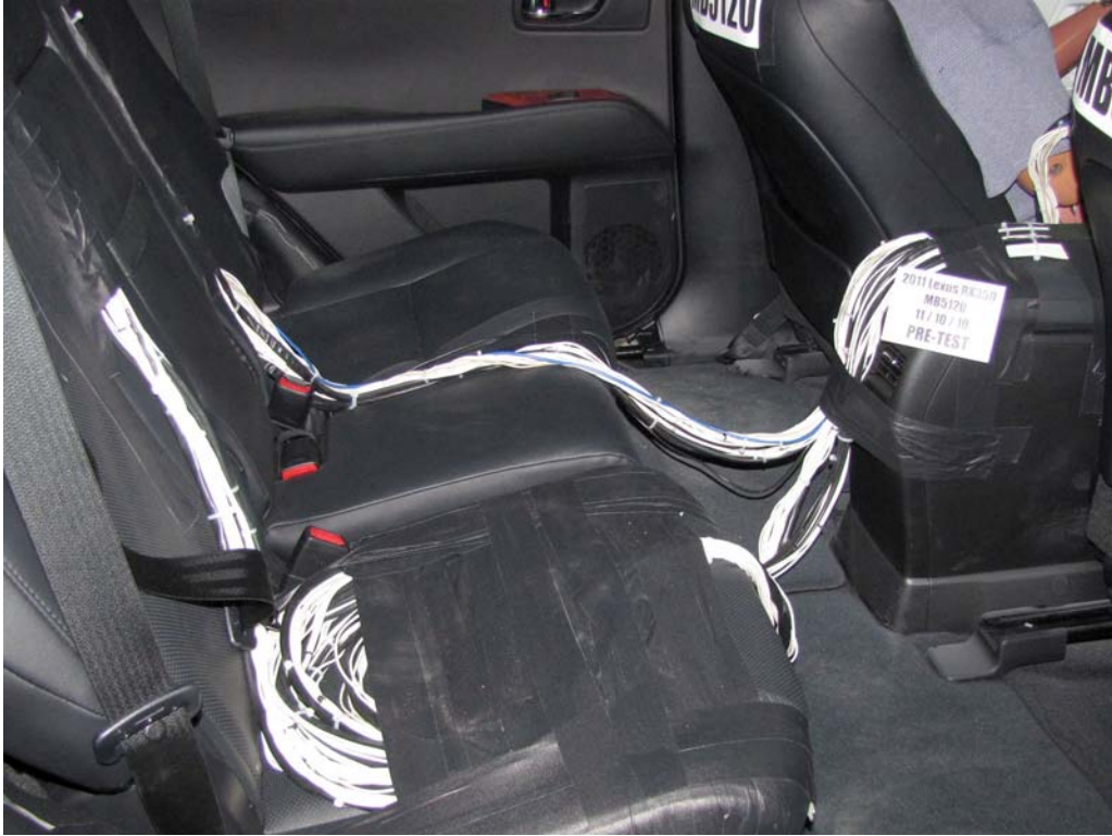
FIGURE 27. Pre-Test Dummy Cable Routing
