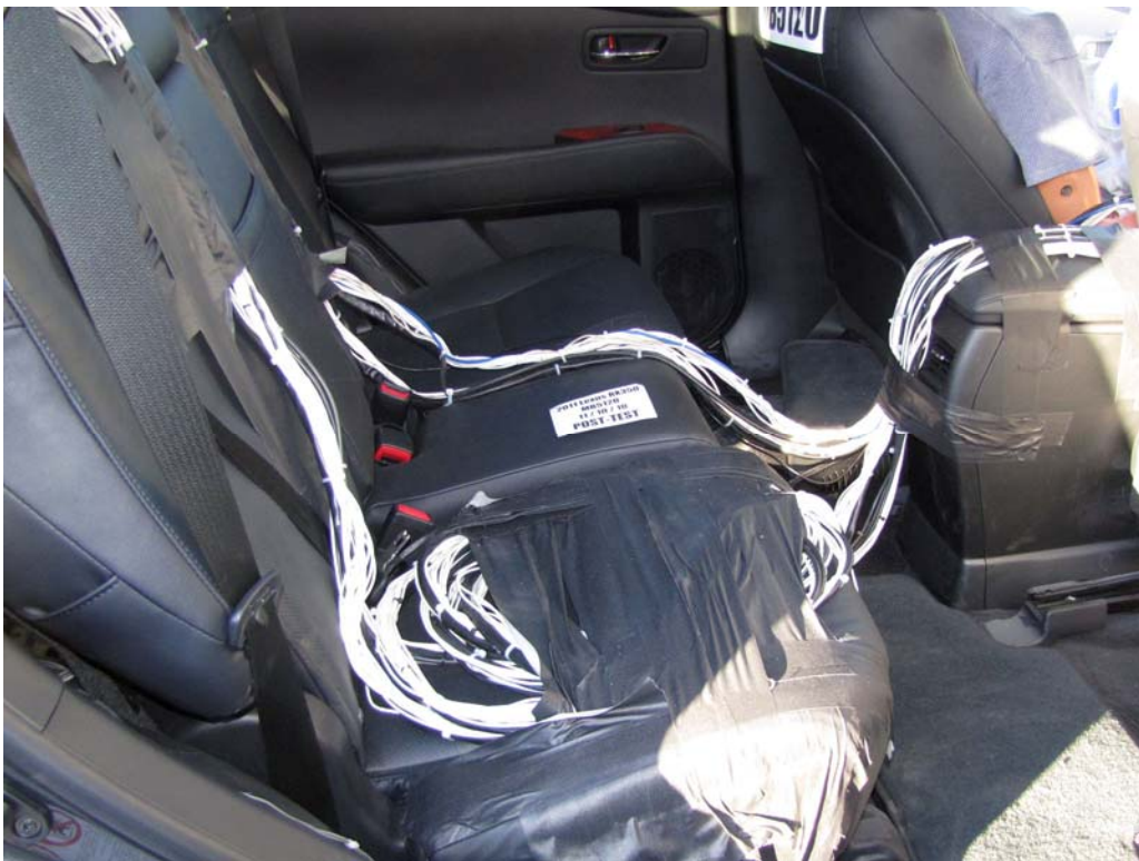
FIGURE 28. Post-Test Dummy Cable Routing
