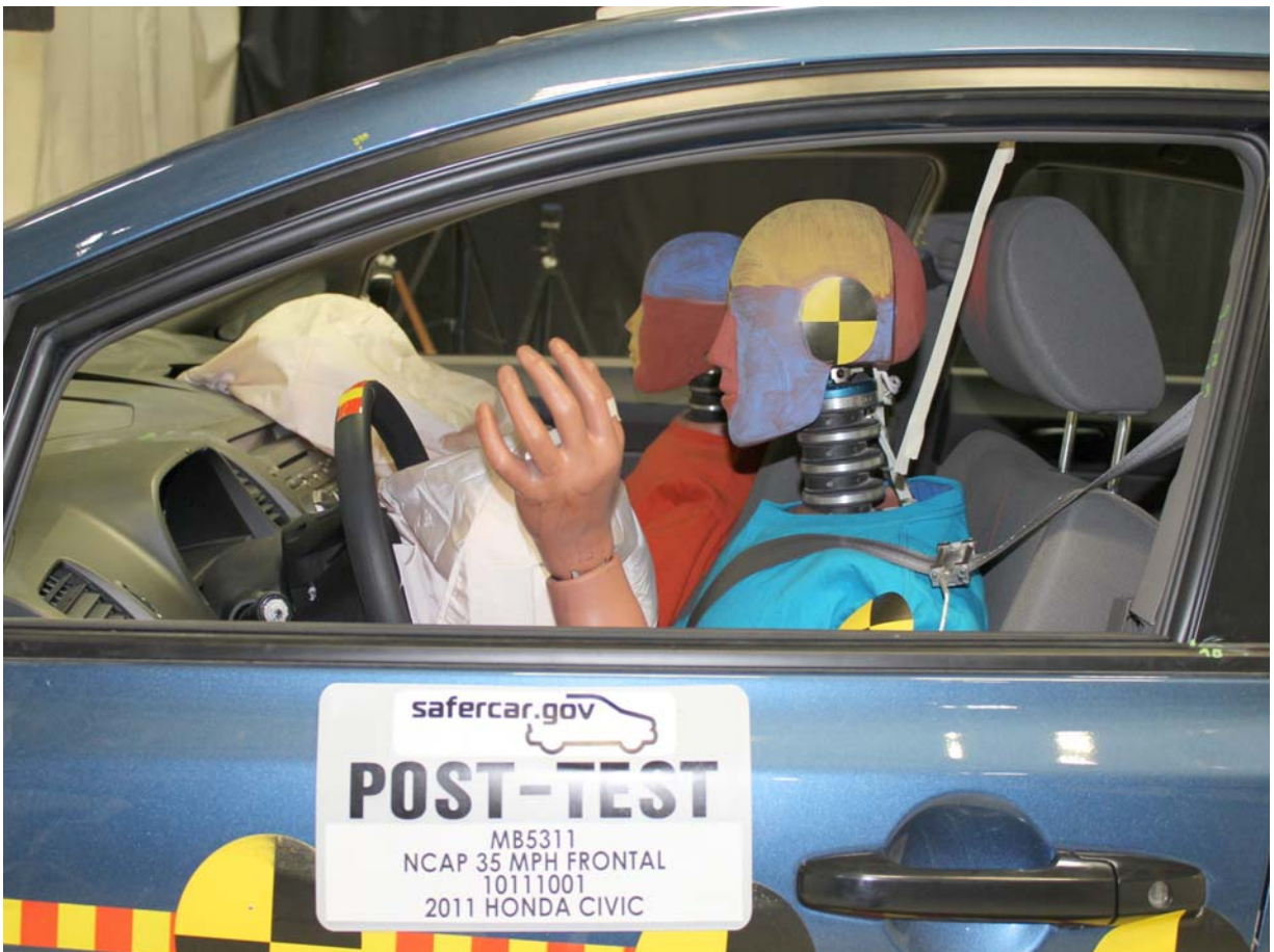
Post-Test Driver Dummy Window View
