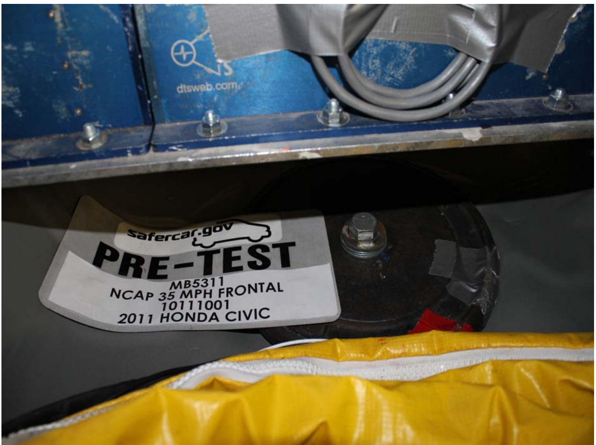
Ballast Installed in Vehicle
