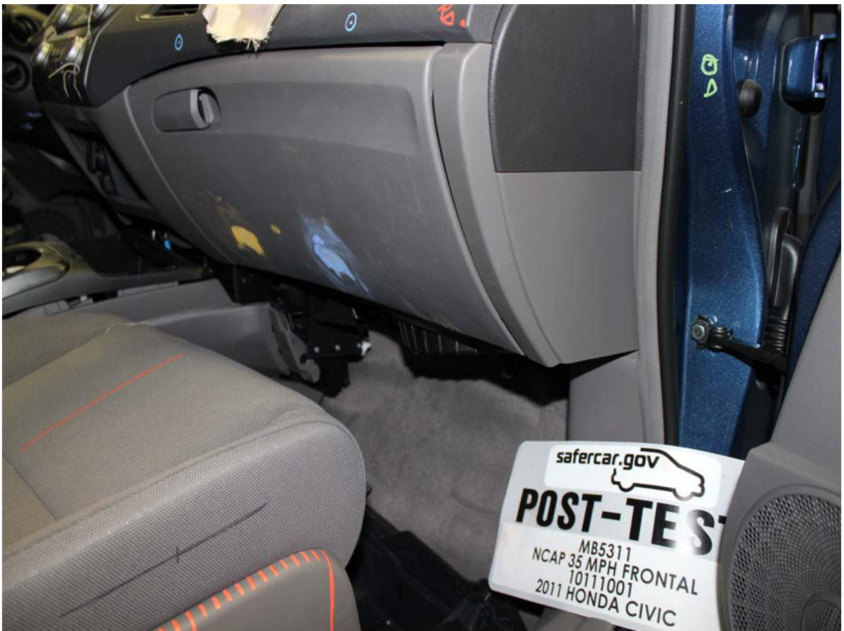
Post-Test Passenger's Side Knee Bolster (without dummy)
