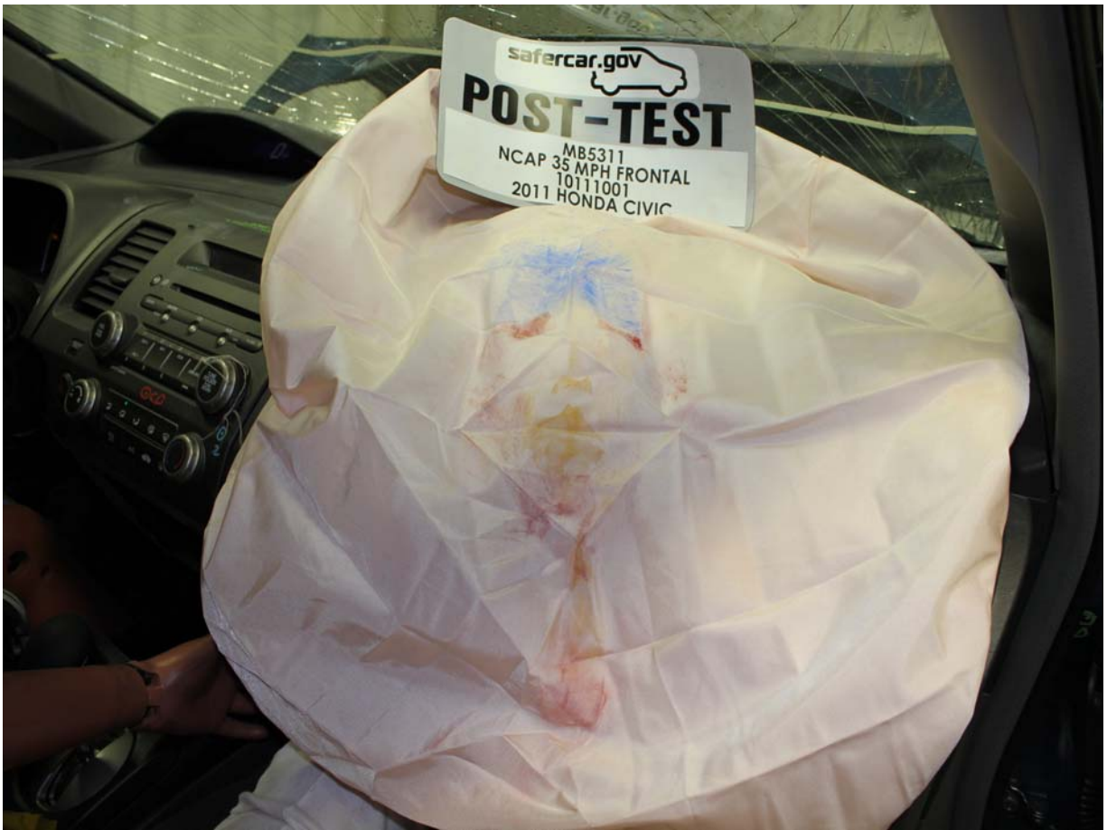
Post-Test Passenger Dummy Contact with Airbag
