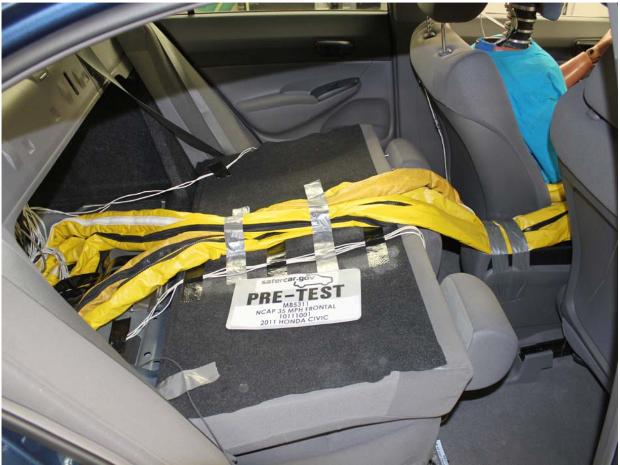
Pre-Test Dummy Cable Routing
