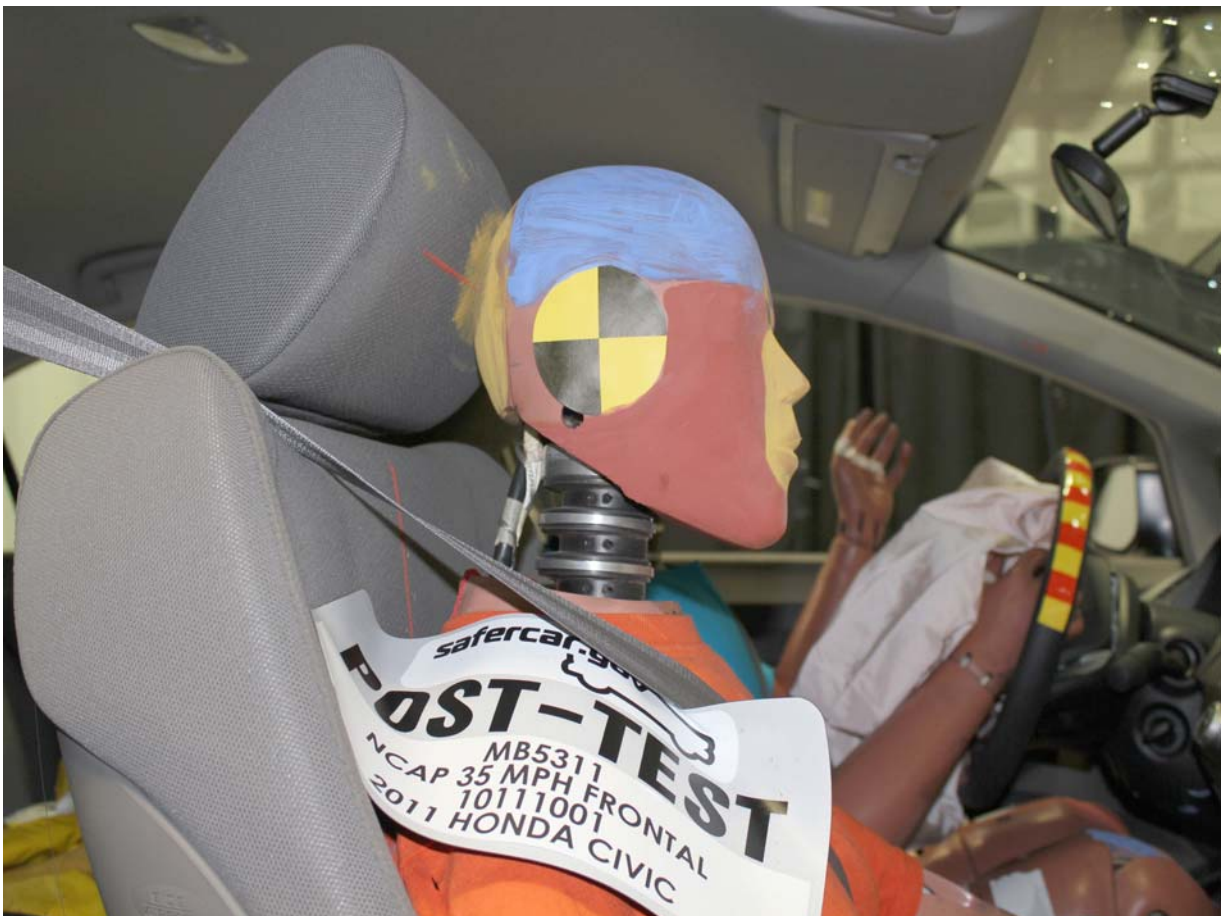
Post-Test Passenger Dummy Contact with Headrest
