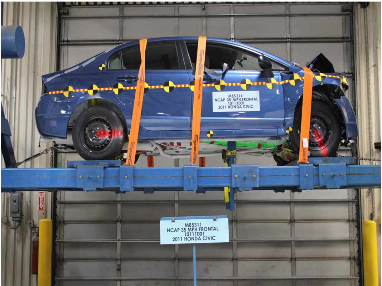
Vehicle at 360 Degrees on Static Rollover Device
