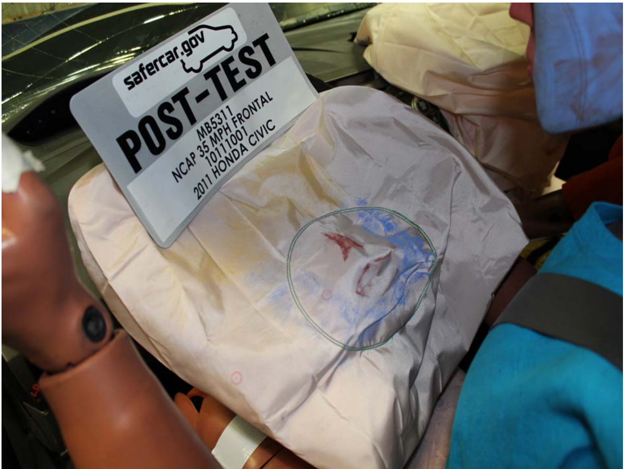
Post-Test Driver Dummy Contact with Airbag
