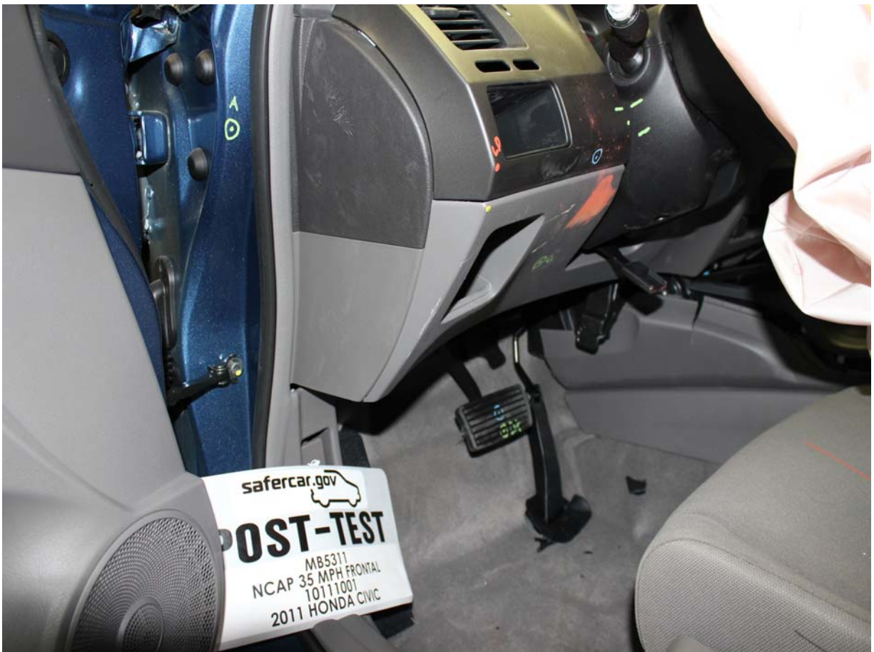
Post-Test Driver's Side Knee Bolster (without dummy)
