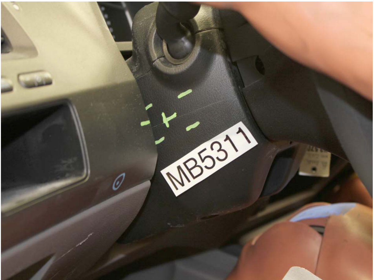
Pre-Test View of Steering Column Shear Capsule
