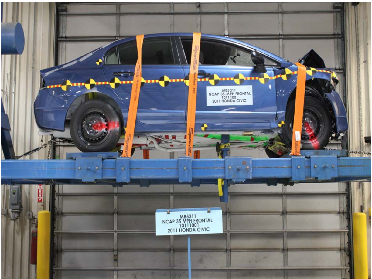
Vehicle at 0 Degrees on Static Rollover Device
