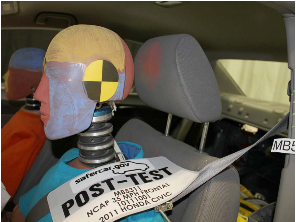
Post-Test Driver Dummy Contact with Headrest
