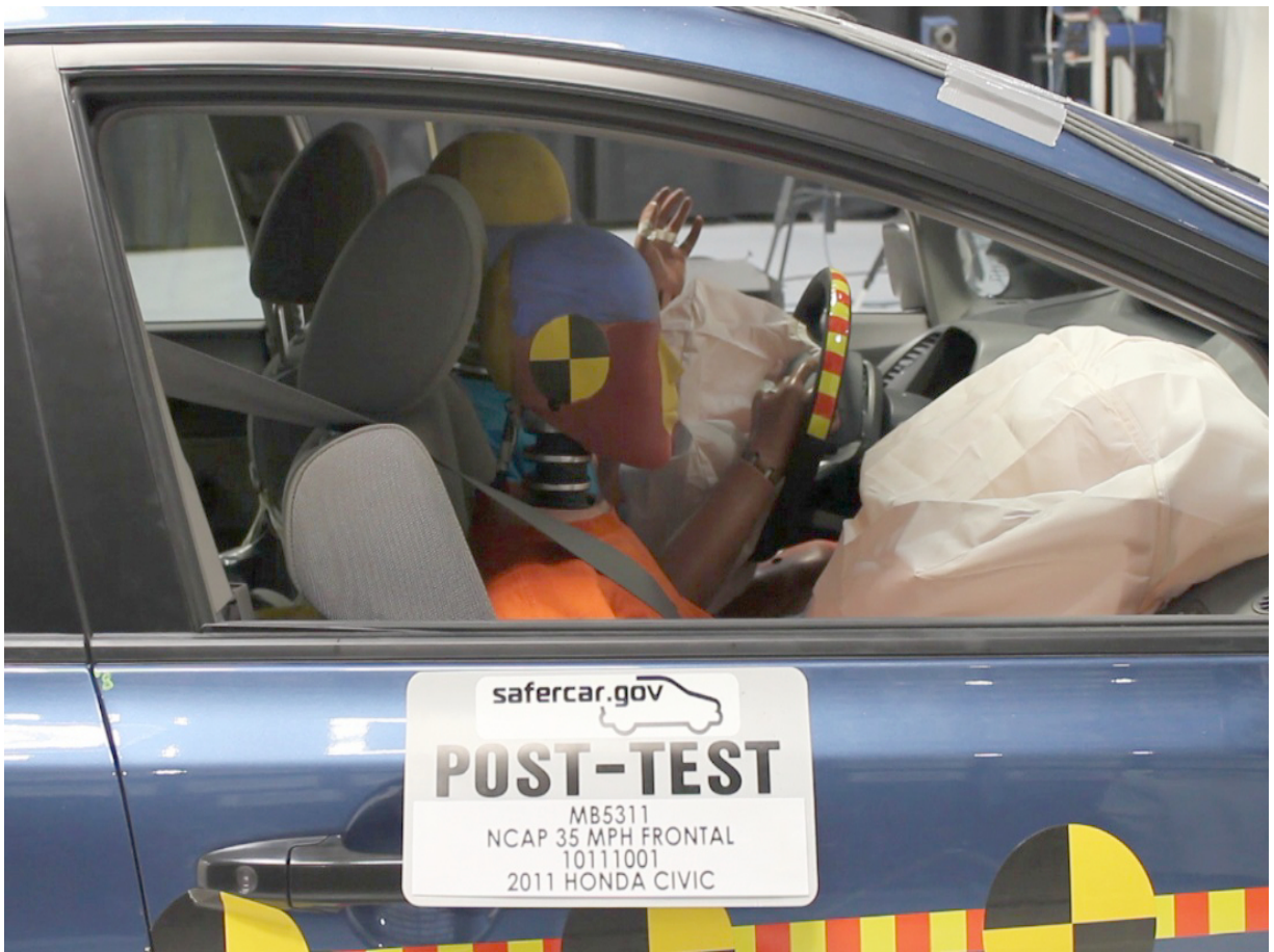
Post-Test Passenger Dummy Window View
