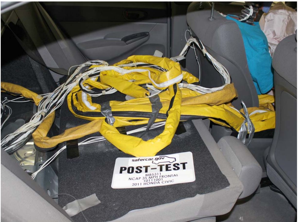
Post-Test Dummy Cable Routing
