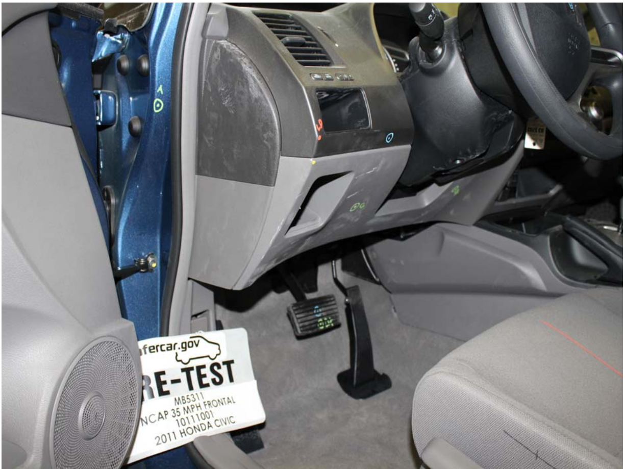
Pre-Test Driver's Side Knee Bolster (without dummy)
