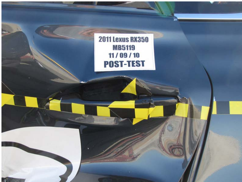
FIGURE 24. Post-Test Left Rear Door Latch Close-Up
