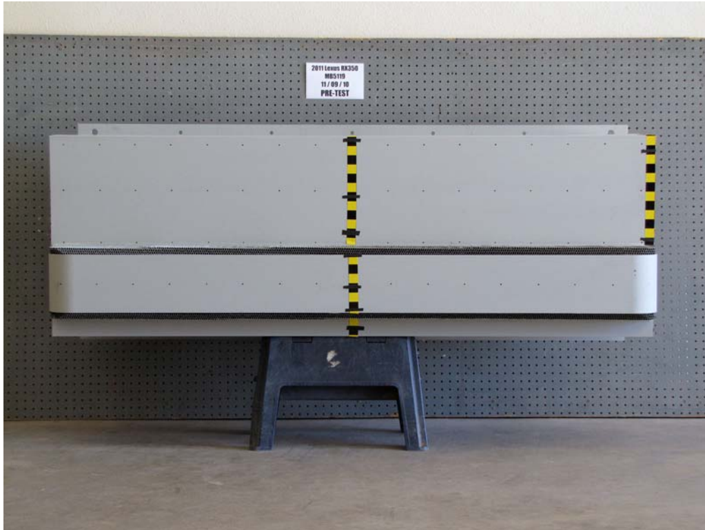
FIGURE 81. Pre-Test Front View of MDB Impactor Face
