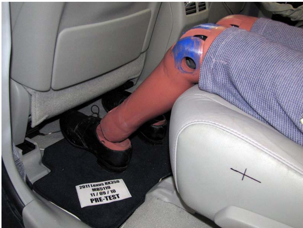
FIGURE 62. Pre-Test Placement of Rear Passenger Dummy's Feet
