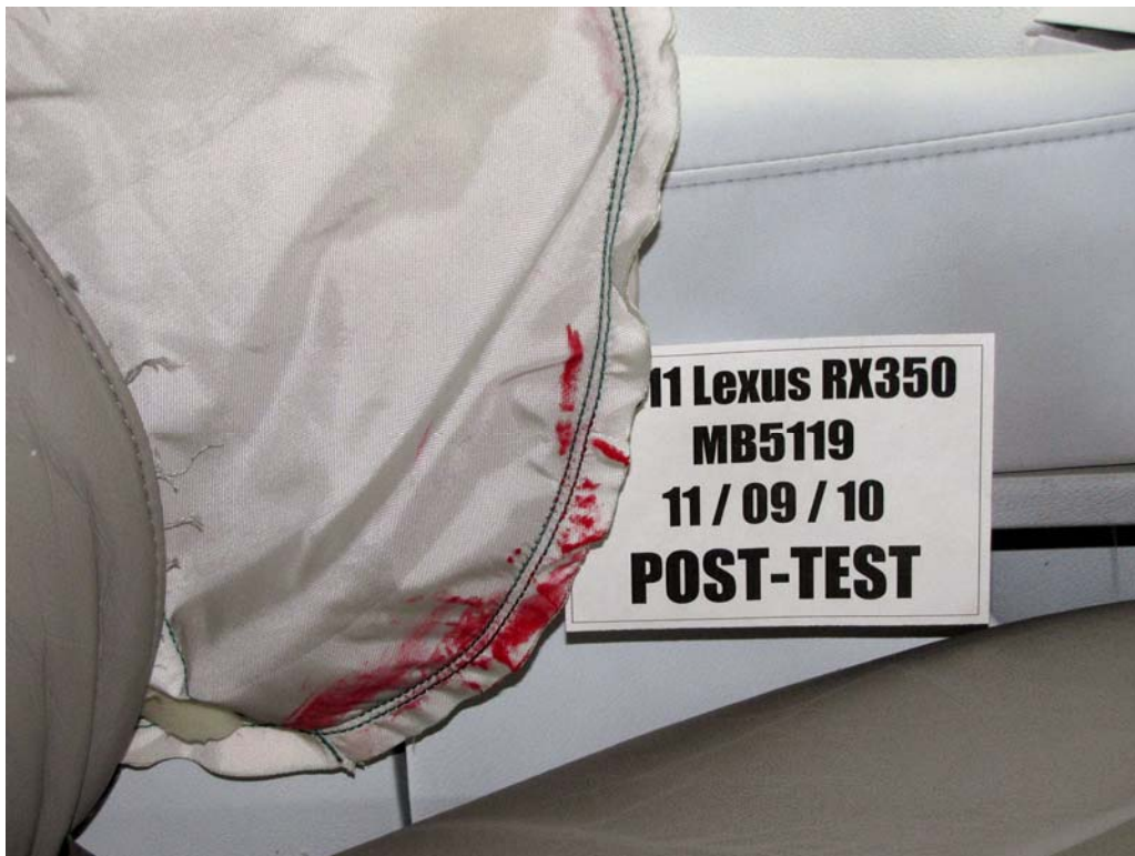
FIGURE 52. Post-Test Driver Dummy Close-Up Pelvis Contact with Side Airbag View
