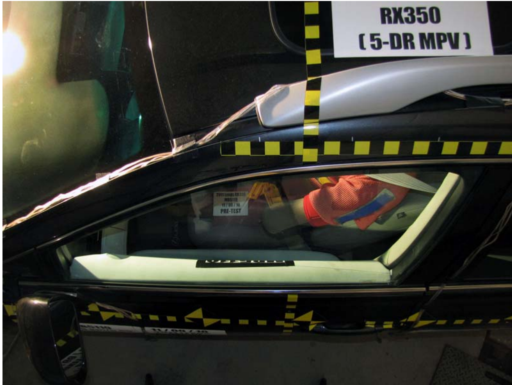
FIGURE 41. Pre-Test Driver Dummy and Door Clearance View
