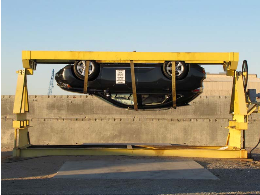
FIGURE 95. FMVSS No. 301/305 Rollover 180 Degrees
