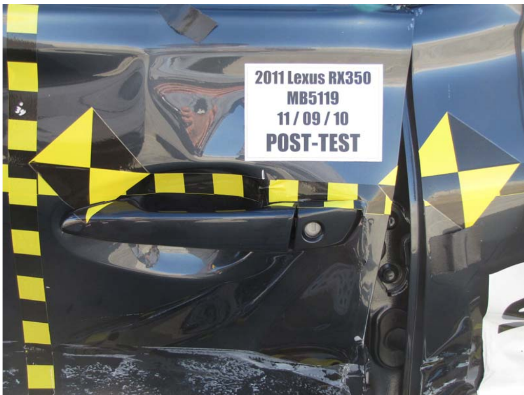
FIGURE 22. Post-Test Left Front Door Latch Close-Up
