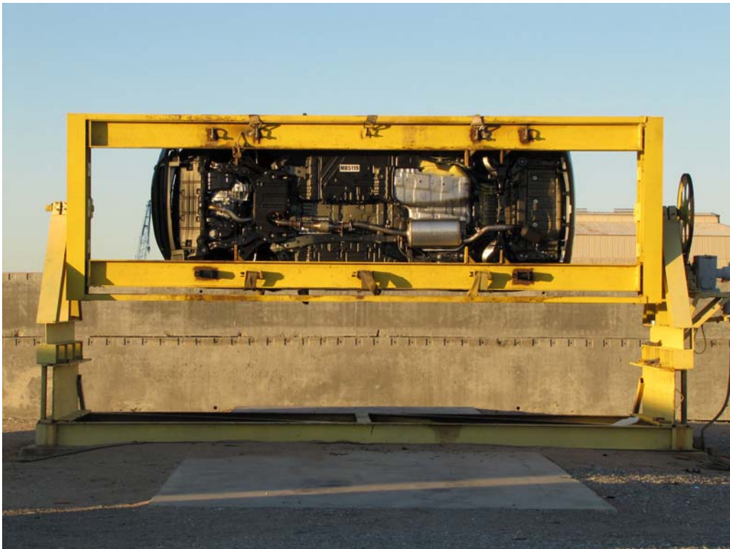
FIGURE 96. FMVSS No. 301/305 Rollover 270 Degrees
