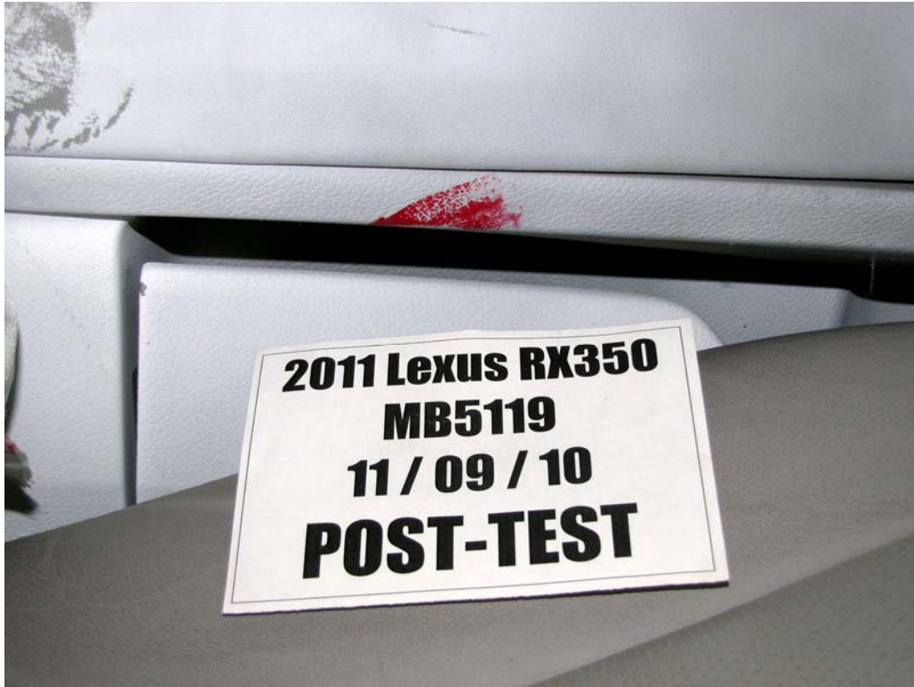
FIGURE 51. Post-Test Driver Dummy Close-Up Pelvis Contact with Vehicle Interior View
