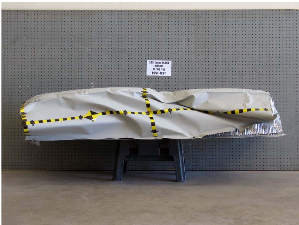
FIGURE 84. Post-Test Top View of MDB Impactor Face
