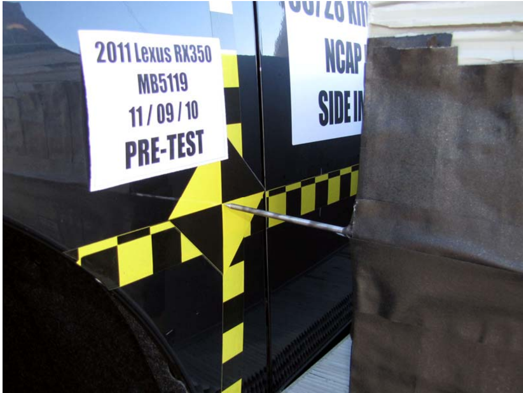
FIGURE 19. Pre-Test Close-Up View of Impact Point Target
