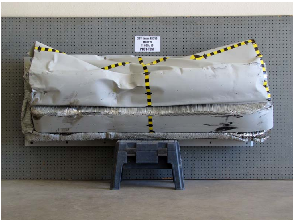
FIGURE 82. Post-Test Front View of MDB Impactor Face
