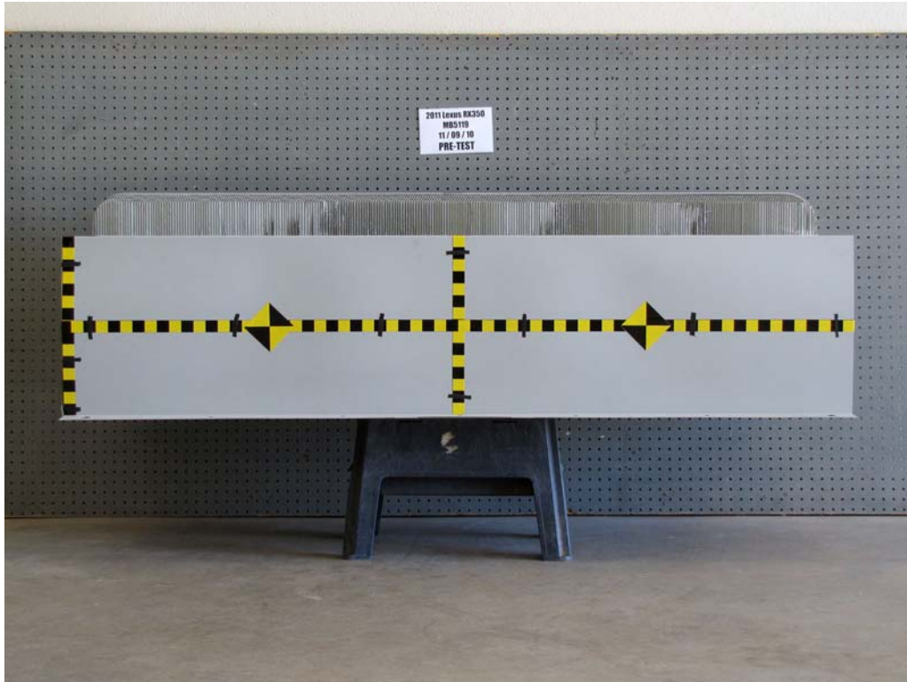
FIGURE 83. Pre-Test Top View of MDB Impactor Face
