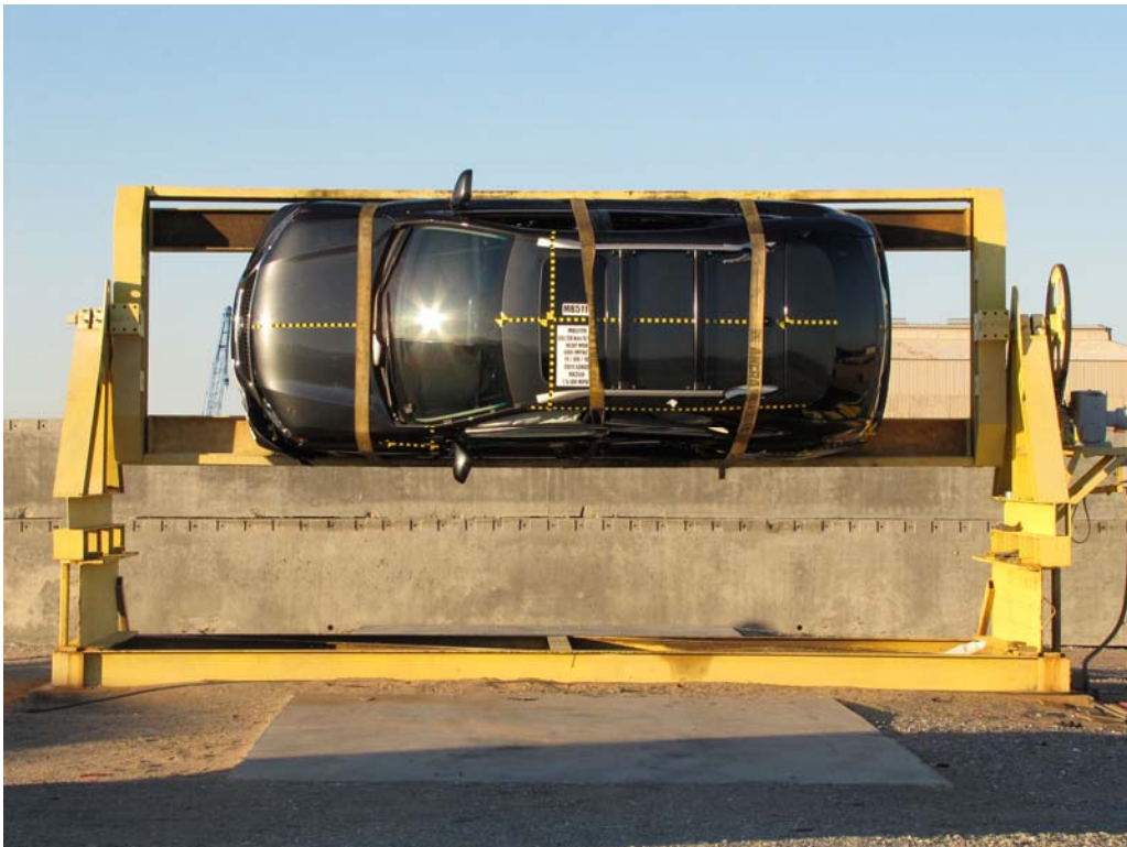
FIGURE 94. FMVSS No. 301/305 Rollover 90 Degrees
