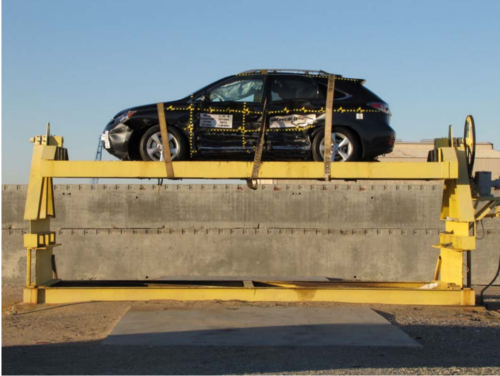
FIGURE 93. FMVSS No. 301/305 Rollover 0 Degrees
