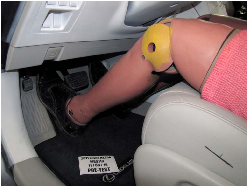
FIGURE 34. Pre-Test Placement of Driver Dummy's Feet
