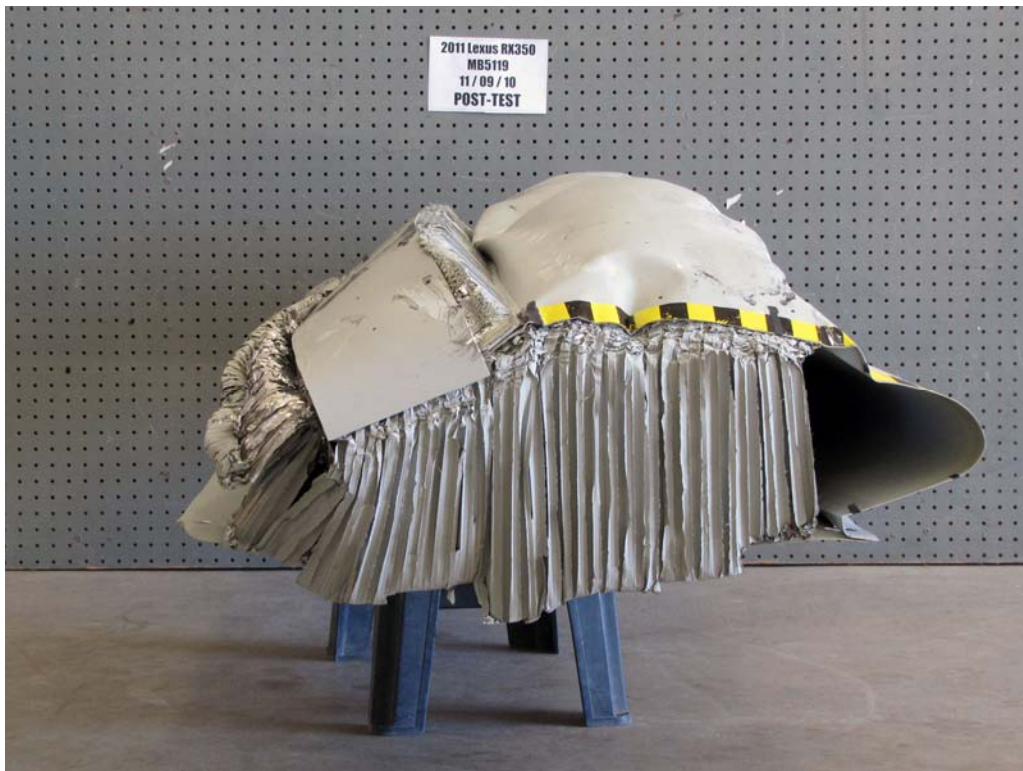
FIGURE 86. Post-Test Left Side View of MDB Impactor Face
