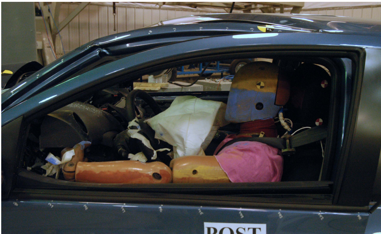
Figure A-36: Post test driver through window
