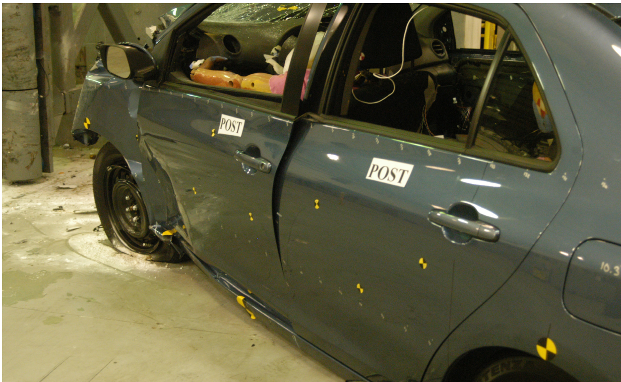
Figure A-24: Post test rear left 3/4 side view of left side doors
