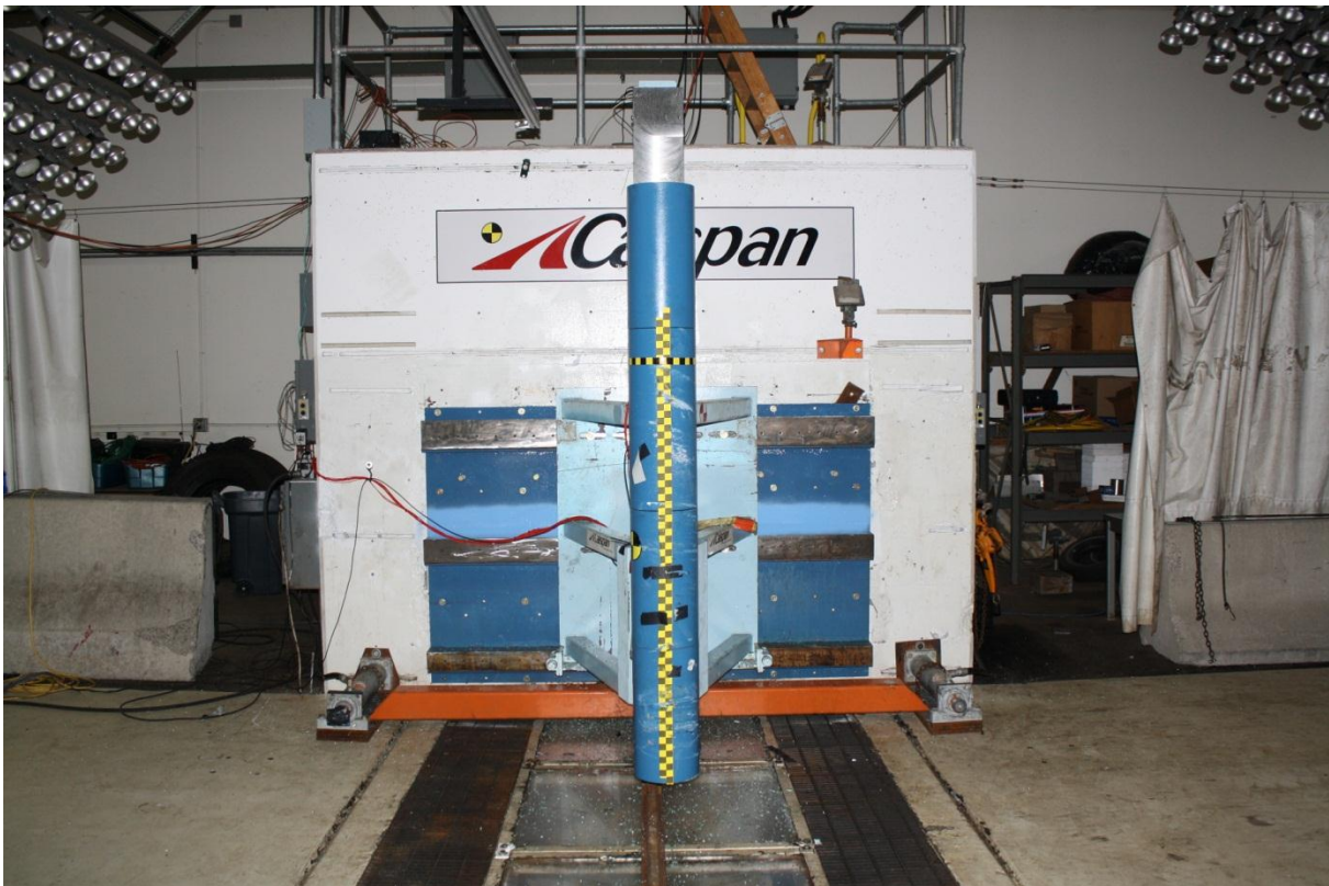
Figure A-56: Post-Test Pole Barrier Front View
