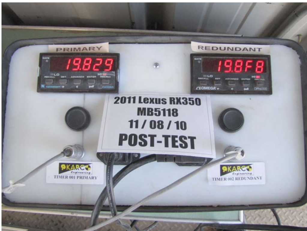
FIGURE 60. Post-Test Primary and Redundant Speed Trap Read-Out
