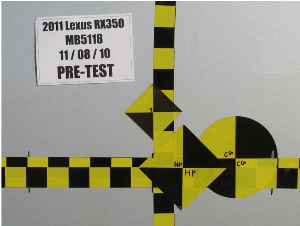
FIGURE 19. Pre-Test Close-Up View of Impact Point Target
