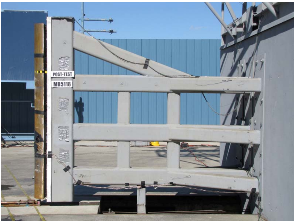
FIGURE 58. Post-Test Pole Barrier Side View
