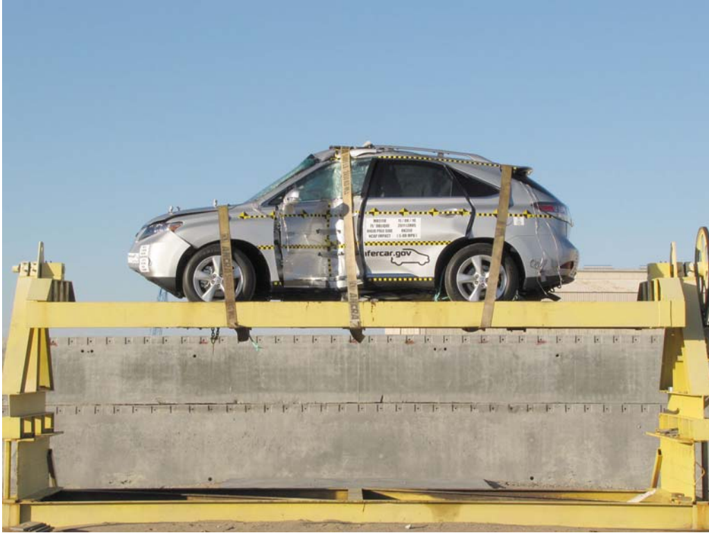
FIGURE 61. FMVSS No. 301-305 Rollover 0 Degrees
