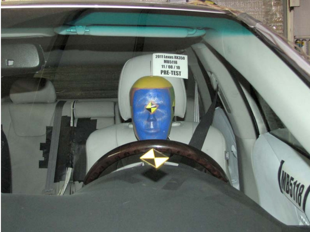
FIGURE 21. Pre-Test Front Close-Up View of Dummy
