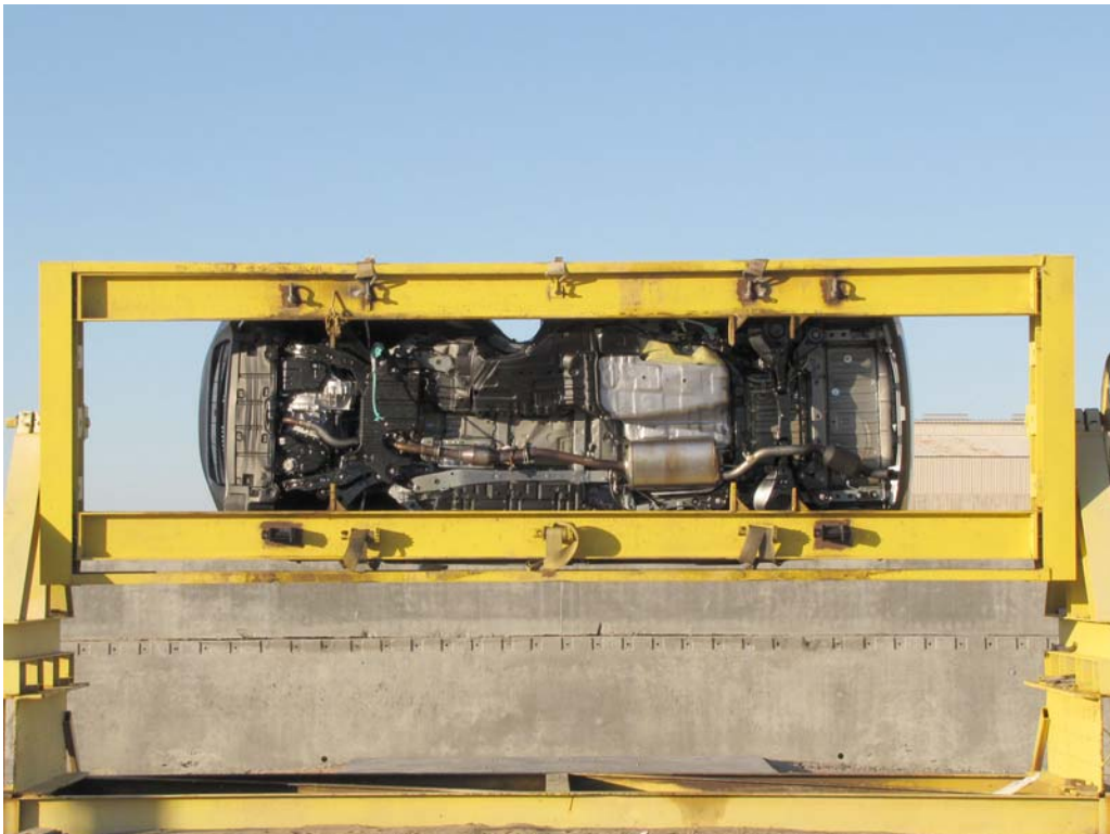
FIGURE 64. FMVSS No. 301-305 Rollover 270 Degrees
