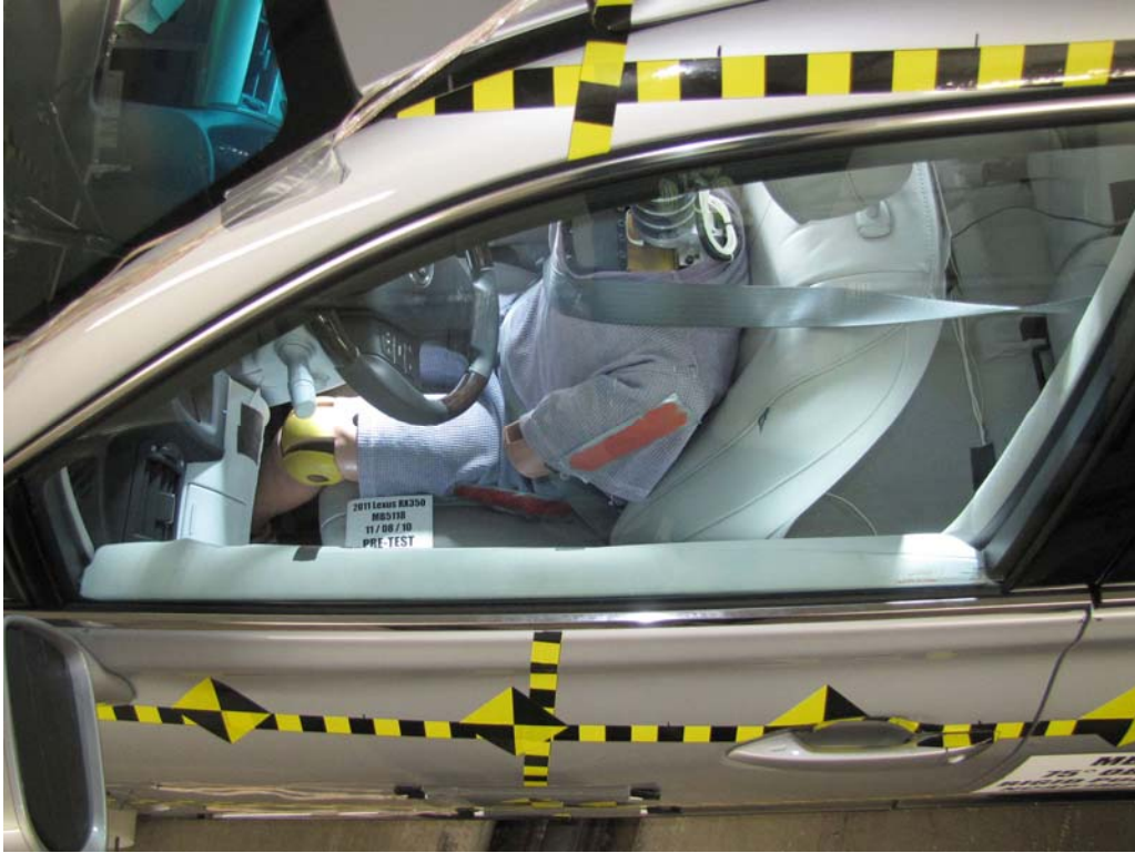
FIGURE 39. Pre-Test Driver Dummy and Door Clearance
