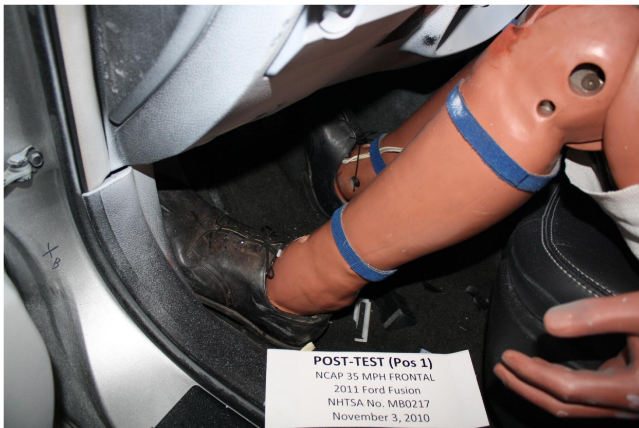
Figure A-38: Post-Test Driver Dummy Feet
