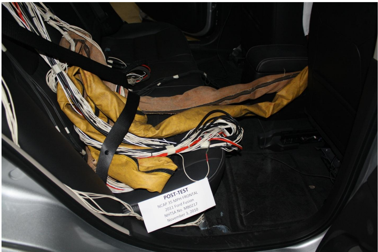
Figure A-28: Post-Test Dummy Cable Routing
