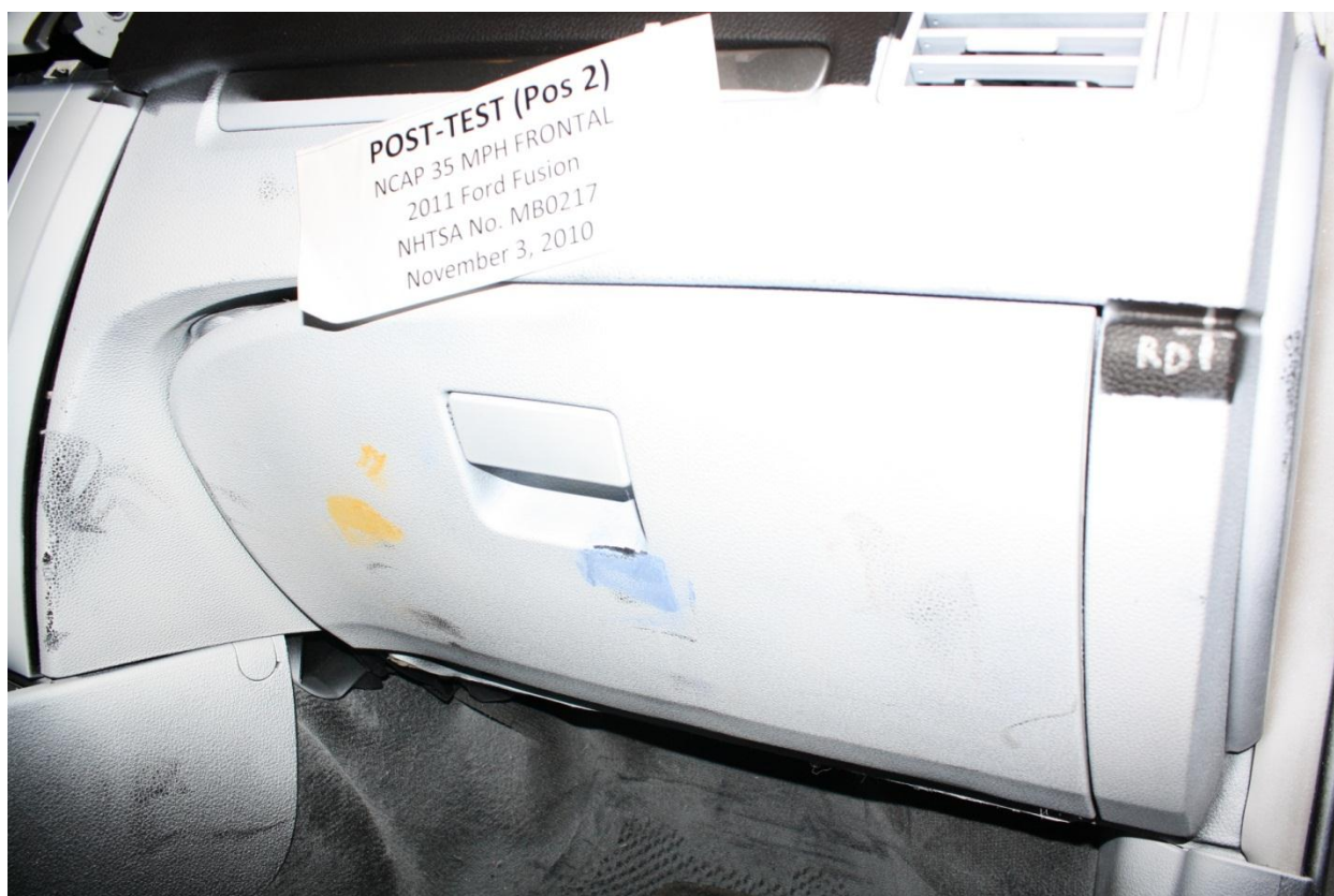
Figure A-57: Post-Test Passenger's Side Knee Bolster
