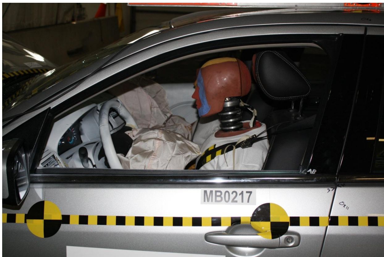
Figure A-32: Post-Test Driver Dummy Window View
