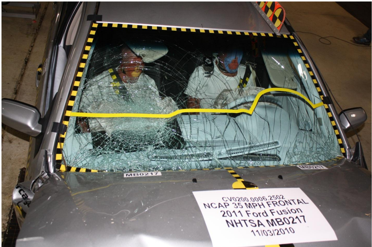
Figure A-18: Post-Test Windshield View
