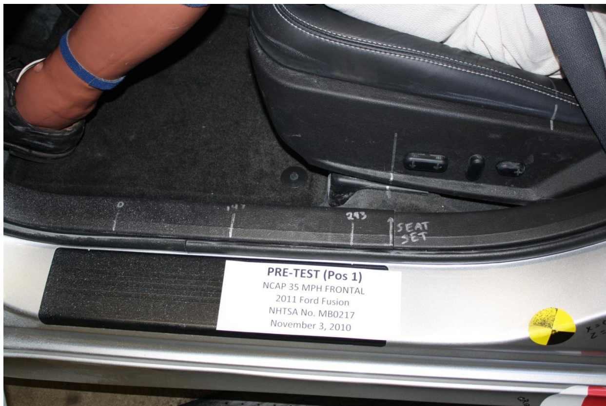
Figure A-35: Pre-Test Driver's Seat Fore-Aft Markings
