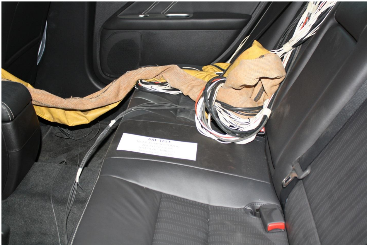
Figure A-27: Pre-Test Dummy Cable Routing
