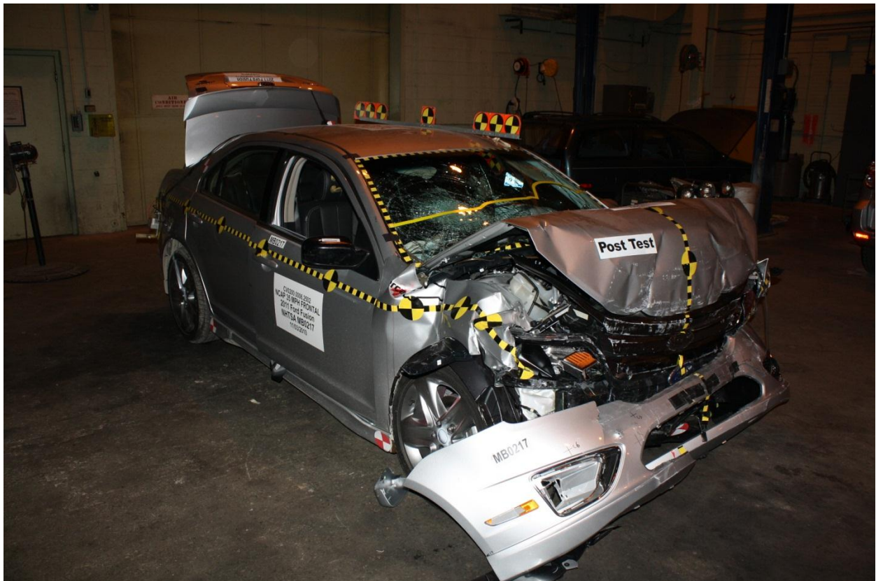
Figure A-14: Post-Test Right \frac{3}{4} View
