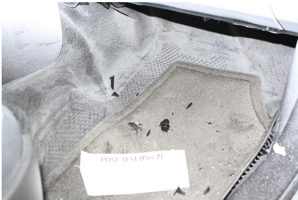
Figure A-59: Post-Test Passenger's Floorpan
