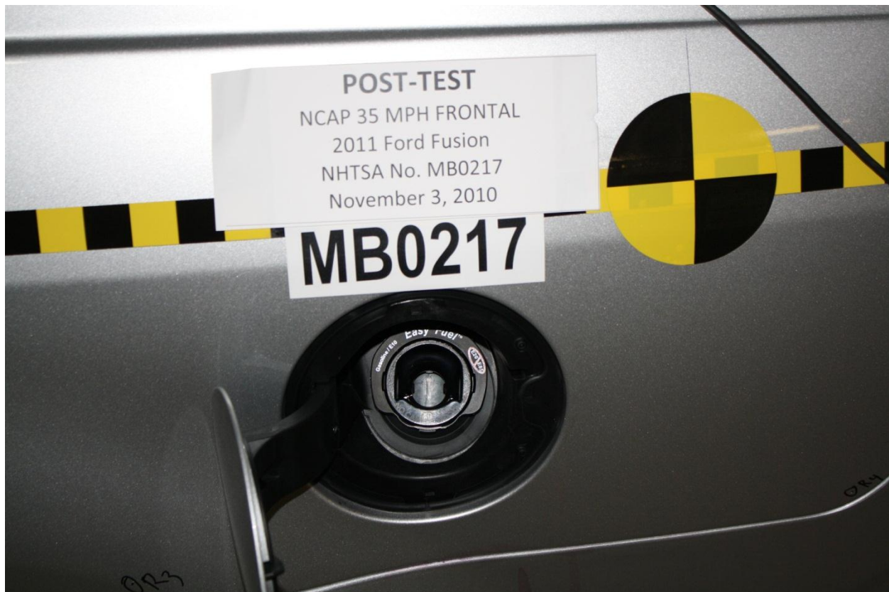
Figure A-22: Post-Test Fuel Filler Cap View
