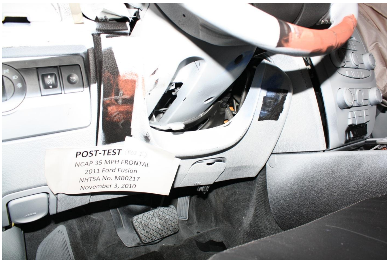
Figure A-40: Post-Test Driver's Side Knee Bolster
