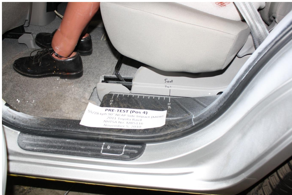
Figure A-64: Pre-test Close-Up Left Side View of Rear Passenger Seat Track Showing Test Position
