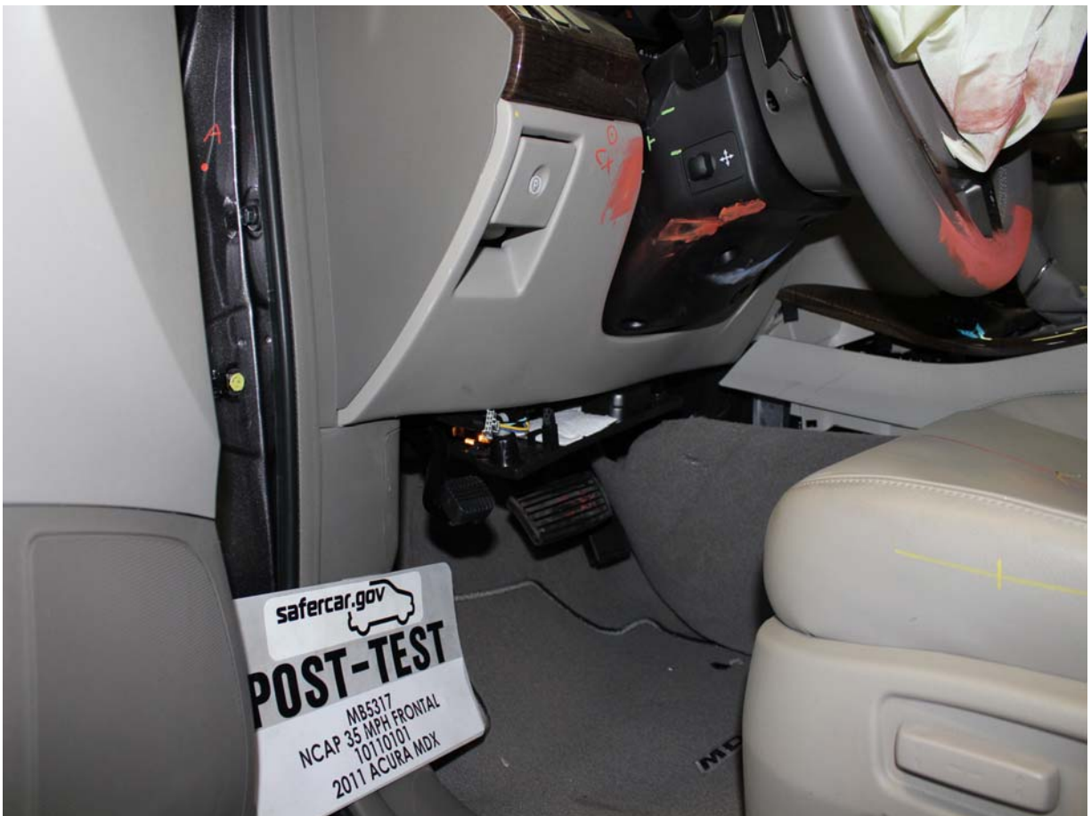
Post-Test Driver Dummy Contact with Knee Bolster
