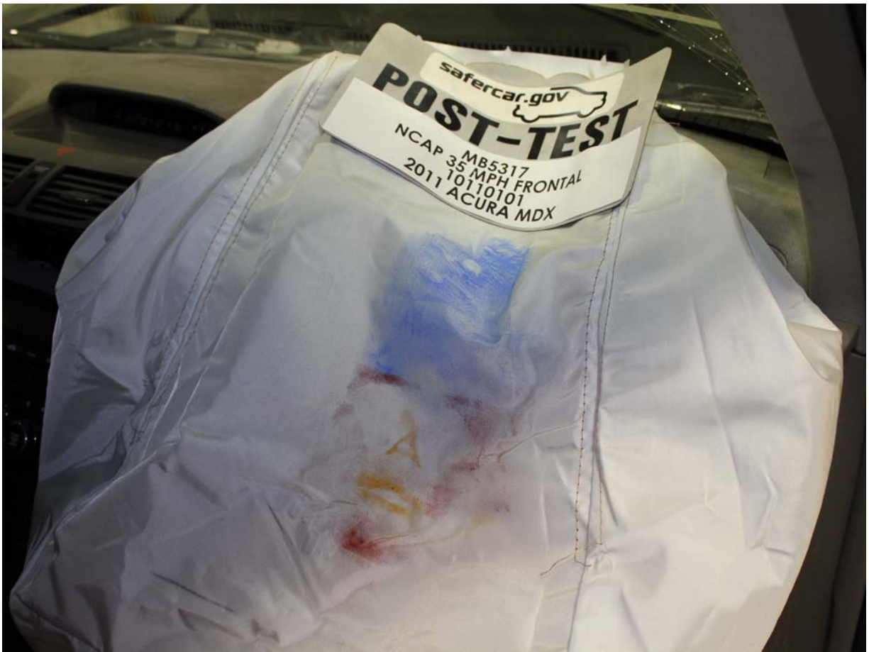
Post-Test Passenger Dummy Contact with Airbag
