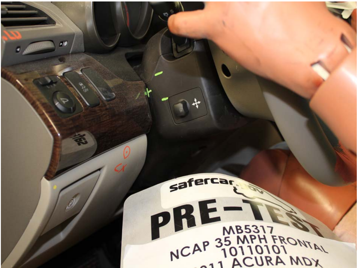
Pre-Test View of Steering Column Shear Capsule
