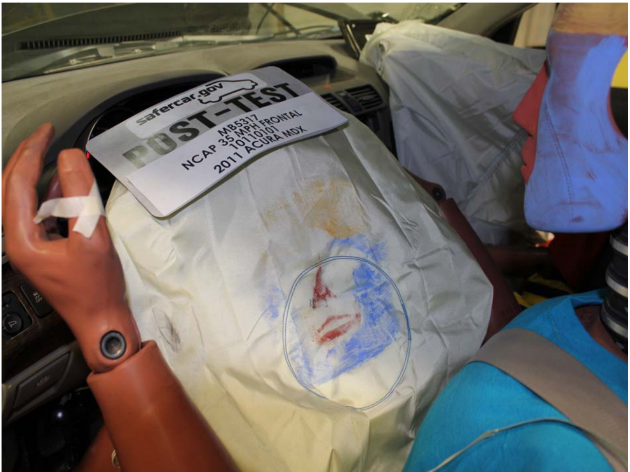
Post-Test Driver Dummy Contact with Airbag
