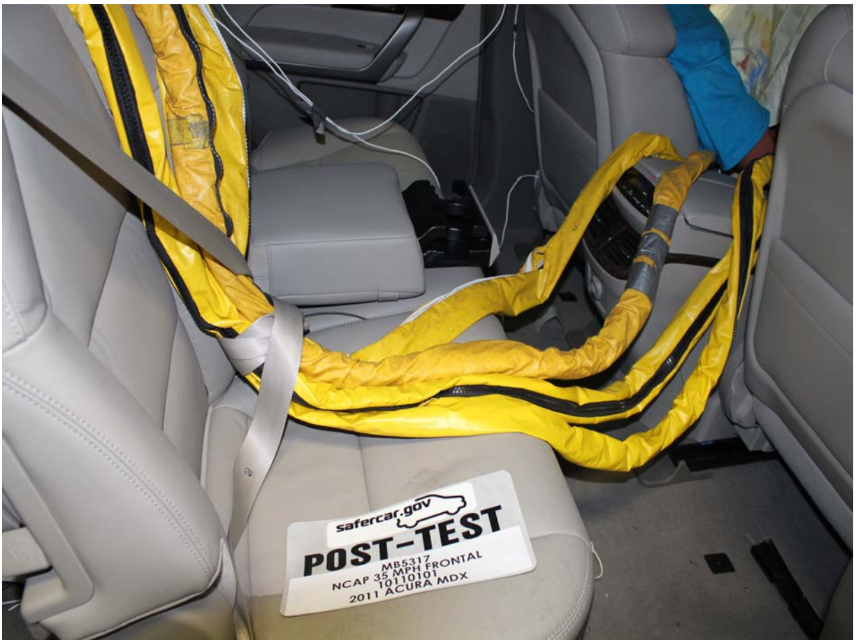
Post-Test Dummy Cable Routing
