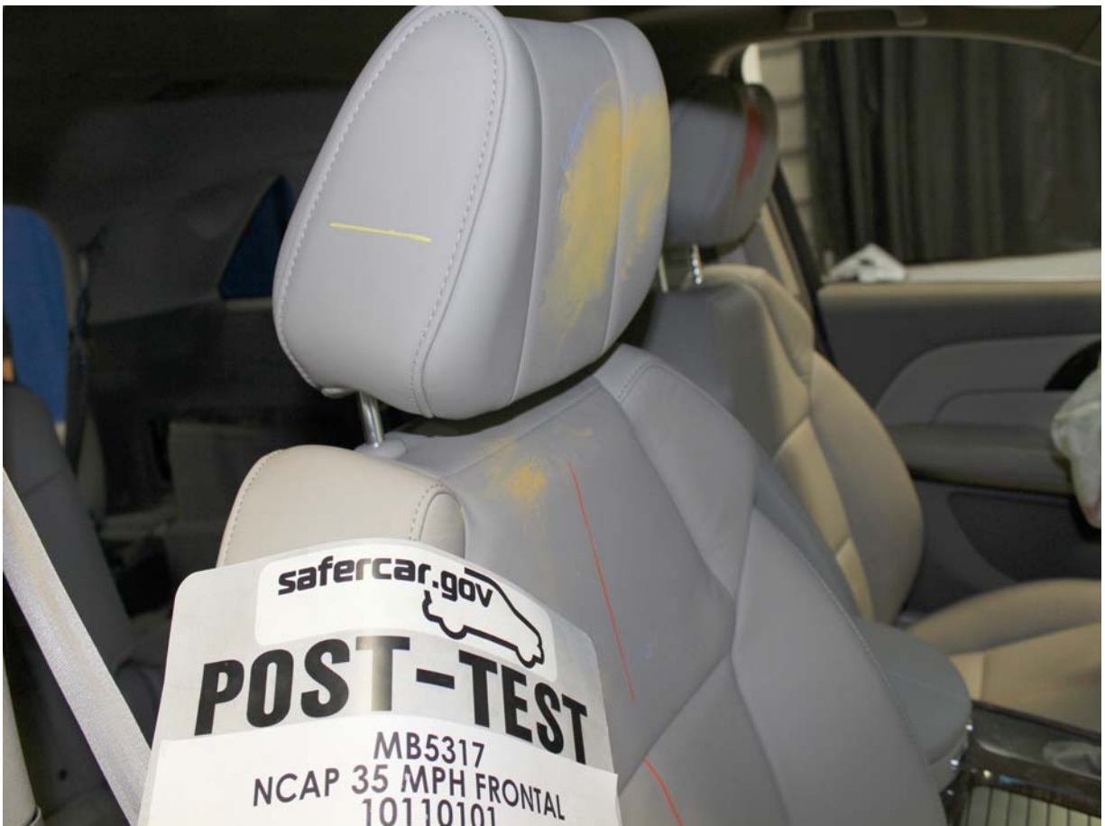
Post-Test Passenger Dummy Contact with Headrest
