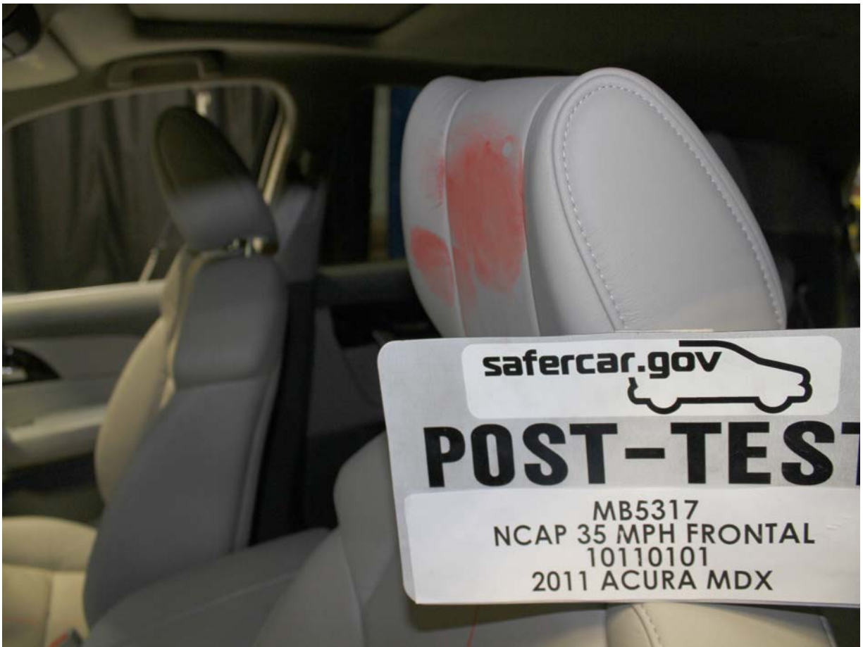
Post-Test Driver Dummy Contact with Headrest
