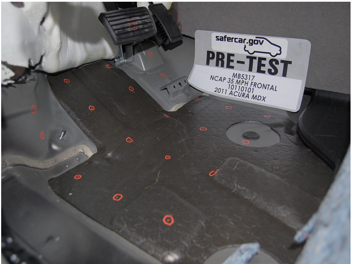
Pre-Test Driver's Side Floorpan
