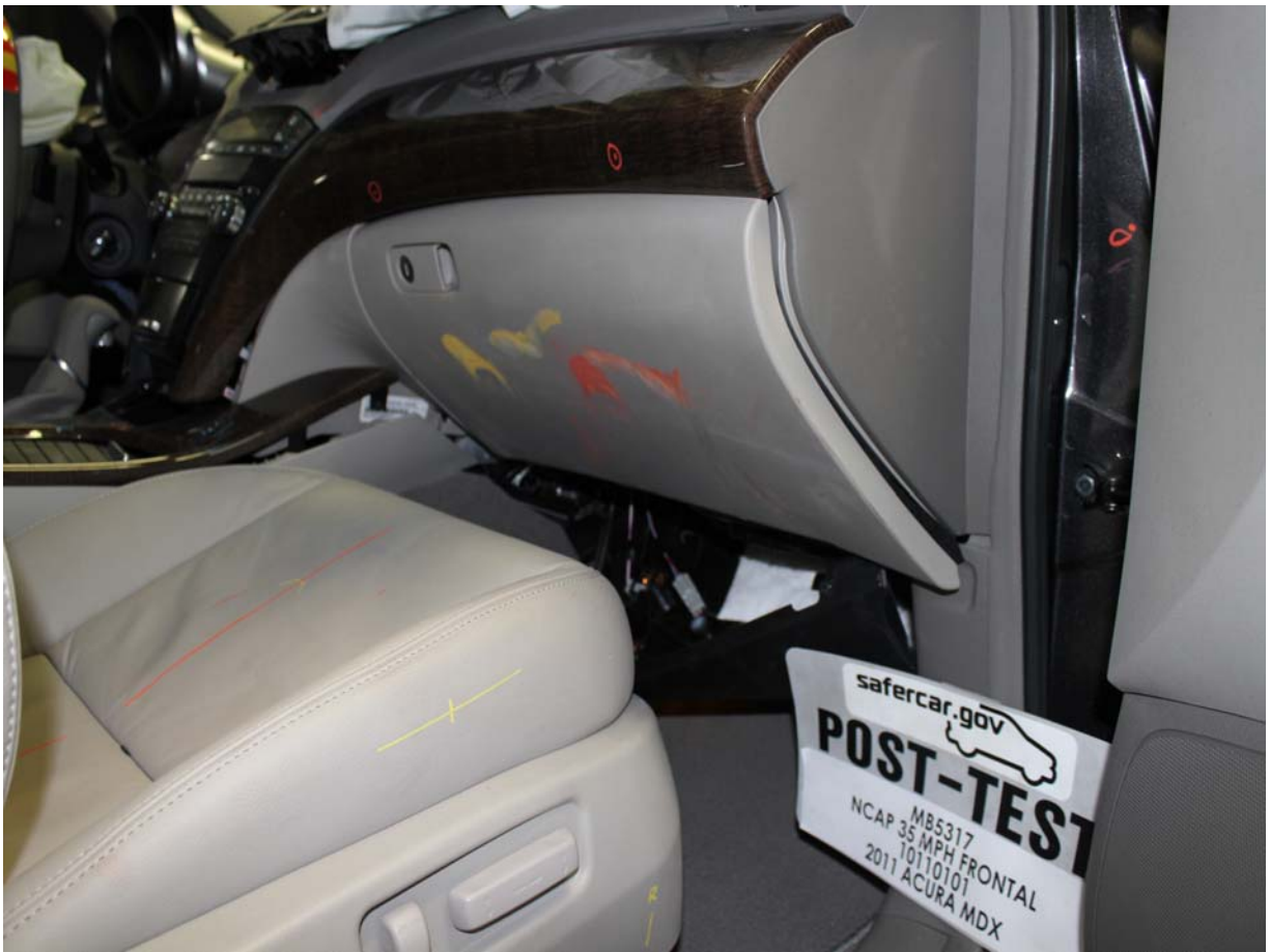
Post-Test Passenger Dummy Contact with Glovebox
