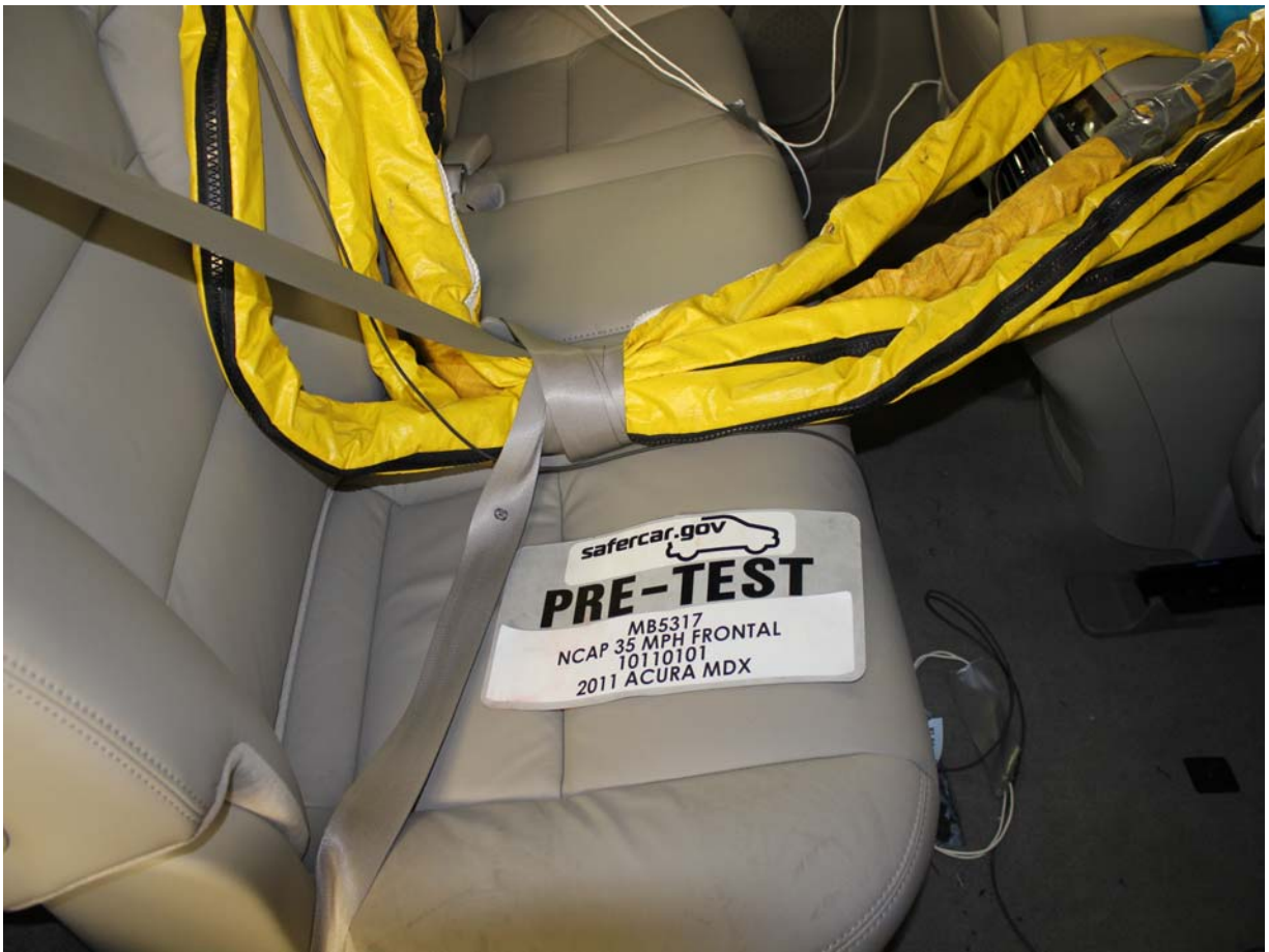
Pre-Test Dummy Cable Routing
