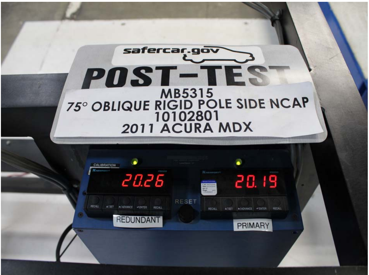
Post-Test Primary and Redundant Speed Trap Read-Out
