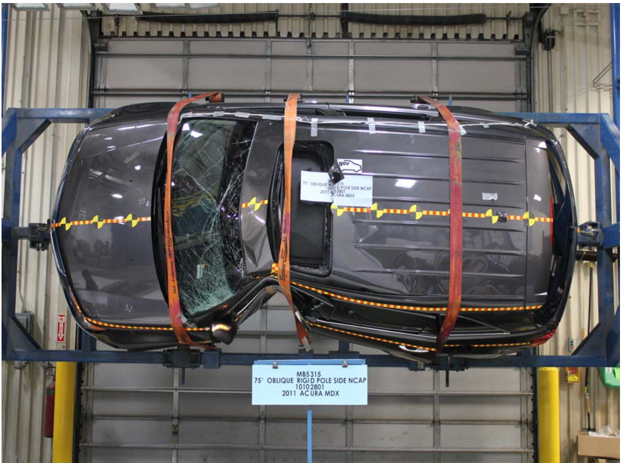
FMVSS No. 301/305 Rollover 90 Degrees
