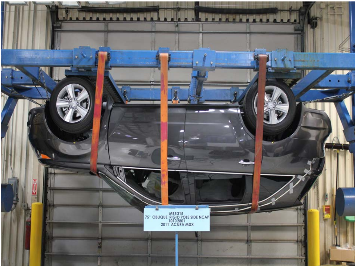
FMVSS No. 301/305 Rollover 180 Degrees
