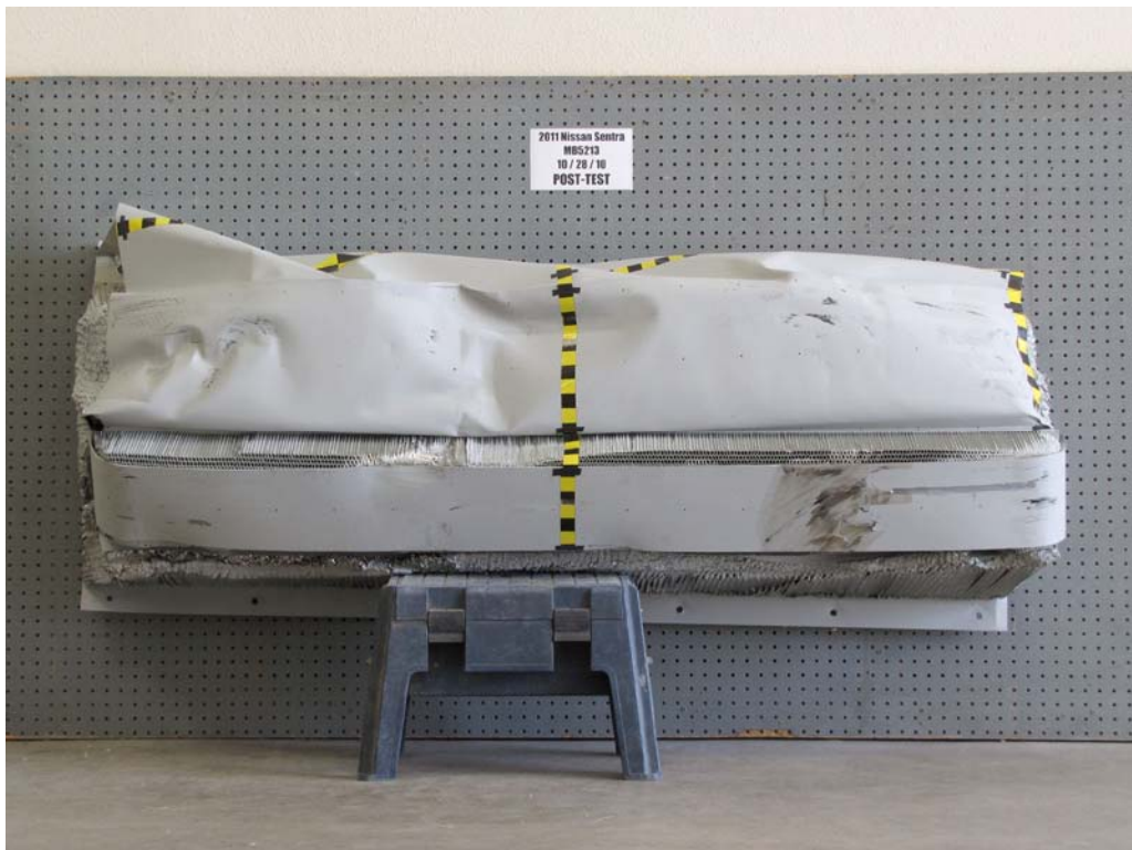
FIGURE 82. Post-Test Front View of MDB Impactor Face
