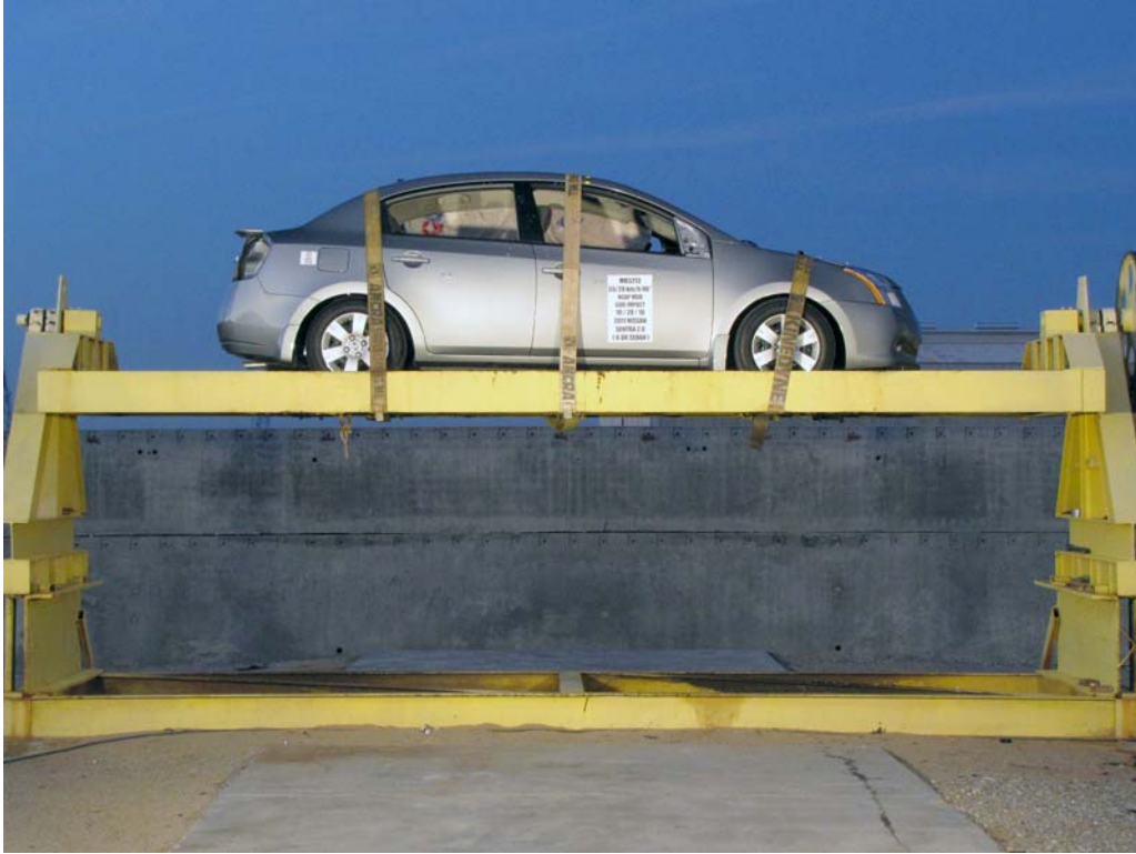
FIGURE 93. FMVSS No. 301/305 Rollover 0 Degrees
