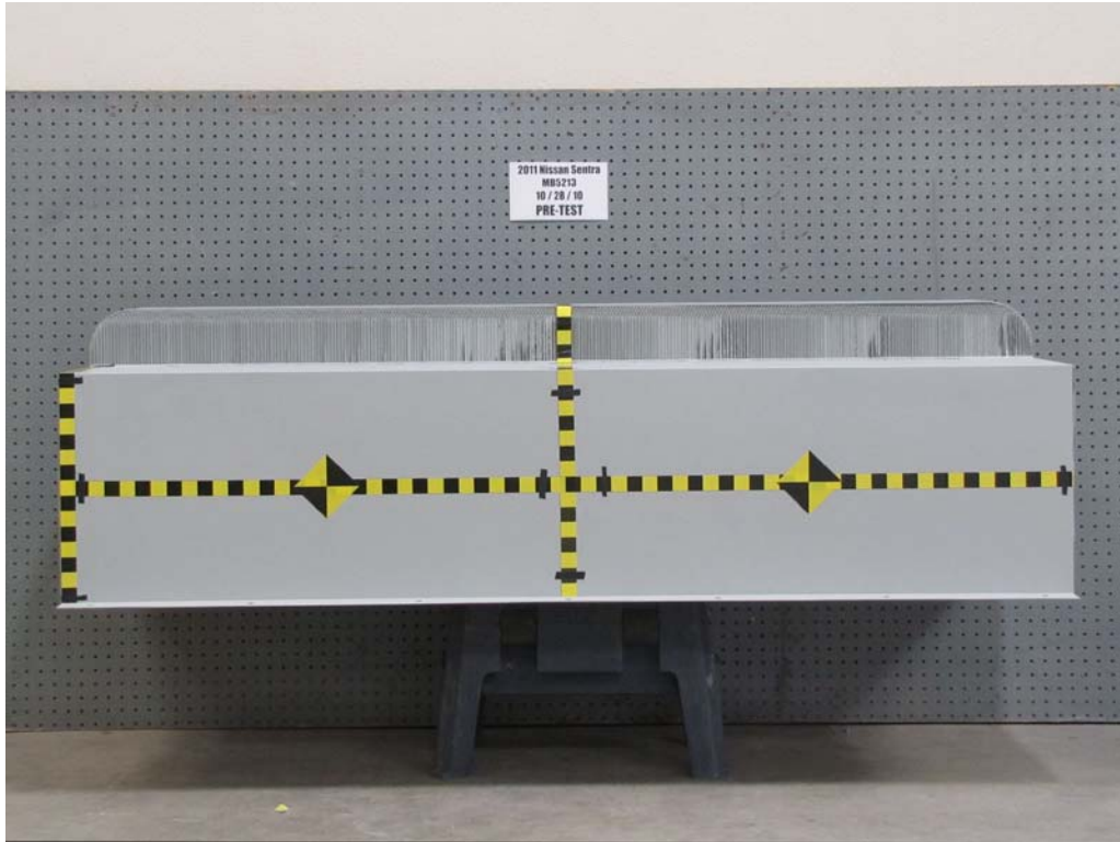
FIGURE 83. Pre-Test Top View of MDB Impactor Face
