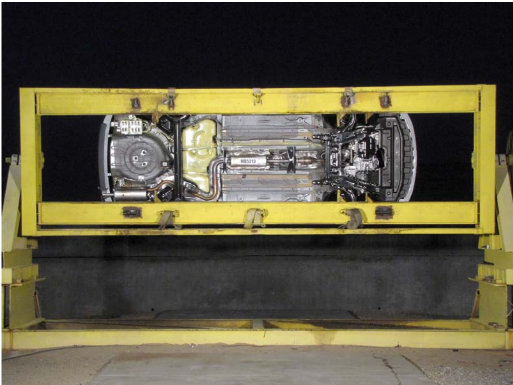
FIGURE 96. FMVSS No. 301/305 Rollover 270 Degrees
