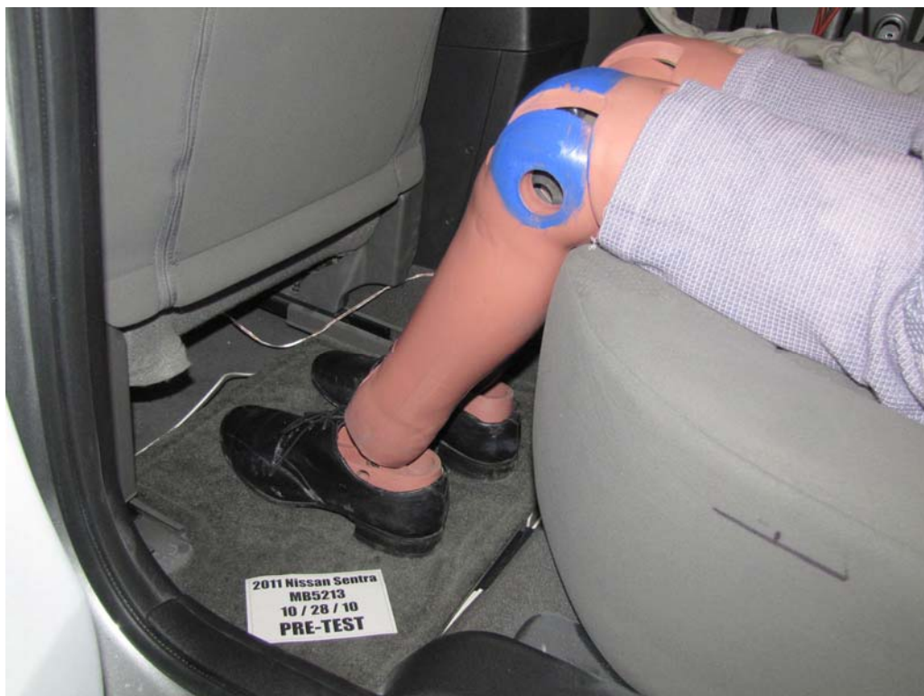
FIGURE 62. Pre-Test Placement of Rear Passenger Dummy's Feet
