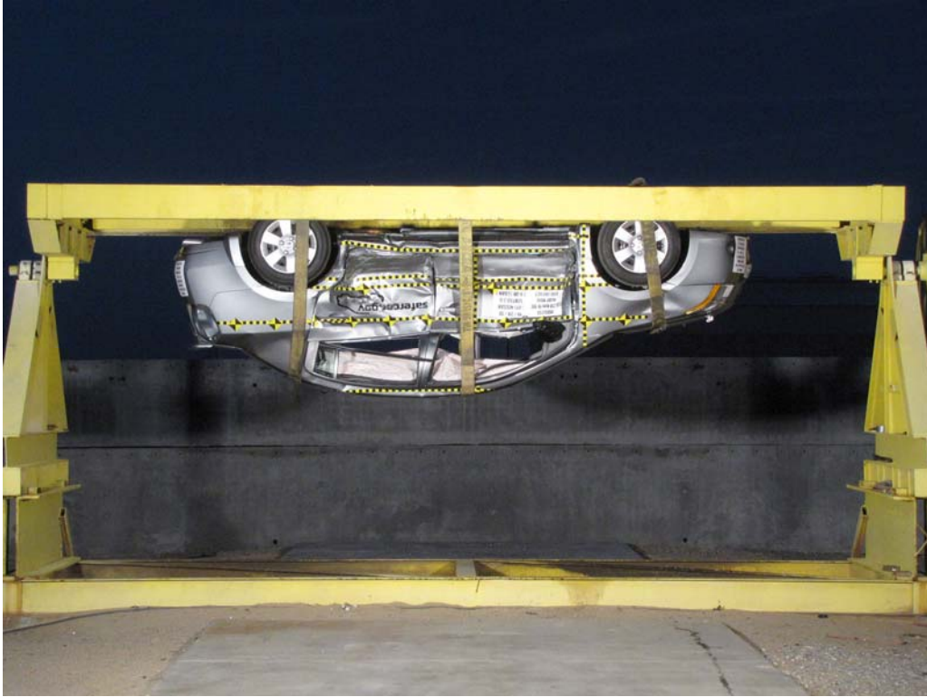
FIGURE 95. FMVSS No. 301/305 Rollover 180 Degrees
