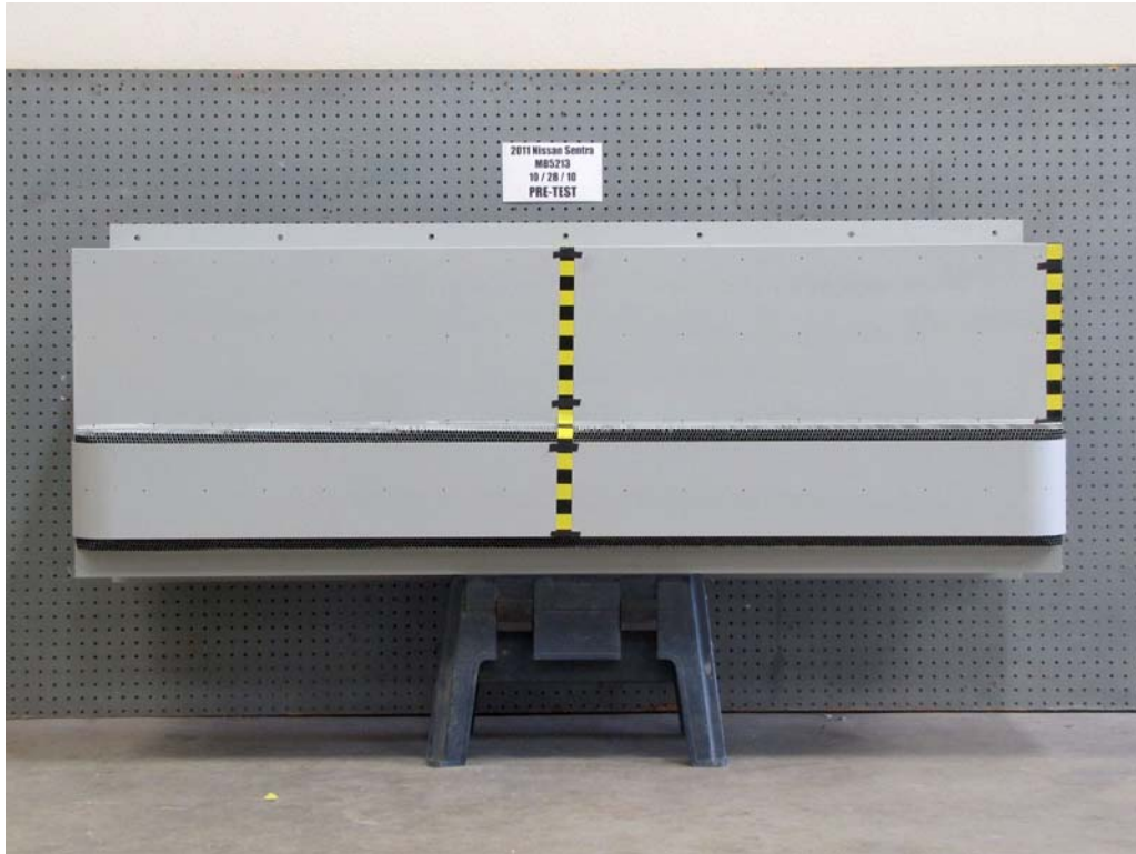
FIGURE 81. Pre-Test Front View of MDB Impactor Face
