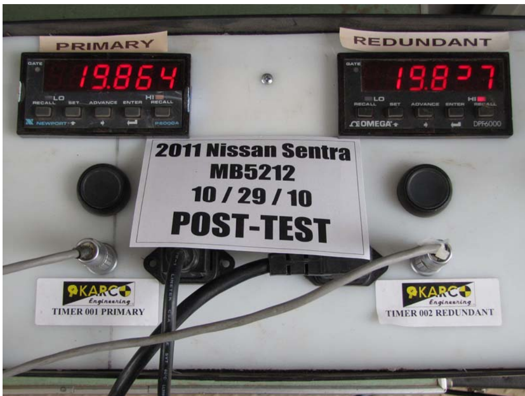
FIGURE 60. Post-Test Primary and Redundant Speed Trap Read-Out
