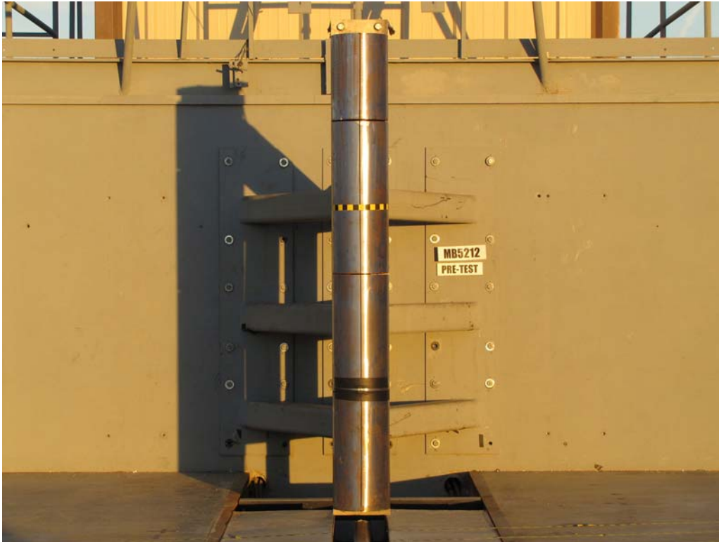
FIGURE 55. Pre-Test Pole Barrier Front View
