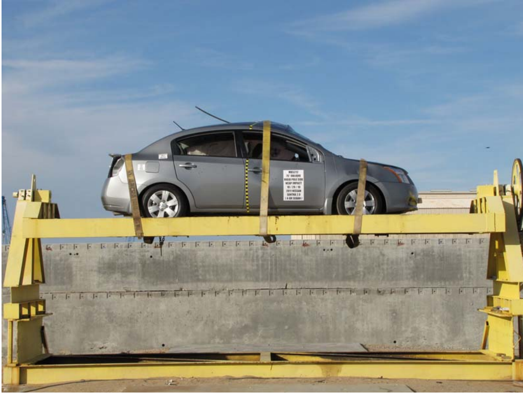
FIGURE 65. FMVSS No. 301-305 Rollover 360 Degrees
