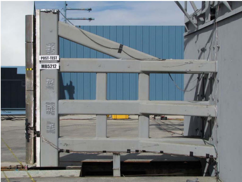
FIGURE 58. Post-Test Pole Barrier Side View
