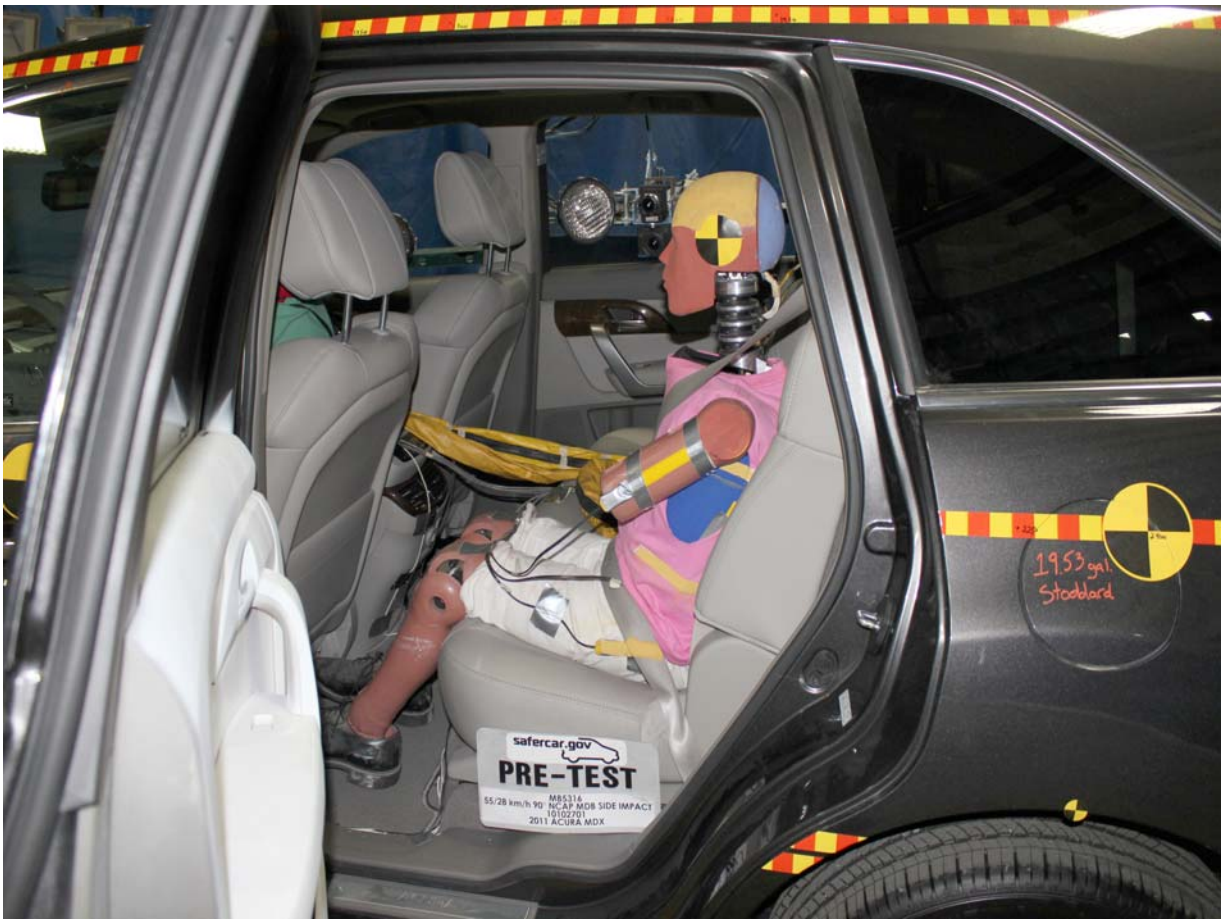
Pre-Test Left Side View of Passenger Dummy Showing Belt, Chalking, and Contact Switches
