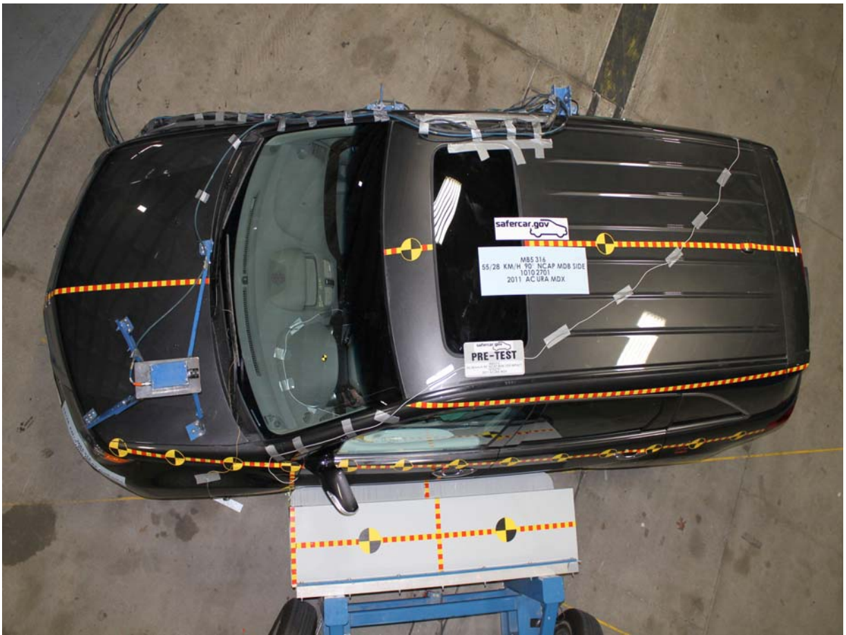
Pre-Test Overhead View of Test Vehicle with MDB Positioned Against Side of Test Vehicle
