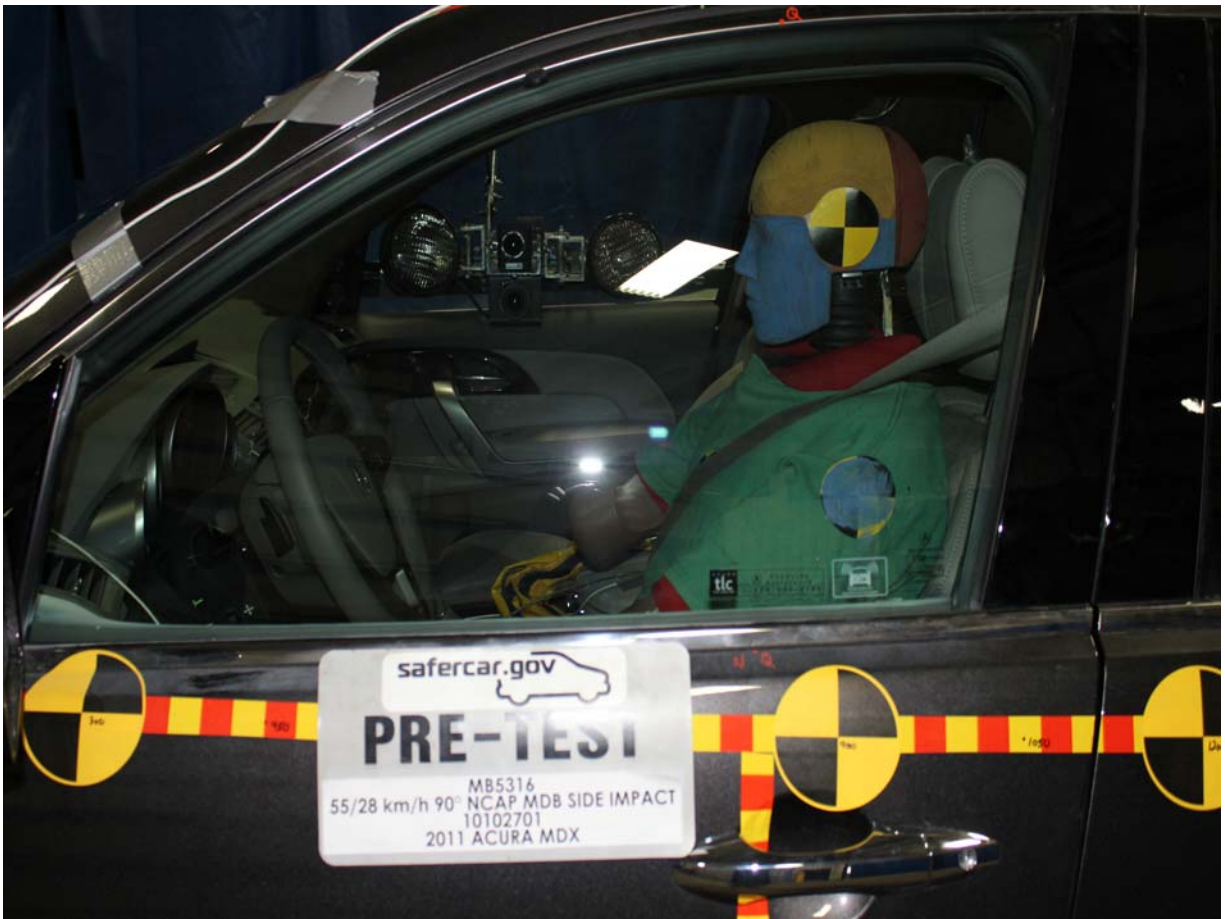
Pre-Test Left Side View of Driver Dummy Shoulder and Door Top View
