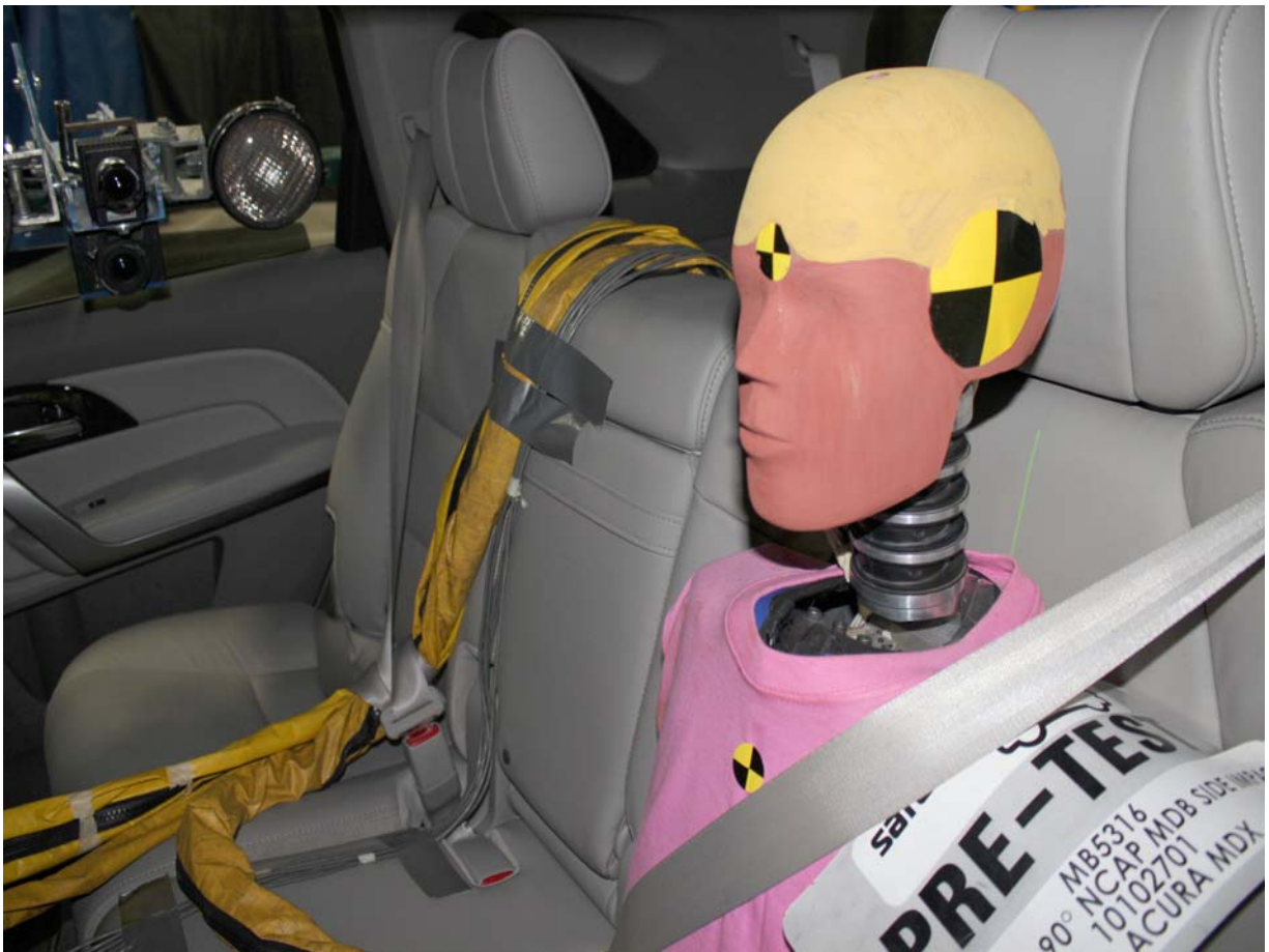
Pre-Test Close-Up Left Side View of Rear Passenger Seat Back or Head Restraint
