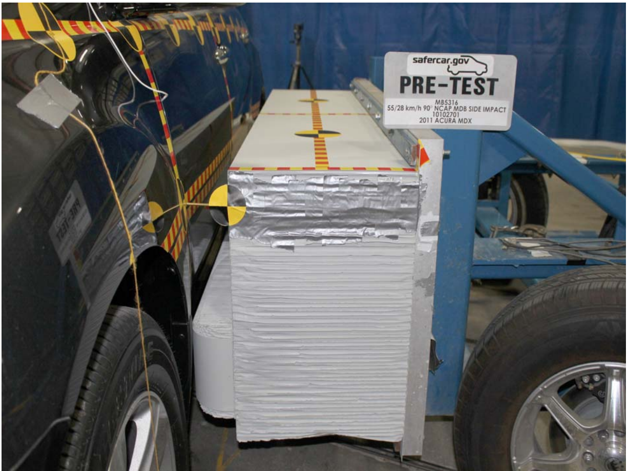
Pre-Test Left Side View of MDB Positioned Against Side of Test Vehicle
