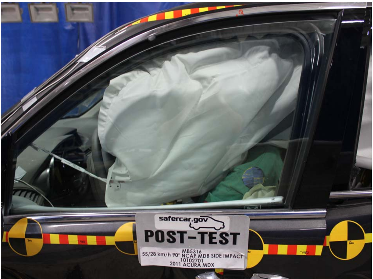
Post-Test Left Side View of Driver Dummy Shoulder and Door Top View
