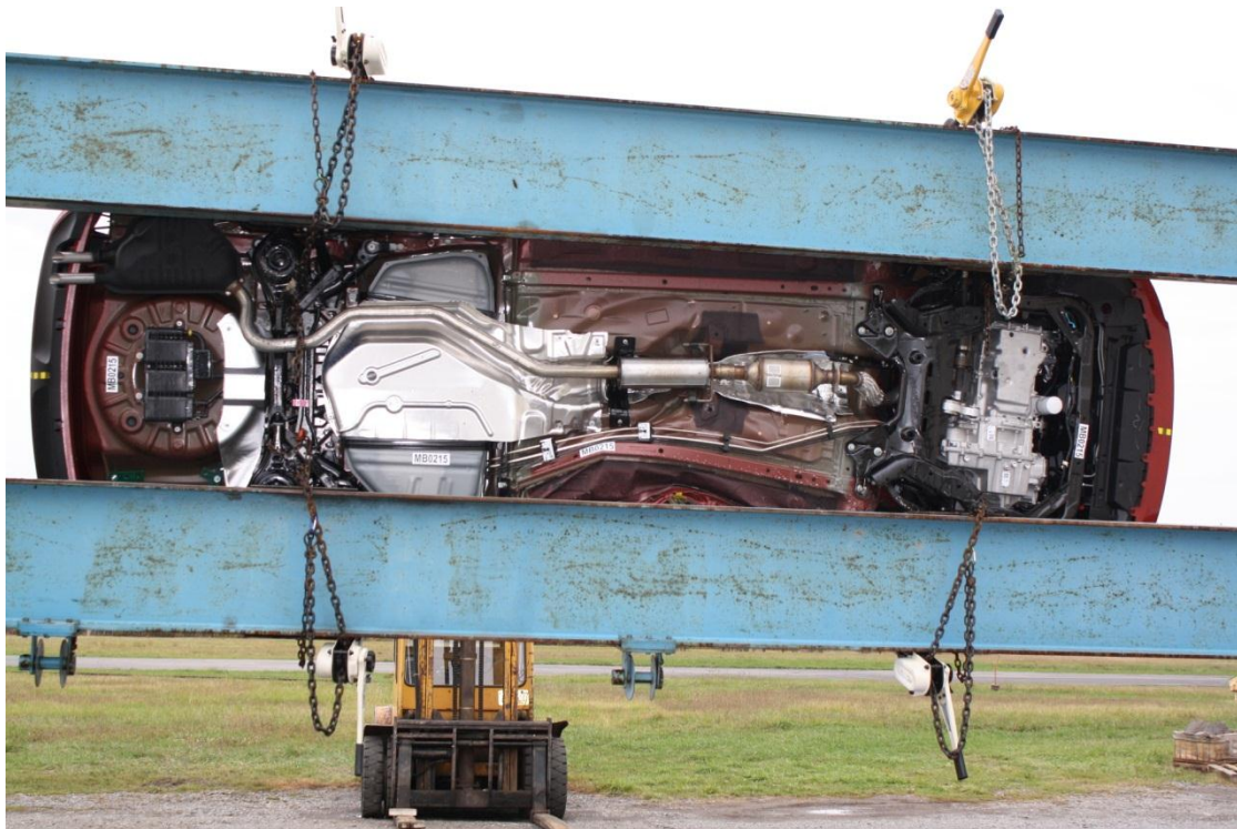
Figure A-62: FMVSS No. 301 Rollover 90°
