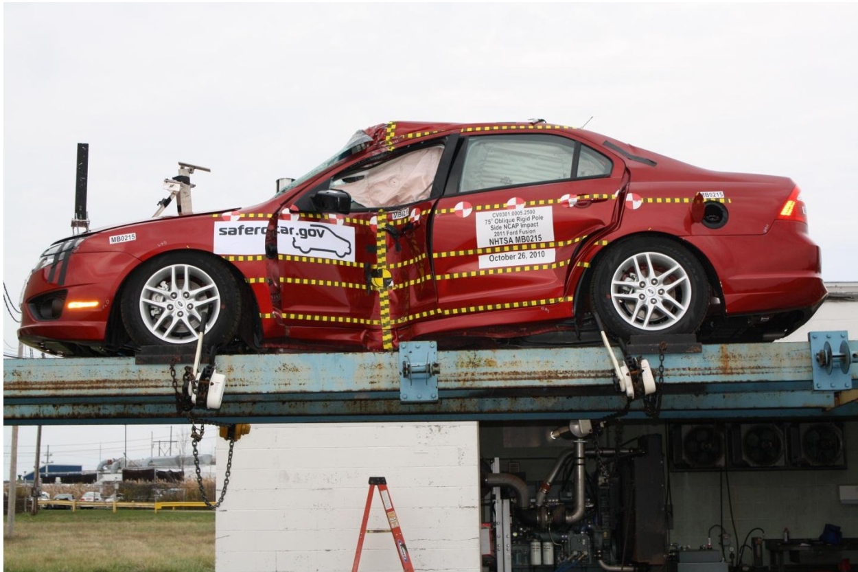
Figure A-65: FMVSS No. 301 Rollover 360°
