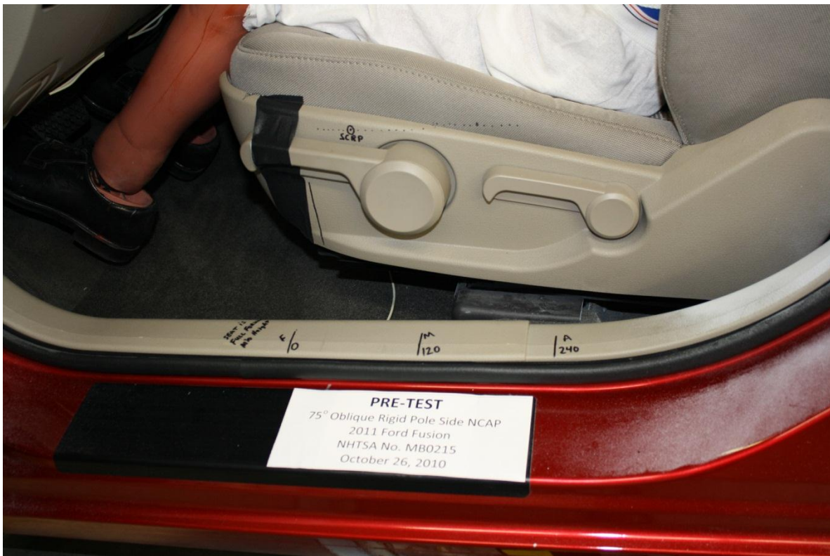
Figure A-36: Pre-Test Close-Up Left Side View of Driver Seat Track Showing Test Position
