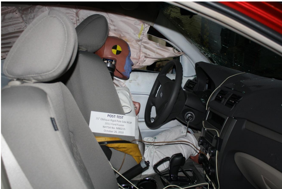
Figure A-42: Post-Test Right Side View of Dummy and Front Seat Occupant
