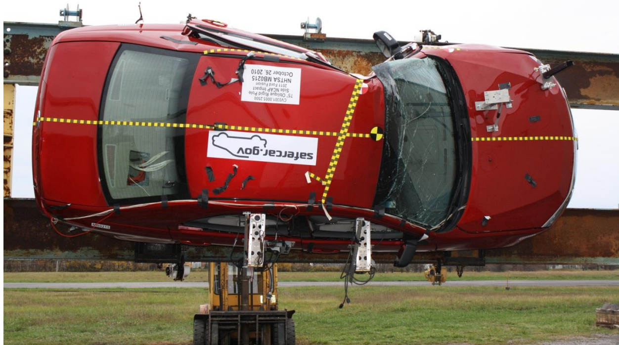
Figure A-64: FMVSS No. 301 Rollover 270°
