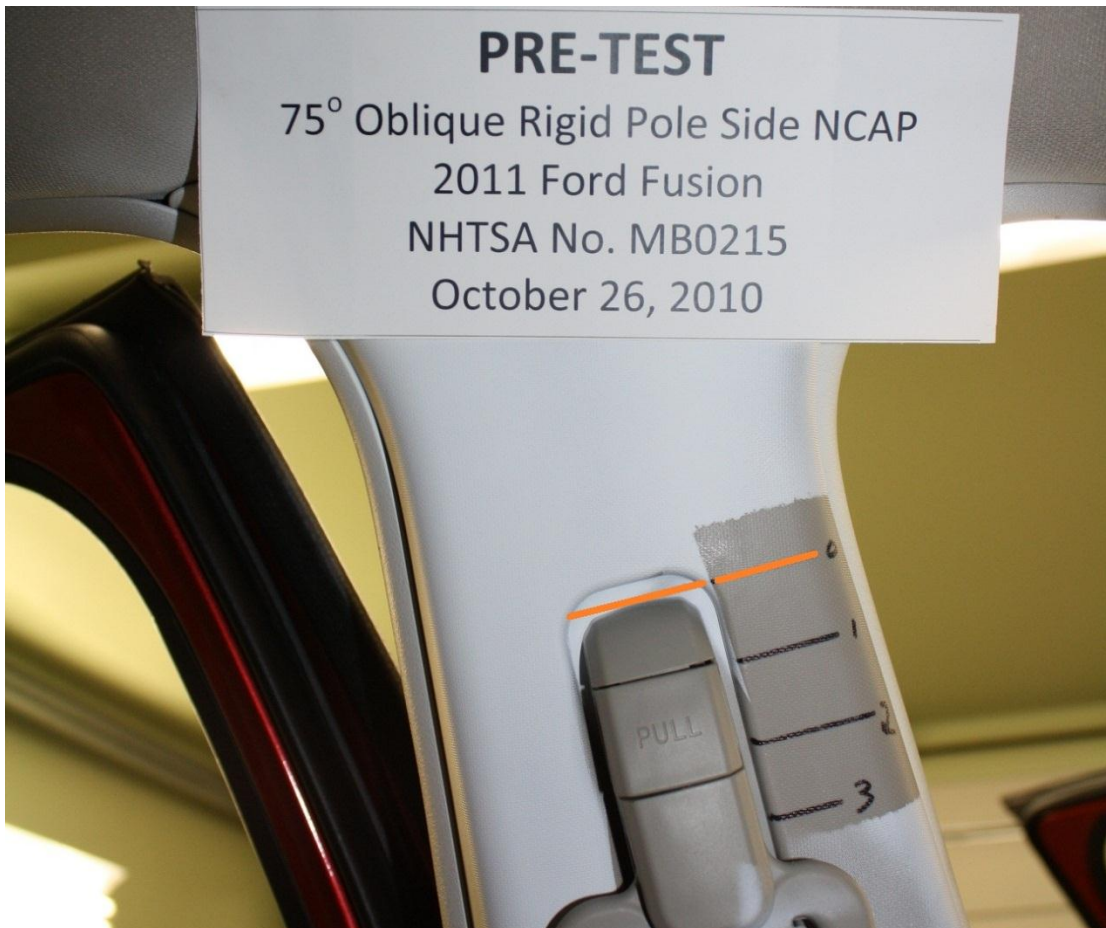
Figure A-33: Pre-Test View of Belt Anchorage for Dummy to Show Position
