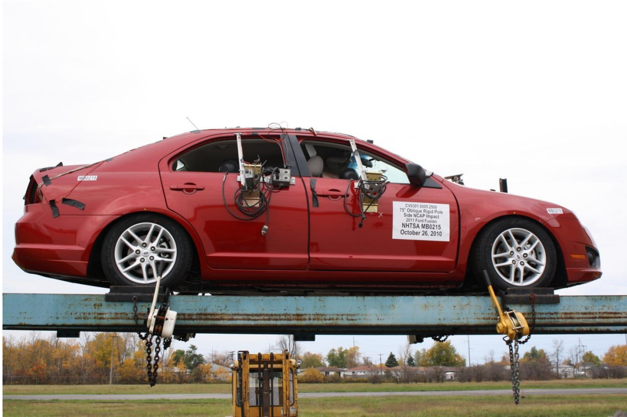
Figure A-61: FMVSS No. 301 Rollover 0°
