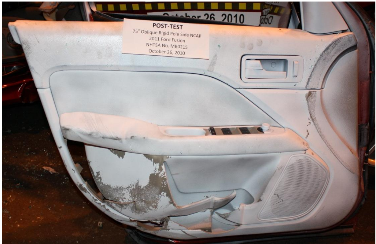
Figure A-44: Post-Test Inner Door Panel View Showing Dummy Contact Location
