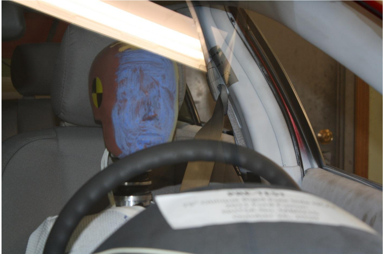
Figure A-27: Pre-Test Frontal View of Dummy Head and Shoulders in Relation to Head Restraint
