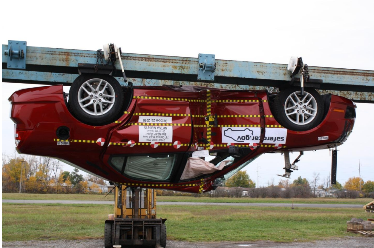
Figure A-63: FMVSS No. 301 Rollover 180°
