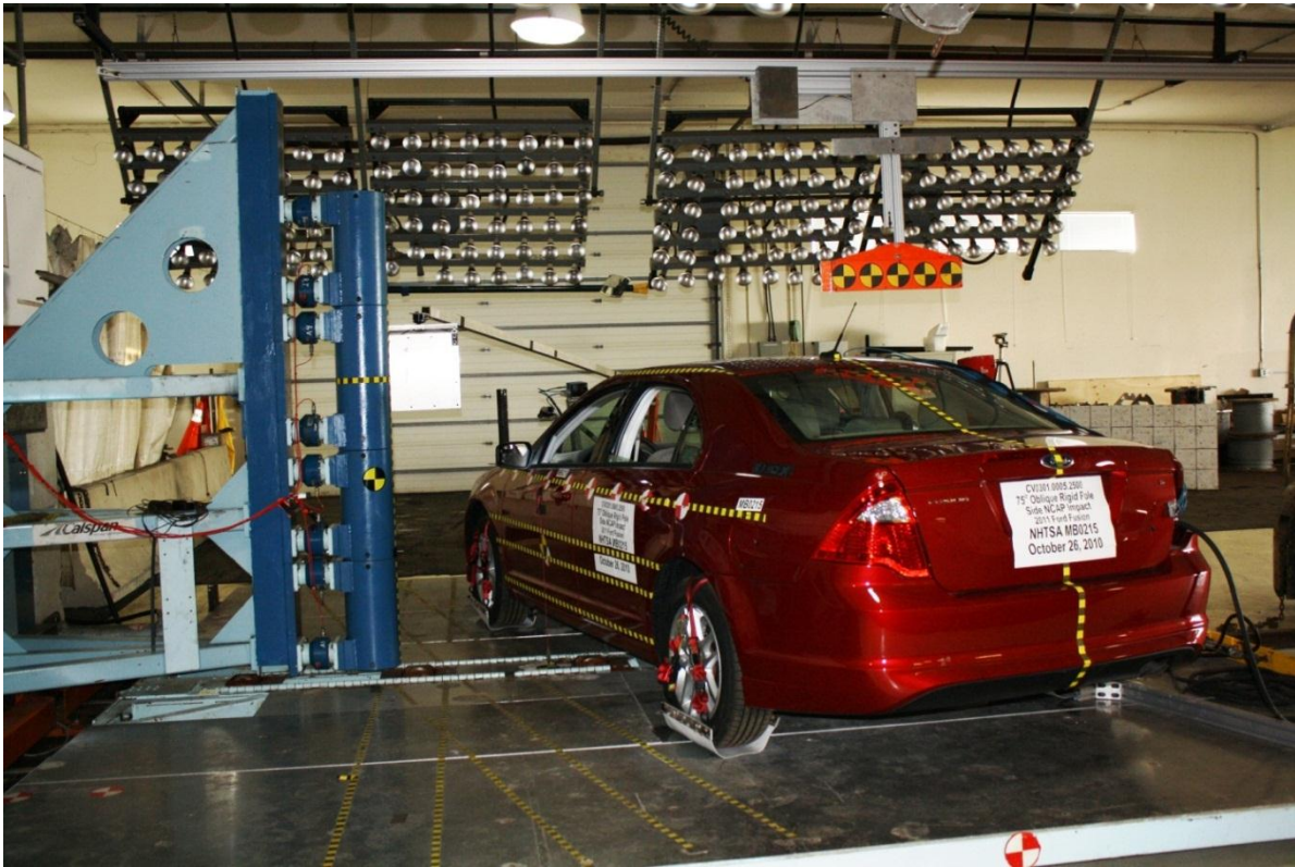
Figure A-17: Pre-Test Left Side View of Pole Positioned Against Side of Vehicle at Ideal Impact Point
